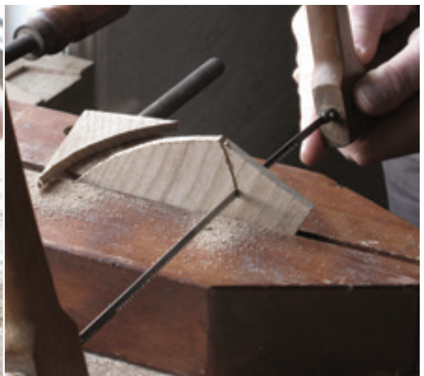
A scraper plane (left) is used to remove marks from the resawing, and using the frame saw again to shape the arch (above). John Lloyd is writing a piece on paring (below) for the next issue
