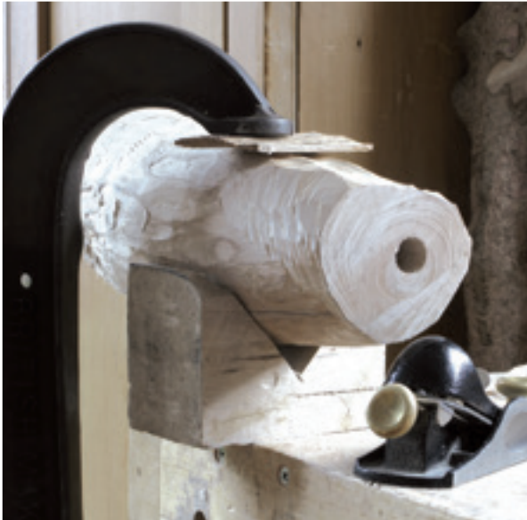
The base supported by the V-block while the top is planed (above). Pinched between a dog in the vice and the V-block (right and below right). Hand-held on the bench (below).
