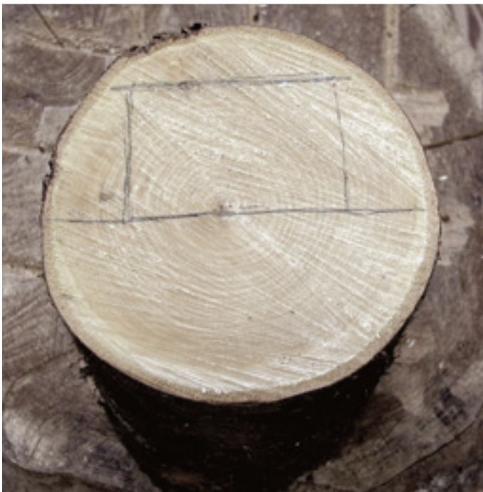
Drew marks up the section he wants to cleave from the log, making sure he avoids the pith, before splitting with a froe
