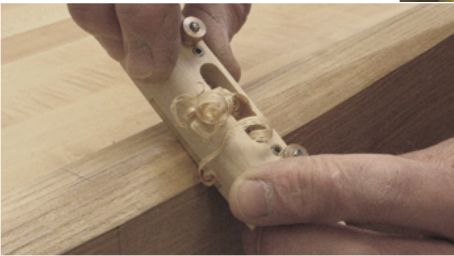
The adjustment mechanism differ between the two kits. The Windsor Workshop one (below) has grub screw adjusters already fitted to the Hock blade, which gives you a bit of a head start
