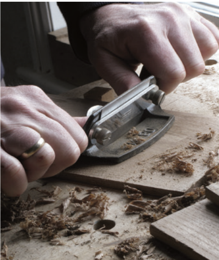
A scraper plane (left) is used to remove marks from the resawing, and using the frame saw again to shape the arch (above). John Lloyd is writing a piece on paring (below) for the next issue
