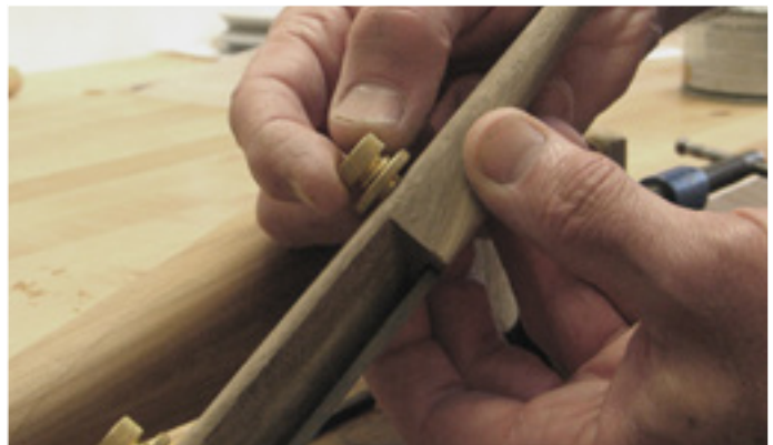
The adjustment mechanism differ between the two kits. The Windsor Workshop one (below) has grub screw adjusters already fitted to the Hock blade, which gives you a bit of a head start
