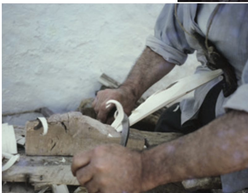
SHAVING HORSE In Spain Tatsuki Kuroda found a maker of Van Gogh chairs doing all his work on a shaving horse, with a curved 'push knife' that is also pulled when working on back splats and seat rails. Some of the shaping is done after the chair has been assembled
