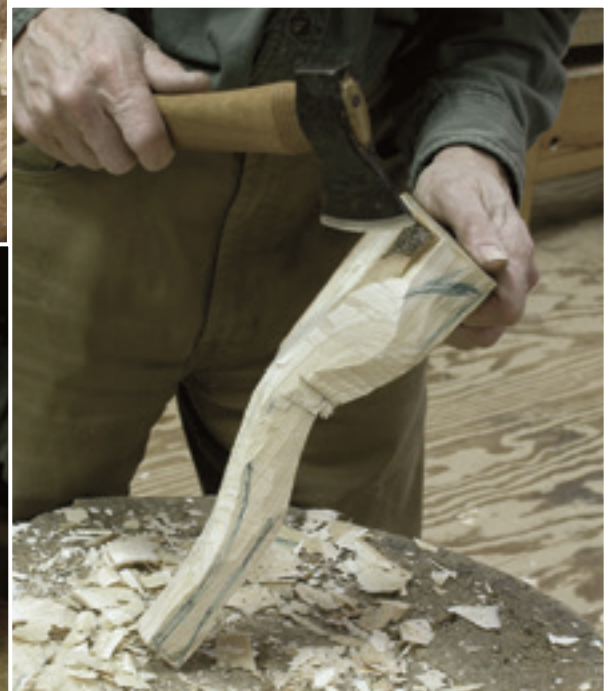
"Notice how the leading edge of the bowl," explains Drew, "starts about 40% below the top of the blank so that the spoon has a nice curve in profile." Drew uses a plastic ruler (left) which is clear so you can see both sides of the line to position it accurately. It is good to start hollowing the bowl when you can still clamp the blank securely (below left)
