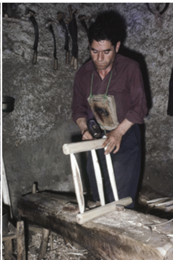
ORDER OF PRODUCTION On his journey to Granada and Guadex in Spain, Tatsuaki Kuroda found the makers assembling the front and back frames first, ready for attaching to one another with the side rails and then of course the seats being rushed
