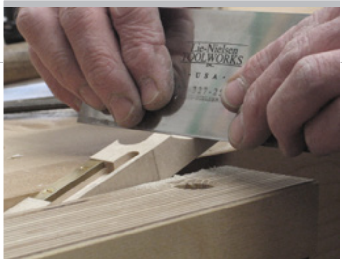
Rasps and cabinet scrapers are good for finishing the 'wings'. A section through the Windsor Workshop spokeshave shows how a rounded nose helps with shaping convex curves
