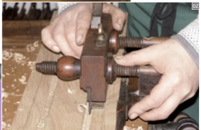
Richard starts by gluing a paper template to the end of each piece, scoring lines with a marking gauge. The plough plane (below) is used to form grooves for widening rebates
