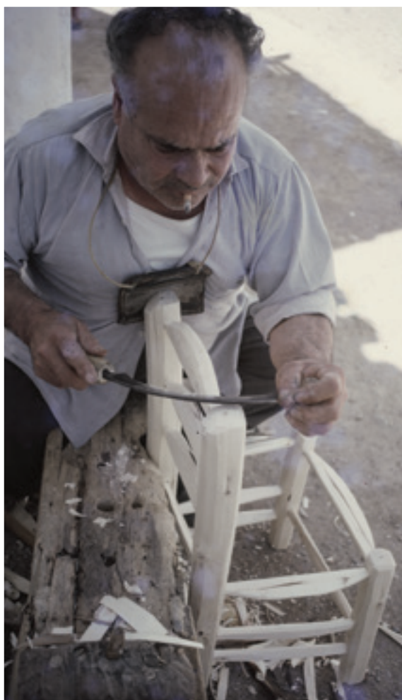
SHAVING HORSE In Spain Tatsuki Kuroda found a maker of Van Gogh chairs doing all his work on a shaving horse, with a curved 'push knife' that is also pulled when working on back splats and seat rails. Some of the shaping is done after the chair has been assembled
