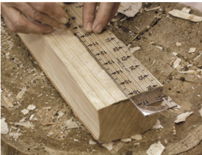
The finer work cleaning up the blank is done with a small axe, chopping away the bark. The hewing doesn't have to be particularly good at this stage
