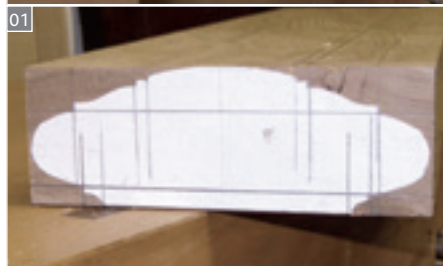
Richard starts by gluing a paper template to the end of each piece, scoring lines with a marking gauge. The plough plane (below) is used to form grooves for widening rebates
