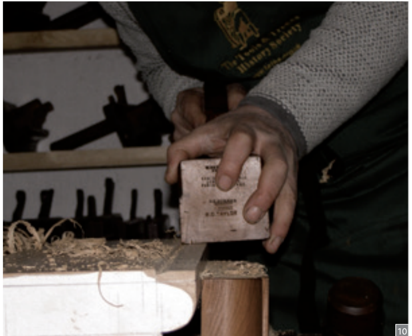
Using a large wooden badger plane to work the rebate (above) before using a small round for the cove (below), rounding with a wide hollow (Pic.12)
