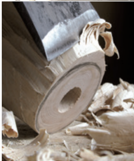
Hewing the top of the ash base to rough shape with a Gransfors Bruks carpenter's axe (above). While boring the flex hole the block was gripped in a V-block by a G-cramp (right)
