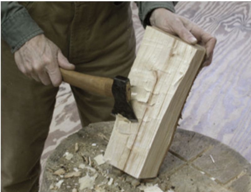
The finer work cleaning up the blank is done with a small axe, chopping away the bark. The hewing doesn't have to be particularly good at this stage
