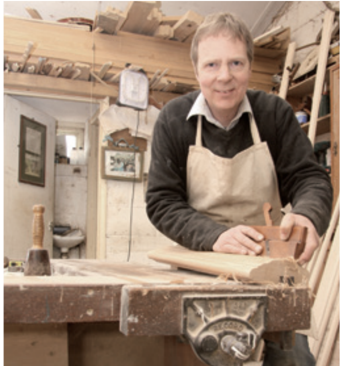
Richard starts by gluing a paper template to the end of each piece, scoring lines with a marking gauge. The plough plane (below) is used to form grooves for widening rebates
