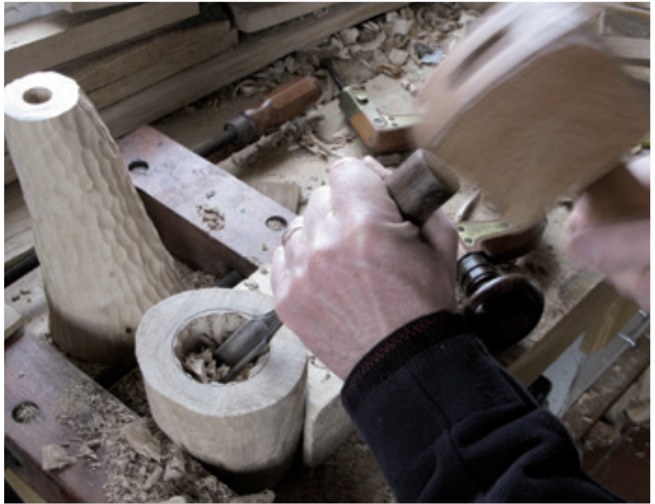
Boring out the middle of the elm shade with a brace and centre bit (left) before excavating waste using a gouge. The shade is gripped by the V-block in a handscrew (above). Smoothing end grain with a block plane (below)
