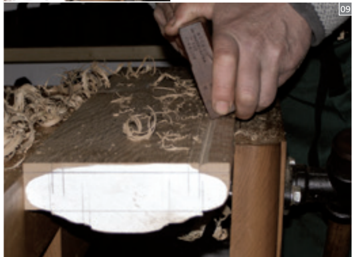
A jack plane (above) is a quick way to remove the waste on the edge, rounding the edge with a narrow hollow plane (left). Then Richard starts on the underside rebates (below)
