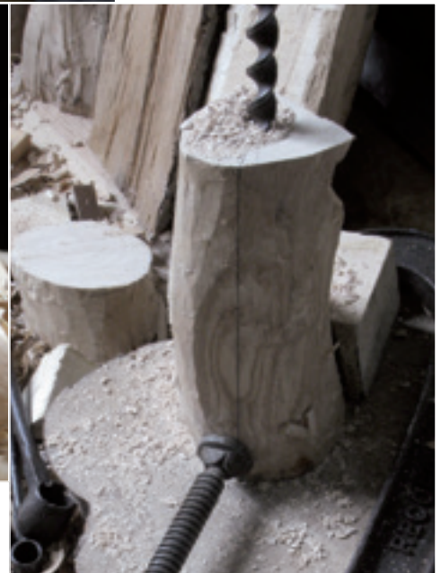
Hewing the top of the ash base to rough shape with a Gransfors Bruks carpenter's axe (above). While boring the flex hole the block was gripped in a V-block by a G-cramp (right)
