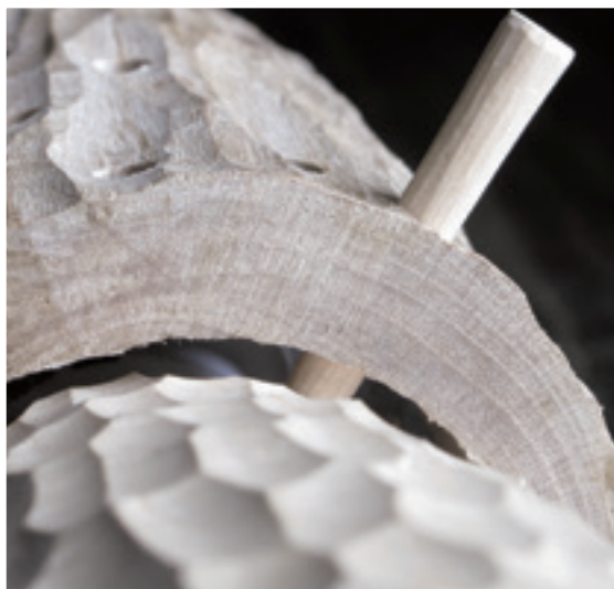
Boring random holes in the shade (above). Tapered hawthorn pins attach the shade to the base (below). In a cidery light (right)
