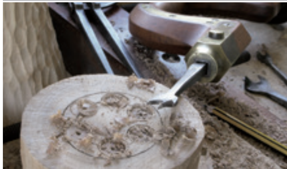
Boring out the middle of the elm shade with a brace and centre bit (left) before excavating waste using a gouge. The shade is gripped by the V-block in a handscrew (above). Smoothing end grain with a block plane (below)
