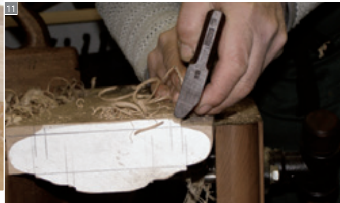
Using a large wooden badger plane to work the rebate (above) before using a small round for the cove (below), rounding with a wide hollow (Pic.12)
