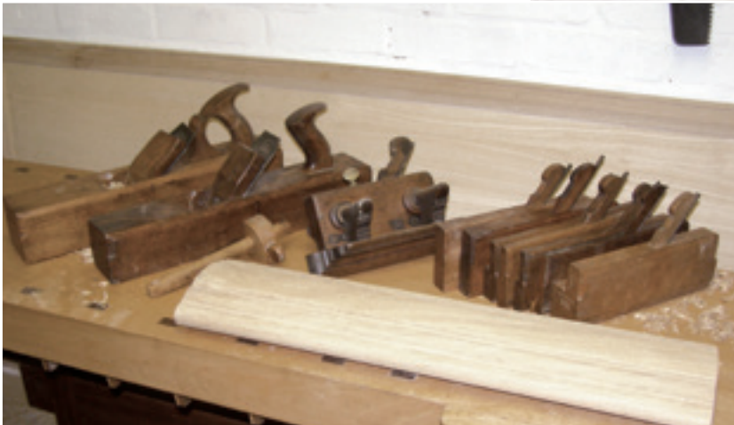
Tools used (from left): Badger rebate plane; jack plane; marking gauge; plough plane; snipe's bill and various hollows and rounds and rebate planes, made by different makers and from different sets. The oak was air-dried for easier use with old tools
