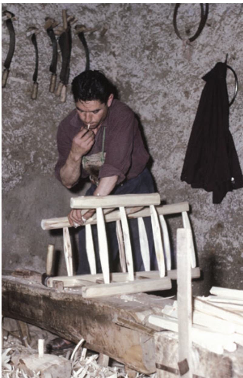
ORDER OF PRODUCTION On his journey to Granada and Guadex in Spain, Tatsuaki Kuroda found the makers assembling the front and back frames first, ready for attaching to one another with the side rails and then of course the seats being rushed
