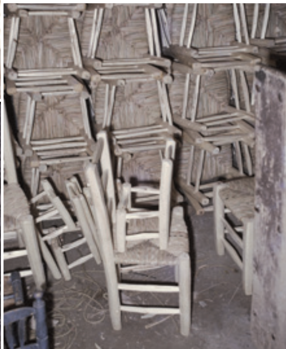
ORDER OF PRODUCTION On his journey to Granada and Guadex in Spain, Tatsuaki Kuroda found the makers assembling the front and back frames first, ready for attaching to one another with the side rails and then of course the seats being rushed
