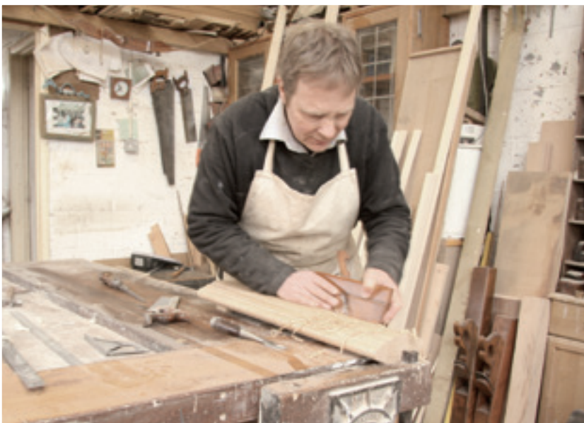
Tools used (from left): Badger rebate plane; jack plane; marking gauge; plough plane; snipe's bill and various hollows and rounds and rebate planes, made by different makers and from different sets. The oak was air-dried for easier use with old tools
