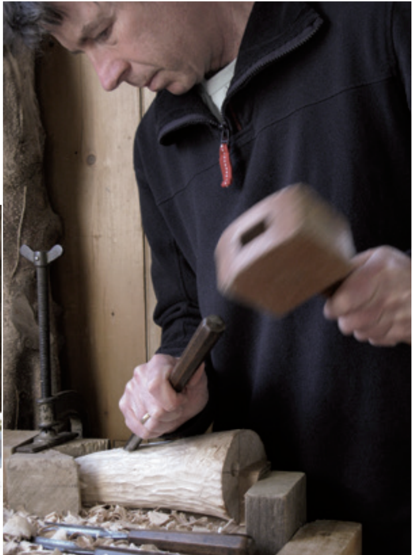
The base supported by the V-block while the top is planed (above). Pinched between a dog in the vice and the V-block (right and below right). Hand-held on the bench (below).
