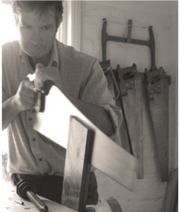
Working with a Disston 28in 41/2tpi rip saw. The design evolved over a few stages (below)
