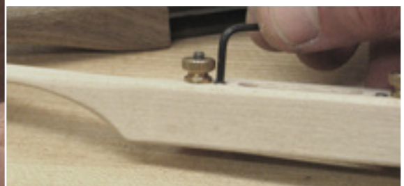
The adjustment mechanism differ between the two kits. The Windsor Workshop one (below) has grub screw adjusters already fitted to the Hock blade, which gives you a bit of a head start
