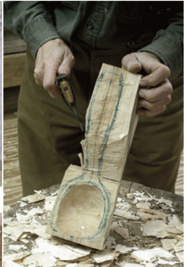
"Notice how the leading edge of the bowl," explains Drew, "starts about 40% below the top of the blank so that the spoon has a nice curve in profile." Drew uses a plastic ruler (left) which is clear so you can see both sides of the line to position it accurately. It is good to start hollowing the bowl when you can still clamp the blank securely (below left)
