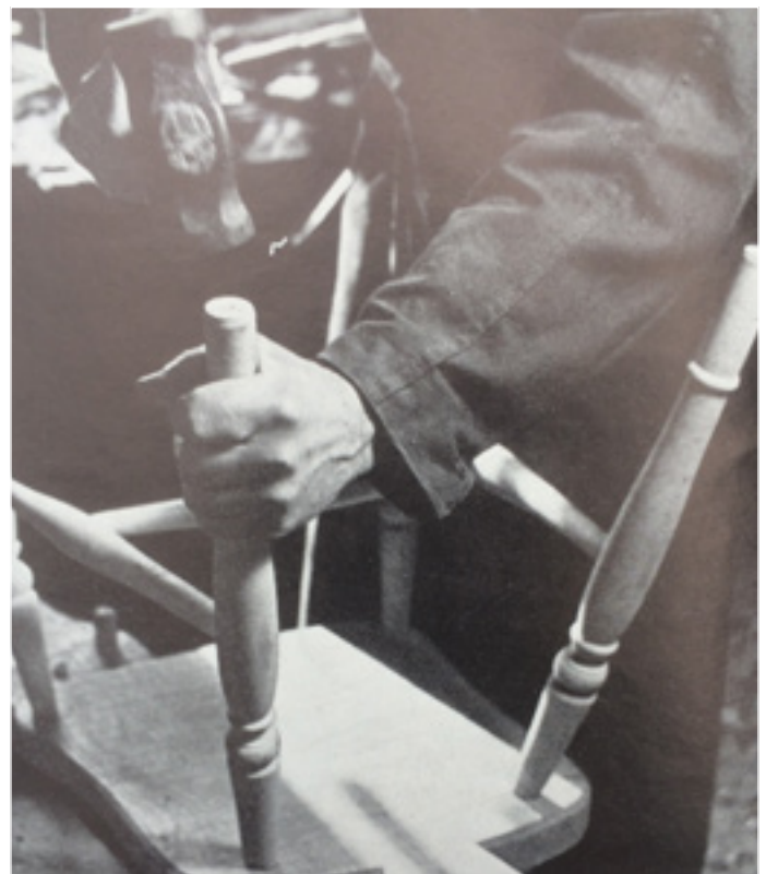
A framer's hammer was used for 'legging-up' a Windsor chair on a framing block
