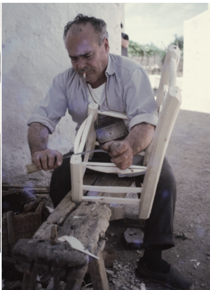
SHAVING HORSE In Spain Tatsuki Kuroda found a maker of Van Gogh chairs doing all his work on a shaving horse, with a curved 'push knife' that is also pulled when working on back splats and seat rails. Some of the shaping is done after the chair has been assembled
