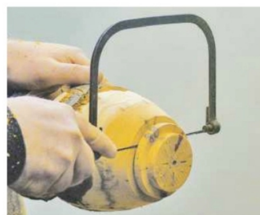
6. If you don't want to part it right off, use a coping saw to complete the cut
