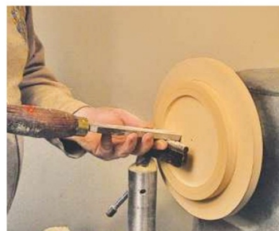
4. Cut a 6mm deep recess with a square-ended scraper to act as a jam chuck for the trivet blank
