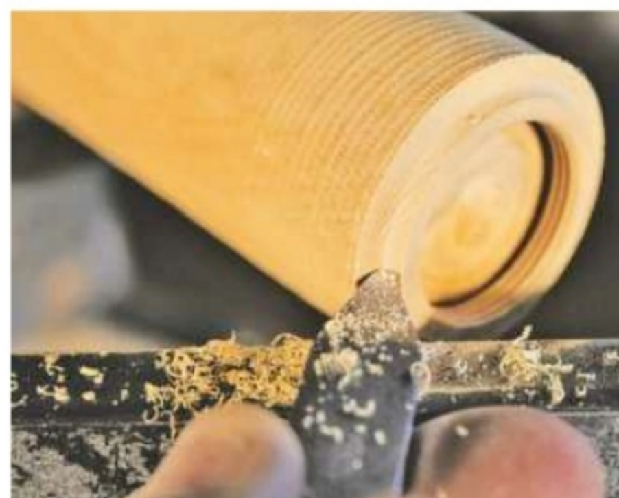
9. Form the small concave moulding on the edge of the lid with a scraper
