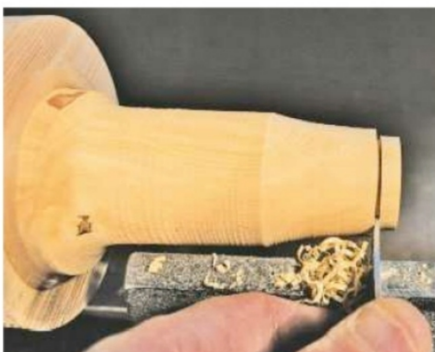
11. As before, cut an end space on the case for the chaser to run into
