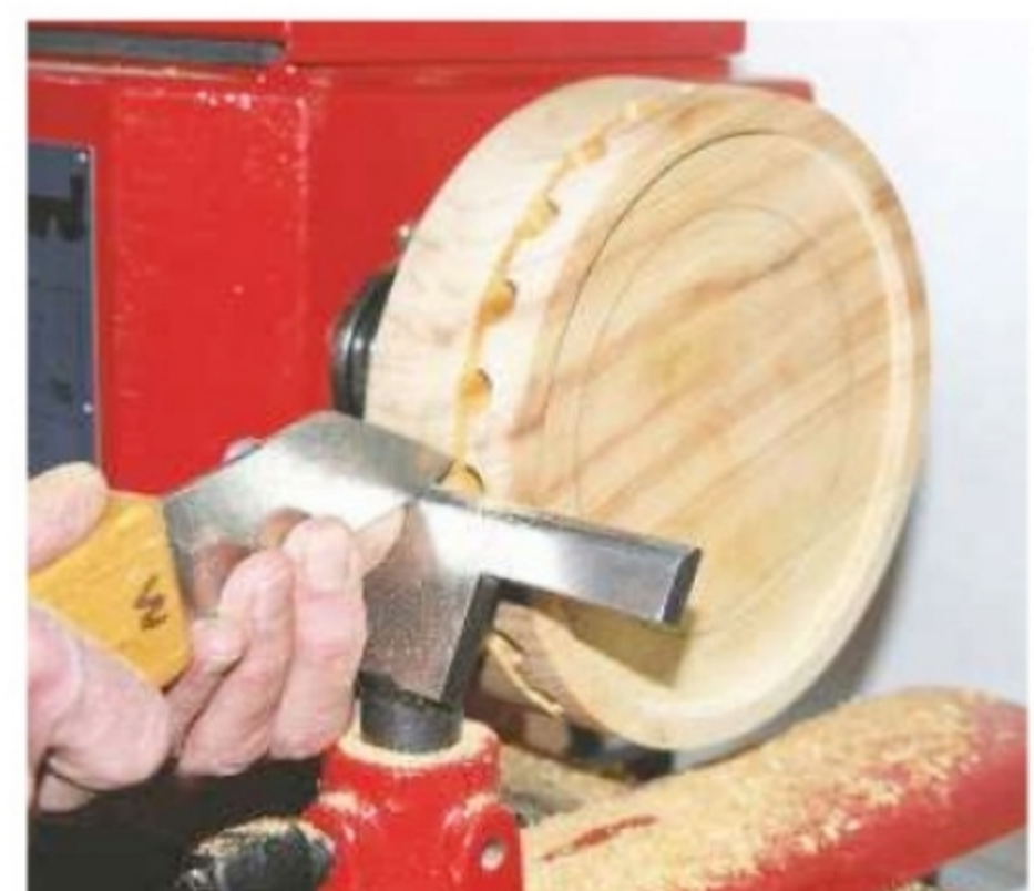
4. Cut into the edge of the blank to a depth of about 30mm
