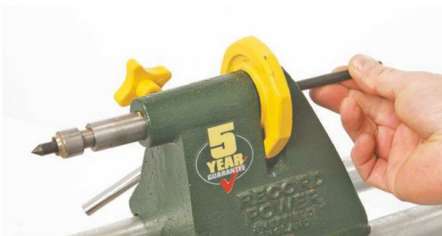
6. Fit the hollow centre and feed in the centring bar to provide a locating point for the blank
