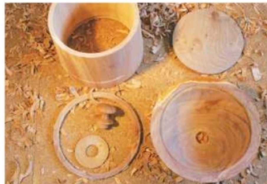
20. The components are now ready for assembly. Note the two ring templates
