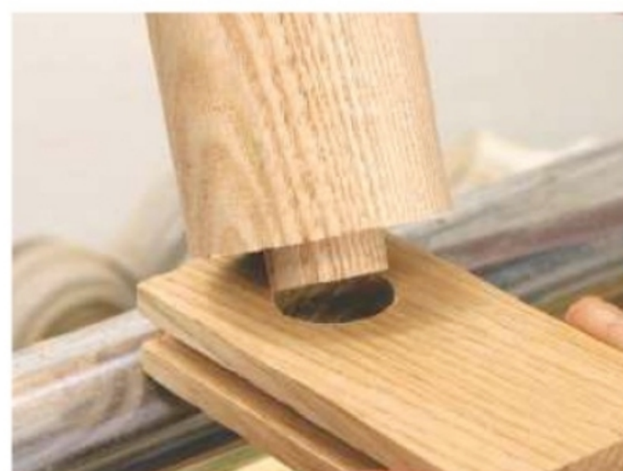
22. To check the spigot size, make up a test gauge from a piece of scrap wood
