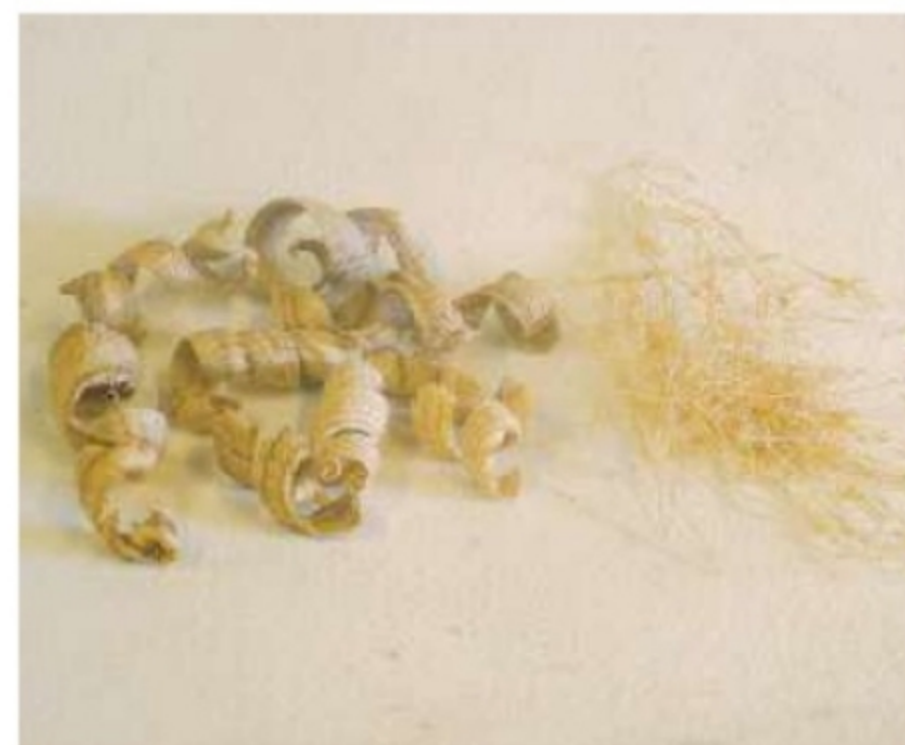
6. Rough-cut shavings are thick, while finishing-cut ones are fine wisps
