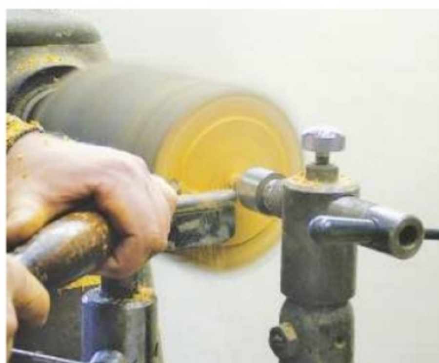
1. Mount the log between centres, true it up and cut a spigot on each end
