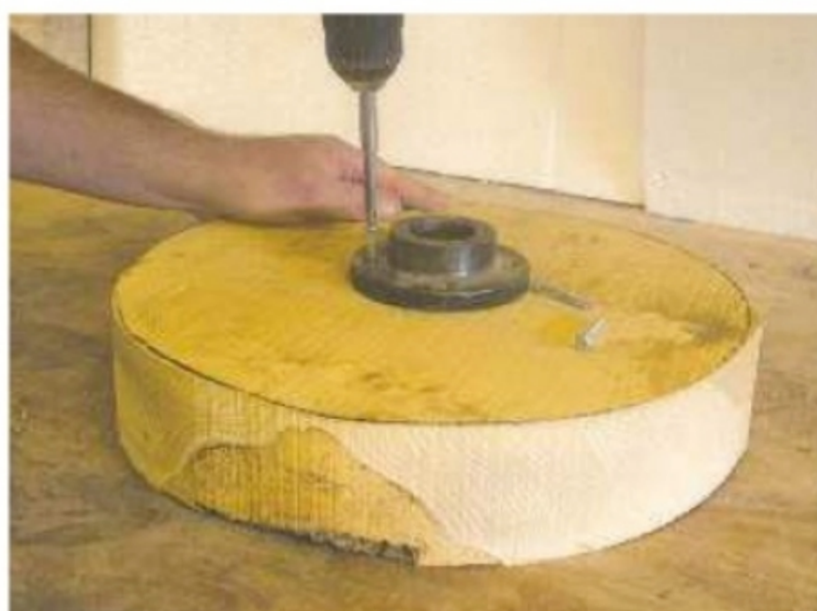
1. Cut the blank for the bowl to round and attach a faceplate
