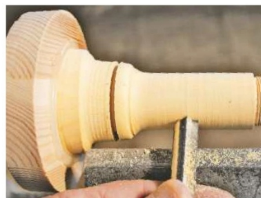
18. Turn the outside shape of the case and add its mouldings and details
