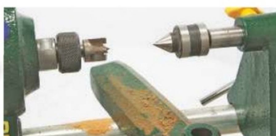
2. Mount the lamp stem blank between centres as normal
