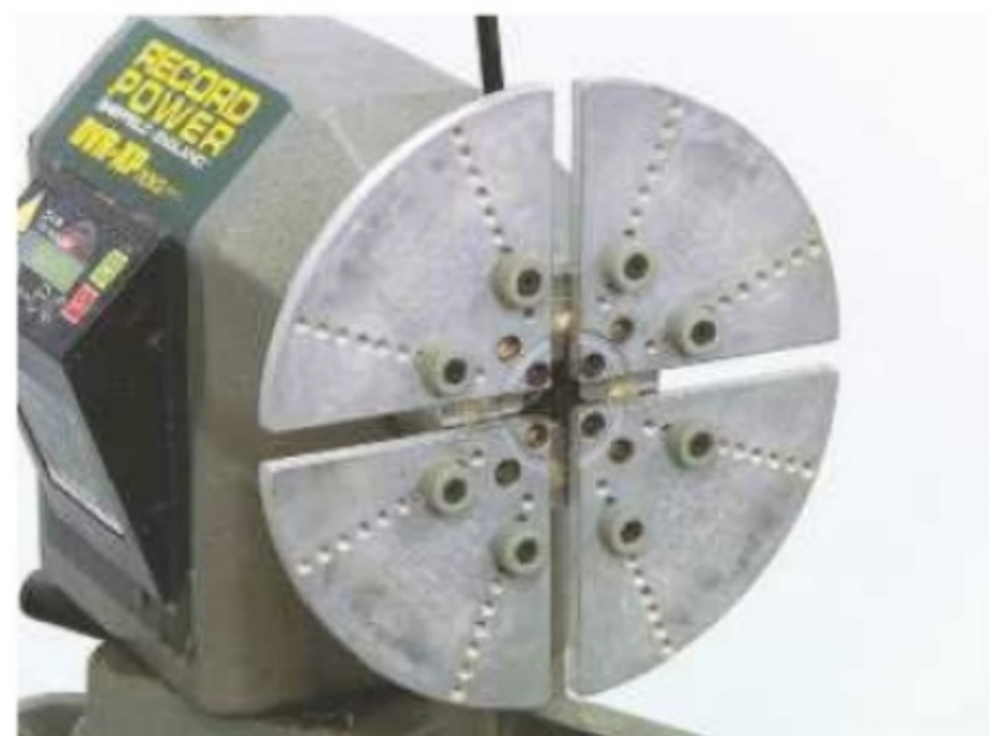
17. Remount the bowl using a combination chuck with large bowl jaws
