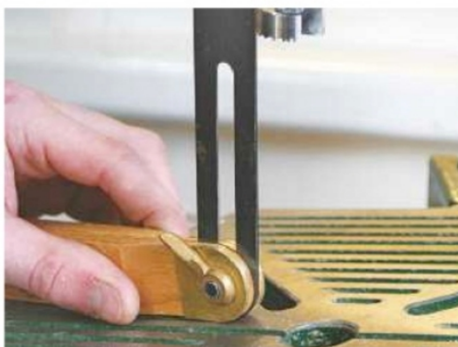
9. Use a sliding bevel to experiment with the splay angle
