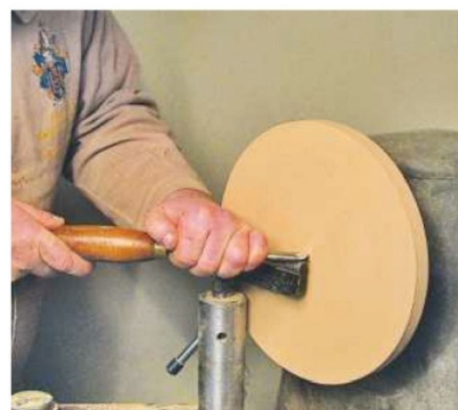
2. True up the larger circle of MDF and mark its precise centre with a skew chisel
