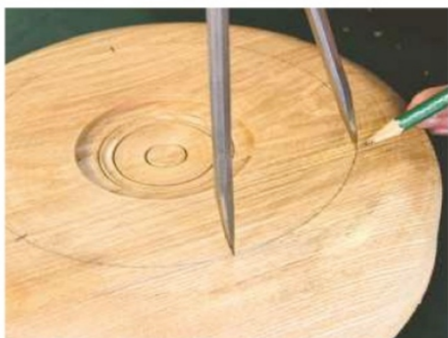
8. Use your dividers to mark six equal steps round the perimeter of the circle
