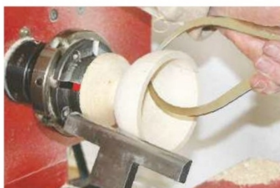
6. Check the wall thickness with callipers; aim for an even 8mm all round
