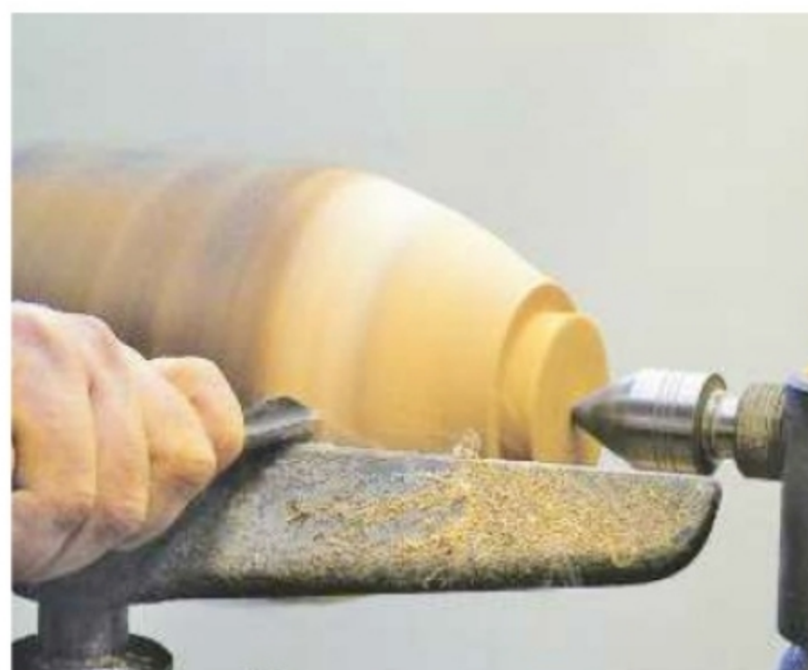
2. Mount the top of the vase in a chuck and start shaping the body using a spindle gouge
