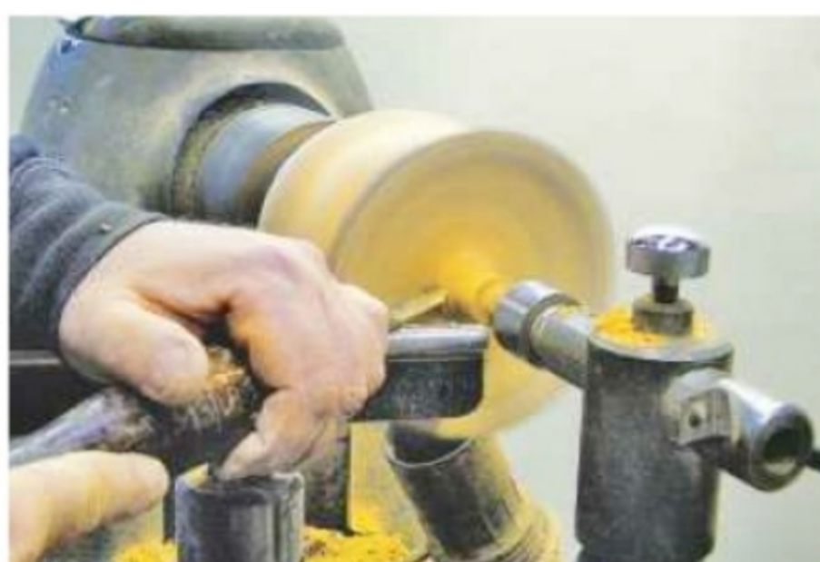
17. Use a \frac{3}{8} in spindle gouge to tidy up the vase rim and reduce the spigot
