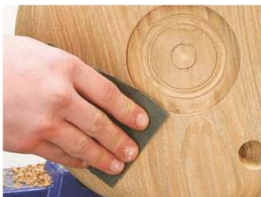
14. Put the disc back on the lathe so you can sand and polish it. Mind the holes with your fingers
