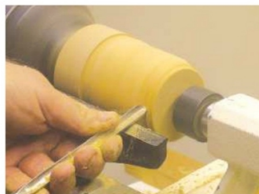
4. Start shaping the top of the apple using a 3/8in spindle gouge
