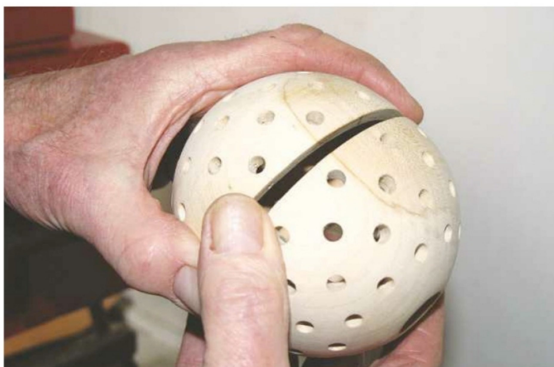
11. Match the grain carefully and offset the holes in the second half
