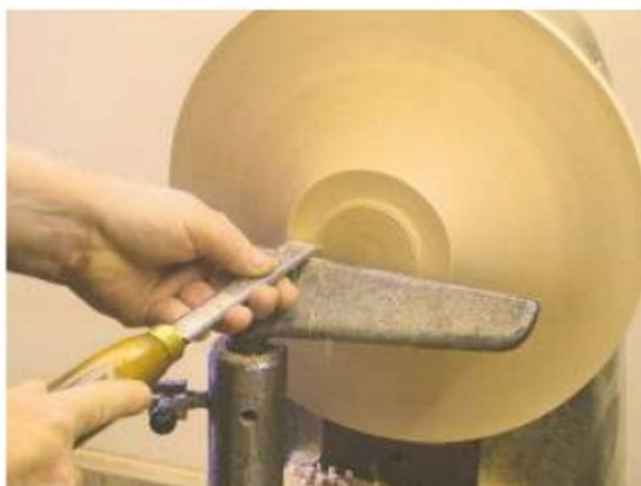
8. Clean up the chucking spigot with a skew chisel on its side
