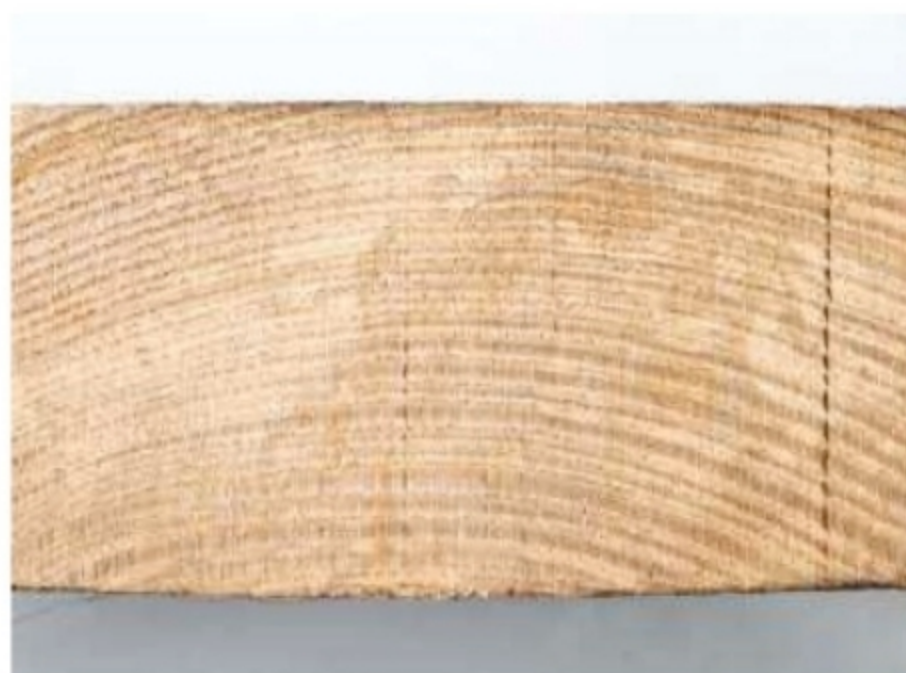
2. Try to avoid choosing wood for the top with cupped rings, which will distort over time
