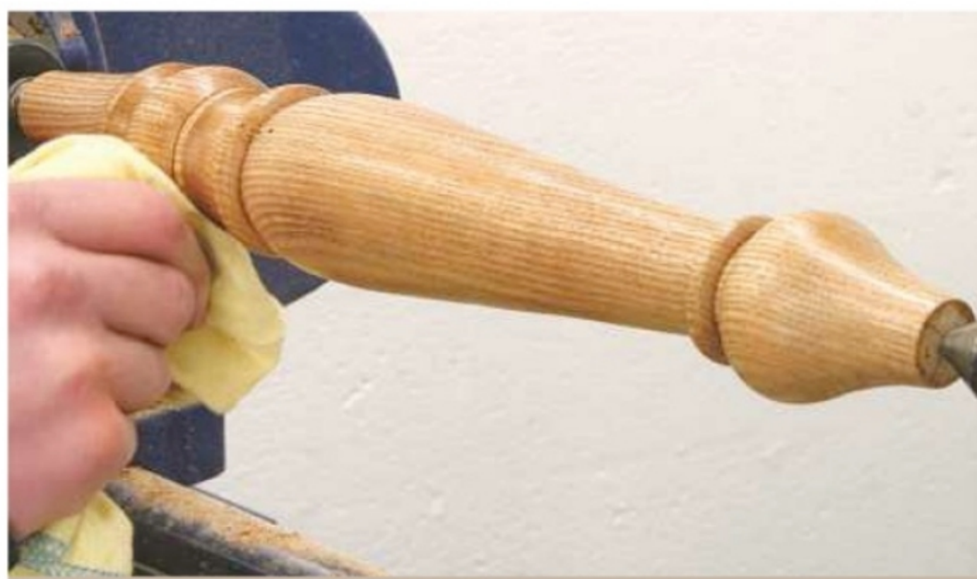
26. Use the same sealer and pastewax mixture you applied to the seat to polish the leg
