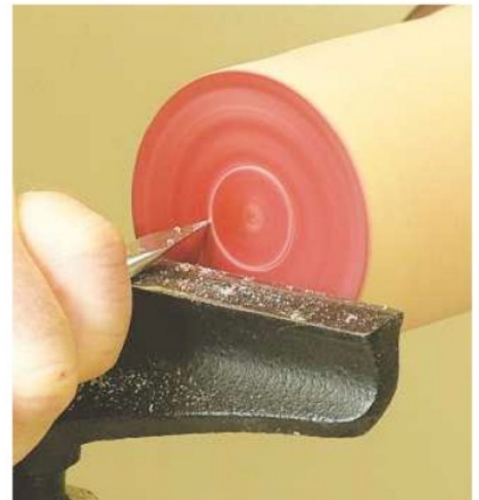
5. This effect can be enhanced by applying some colour to the wood and by incising a few V grooves with the optional point tool
