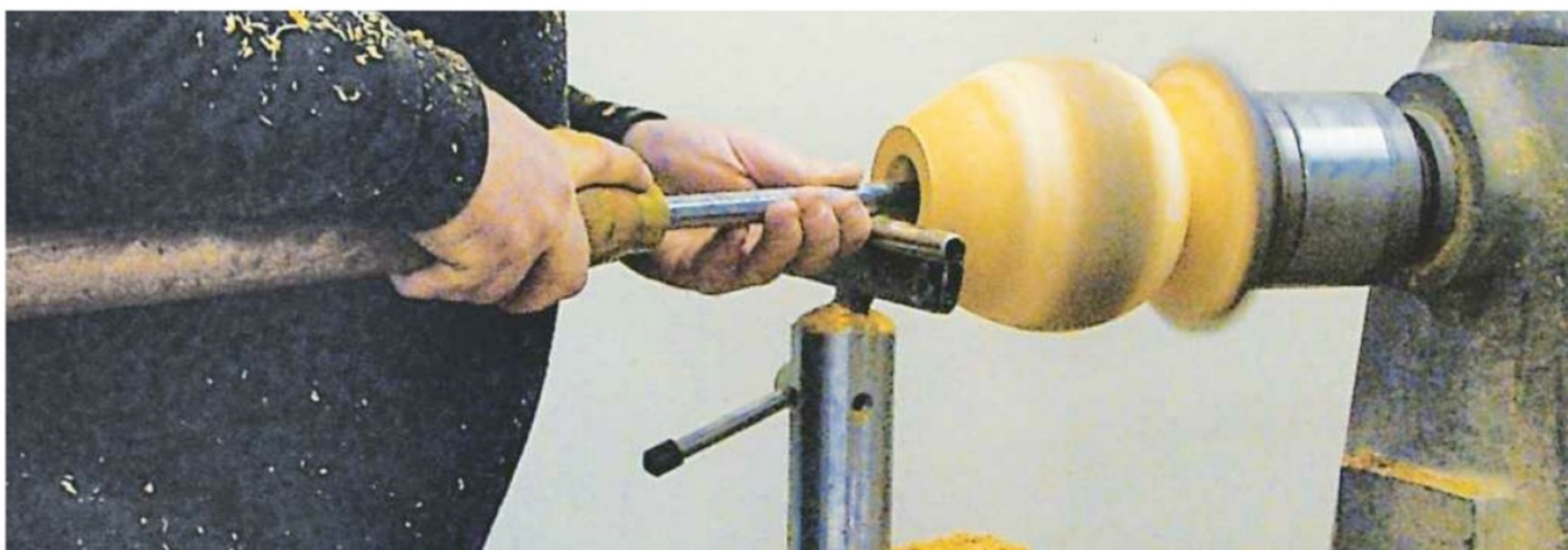
10. This upright stance helps avoid backache. My forearm is resting on top of the tool's handle
