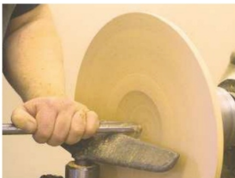
11. Then swing the tool handle towards you and rotate the flute up
