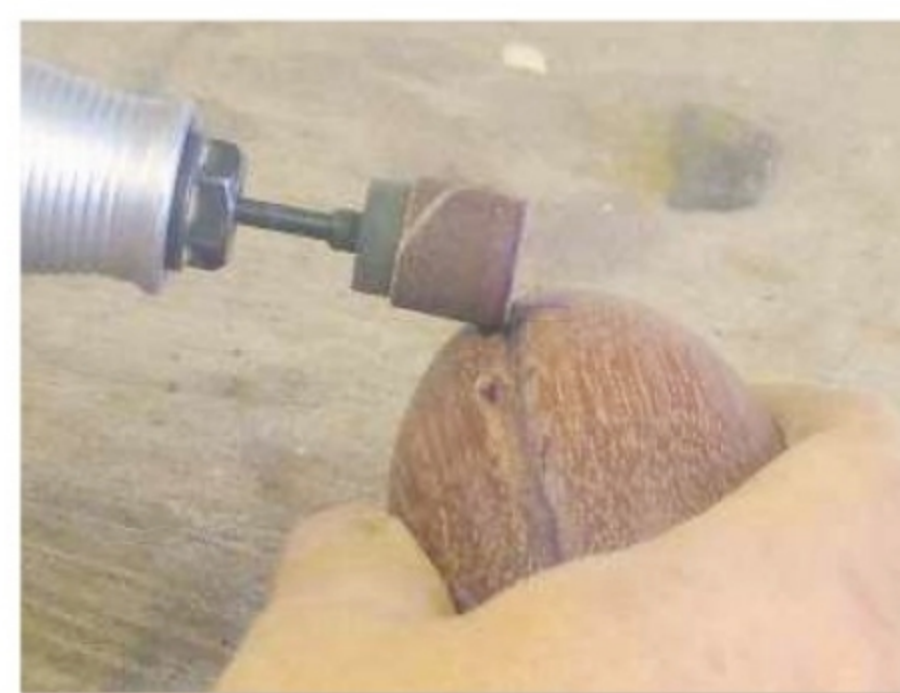
19. Create the groove common in plums with a sanding drum on a flexible shaft
