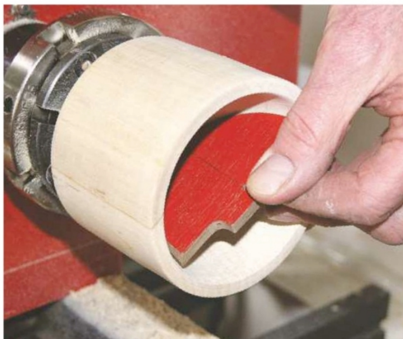
3. Check the progression of the inside curve with your internal template (see the panel below) as you proceed
