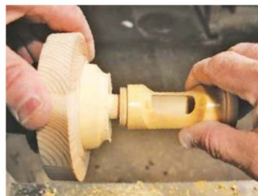
24. ...turn it down to form a slim mandrel chuck. Then jam the case onto it
