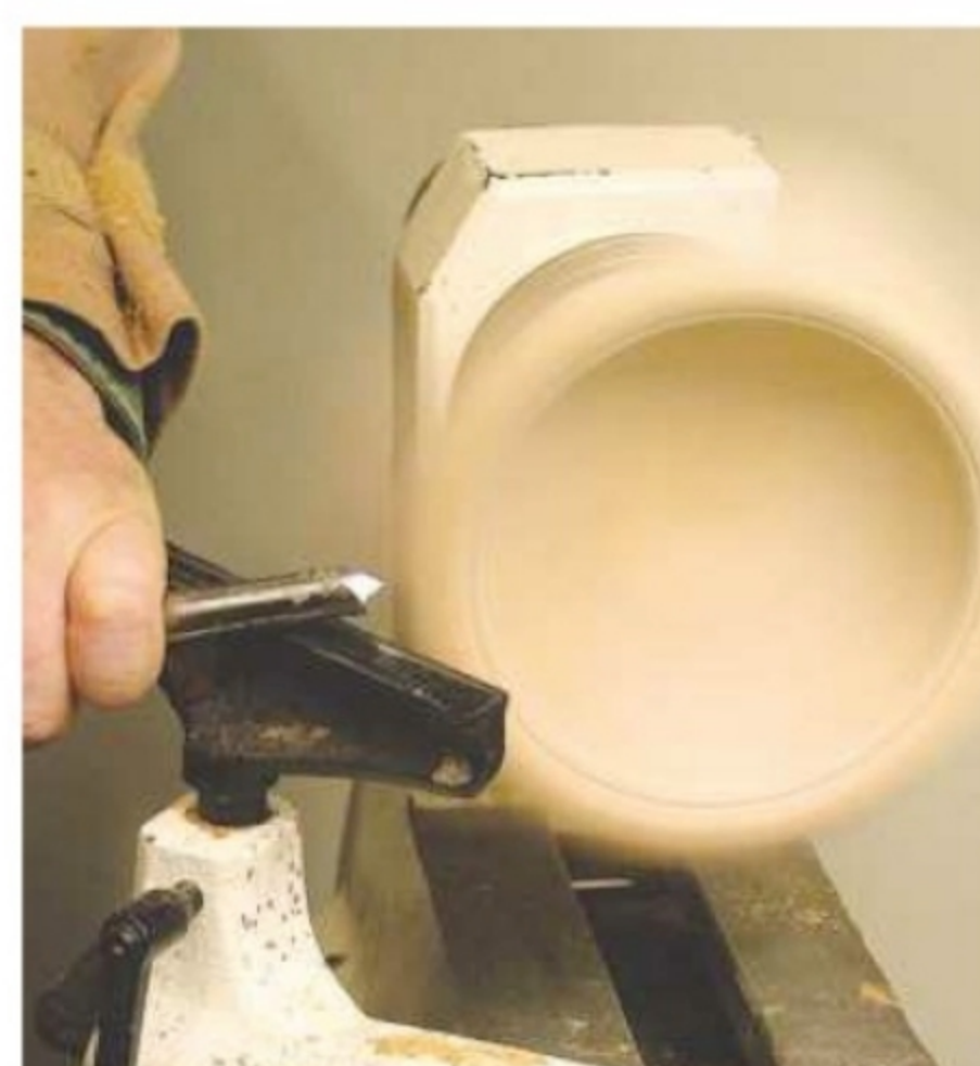
3. Either sand the work or take a very light finishing cut with a chisel to remove wood down to the bottom of the indentations
