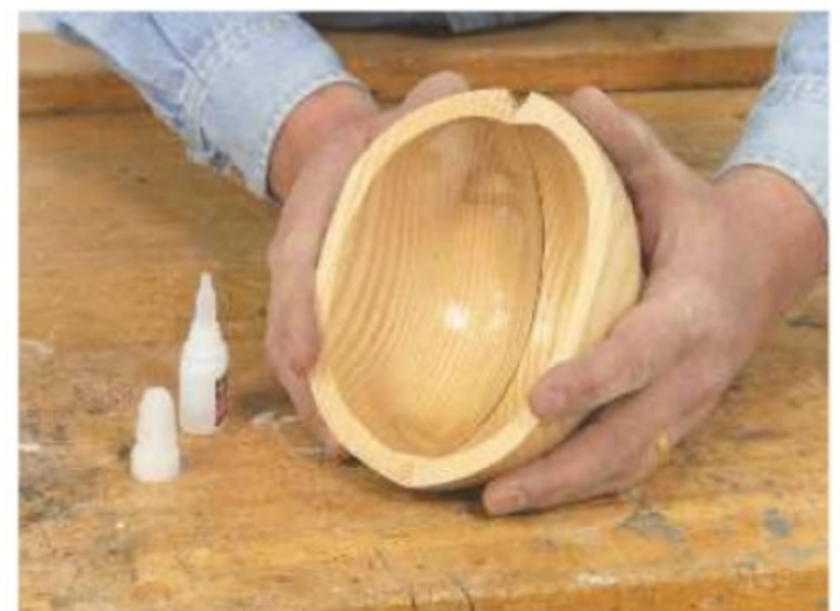
26. Assemble the two bowl halves, then sand and polish the rim and create a flat base
