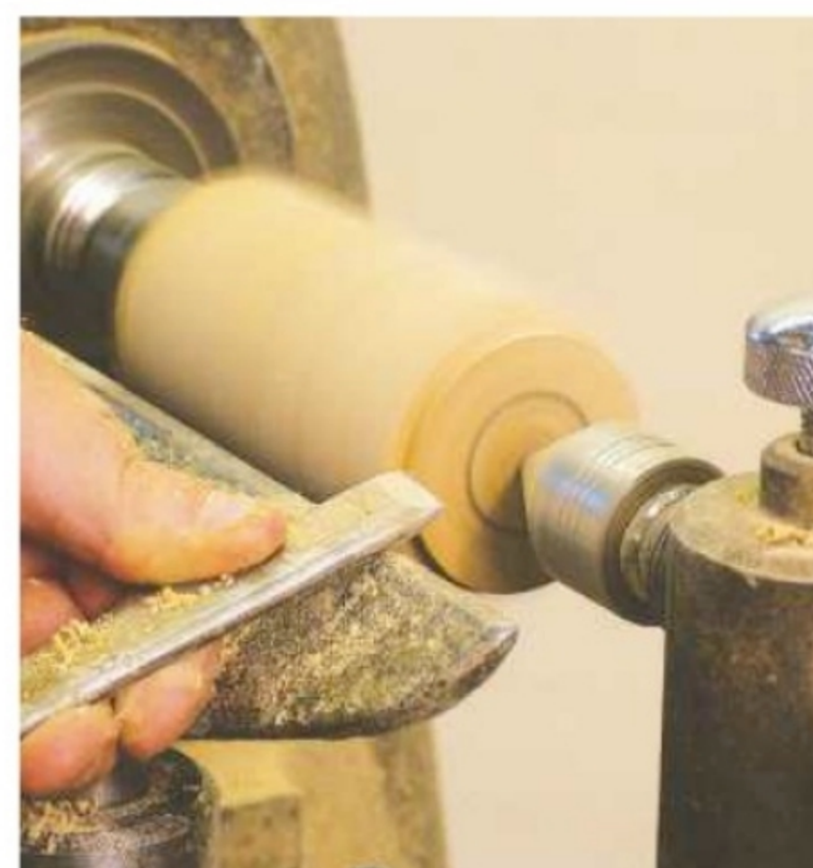
10. Mount the blank between its true centres and turn a spigot on each end to fit your chuck
