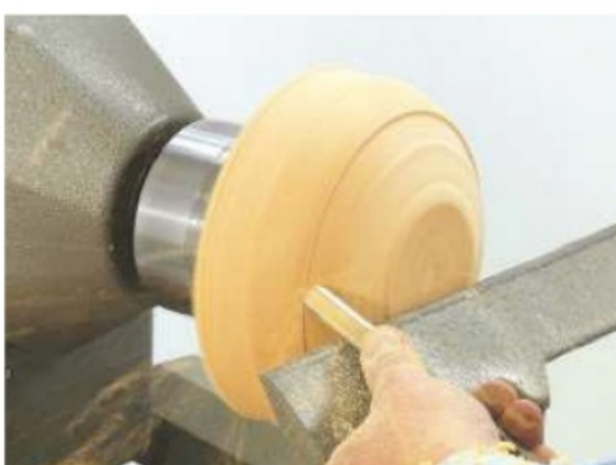
5. True up the face in the same way and start turning away the bowl profile
