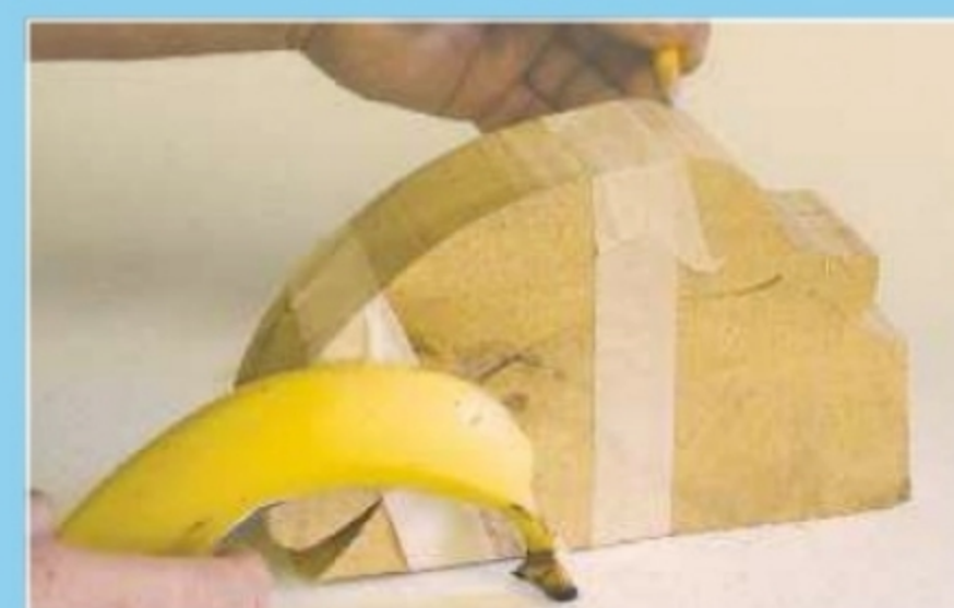
C. Tape the banana to the offcut and add the shape of the sides
