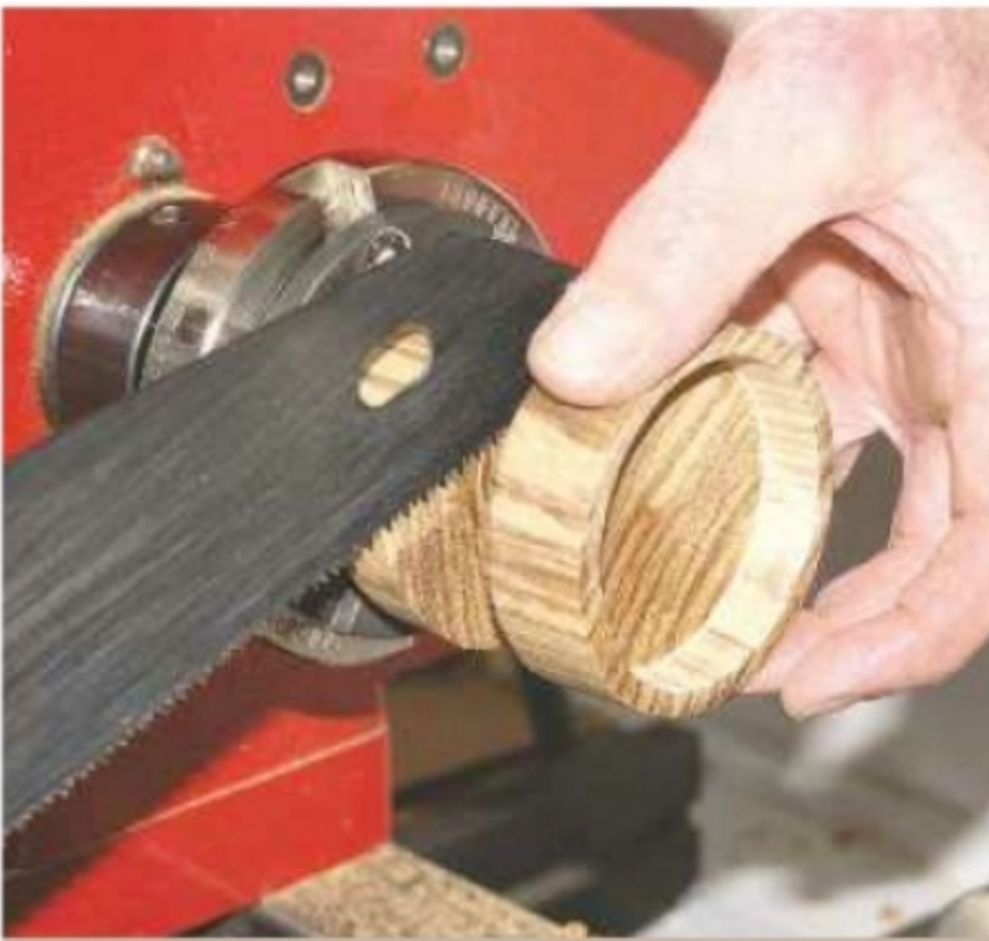
6. Check the lid depth and part it off
