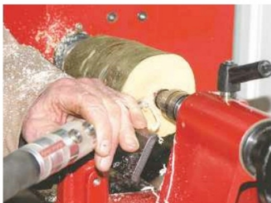
3. Set the lathe speed to 1500rpm and use a bowl gouge to face off the end of the blank
