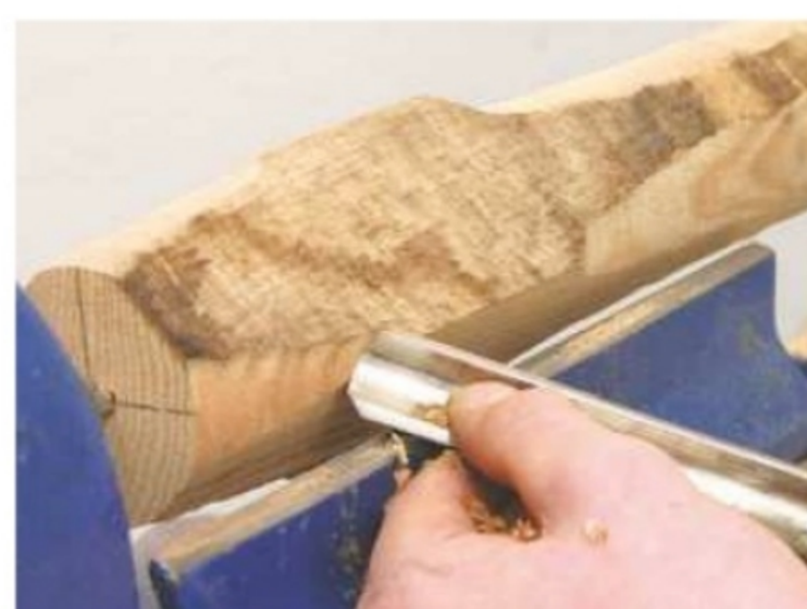
19. Mount the first leg blank between centres and turn it to a cylinder
