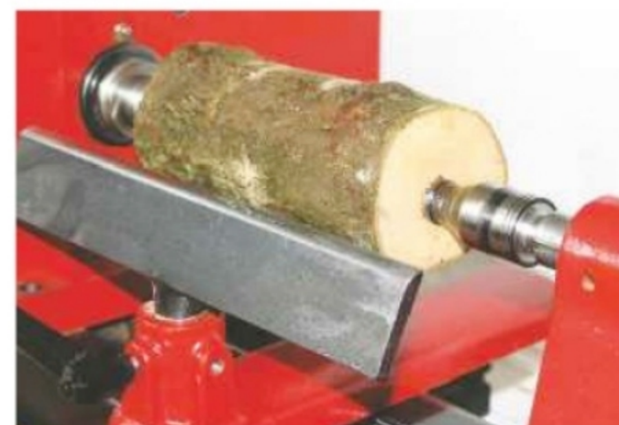
2. Mount the blank between centres and spin it to check that it clears the toolrest
