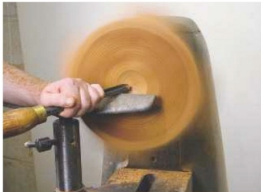
13. Check that the rim of the bowl is dead flat, and trim it if necessary
