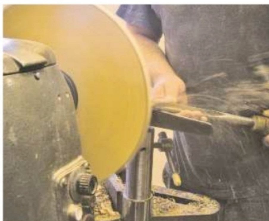
4. True up the edge of the bowl using the very tip of the tool
