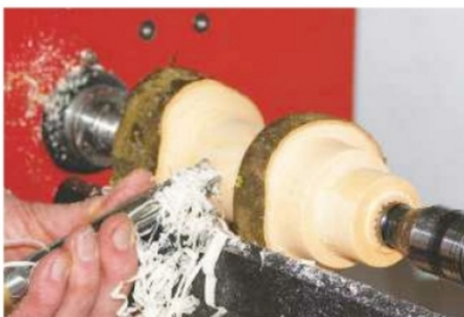
6. Remove some surplus wood from the stem and base area to reduce the imbalance
