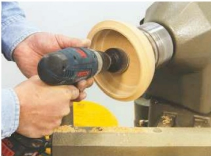
12. Sand the interior of the bowl, working down through the grades to 400 grit
