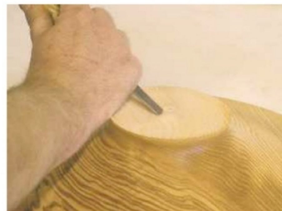
18. Take the bowl off the lathe and cut off the stub with a chisel
