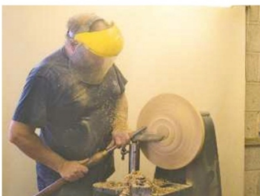
3. ...and mounted it using a screwchuck in my combination chuck
