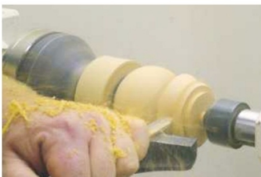
15. Reverse-mount the satsuma on the screw chuck and start shaping the bottom
