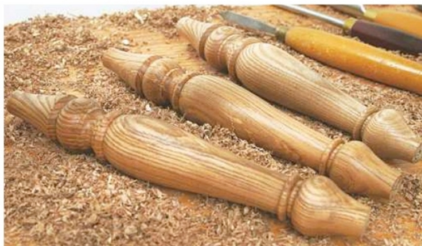
31. The three finished legs should look identical if your copying has been accurate
