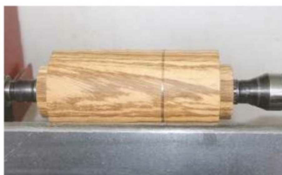
1. Form spigots and mark the cutting line
