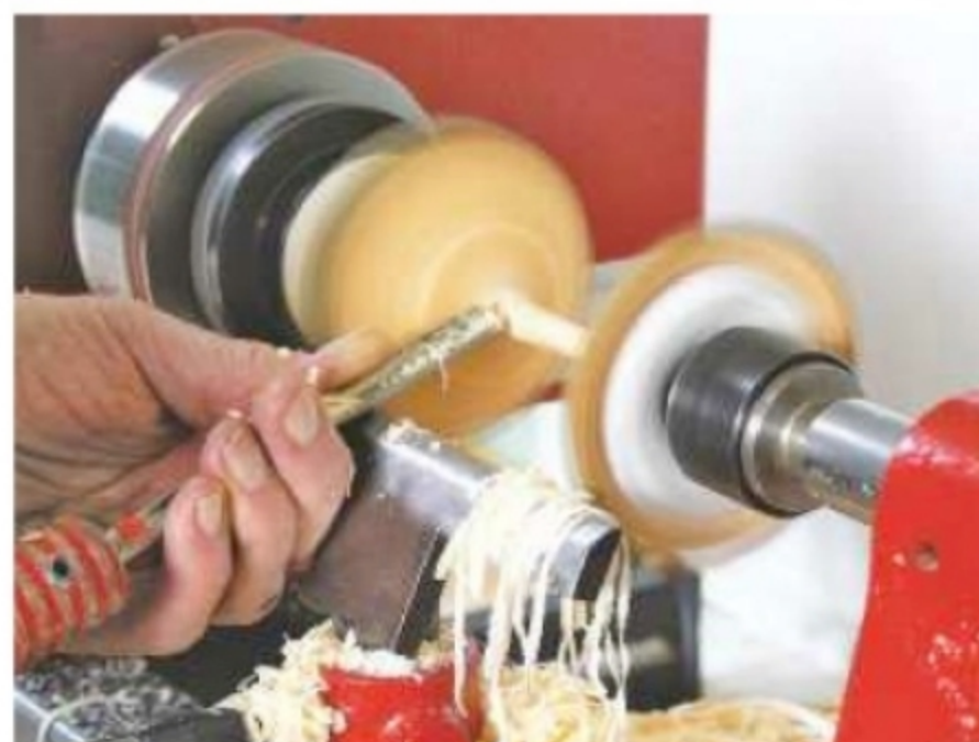
13. Turn the stem in 12mm wide stages from top to base, aiming to get it as thin as you dare!
