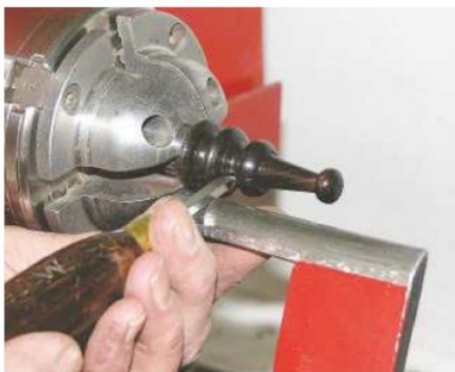
13. Turn the two finials with spigots to fit the holes in the pomander
