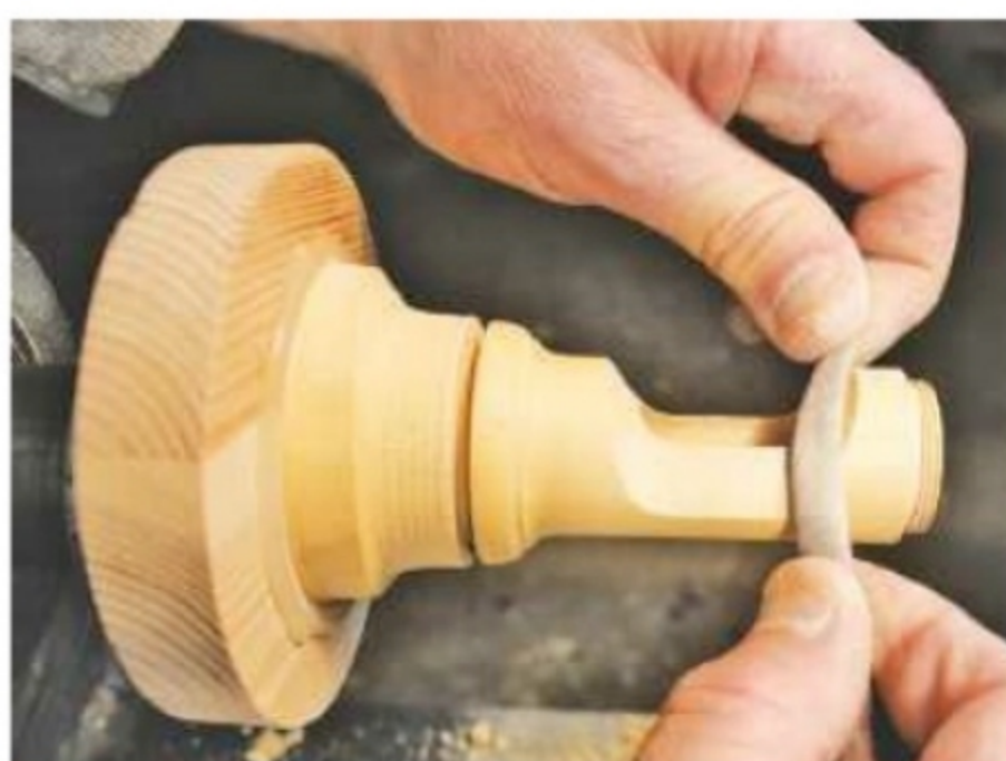
22. Check the fit of the hourglass, then trim and sand the window by hand
