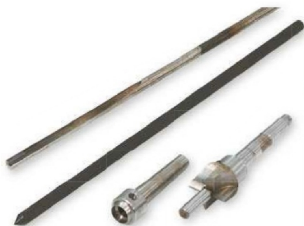
1. The long-hole boring kit includes the auger, centring bar, hollow centre and counterbore tool
