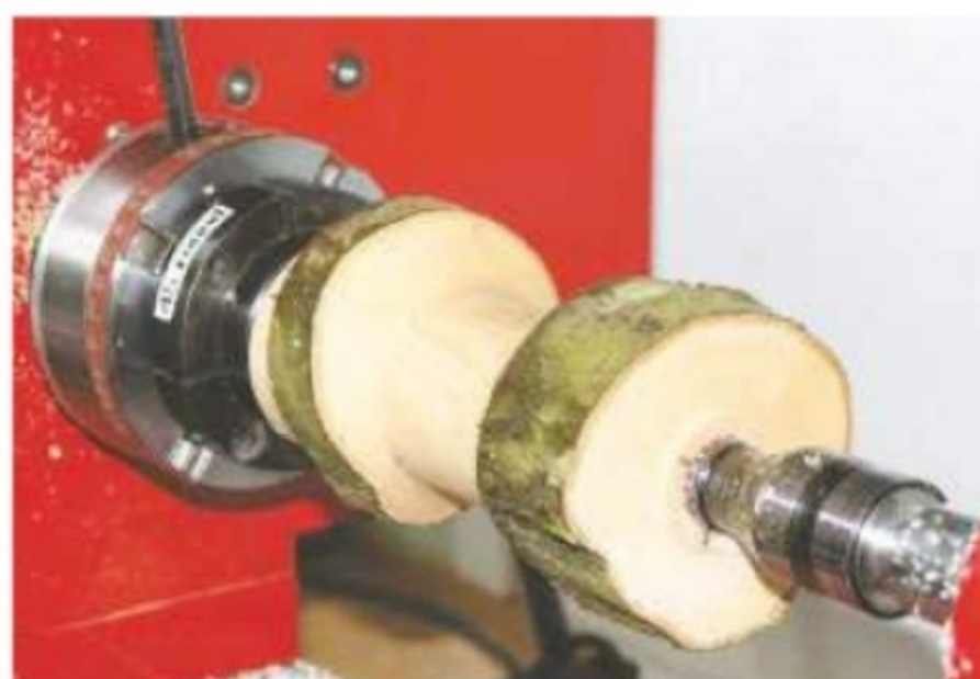
7. Screw on the chuck, mount the spigot in the jaws and bring up the tailstock before tightening up
