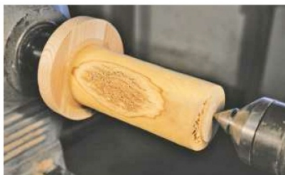
1. Glue the blank cylinder of boxwood to the centre of a softwood disc
