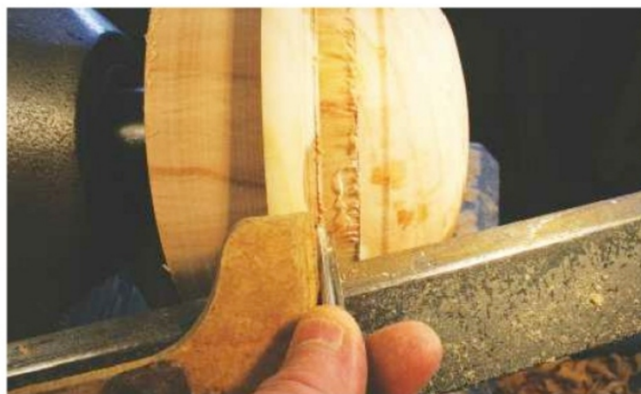
8. Use a toolrest support to control the gouge while cutting a concave curve
