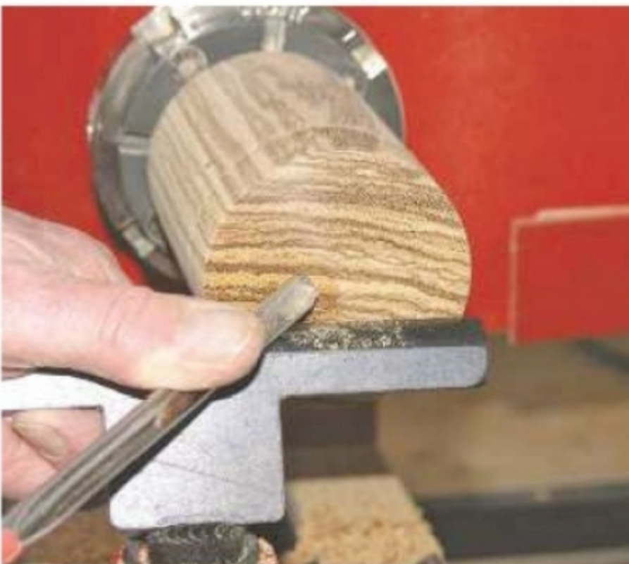
9. True off the top of the lid and sand it
