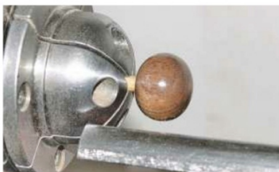
14. Mount the knob blank on a dowel to act as a spigot, then turn it to shape and apply the finish
