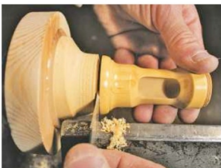
23. Then part off the work. Leave the waste on the softwood disc and...
