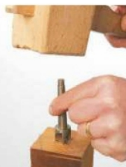
3. Knock the drive centre into the blank with an old mallet
