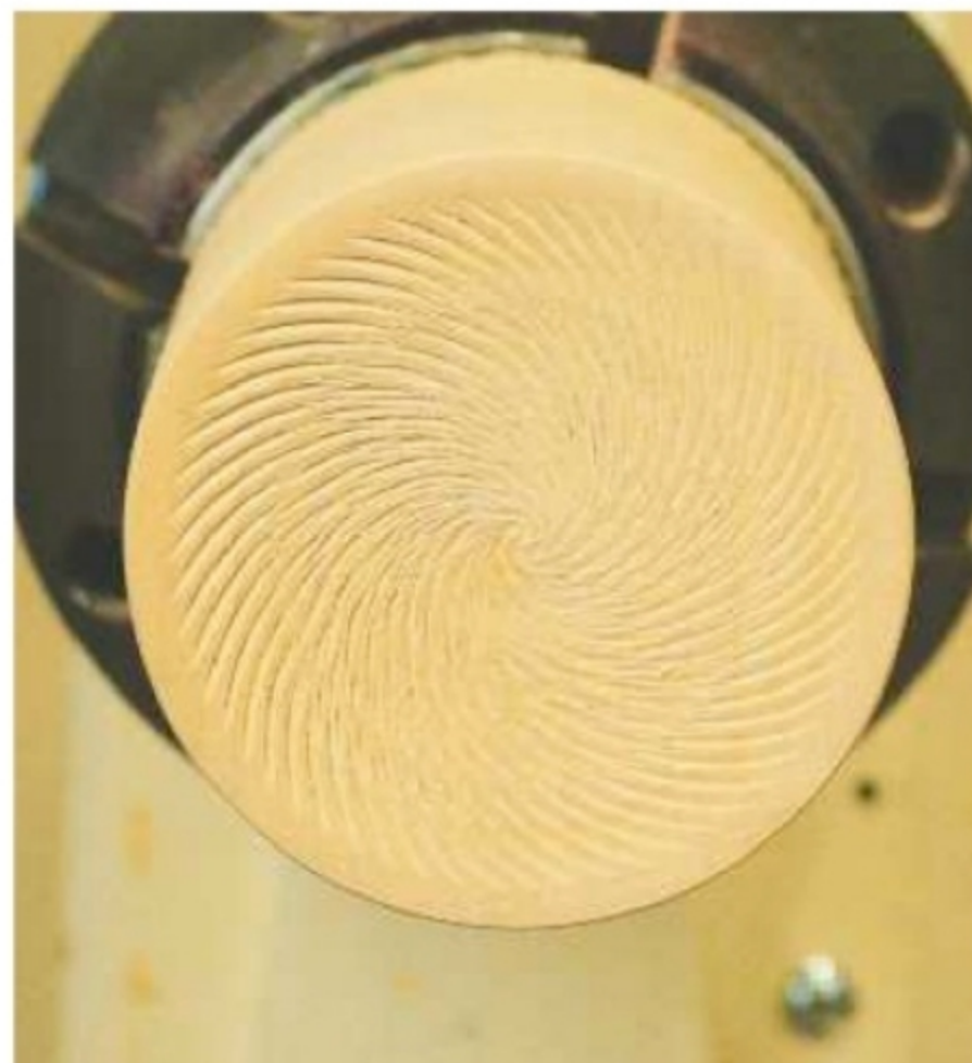
4. This produces a spiral effect. Cutting end grain like this leaves a few torn fibres, and these are easily cleaned off with the natural hog's hair brush supplied with the tool. Simply push the brush into the textured area with the lathe running at around about 1200rpm
