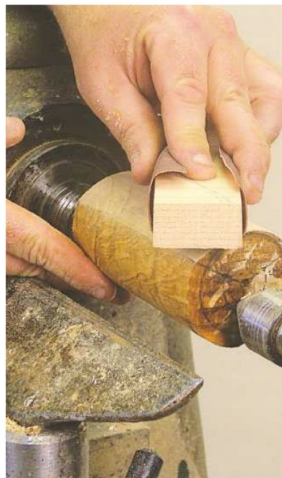
8. Then stop the lathe so you can hand-sand the blank in the direction of the wood grain
