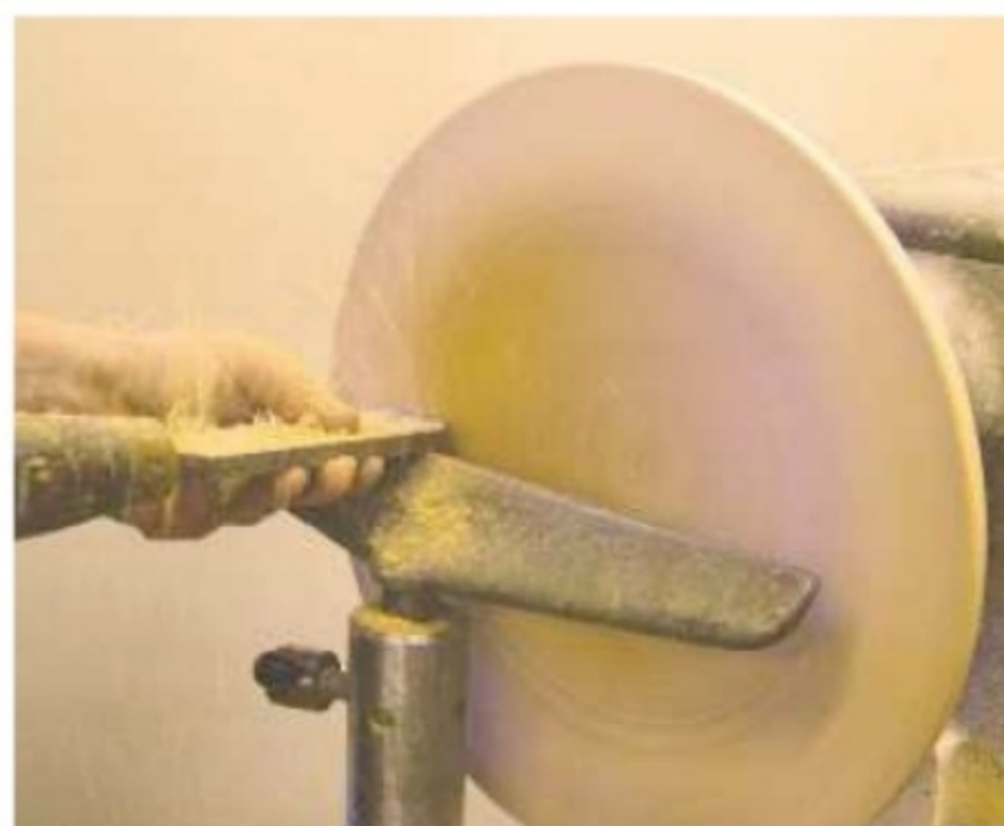
13. Finish the inside of the bowl with a round-nosed scraper
