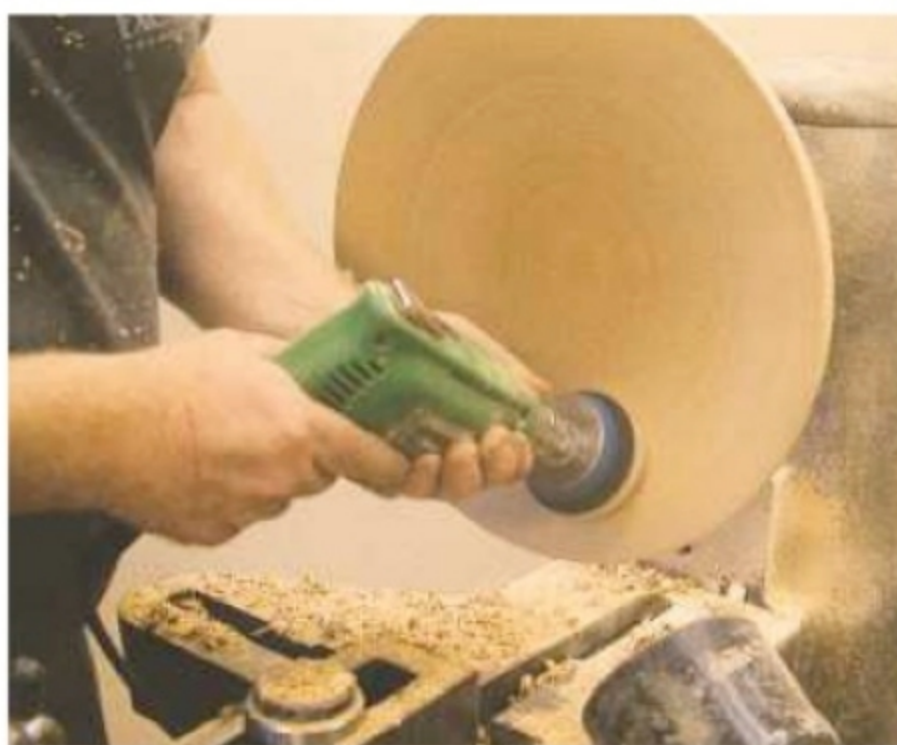
14. Power-sand the interior with the dust extract hose nearby
