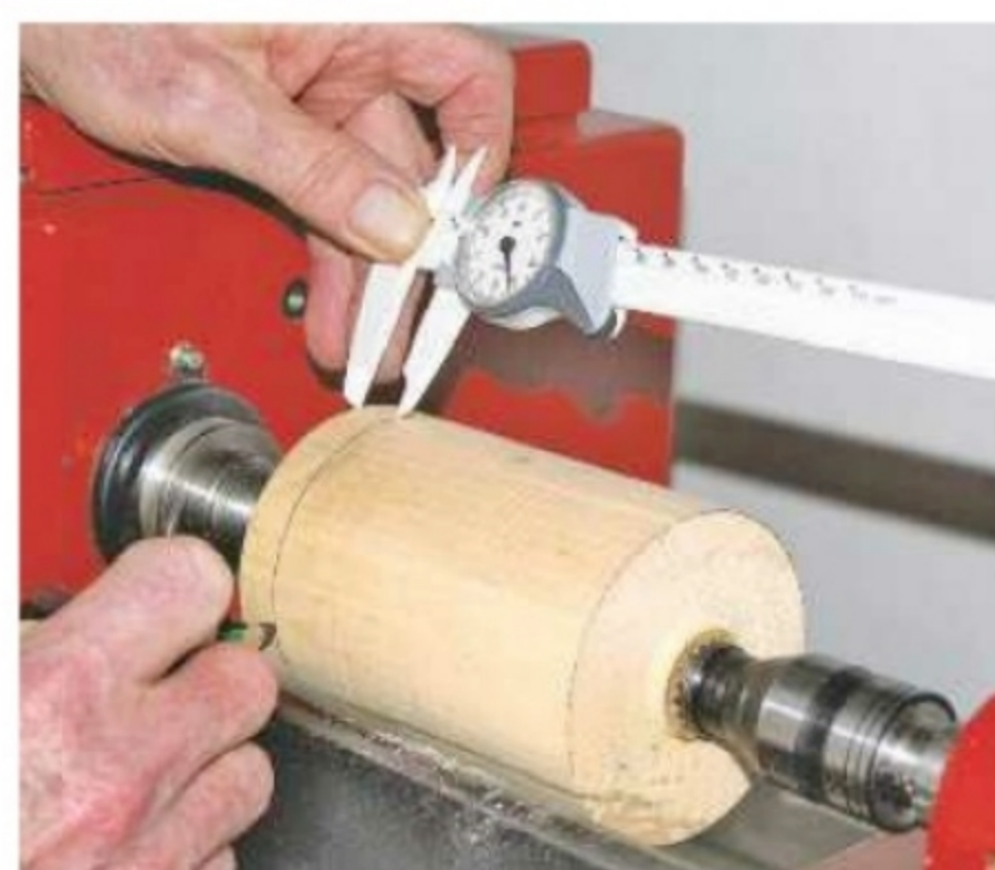
2. Form a spigot at one end to match the chuck jaws you're using
