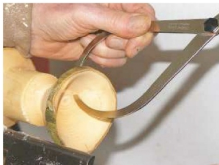
11. Alternatively you can measure the wall thickness using external/internal callipers
