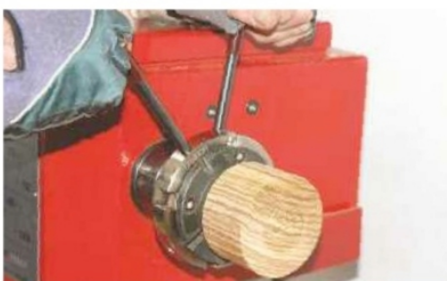
4. Fit the lid blank in the scroll-chuck jaws
