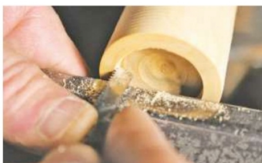
5. Start the thread by holding the chaser lightly against the side wall
