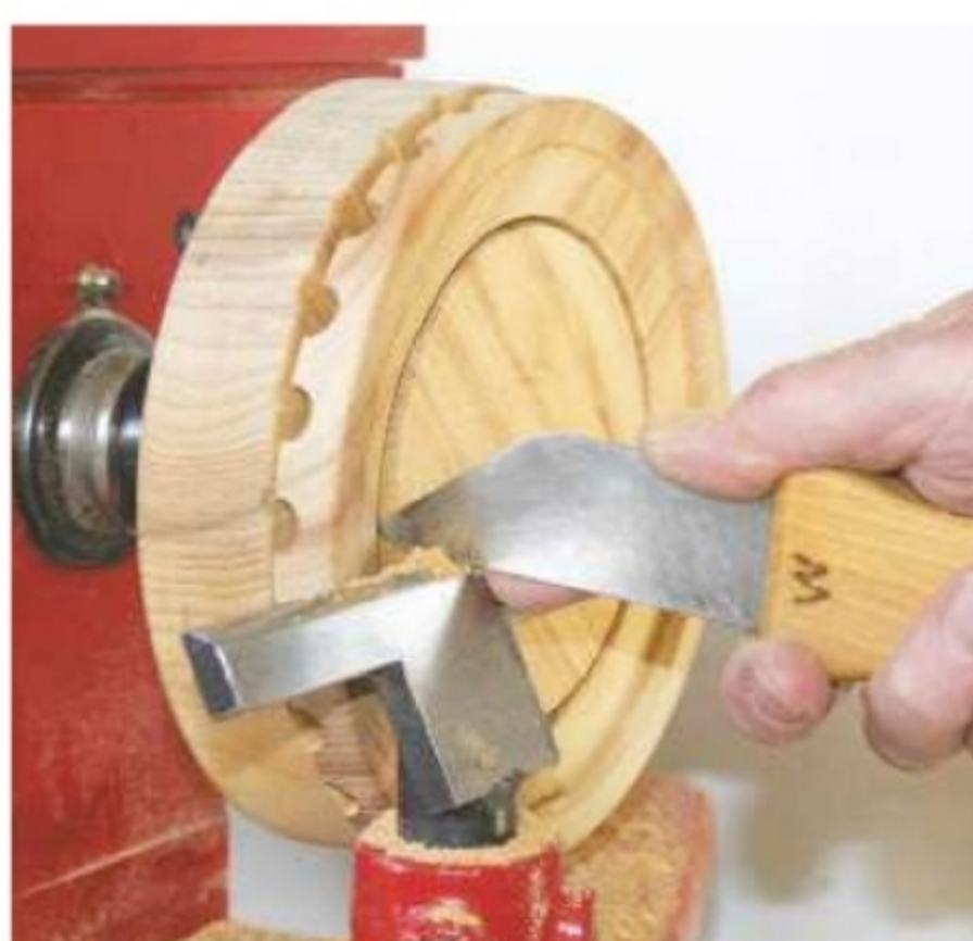
5. Then part through the face of the blank until a free ring is formed
