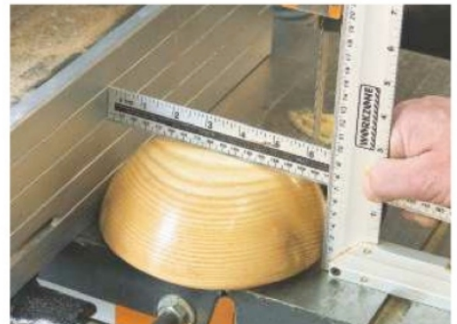
20. Use a square and a rule to find the precise diameter of the bowl
