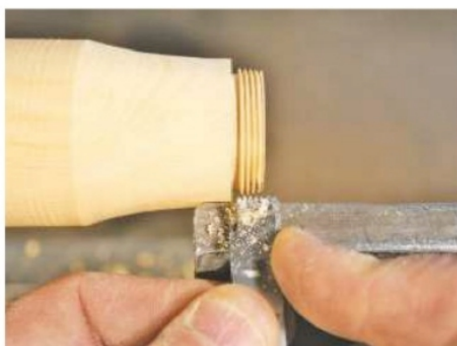
14. Withdraw the chaser at the end of the run so it misses the shoulder
