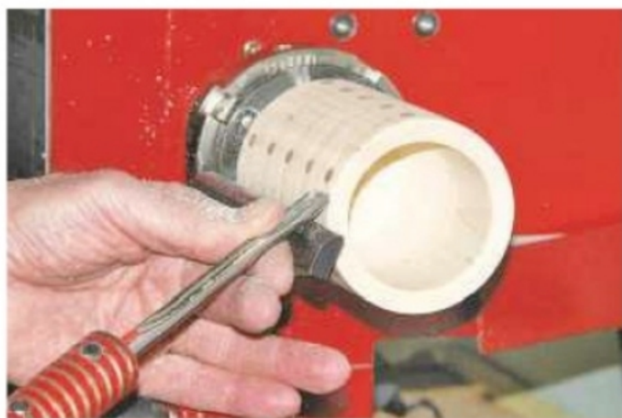
11. Use a sharp gouge to turn the dowels flush; then sand the outside and apply cellulose sealer
