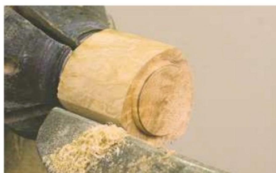
13. Taper the spigot and push the lid onto it so its inner surface burnishes the spigot
