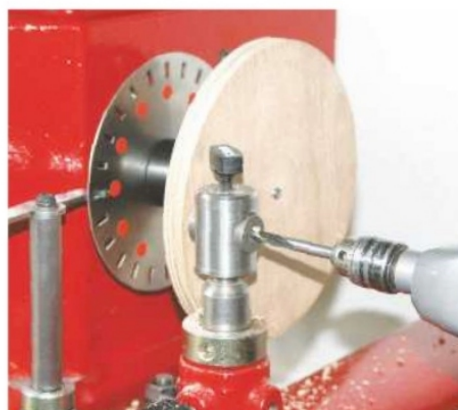
1. Drill 12 holes right through both discs, 10mm in from the edge
