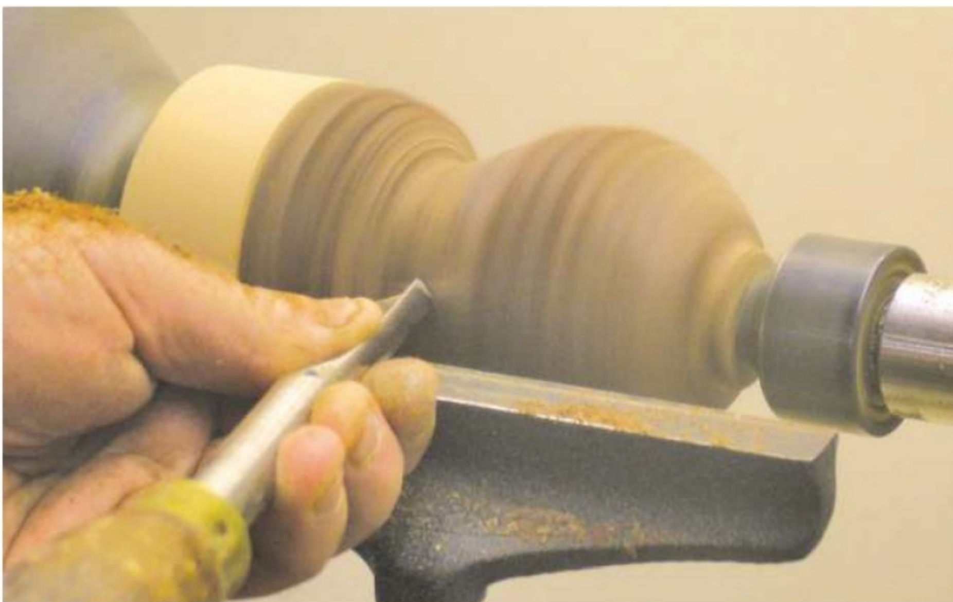
12. Start shaping the pear using a spindle gouge as before
