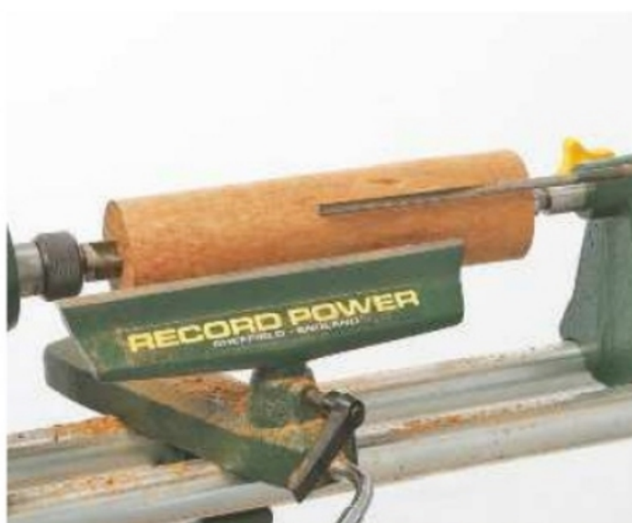
15. At the halfway point, withdraw the auger to check progress
