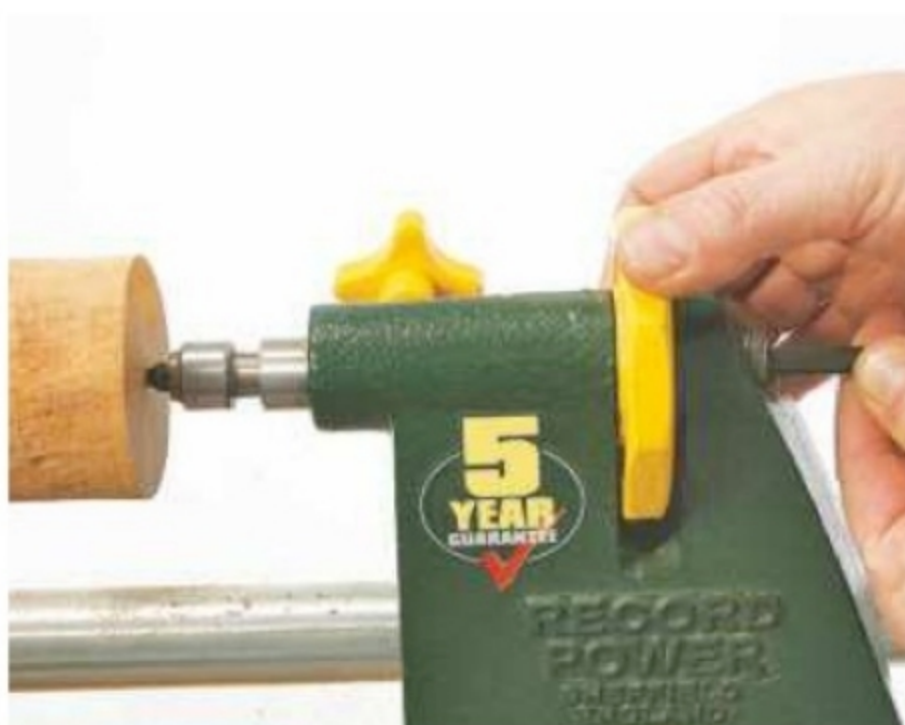
7. Keep the pressure on as you wind in the tailstock barrel...
