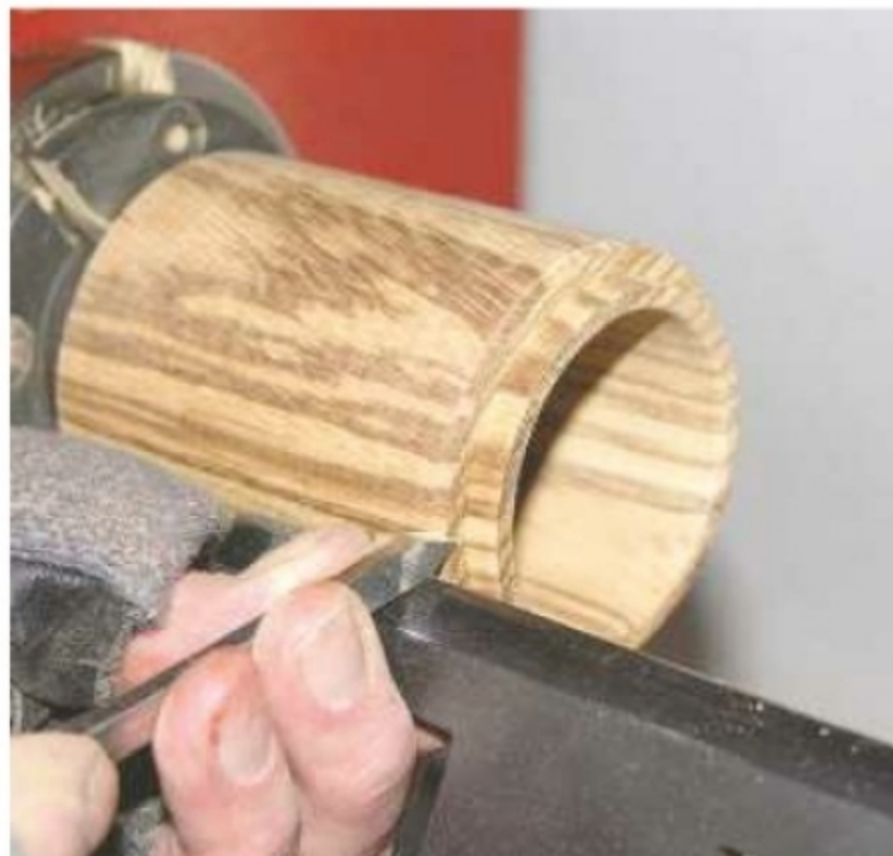
13. Form a secondary shoulder on the rim
