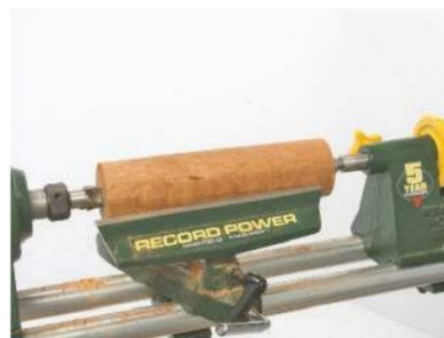
19. Line up the tailstock end as before and complete the boring
