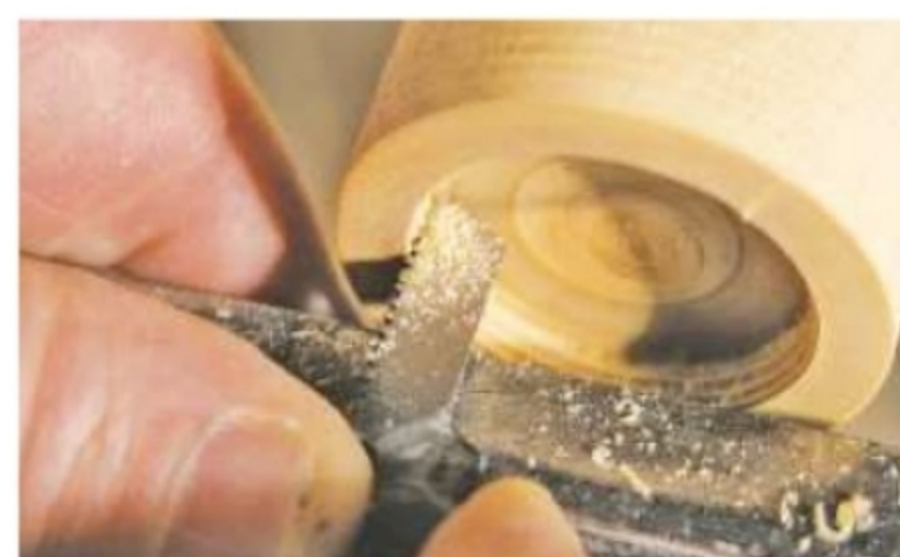
6. As the thread gets deeper, press harder so the teeth dig into the wood
