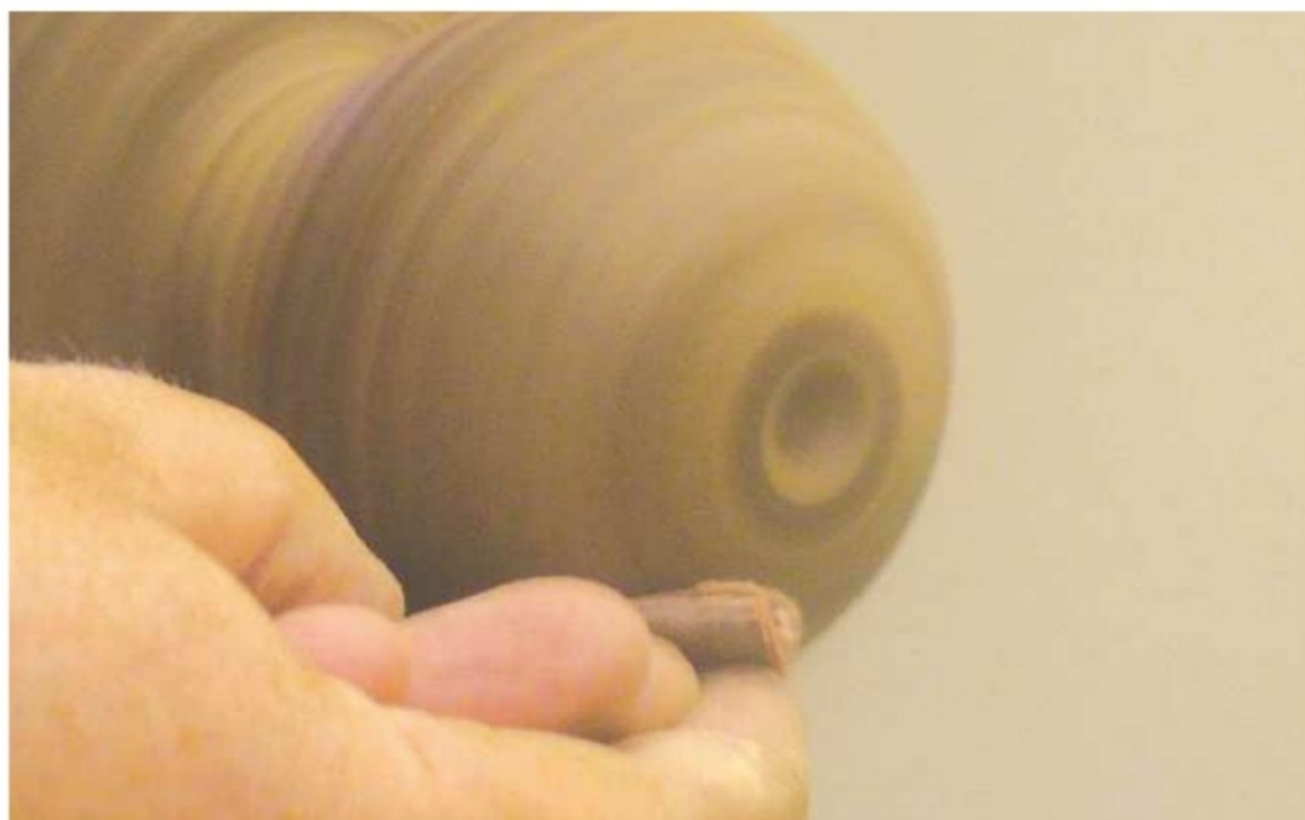
13. Sand with your fingers flat on the underside of the work; remove the toolrest first
