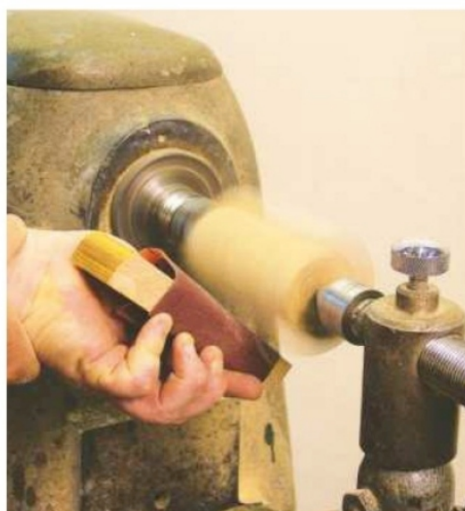
7. Fold abrasive paper round a wood block and hold this gently against the revolving blank
