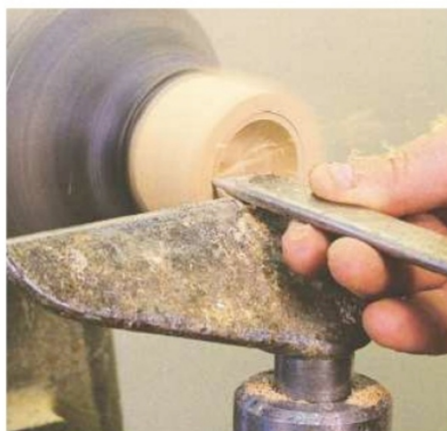
11. Use a skew chisel to cut a parallel-sided recess in the underside of the lid
