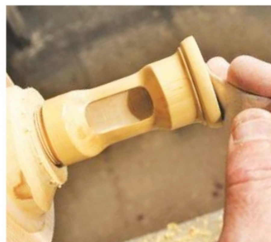
25. Trim, sand and polish the end, fit the sandglass in its window and screw on the lid
