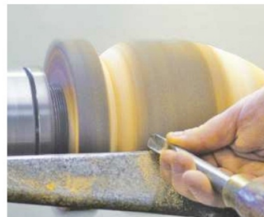
3. Define the neck of the vase by making V cuts with a spindle gouge
