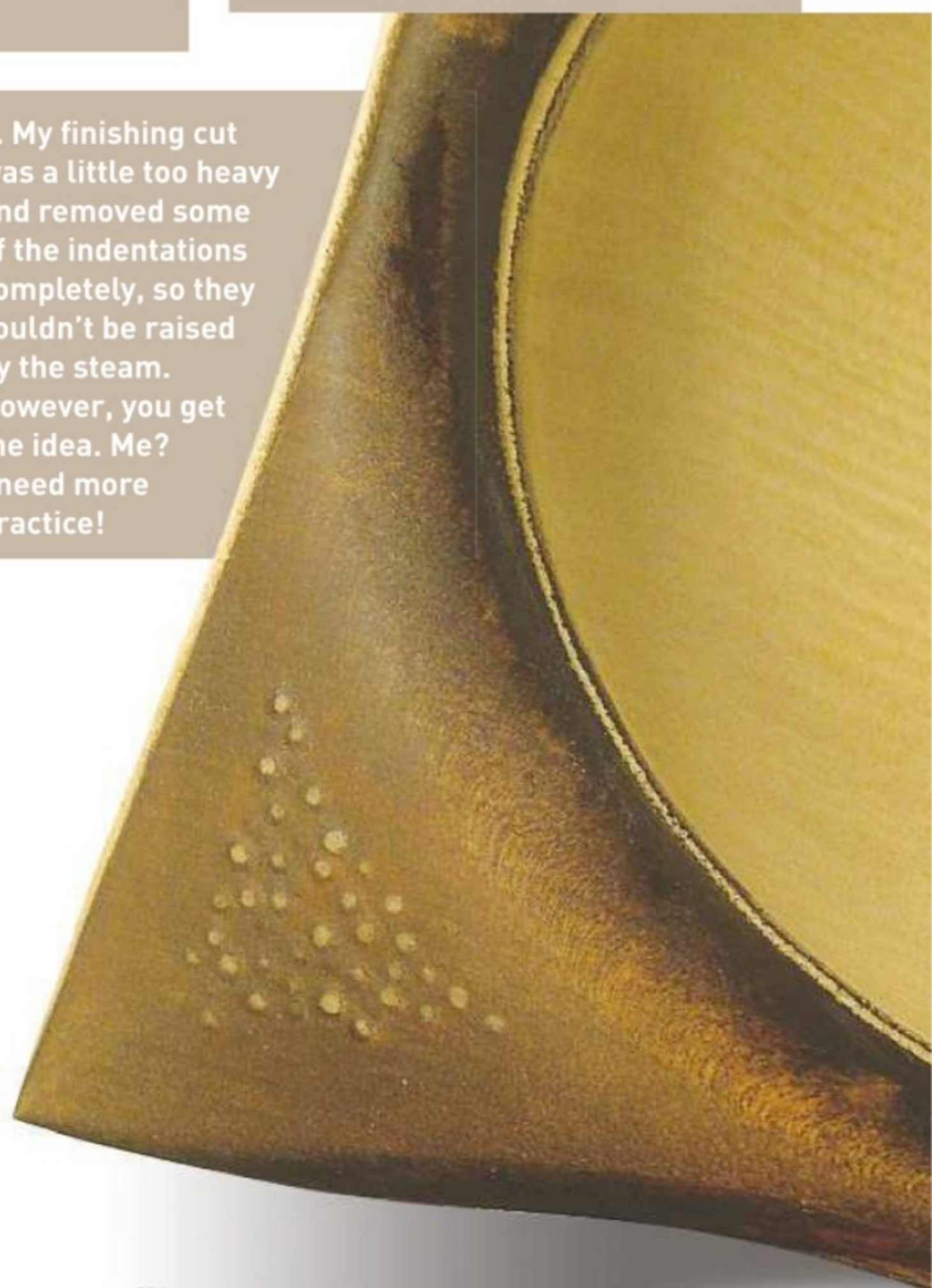
3. Either sand the work or take a very light finishing cut with a chisel to remove wood down to the bottom of the indentations
