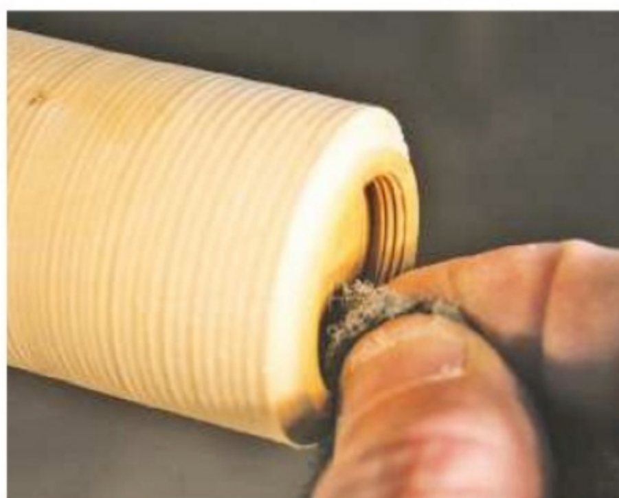
8. Smooth the threads with abrasive nylon matting and rub in some wax
