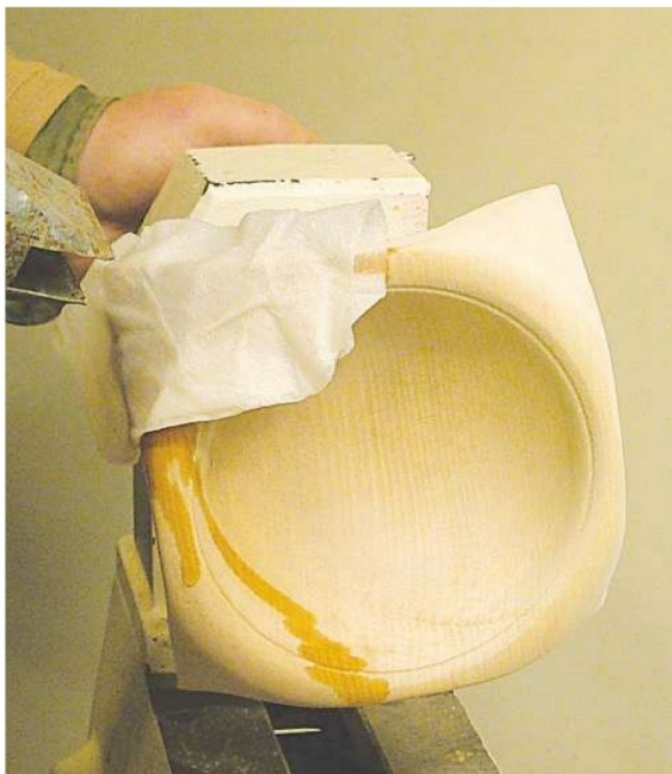
4. Wet the wood, cover it with a wet cloth or paper towel and use a hot air gun to heat the wood. The steam created will swell the fibres and raise each dent into a projecting pimple
