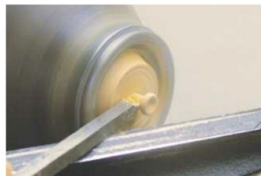
16. Turn a small button about 5mm in diameter to cover the screw hole in the satsuma
