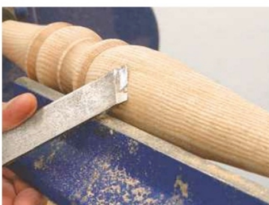
24. Smooth the long tapering centre section of the leg with a skew chisel
