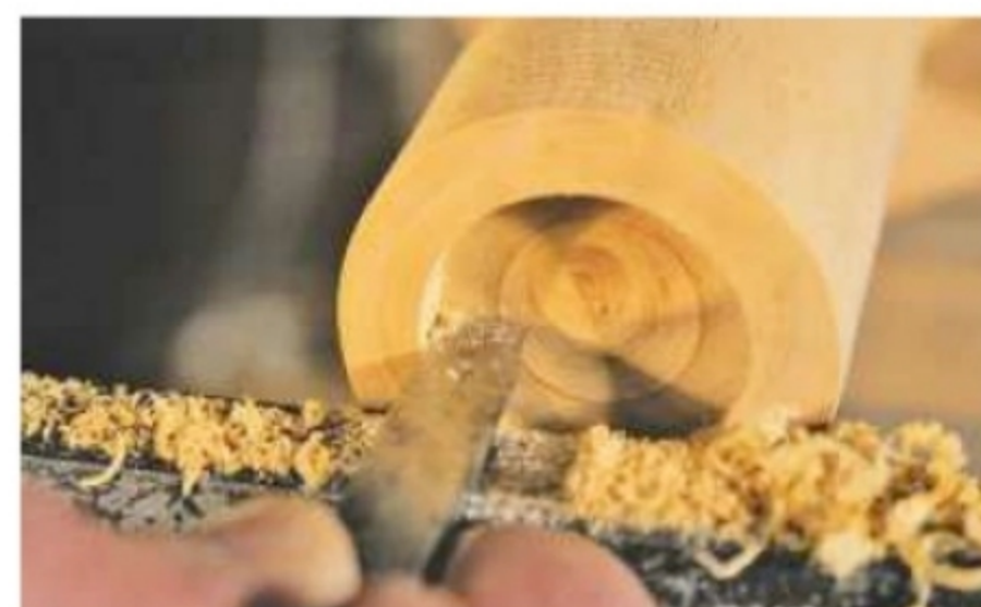
3. Clean up the corners of the recess with a small square-end scraper
