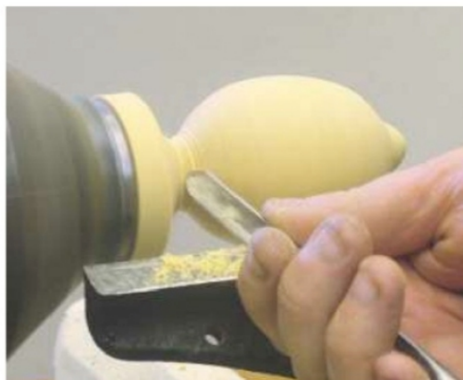
7. Shape the bottom part of the lemon, taking it down to about 10mm in diameter
