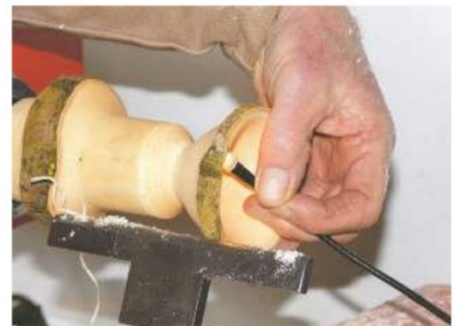
10. Check that the wall thickness is uniform using a small worklight or an LED torch
