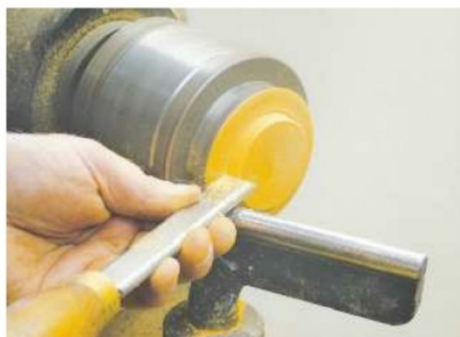
14. Mount the plug, transfer the size of the hole to it and cut a taper on it using a skew chisel
