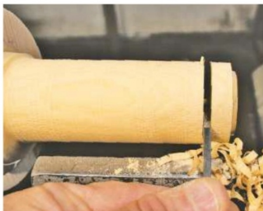
10. Allow for the thickness of the top of the lid as you part it off the lathe
