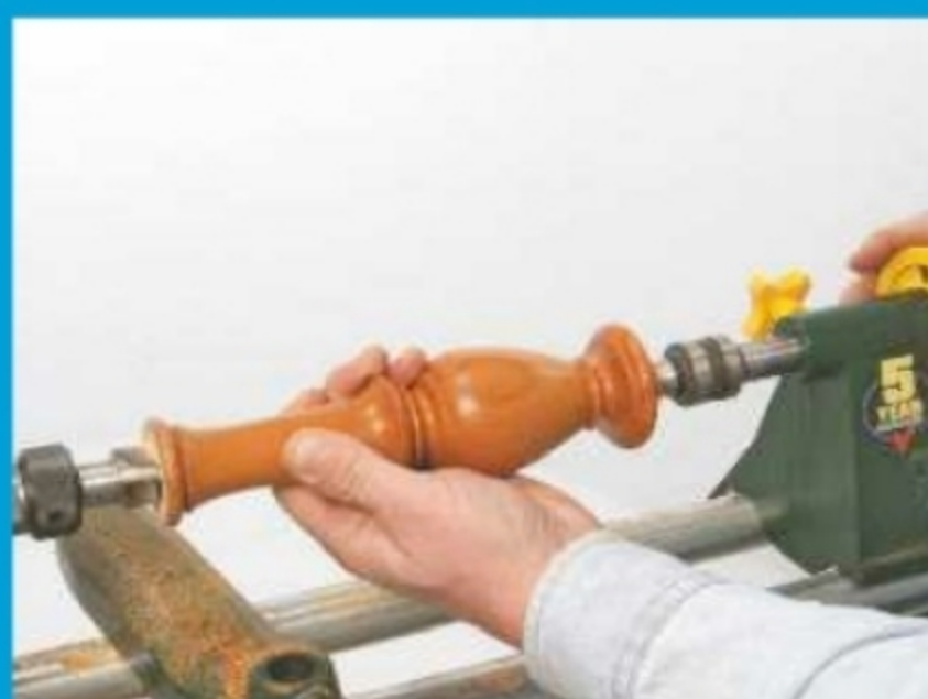
A. Use the counterbore tool to bore a recess for the fixing plate
