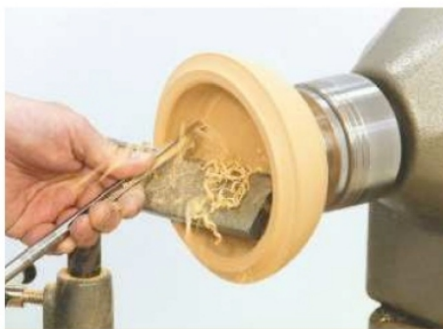
10. The short bevel on the gouge allows you to undercut the lip of the bowl
