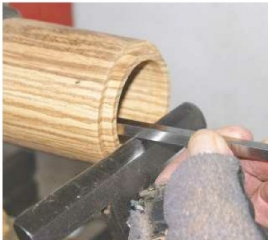
10. Start to hollow out the body of the box
