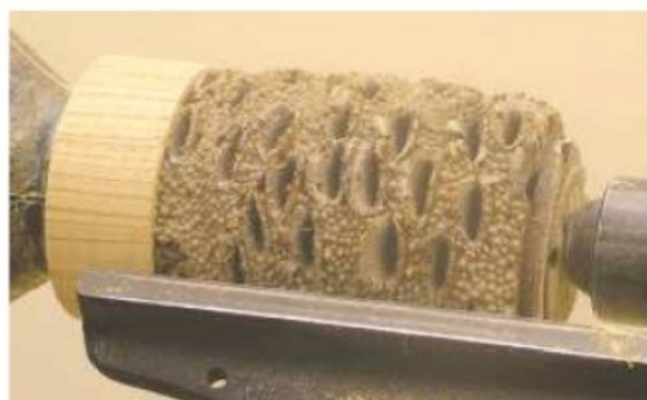
11. To make the pear, mount the banksia nut on the screwchuck ready for shaping
