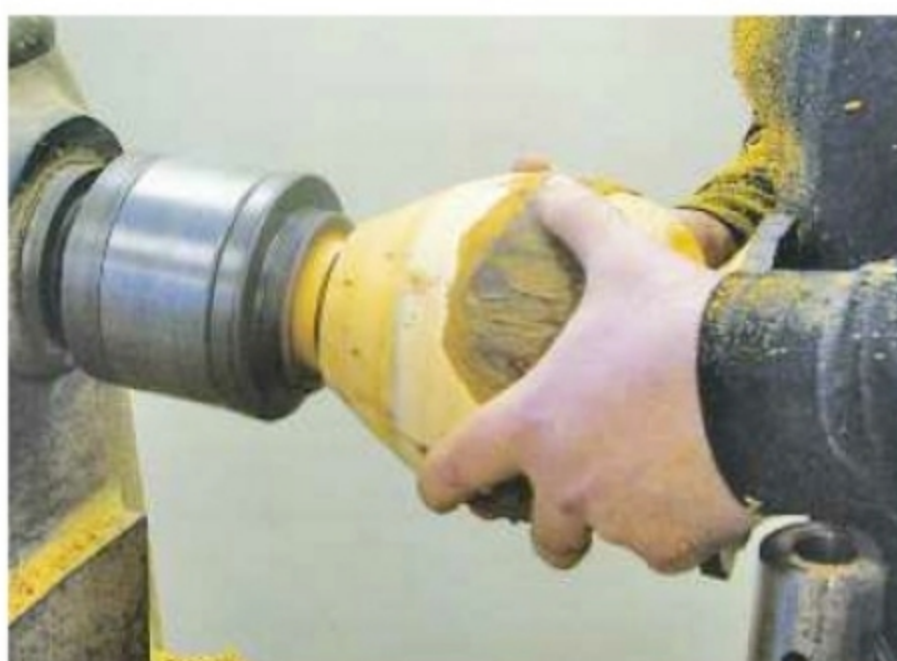
15. Offer up the vase to make a mark on the taper. Cut the plug sides parallel down to this mark
