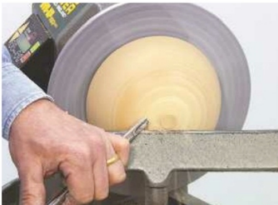
18. Maintain the same curve round the base as you remove the spigot
