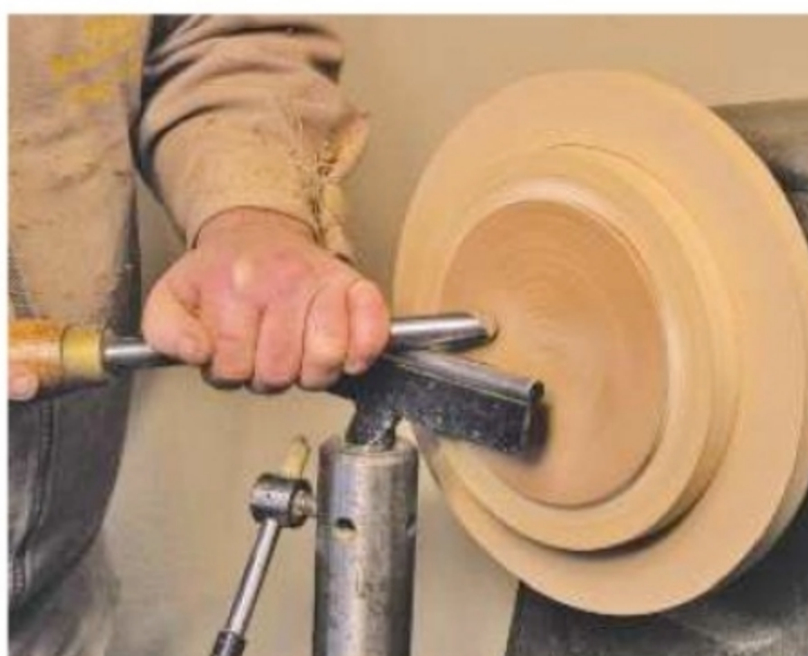
6. True up the face of the blank with a fingernail profile bowl gouge
