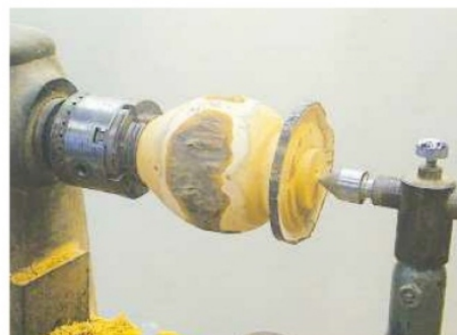
16. Glue the plug in place and use the tailstock to apply pressure until the glue dries
