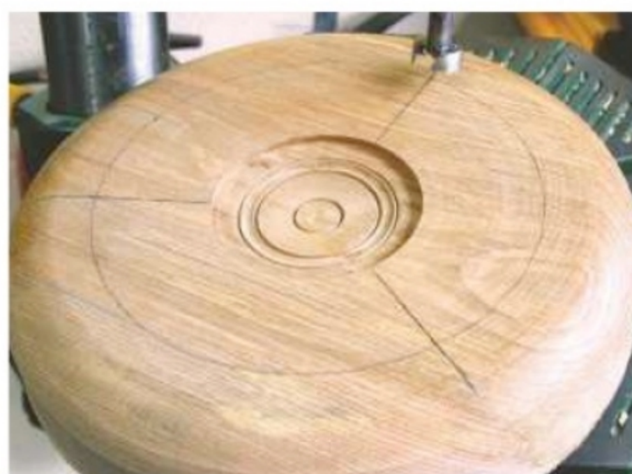
11. Draw pencil lines at the three hole positions to aid the orientation of the drill bit
