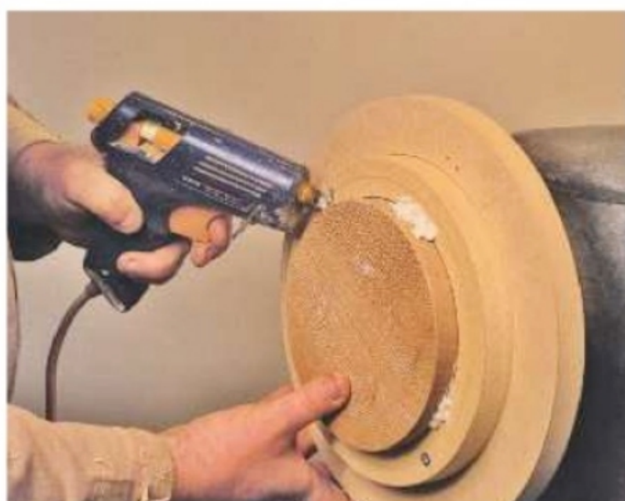
5. Fit the trivet blank into the recess, securing it with hot-melt glue
