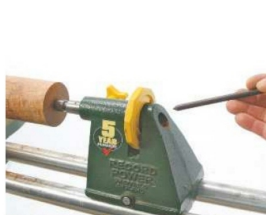
9. As it grips, lock up the barrel and pull out the centring bar
