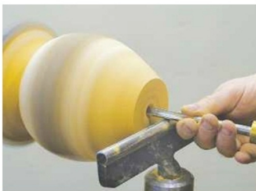
8. Use a \frac{3}{8} in spindle gouge to start boring a hole into the base of the vase
