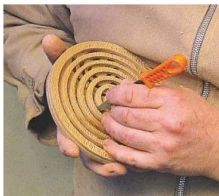
14. Remove wood fibres from the intersections with abrasive paper or a needle file
