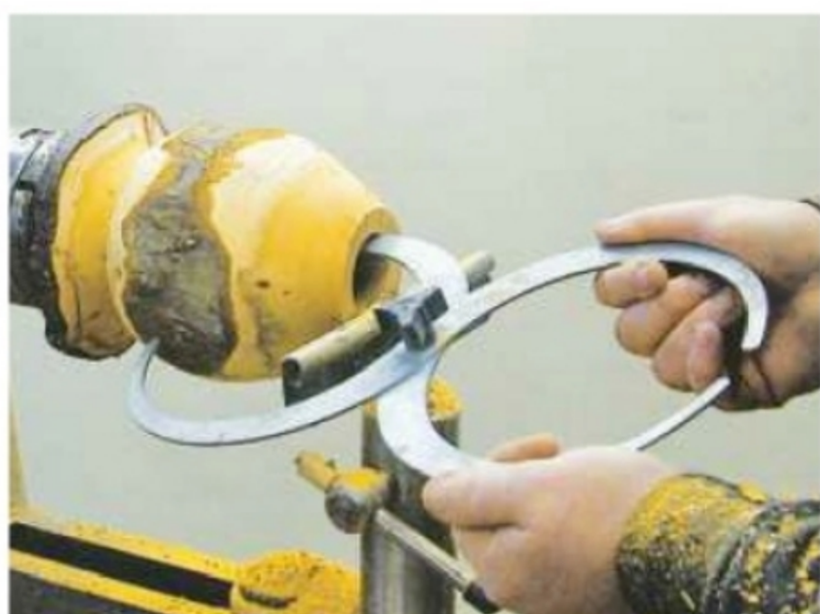
11. Double-ended callipers will give an accurate indication of the wall thickness
