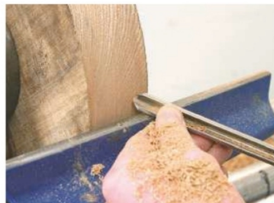
4. True up the edge first, then clean up the face and dish it slightly in the centre
