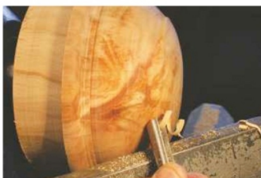
9. Complete the dome shape of the lid with the bowl gouge, using a slicing cut
