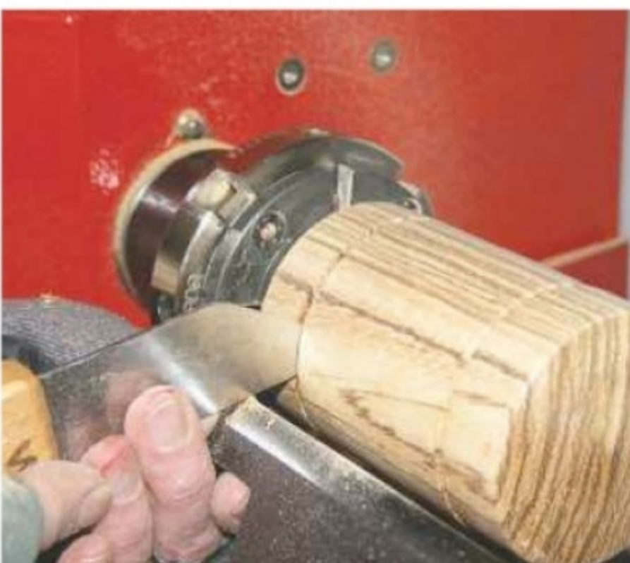
15. Partially part off the body at the mark
