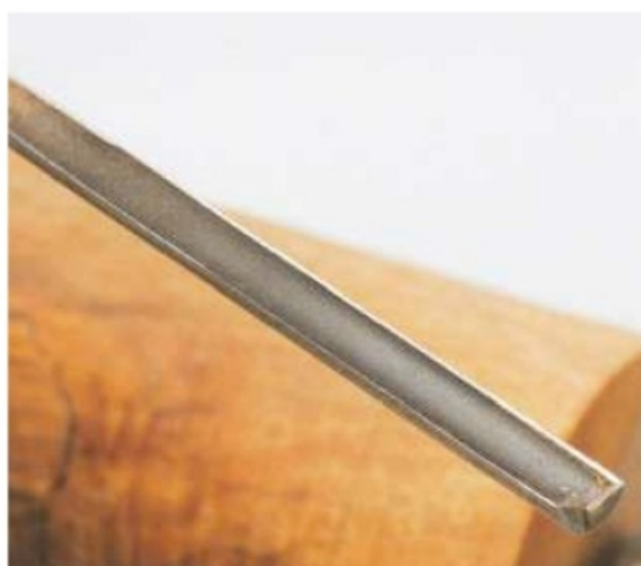
12. The best type of auger to use is the fluted shell type
