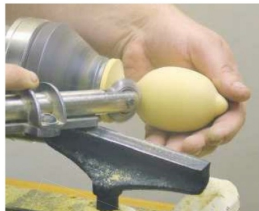
8. Support the lemon by cupping it in one hand while texturing it with the other
