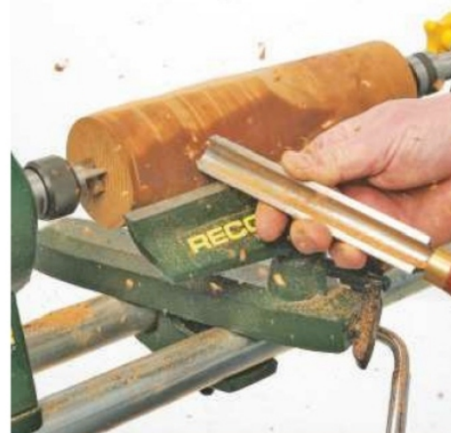
4. Rough the blank down to a parallel-sided cylinder
