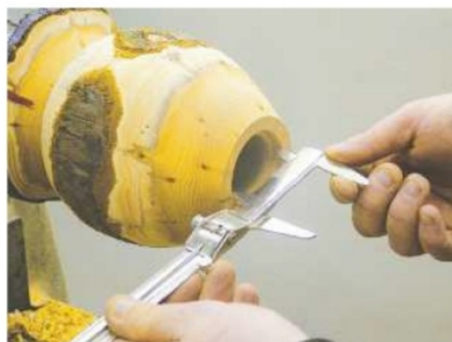
13. Measure the size of the hole with Vernier callipers; then remove the vase from the chuck
