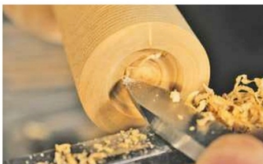
2. Use a small scraper to form a shallow recess in the end of the work
