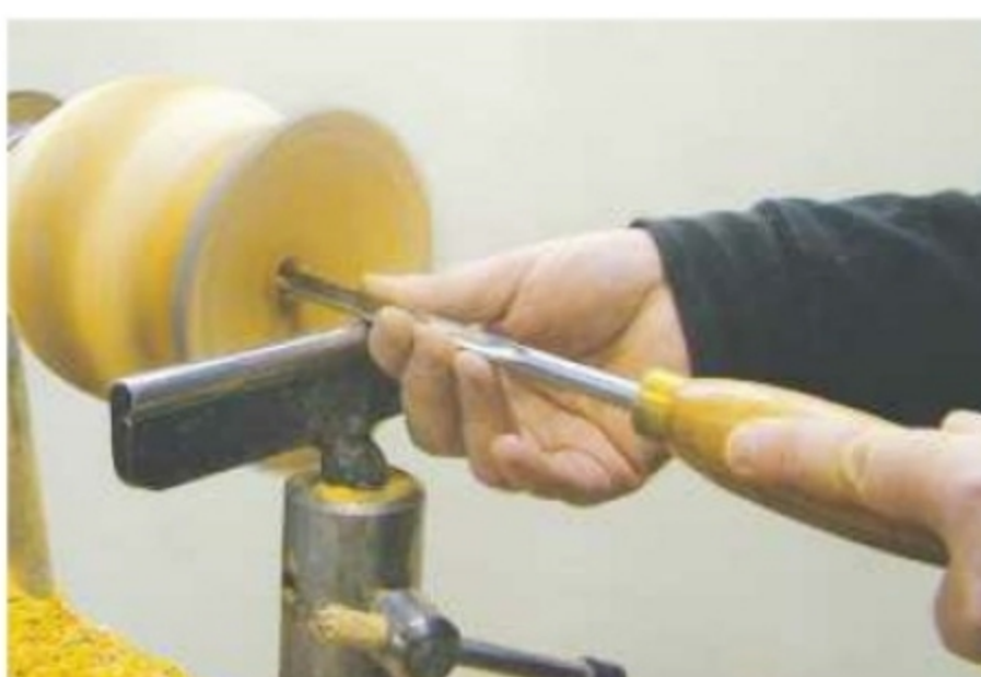
18. Bore a hole in the top to meet the cavity inside; then blend the hole into the rim
