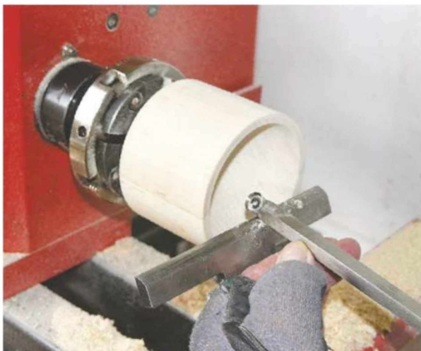
2. Mount one half of the blank in the chuck jaws and start to hollow it out
