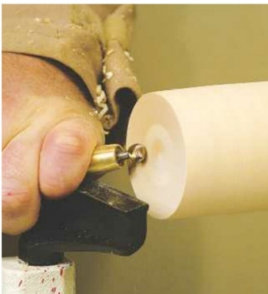
3. With the toolrest lowered I'm cutting just above centre, so the handle needs to be held well down. The lathe speed is about 700rpm. Starting in the centre of the piece, slowly drag the tool along the toolrest towards the edge
