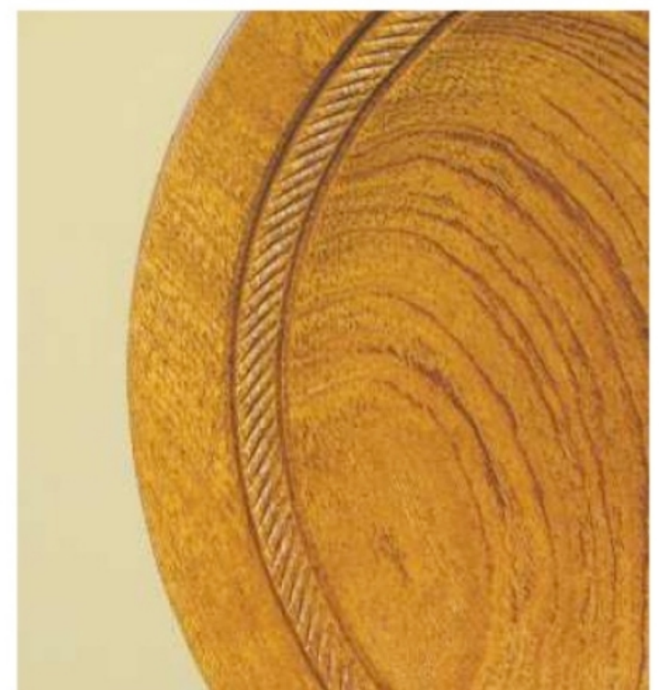
8. I textured the rim of this platter with the ball cutter at 700rpm. This time keep the tool still; don't drag it across the toolrest. Press hard and allow time for the cutter to create the decoration
