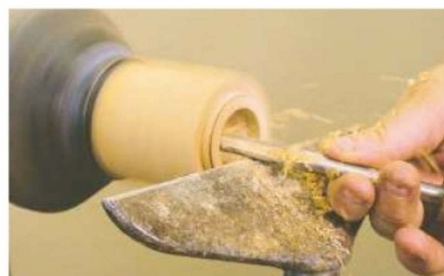
14. Hollow out the box, sand and polish the interior, then cut the tapered spigot parallel
