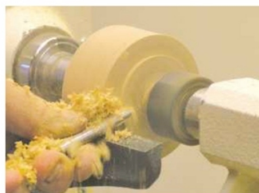
2. Cut a spigot using a skew chisel on its side to make a peeling cut
