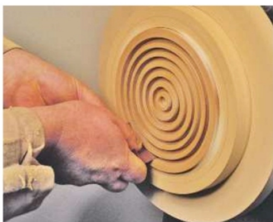
9. Remove the tool rest and sand each groove with folded abrasive paper
