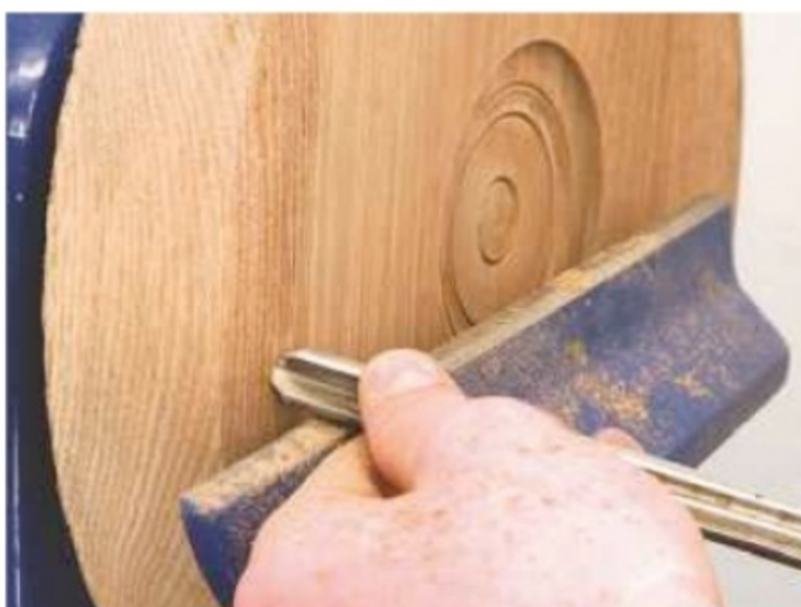
6. Radius over the whole edge to create a smooth profile, which looks better than a square edge
