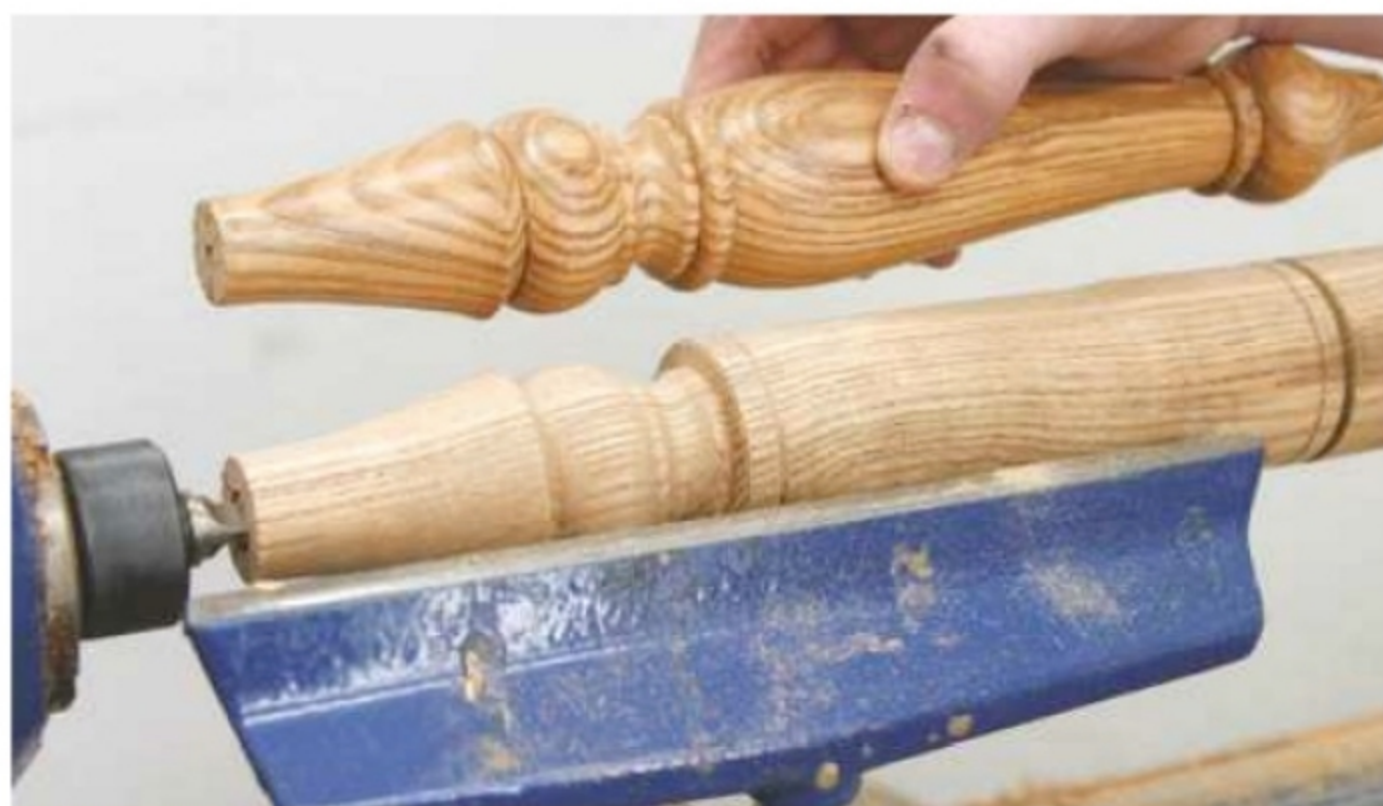
30. As you work, check your progress with the first leg held alongside the piece you're turning
