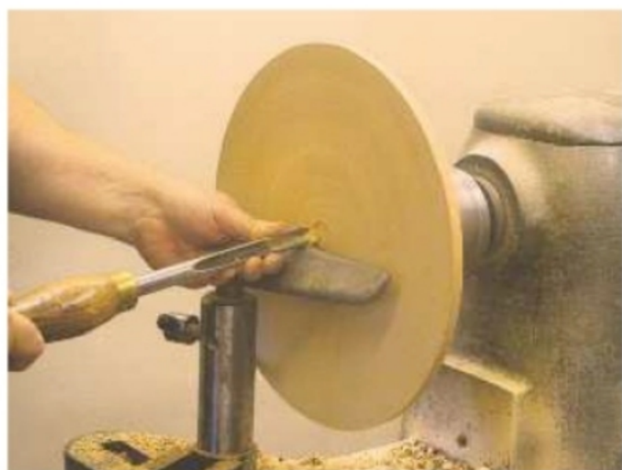
10. Start the hollowing-out cut to the left of centre, using the point of the tool
