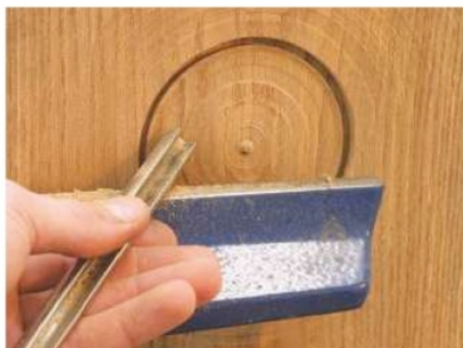
5. Form a recess in the centre of the disc to take the expanding jaws of your chuck
