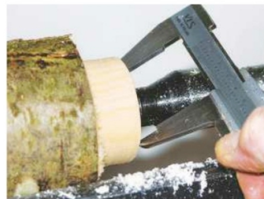
5. Stop the lathe and use callipers to check that the length and diameter of the spigot are correct
