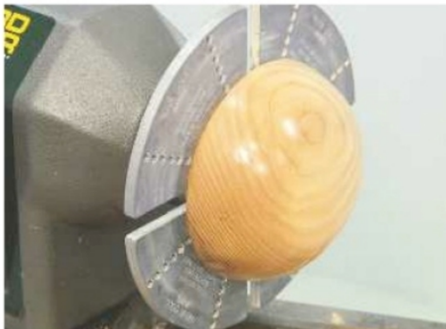
19. Sand, seal and finish the outside surface as you did for the inside
