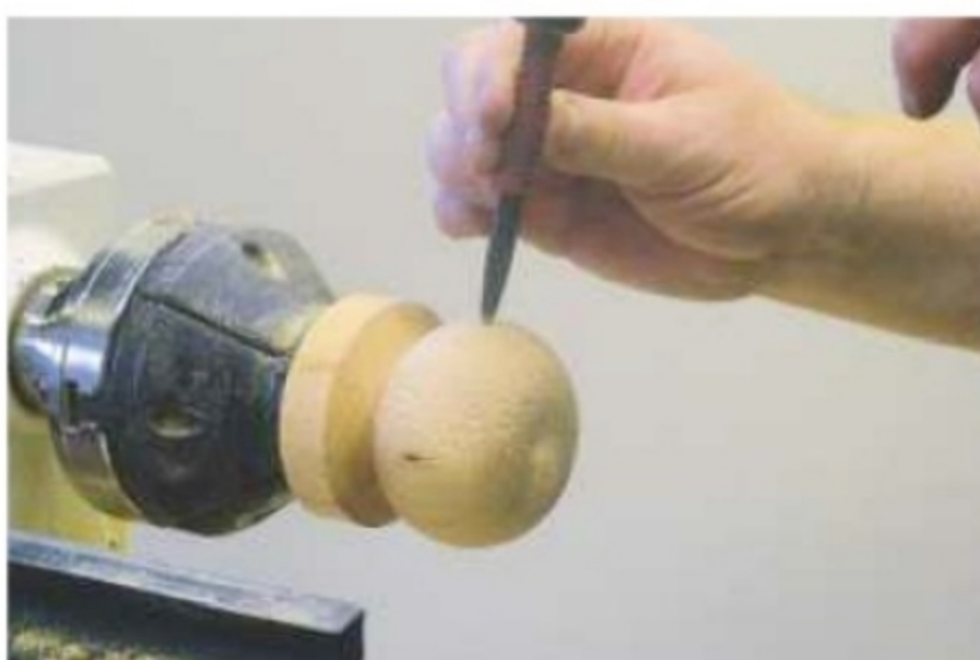
12. Stipple the surface all over using a hammer and rounded punch
