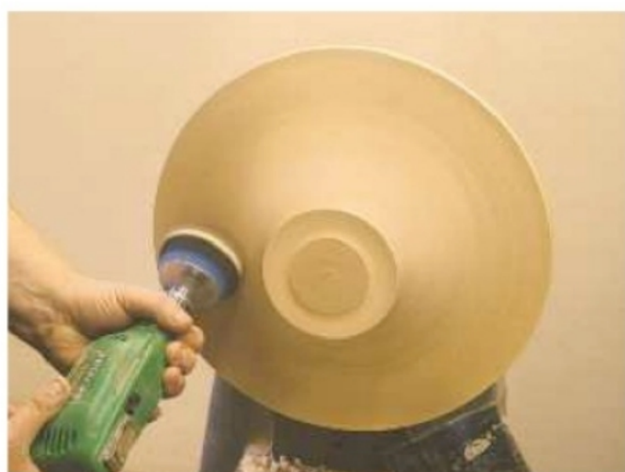
7. Power-sand the base using the bottom edge of the abrasive disc
