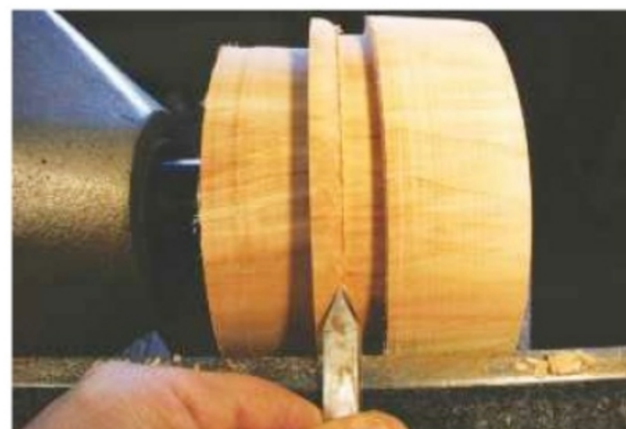
7. Form the convex curve on the edge of lid with the parting tool on its side
