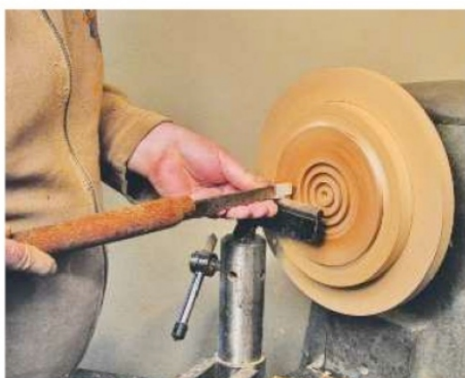
7. Cut a series of concentric grooves in the blank using a parting tool
