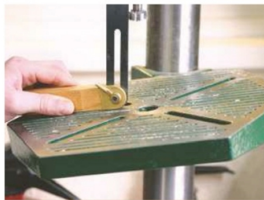
10. If you have a drill press, tilt the table to the desired angle; 10° is about right
