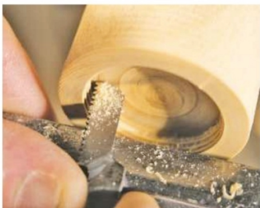
7. At the end of the thread run, push the chaser clear of the threads
