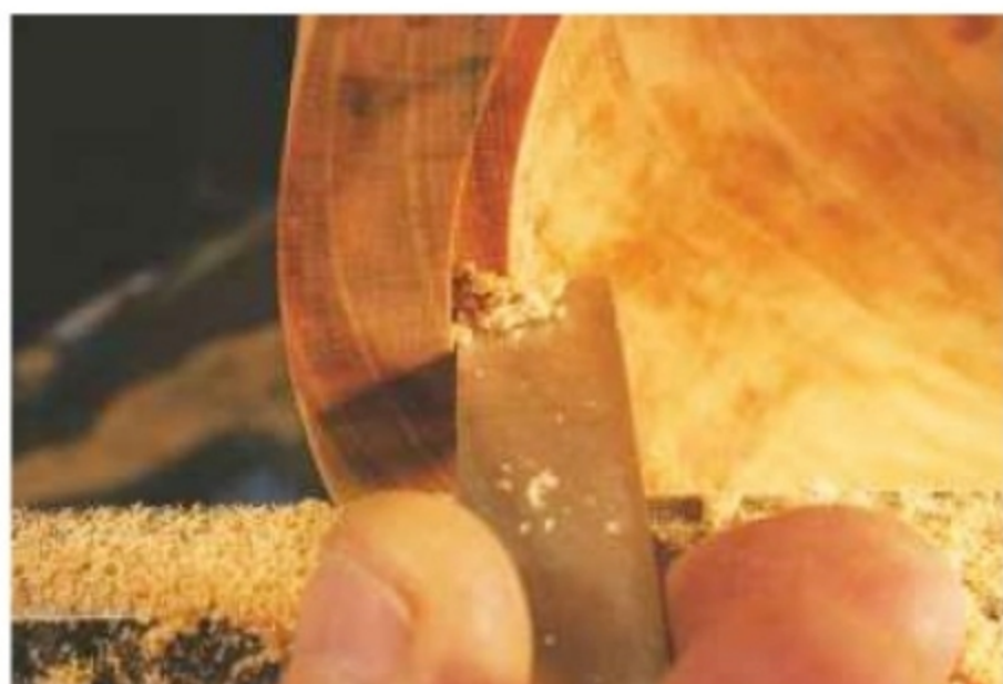
5. Form a rebate round the inside edge of the lid using a square scraper
