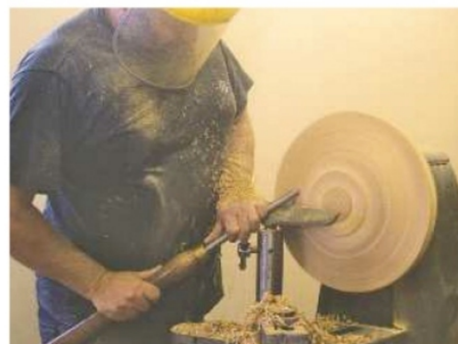
3. Start the cut in the centre and work slowly towards the edge
