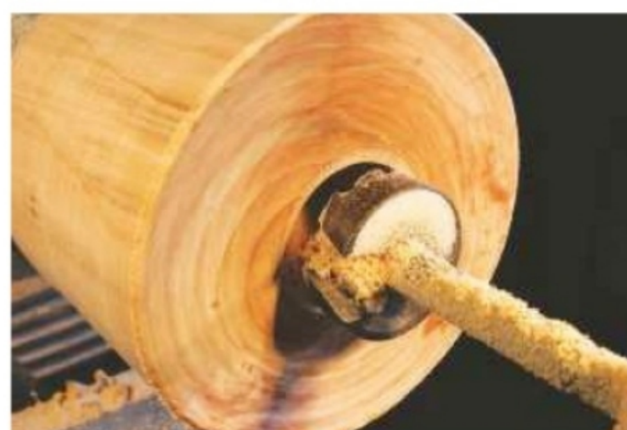
11. Bore a pilot hole in the base with a saw-toothed centre bit held in the tailstock
