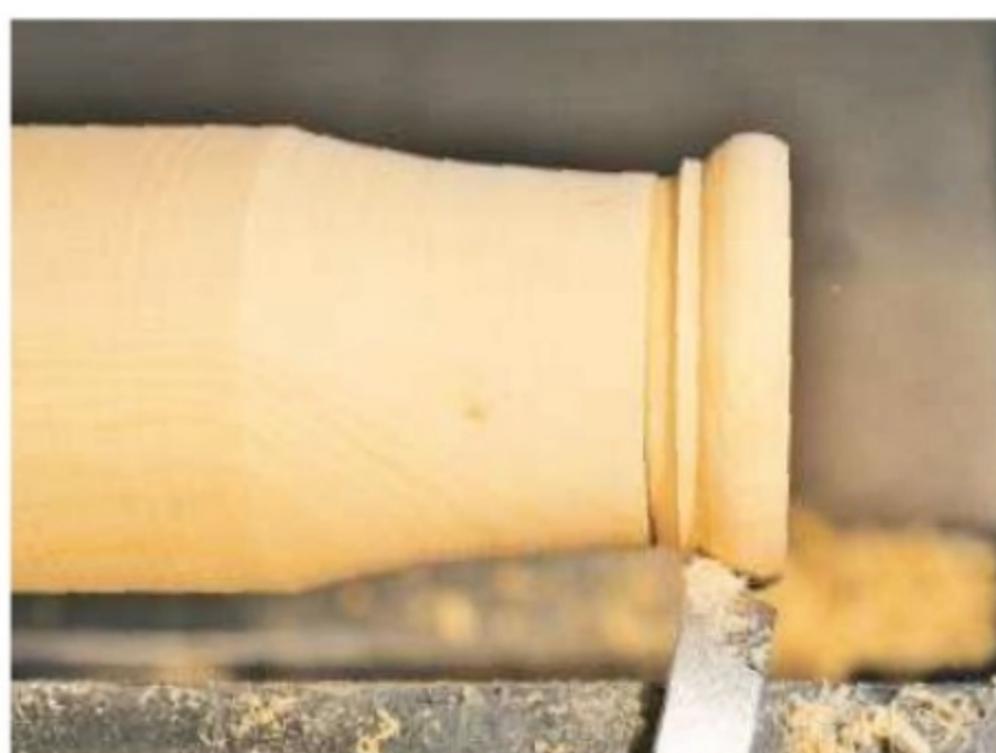
16. Leave the lid screwed on while you form its decorative mouldings
