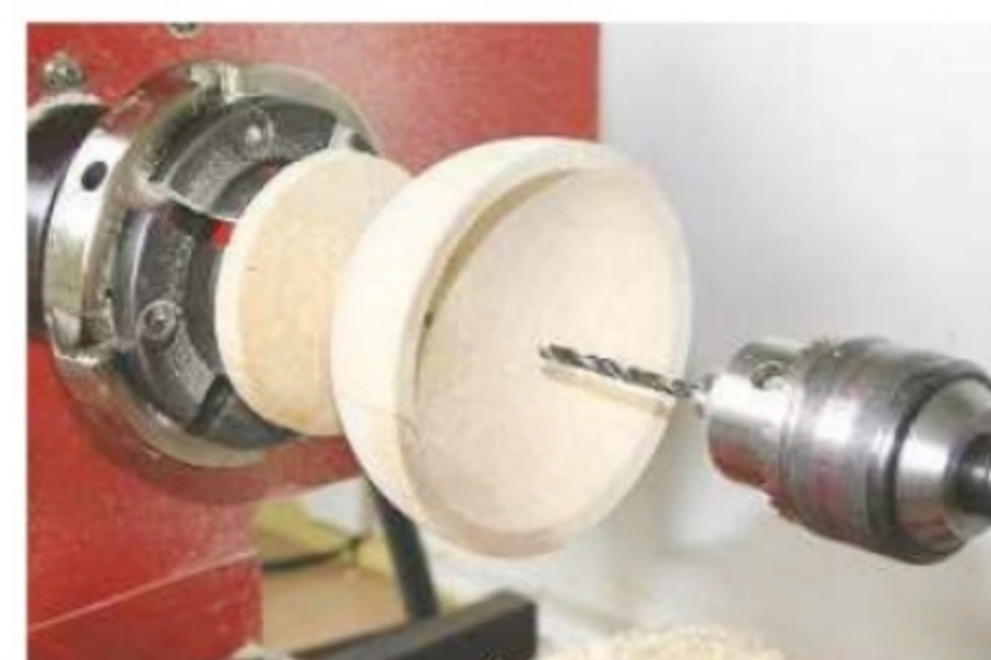
7. Drill a 6mm diameter hole in the centre of the top half...
