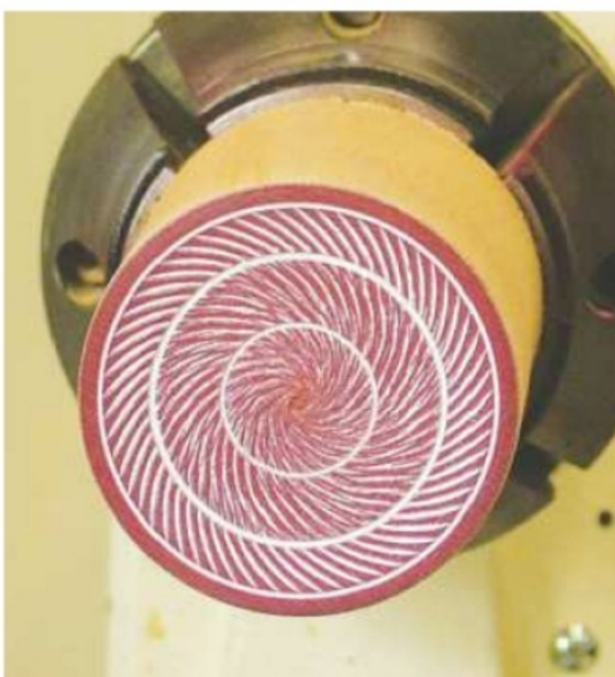
6. You can make the texture stand out even further by rubbing in some liming wax and then cleaning off the excess with oil
