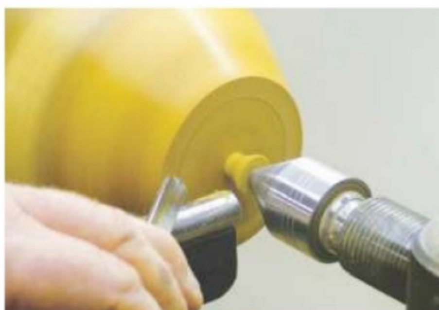
20. Use a spindle gouge to reduce the spigot and leave just a small stub to be chiselled off
