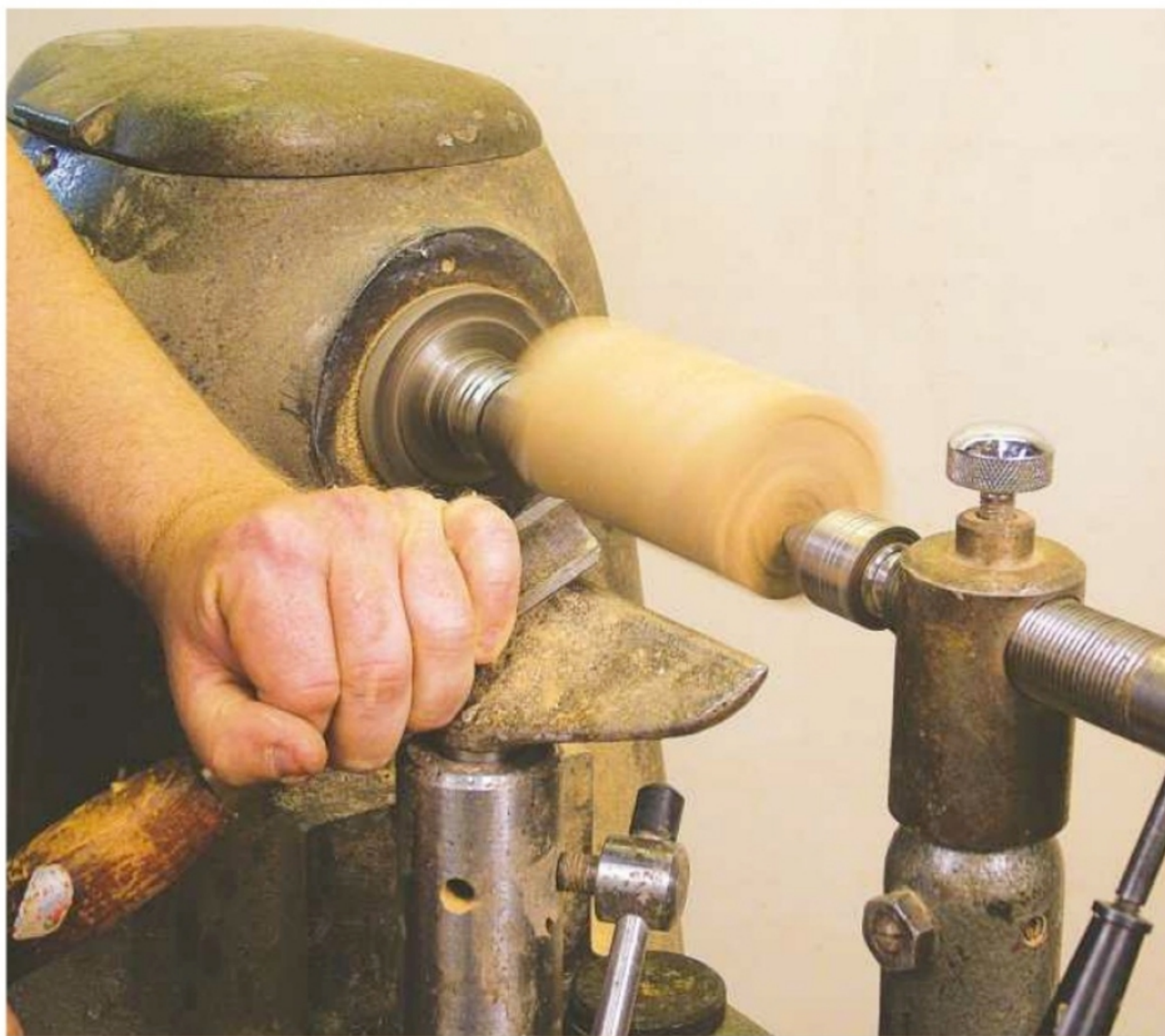
5. Mount the blank and use a spindle roughing gouge to start shaping the first face
