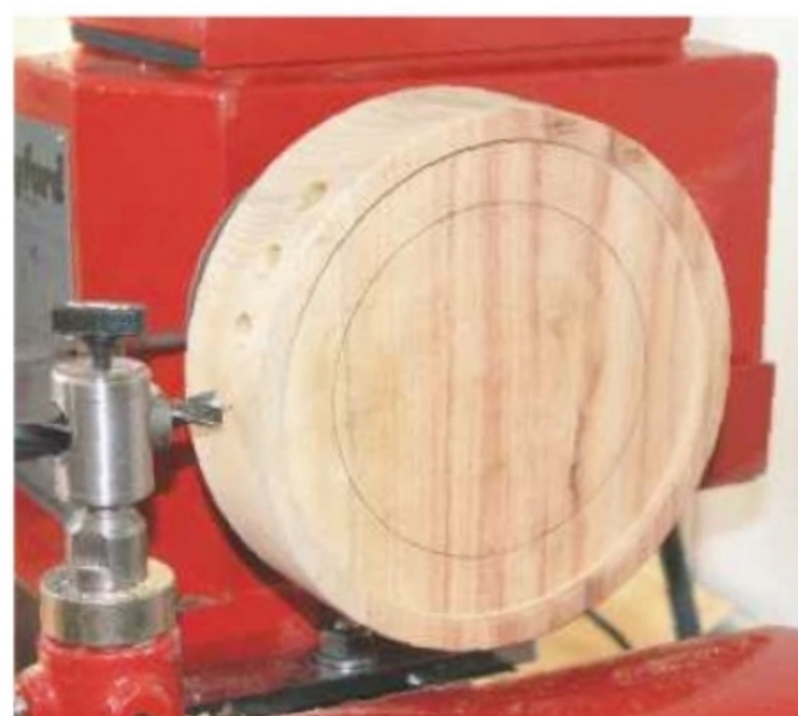
3. Drill a total of 24 holes to a depth of 25mm around the edge
