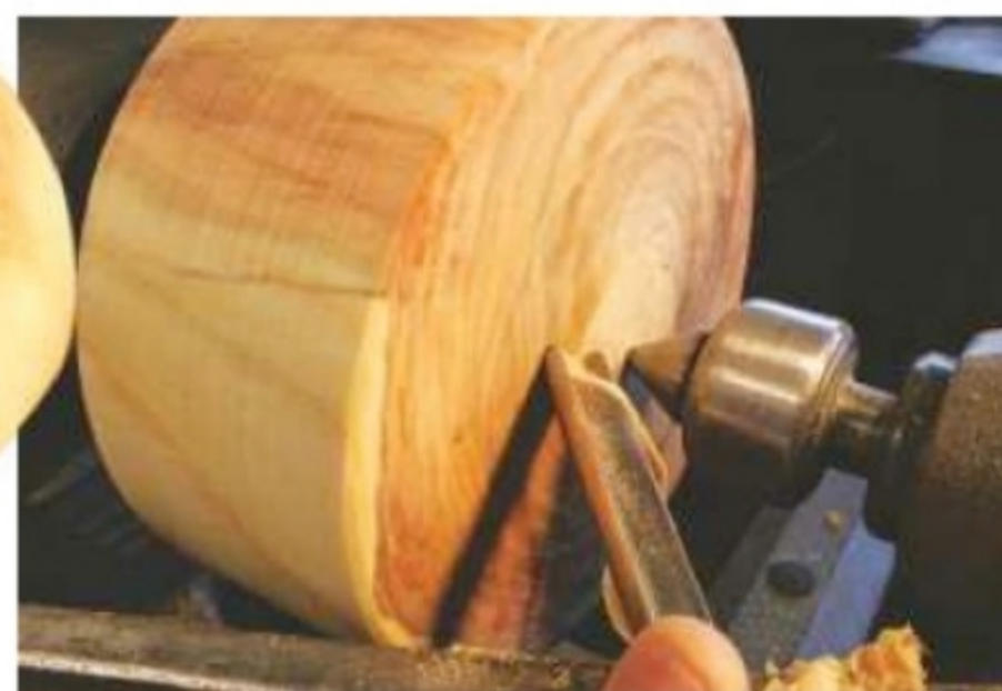
2. Rotate the toolrest through 45° and slice one end square with a bowl gouge
