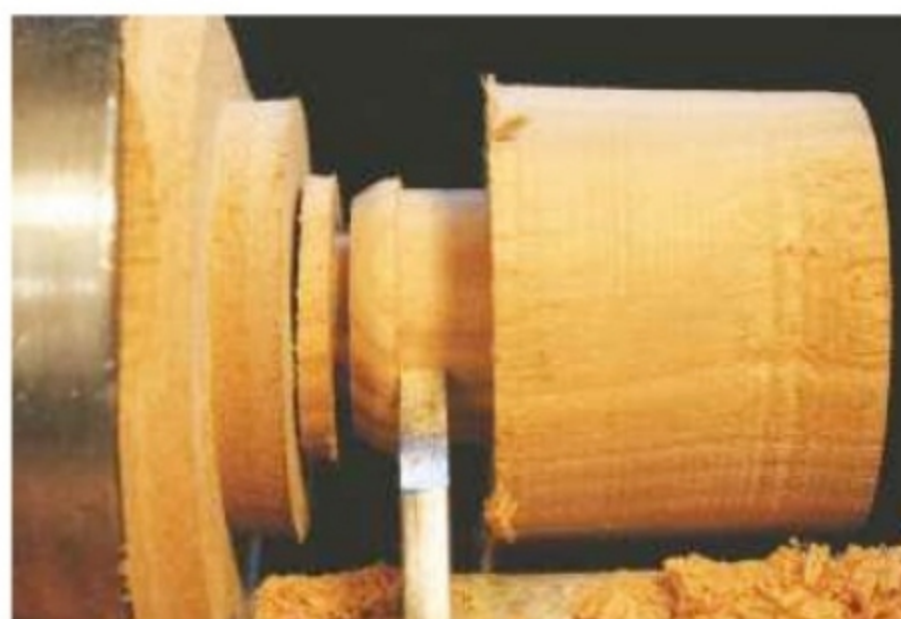
16. Turn the knob blank to a cylinder and form a lipped spigot on the inner end
