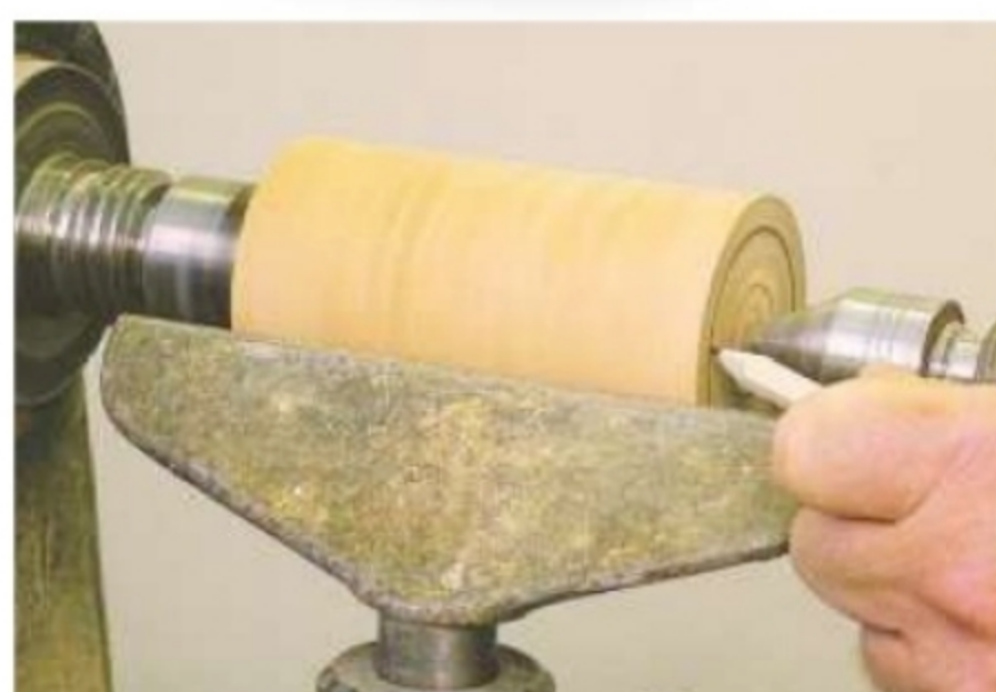
1. After turning the blank to a cylinder, mark two circles on each end at 25 and 50mm diameters
