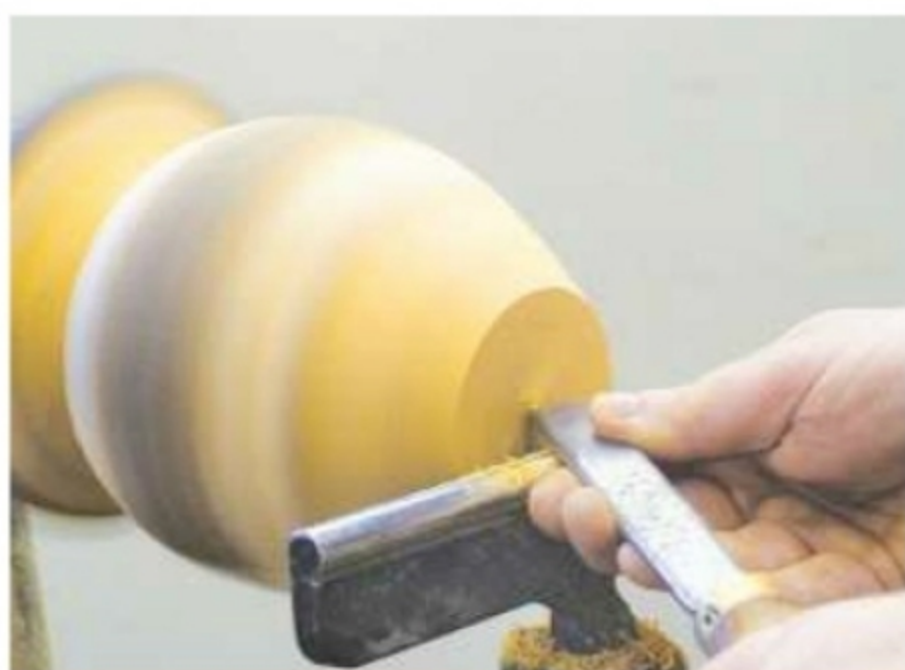
7. Clean up the base and mark the centre using the point of a skew chisel
