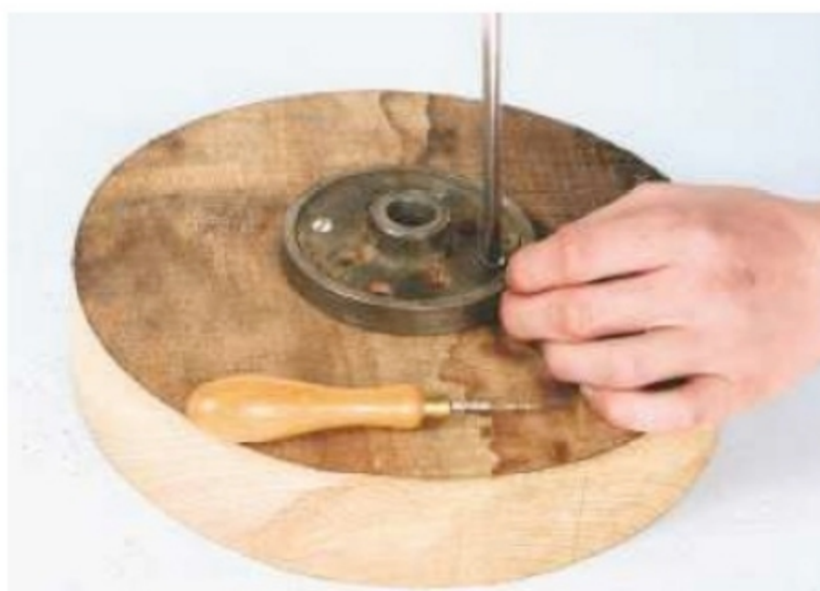
3. Screw on the faceplate using the shortest possible screws. Use a bradawl for the pilot holes
