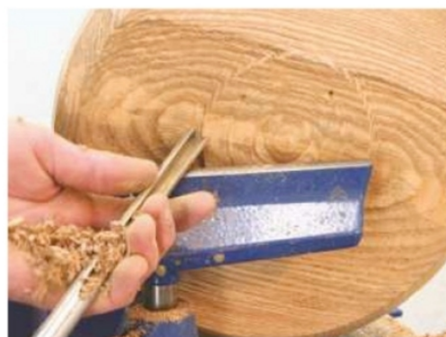
16. Dish the top to remove any trace of the faceplate fixing screws
