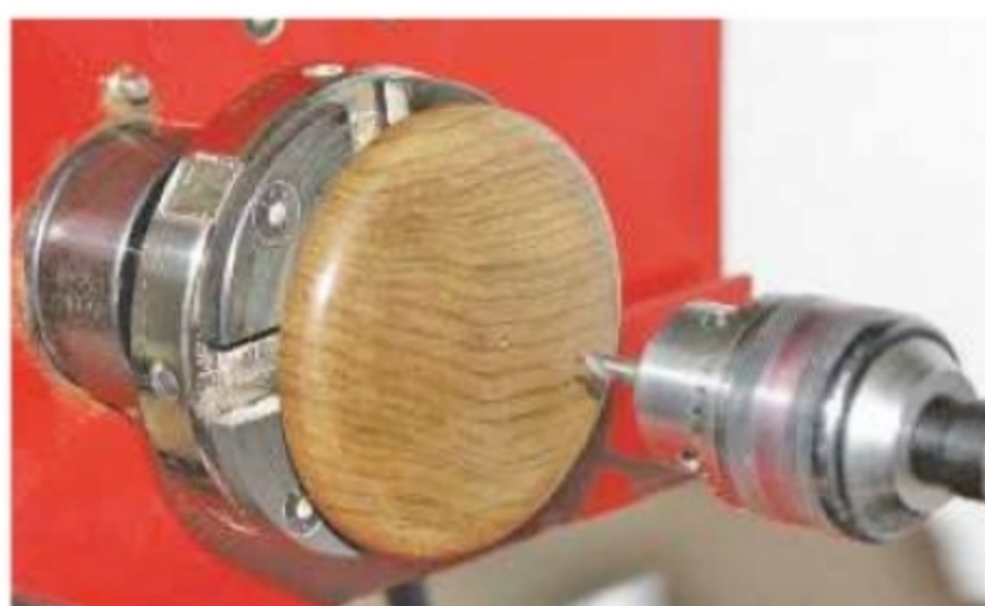
13. Shape the top into a slight dome and drill a hole for the knob spigot
