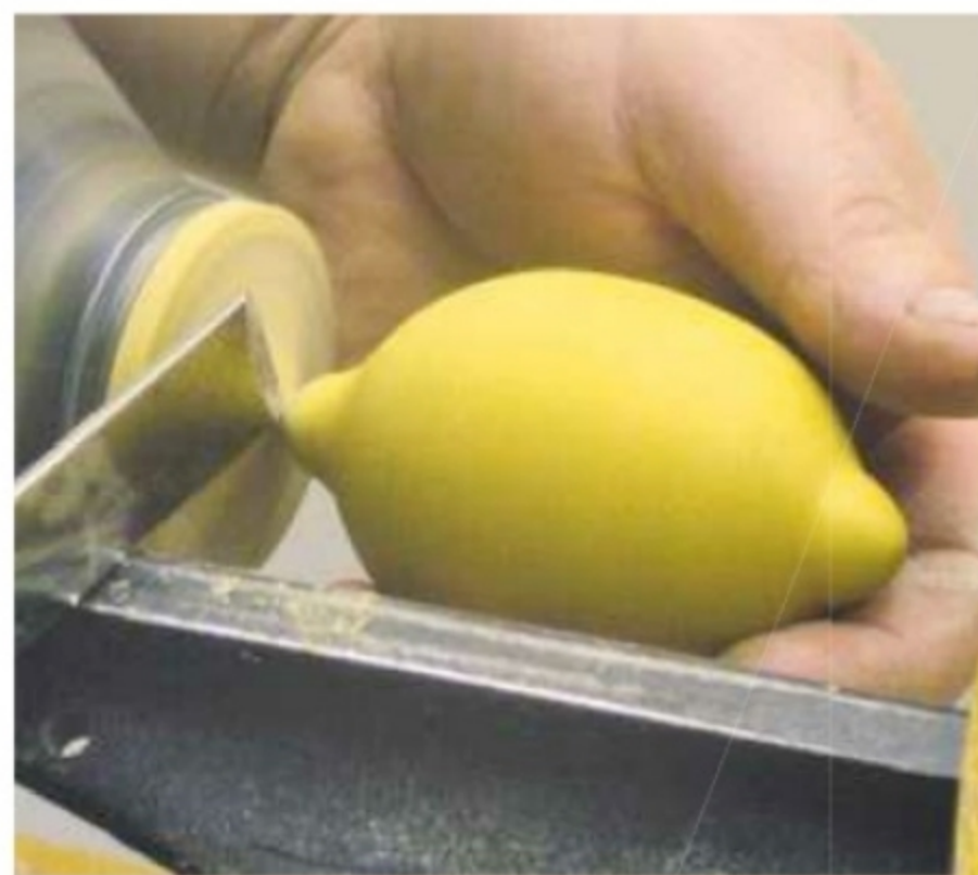
9. Shape the last part of the lemon using just the tip of the skew to avoid a dig-in
