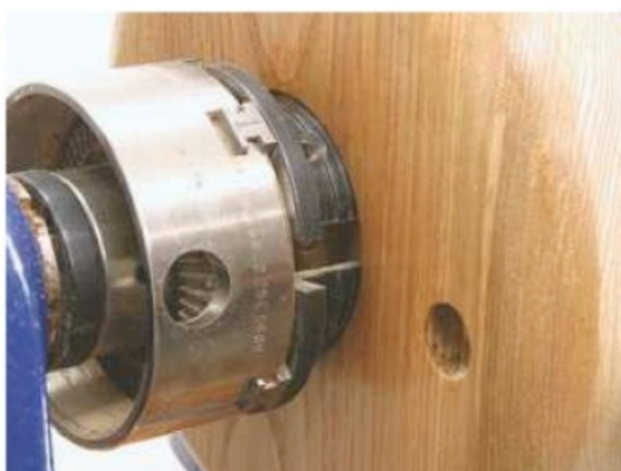
15. Reverse the top onto the expanding chuck and make sure it's well seated in the recess
