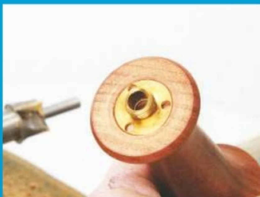
B. Mark and drill pilot holes, then screw the plate into place
