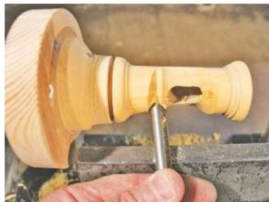
21. Cut in from each side of the hollow so you don't dislodge the work
