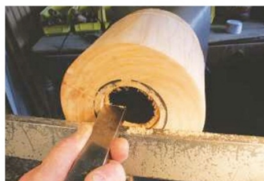
14. Reverse the base onto a jam chuck and complete the hollowing-out process
