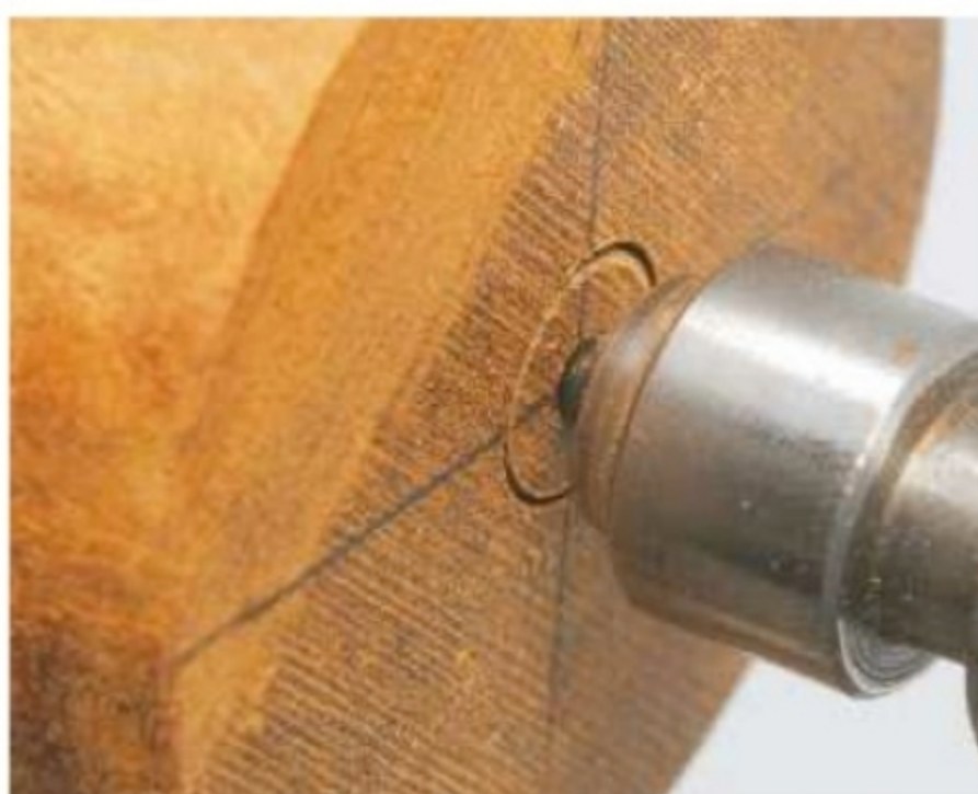
8. ...and the centre ring starts to bite into the end of the blank
