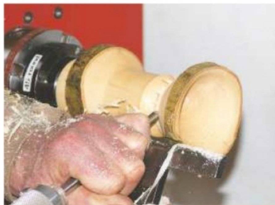
9. Use the same gouge to turn the outside of the bowl, working down towards the stem
