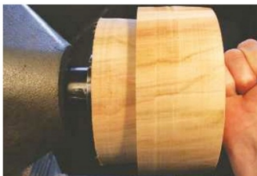
6. Part off the work and mount it onto a jam chuck held on a faceplate
