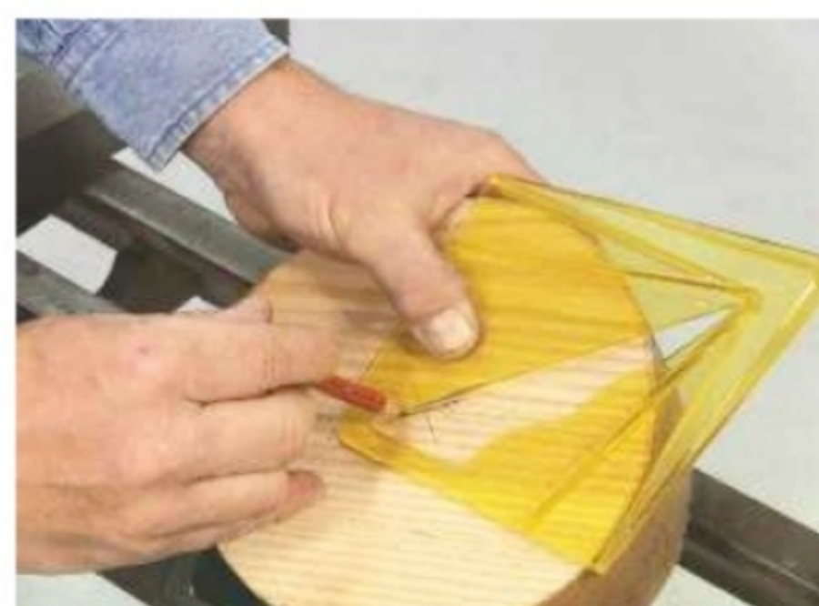
2. I used a proprietary centre finder to mark the blank's exact centre...
