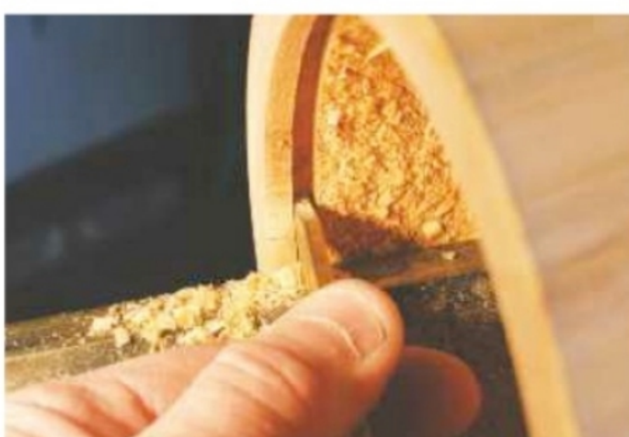
13. Cut the housing groove in the base for the floor panel with a parting tool
