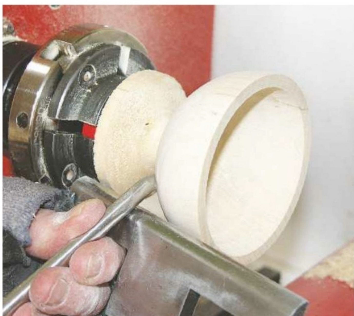
4. Switch to the bowl gouge and start to shape the outside of the hemisphere
