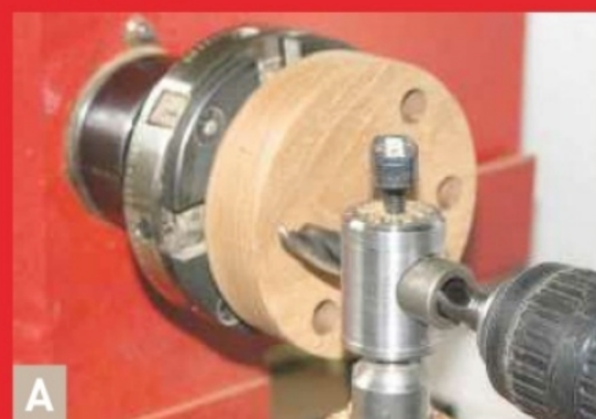
14. Mount the knob blank on a dowel to act as a spigot, then turn it to shape and apply the finish
