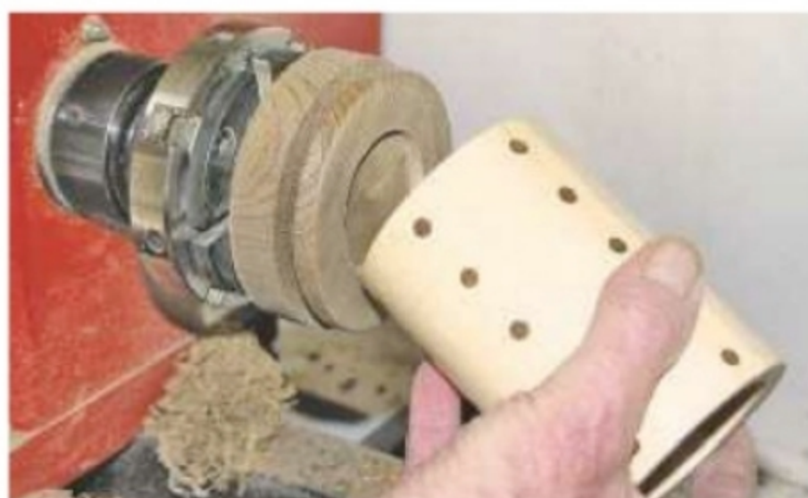
12. Turn a recess in the base blank to take the spigot on the pot base
