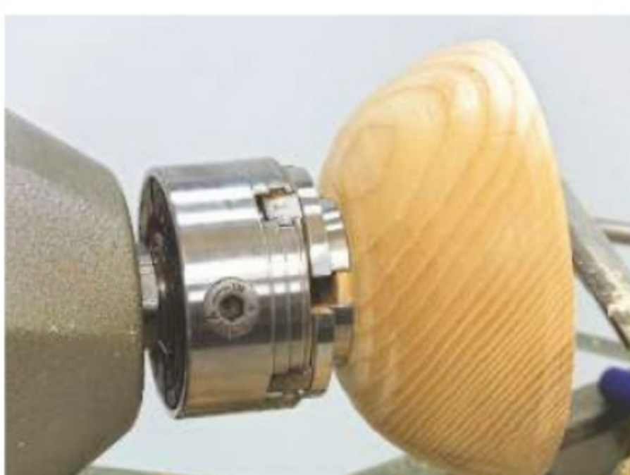
7. Form a temporary spigot on the base and reverse the bowl on the chuck
