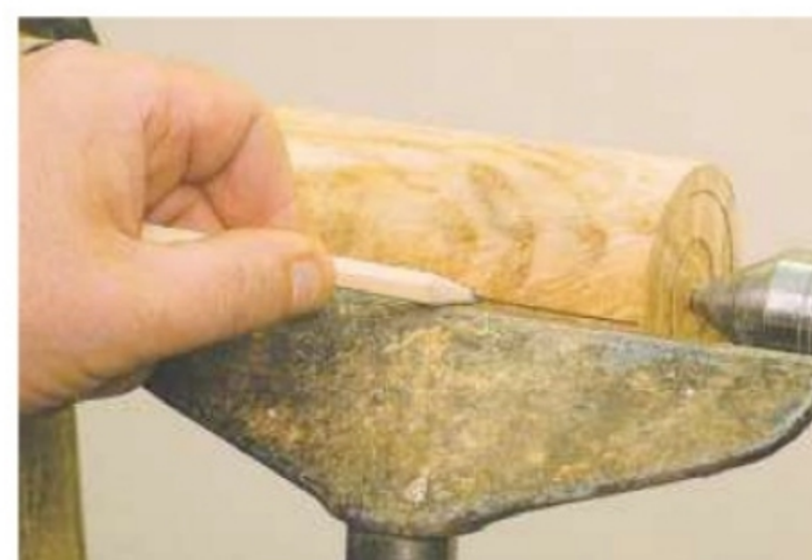
2. Use an indexing system if you have one to draw lines 120° apart on the sides of the blank
