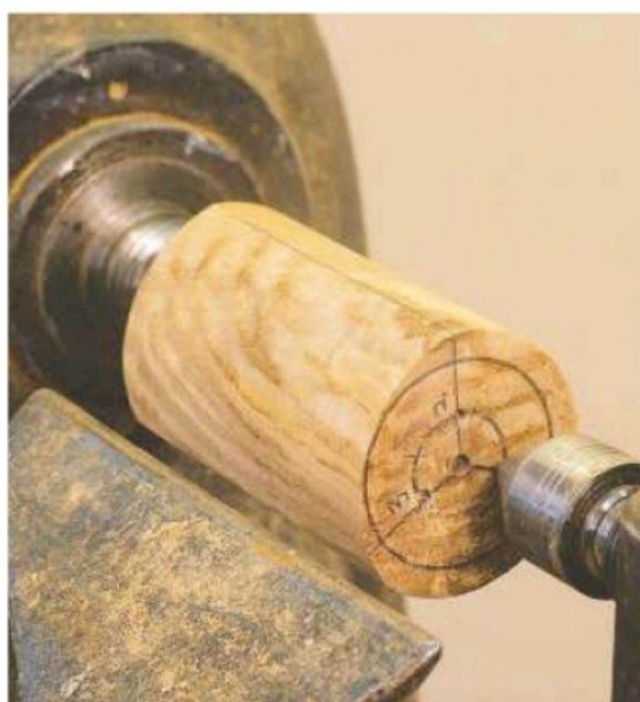
6. Continue cutting this face until the curve just touches the 50mm circle on the end of the blank
