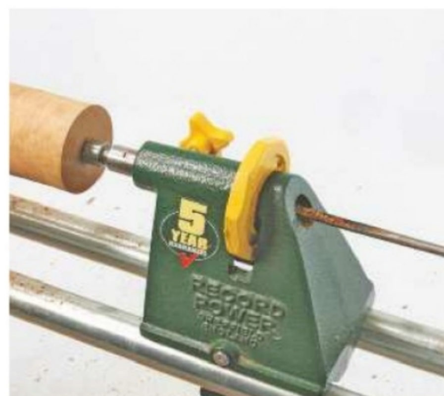
14. Bore about 20mm, then withdraw the auger to clear the swarf
