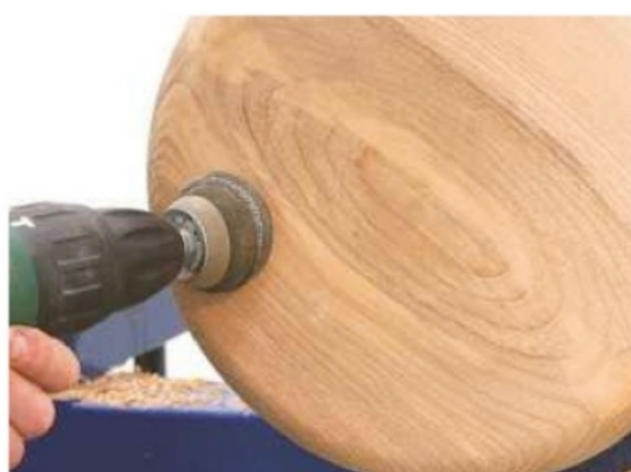
17. Power-sand the top with a Velcro pad, working down to 400 grit
