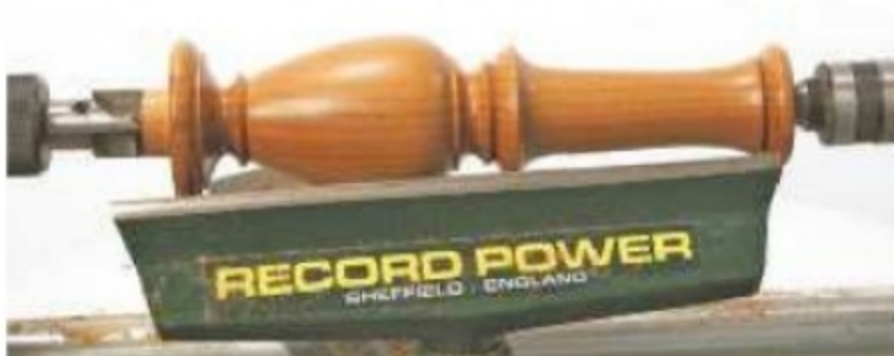
21. Fit a conventional revolving centre and complete the turning
