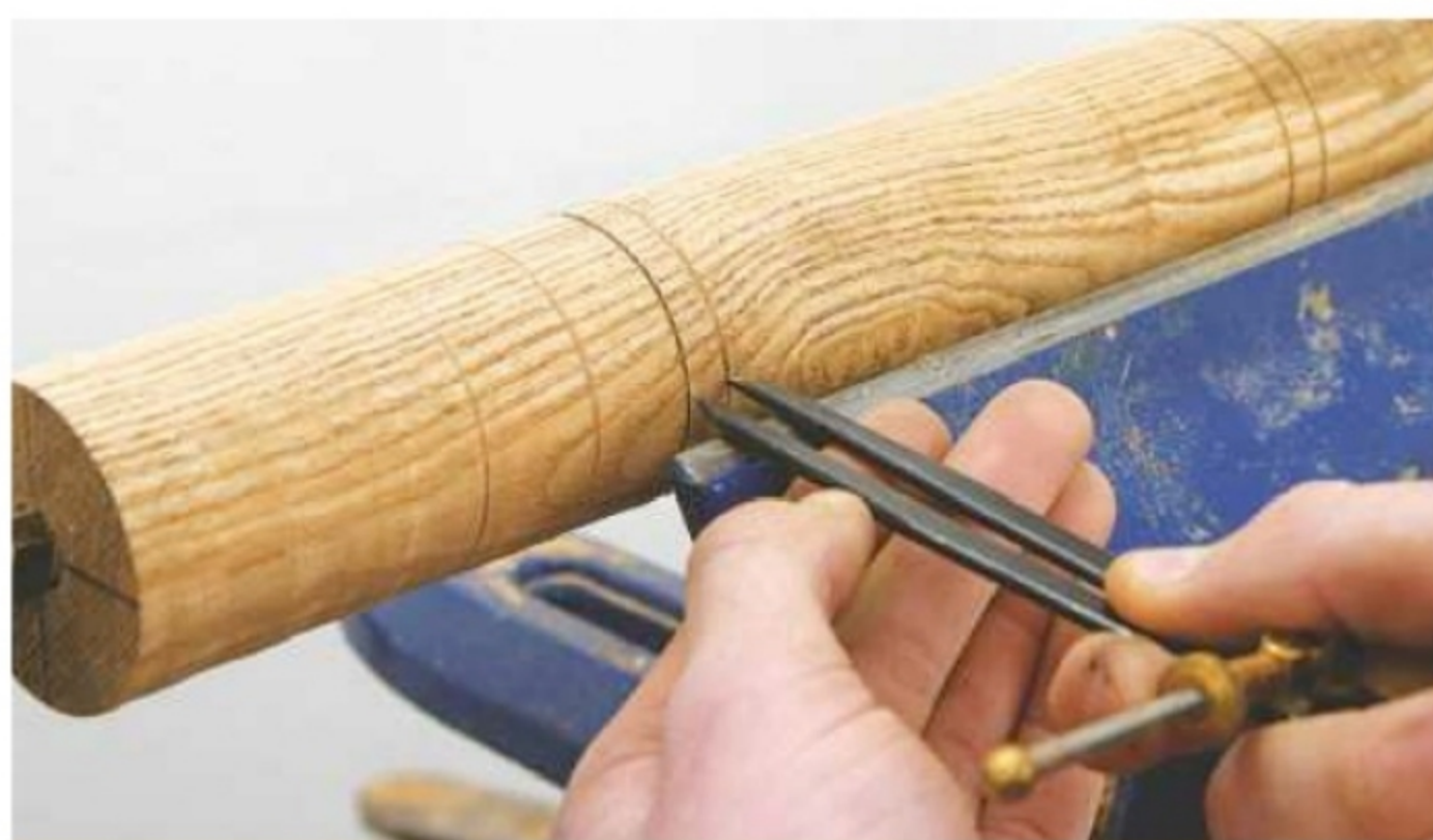
28. Reduce the second leg to a cylinder and mark the detail positions
