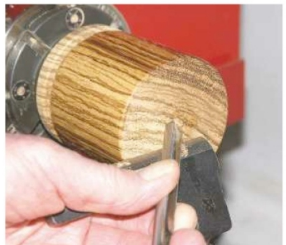
17. Reverse the body and tidy up the base
