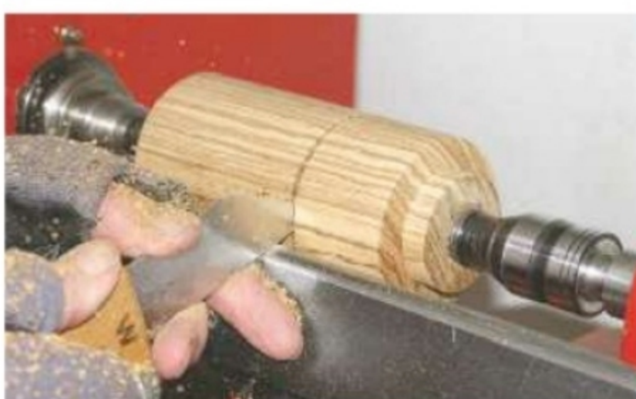
2. Part off the lid with a thin parting tool
