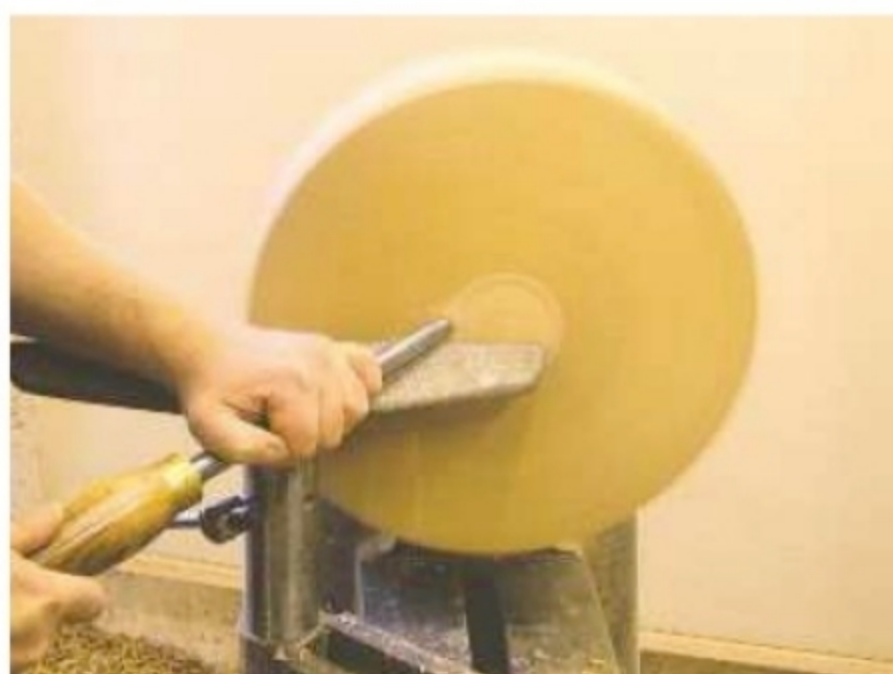
2. Face off the bottom using a pull cut with the 1/2in bowl gouge
