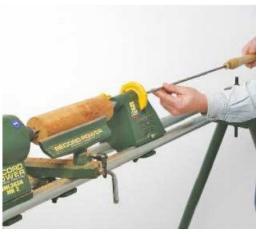
13. Apply firm pressure on the end of the auger to begin with
