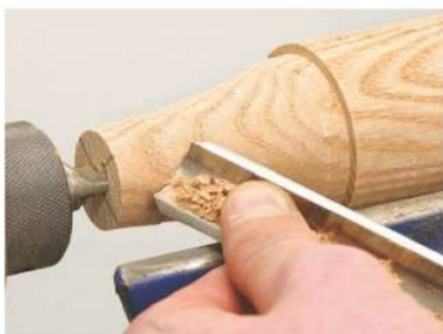
20. Use a mini drive centre so you can reduce the foot to a small diameter
