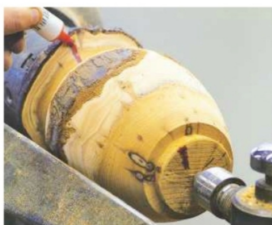
4. Make a reference mark on the vase and base so you can realign the grain later
