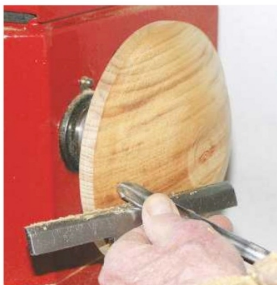
7. Reverse the blank and turn the top surface to a domed shape
