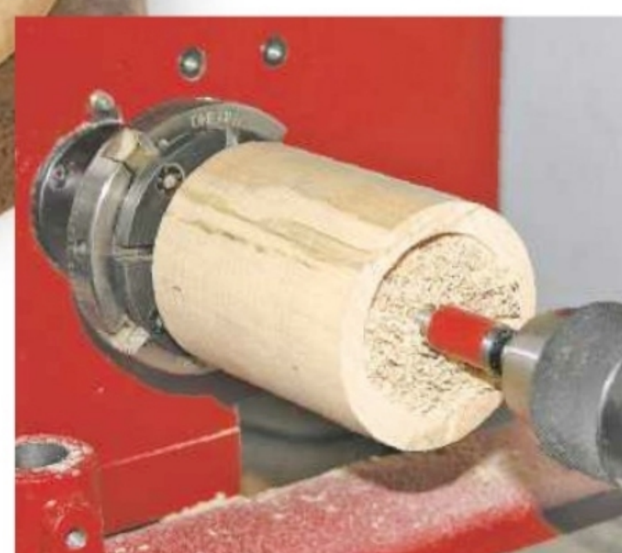
5. Withdraw the bit from time to time to clear out the shavings
