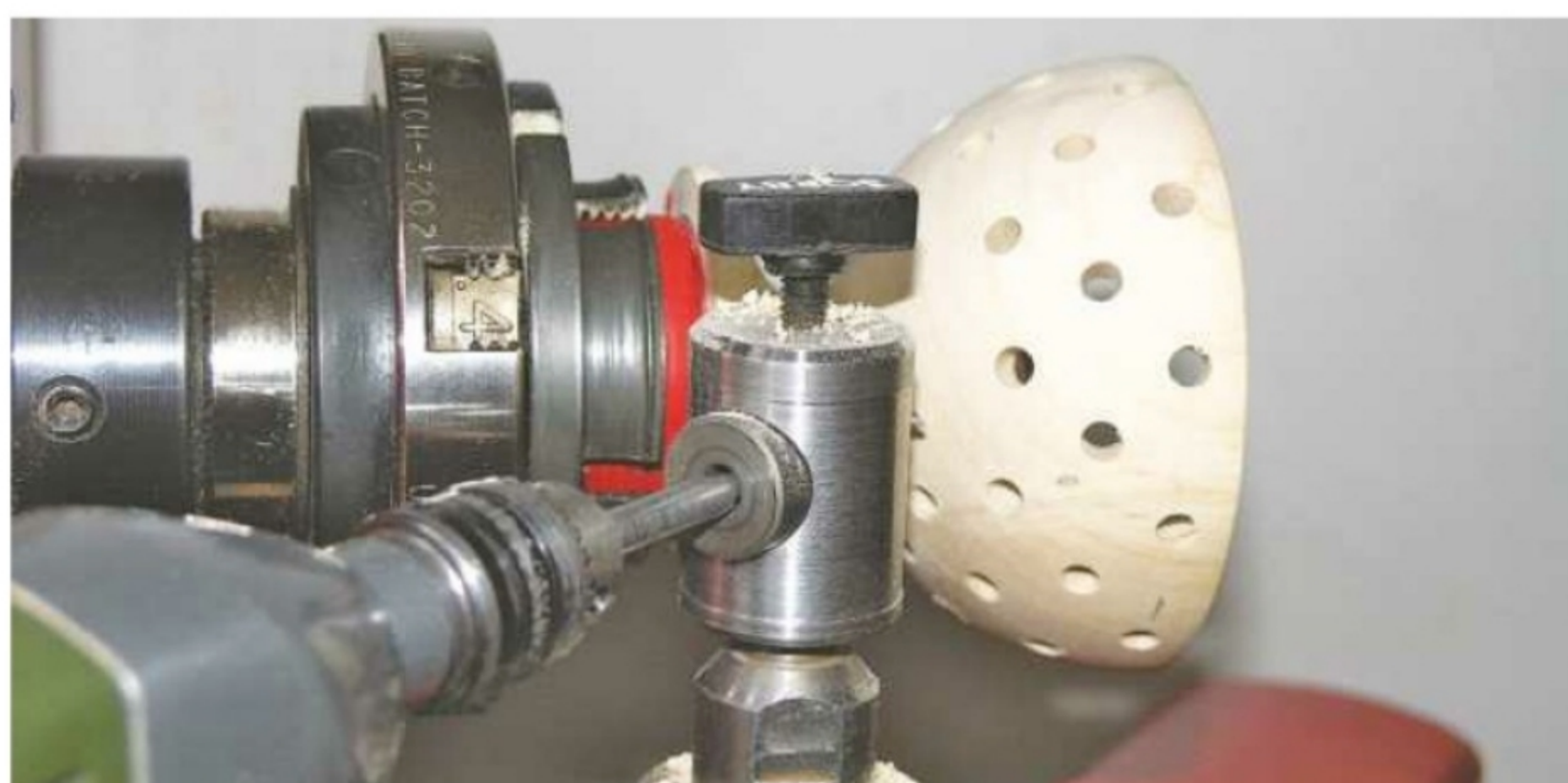
10. Move the jig for each row so the drill is always at 90° to the surface
