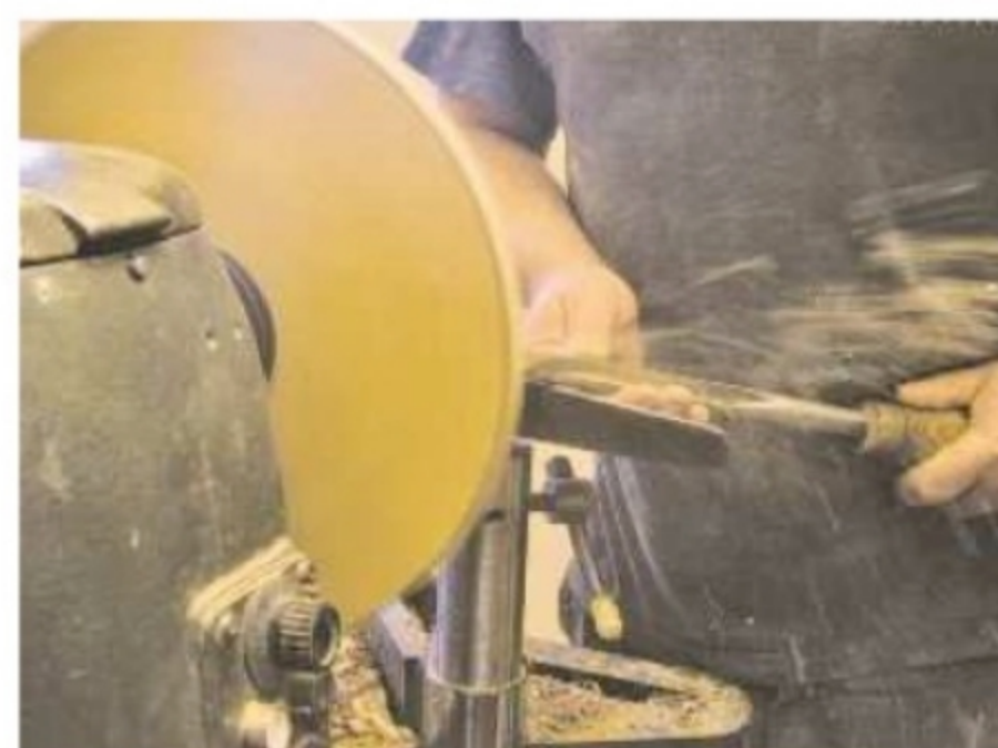
4. The first turning stage was to rough down the edge to get it balanced
