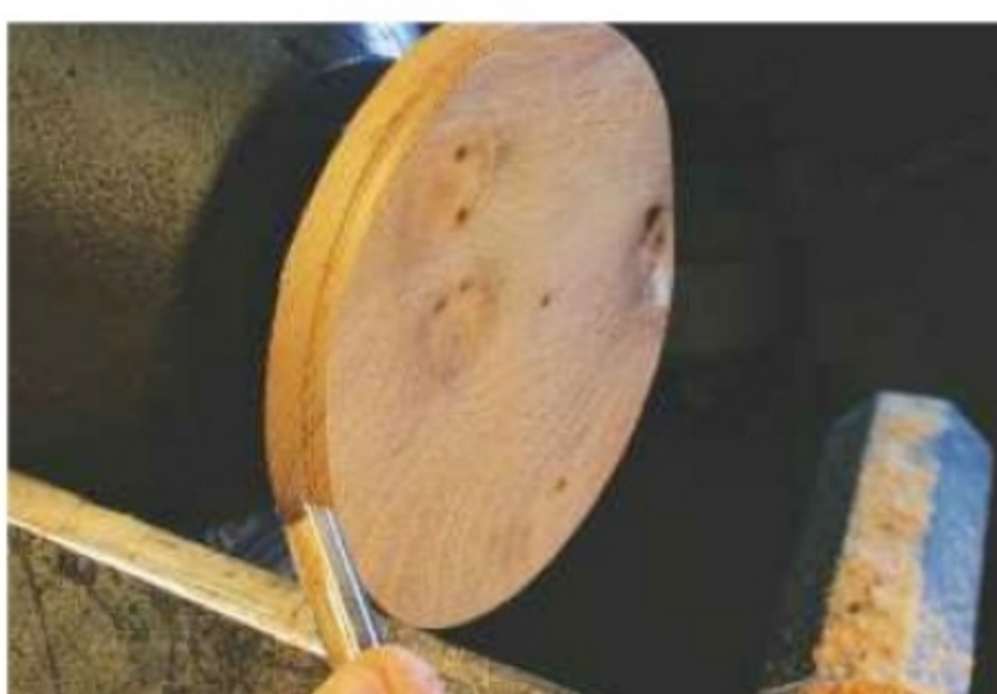
19. Cut the floor panel down to the diameter required and chamfer the edges
