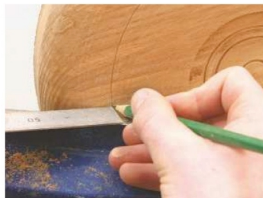
7. Mark a pencil line round the disc 40mm in from the edge to indicate where the legs will fit
