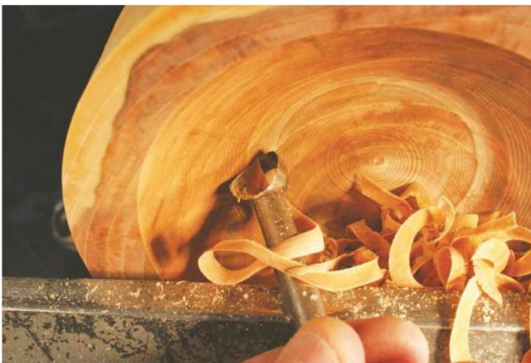
4. Use a ring tool to hollow out the inside of the lid; clear the shavings regularly
