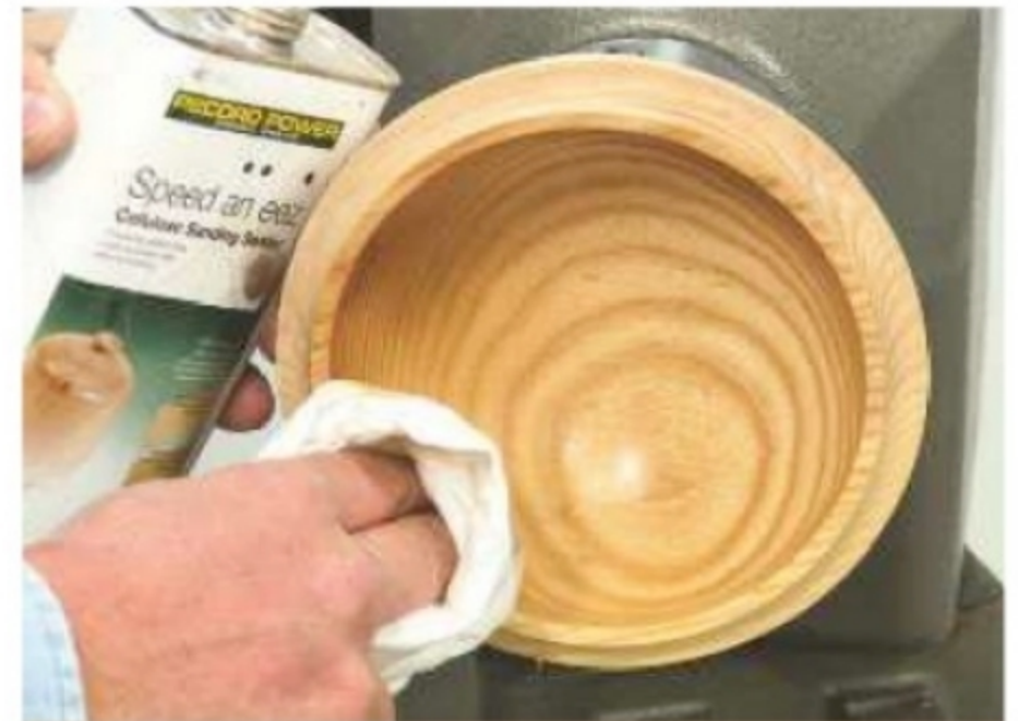
14. Apply several coats of cellulose sanding sealer with the lathe stationary
