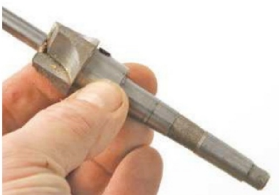
16. The counterbore tool is fitted with a central \frac{5}{16} in pilot
