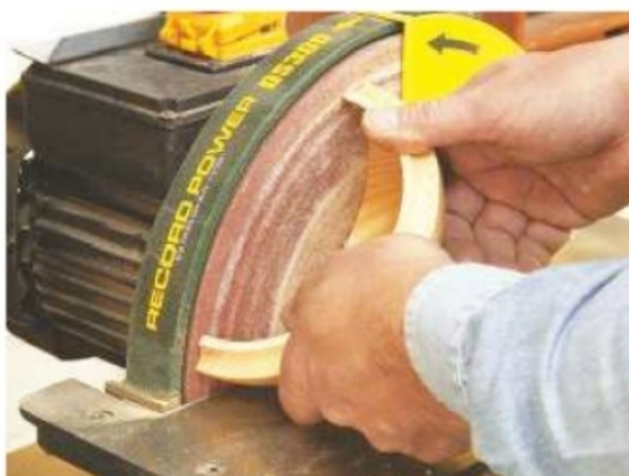
22. True up the two bandsawn faces on a disc sander to get a perfect join
