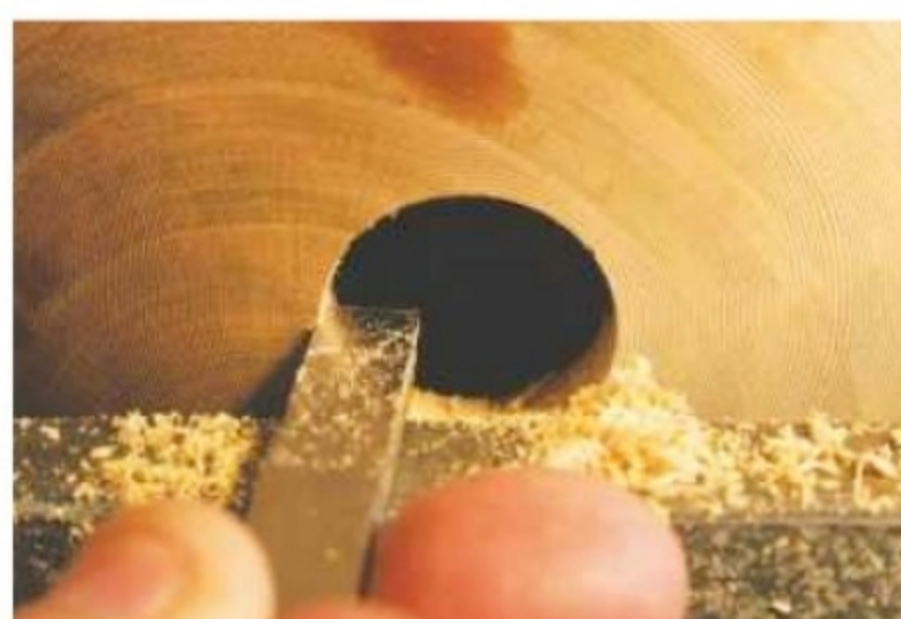
10. Form a hole in the lid for the knob and widen it with a small square scraper
