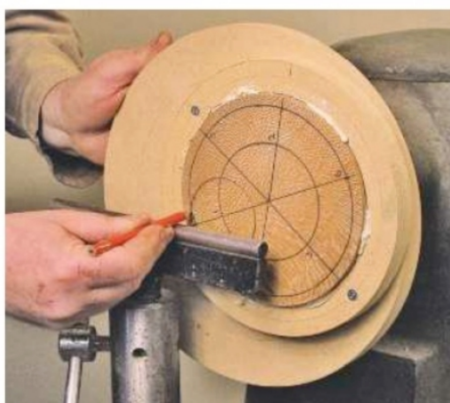
12. Rotate the MDF and use a pencil to mark the widest diameter circle round this centre
