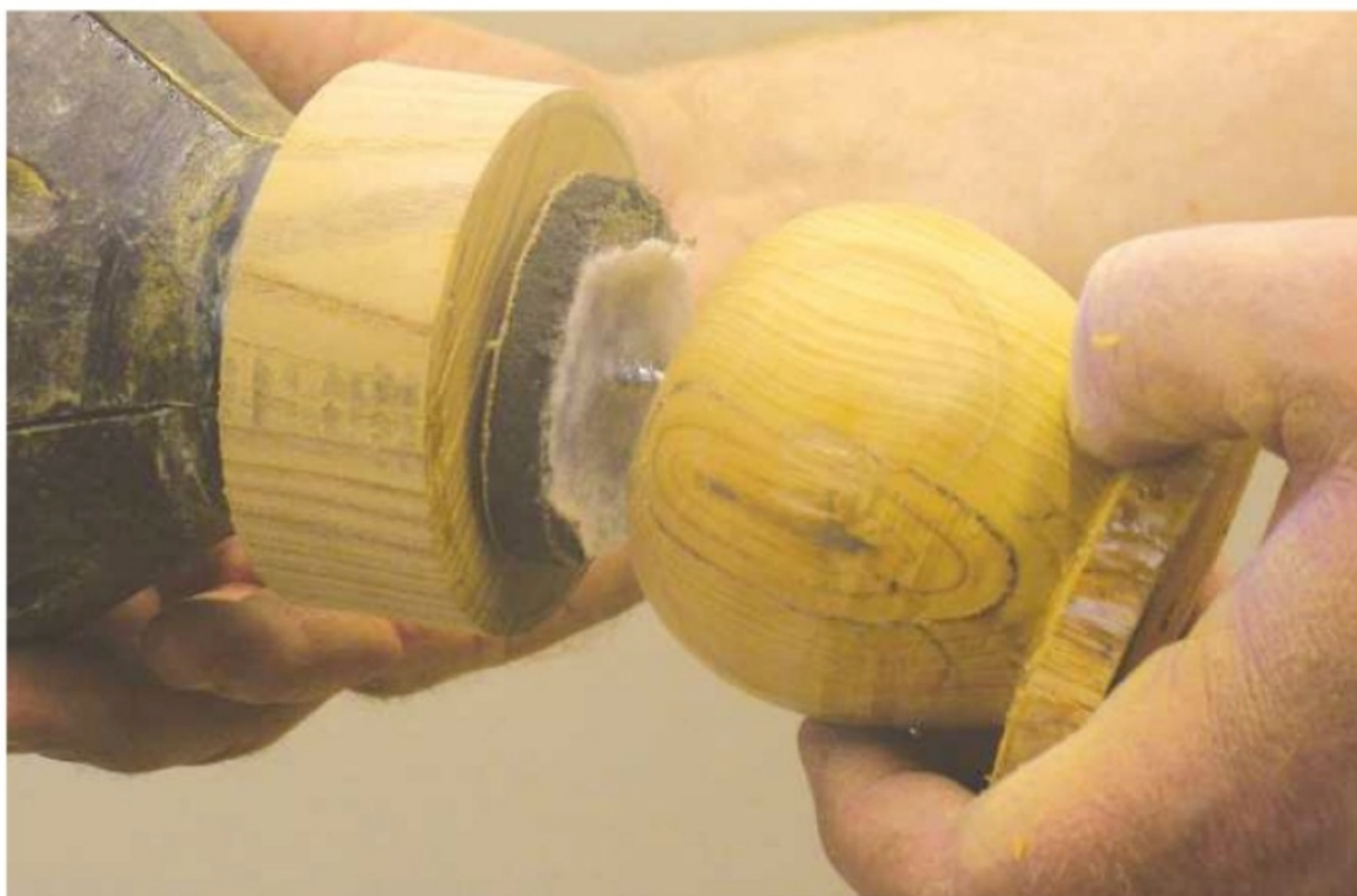
7. Reverse the blank, using a foam pad to protect the surface
