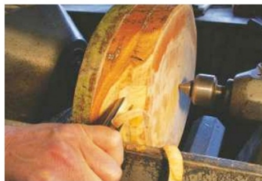
1. Turn the lid section to a cylinder; note the overhand grip for extra control
