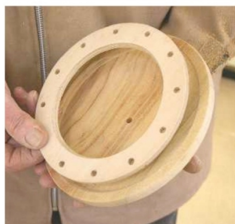
6. Form a rebate in the top and test the fit of the plywood ring in it
