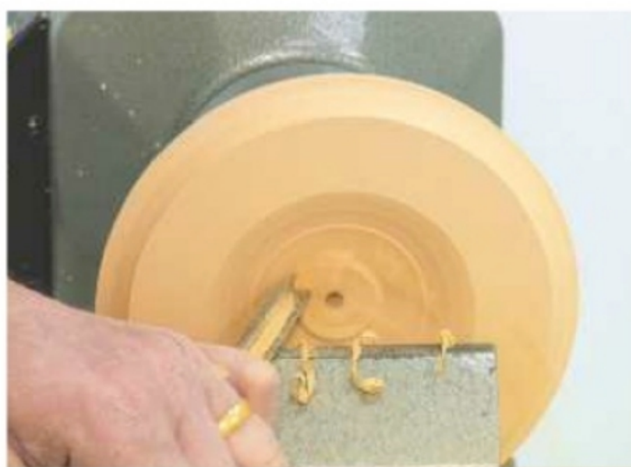
9. With the outer dimension established, start hollowing out the core of the bowl
