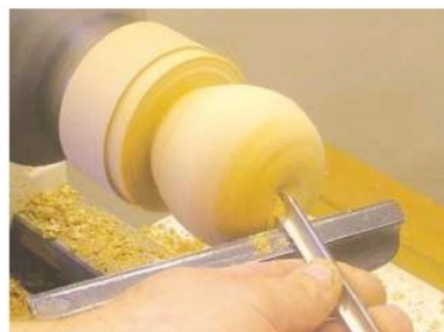
6. Use the bottom wing of the gouge to blend in the curve
