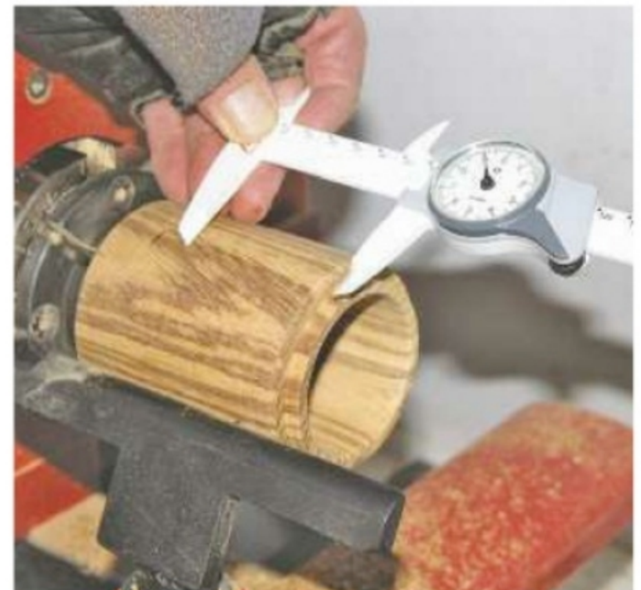
14. Mark the depth of the body with your callipers
