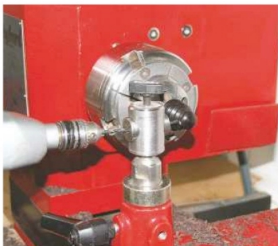
14. Drill a small hole through the top finial for the hanging cord
