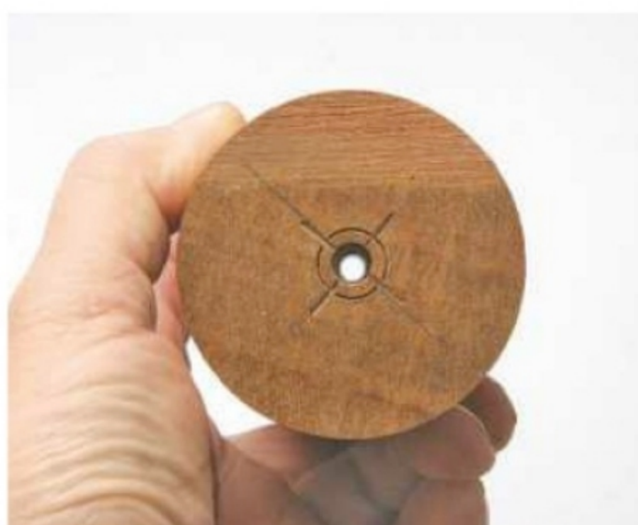
20. Take the blank off and check that the holes meet perfectly
