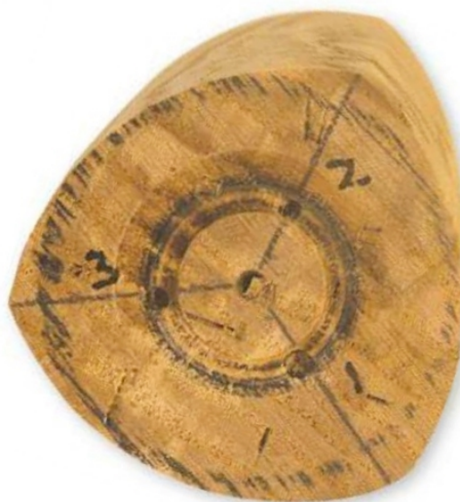
9. Repeat the process to curve the other two sides, and a blank like this will be the end result
