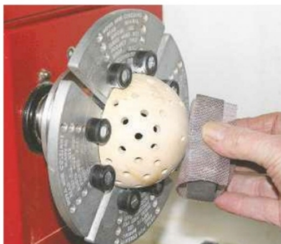
12. Mount each hemisphere on Cole jaws so you can remove the spigot and sand the surface smooth
