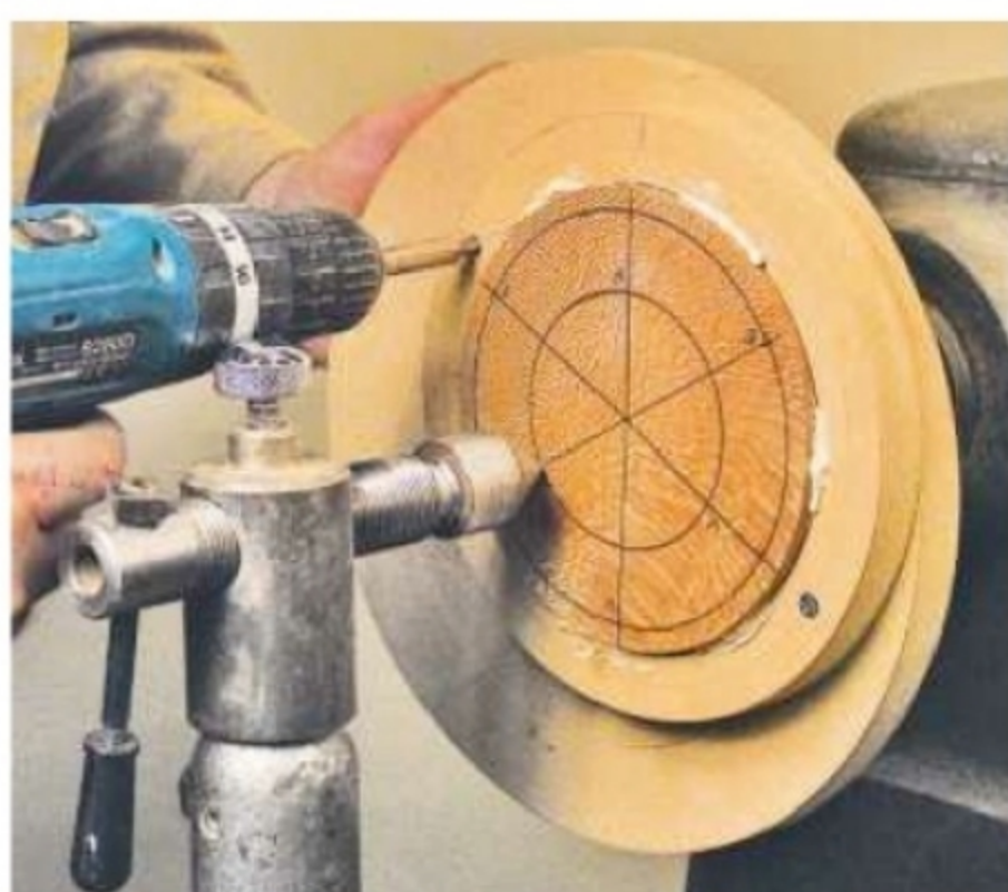
11. Move the jam chuck round the backing MDF until point 1 is centred on the lathe
