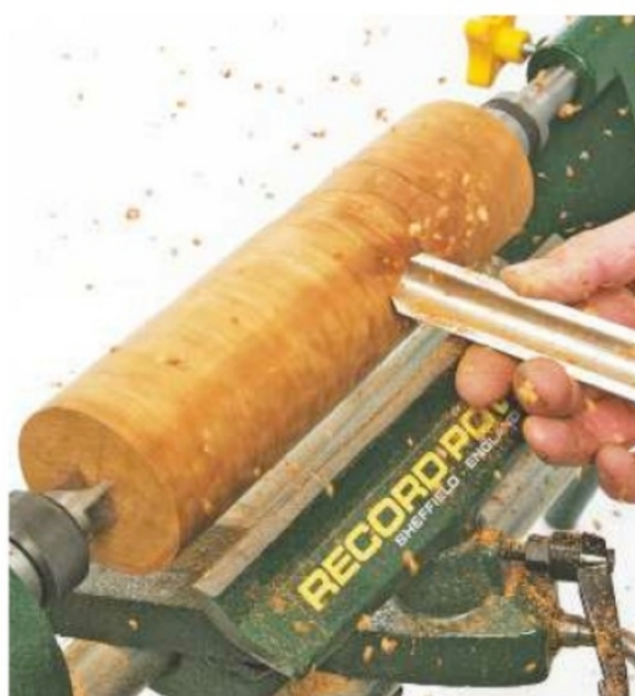
5. Run your index finger against the tool rest as a guide
