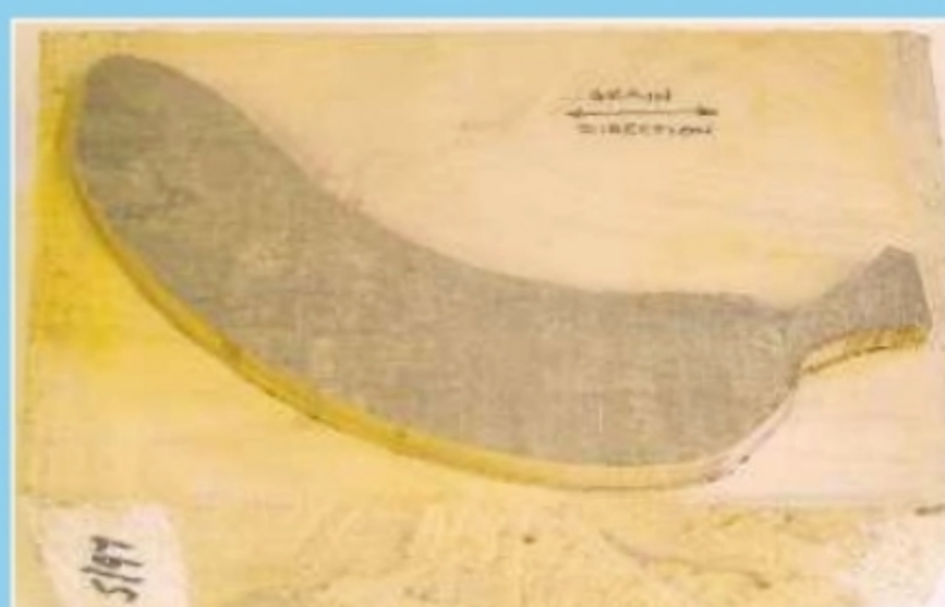
A. Draw round a real banana or a template. Note the grain direction
