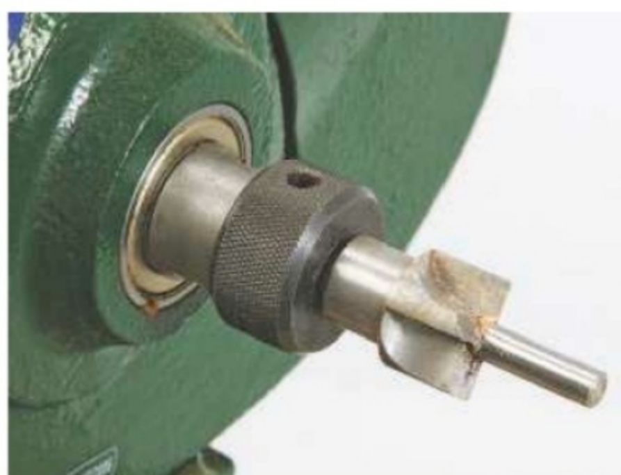
18. Fit the counterbore tool in the headstock and mount the blank
