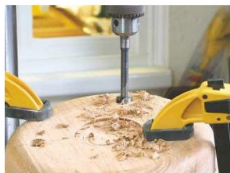
13. Clamp the blank securely to the table and drill the three leg holes in turn
