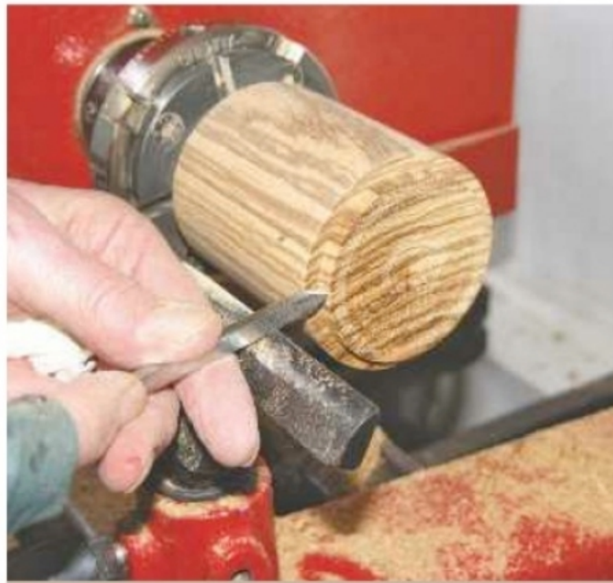
7. Mount the body and form a jam chuck
