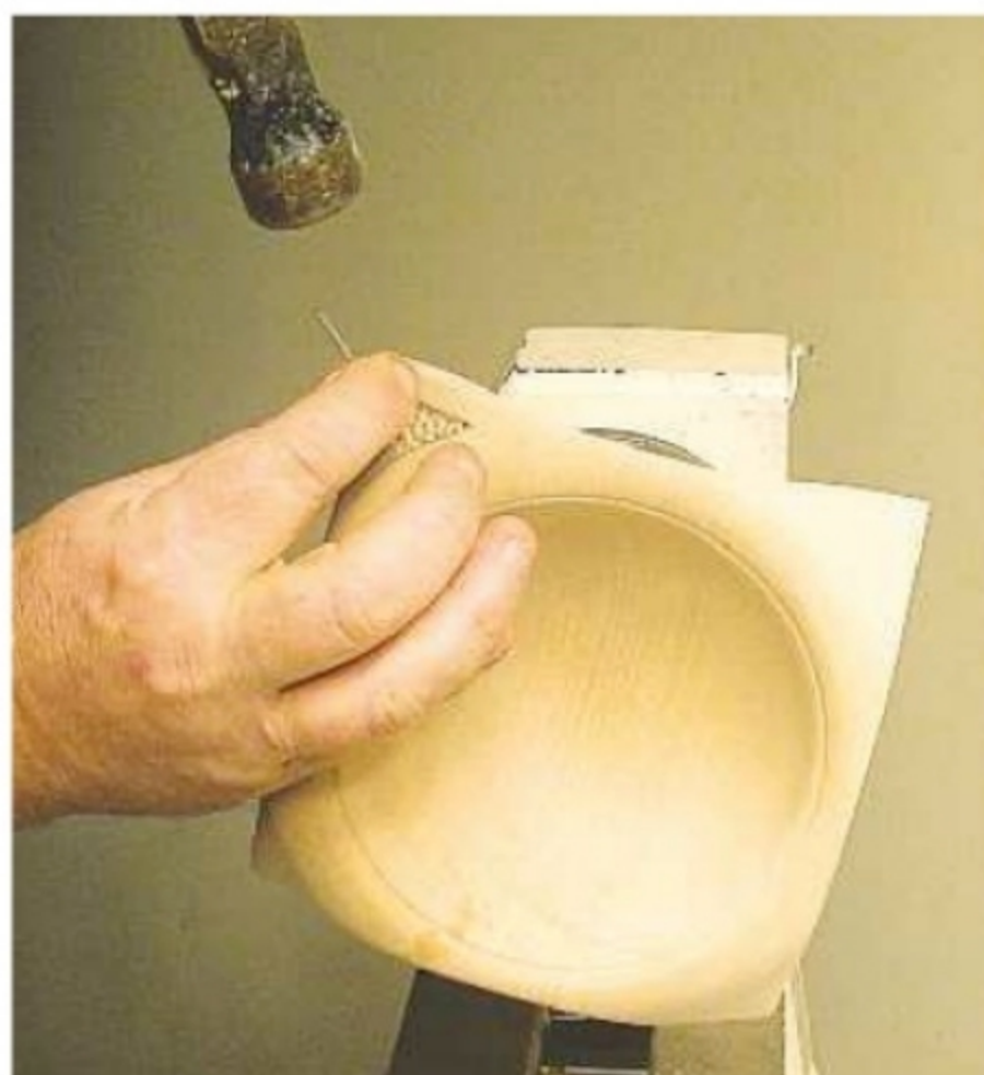
1. Tap your punch with a hammer to make each indentation. You can create a random pattern, or draw a design on the wood and follow that. Try to make all your indentations the same depth
