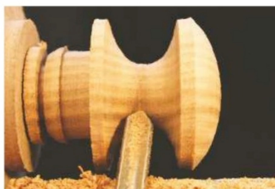
18. ...and reduce the neck of the knob to about a third of its overall diameter
