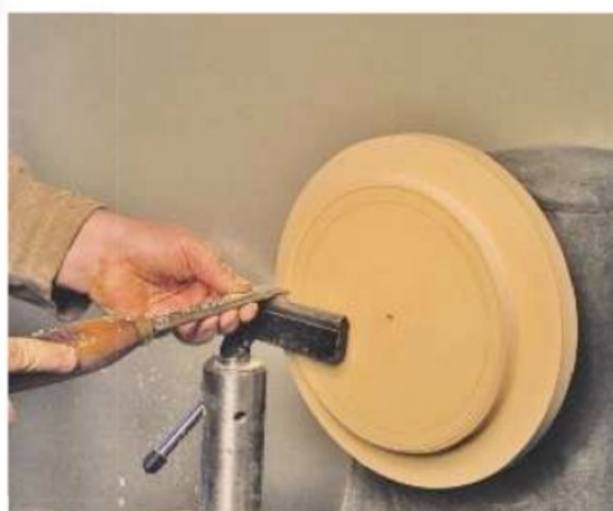
3. Screw the smaller MDF circle to the larger one and true it up with the skew
