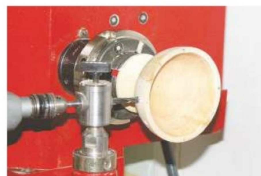
9. Set up the drilling jig and start to drill the first row of holes
