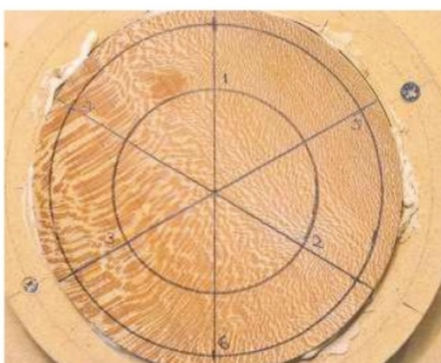
10. Mark two concentric circles on the blank and divide them into six segments
