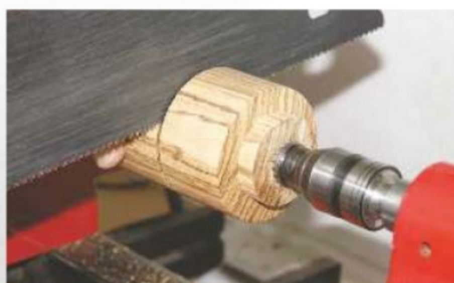
3. Complete the parting off with a saw cut
