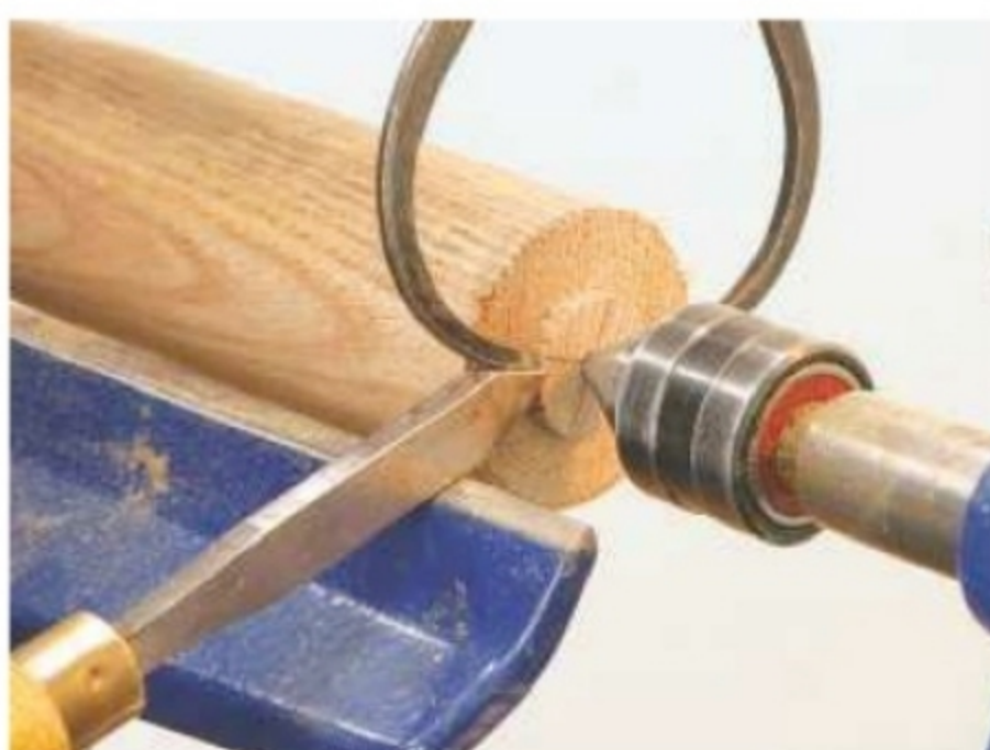
21. At the other end, reduce the leg to fit into the holes in the top
