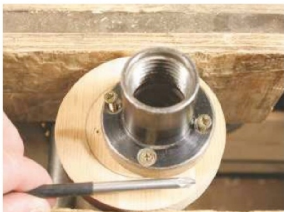
19. Unscrew the faceplate and position it off-centre on the softwood
