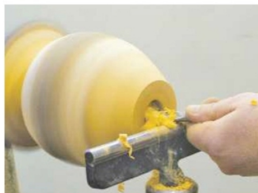
9. Hollow out the vase, starting in the hole and swinging the handle away from you
