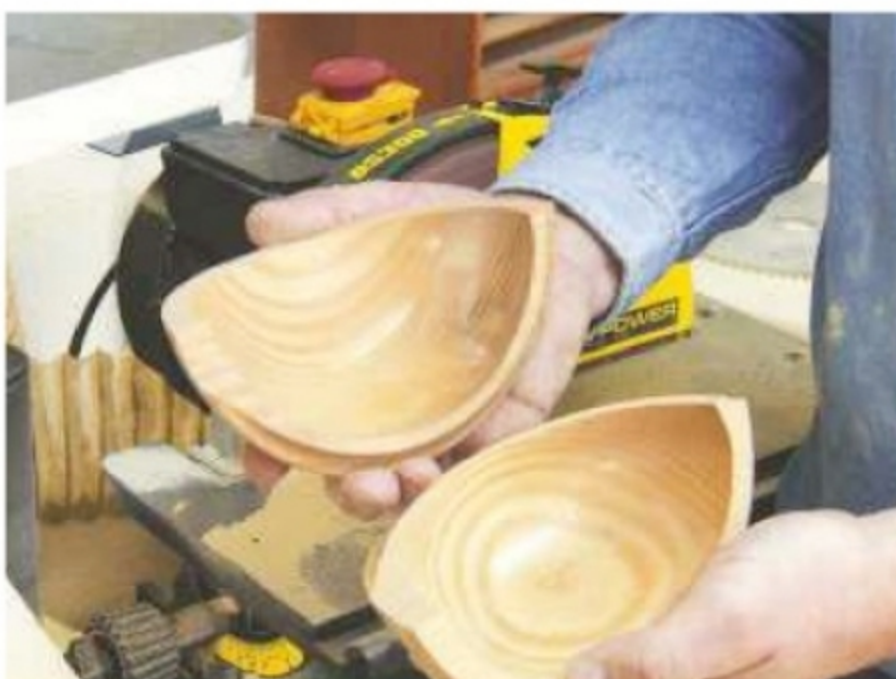
24. I decided to alter their profile by sanding away one end of each half...
