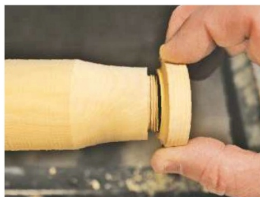
15. After every three or four passes, test the thread by winding on the lid
