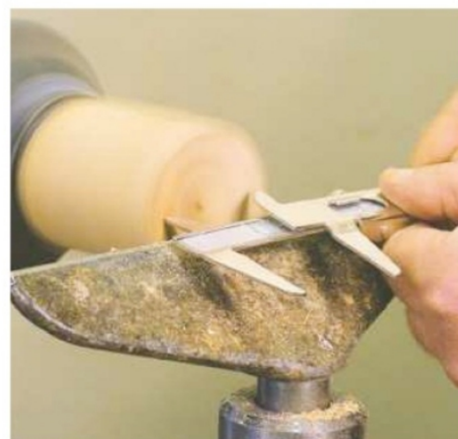
12. Mount the base in the chuck and use Vernier callipers to mark the lid's diameter on its top
