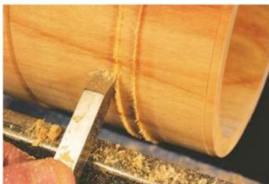
15. Cut a plinth on the base and form the straight sides with a beading tool
