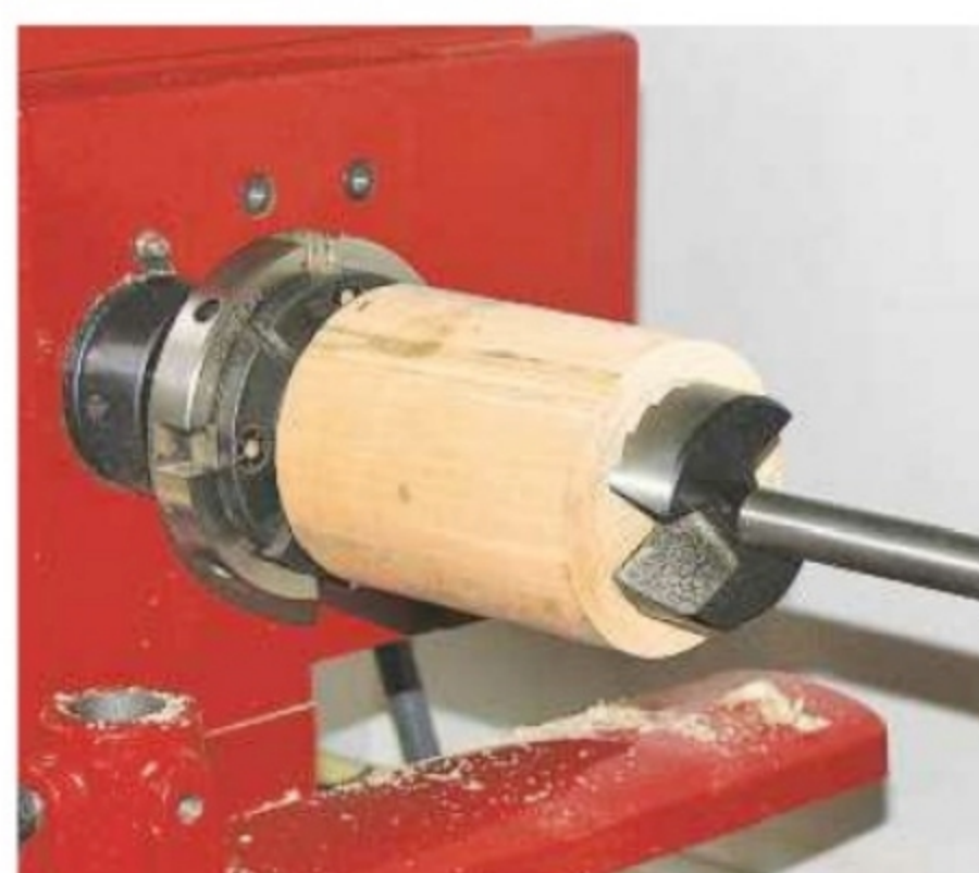
3. Fit a drill chuck in the tailstock with a 60mm sawtooth Forstner bit
