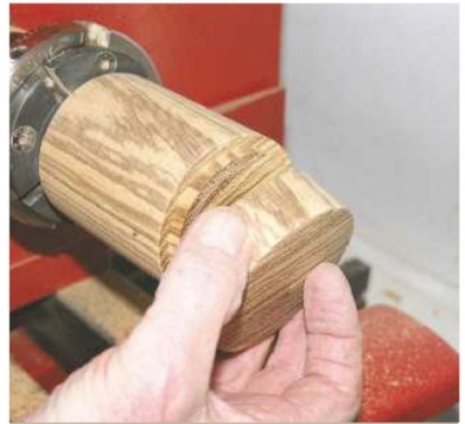
8. Reverse the lid and fit it on the chuck
