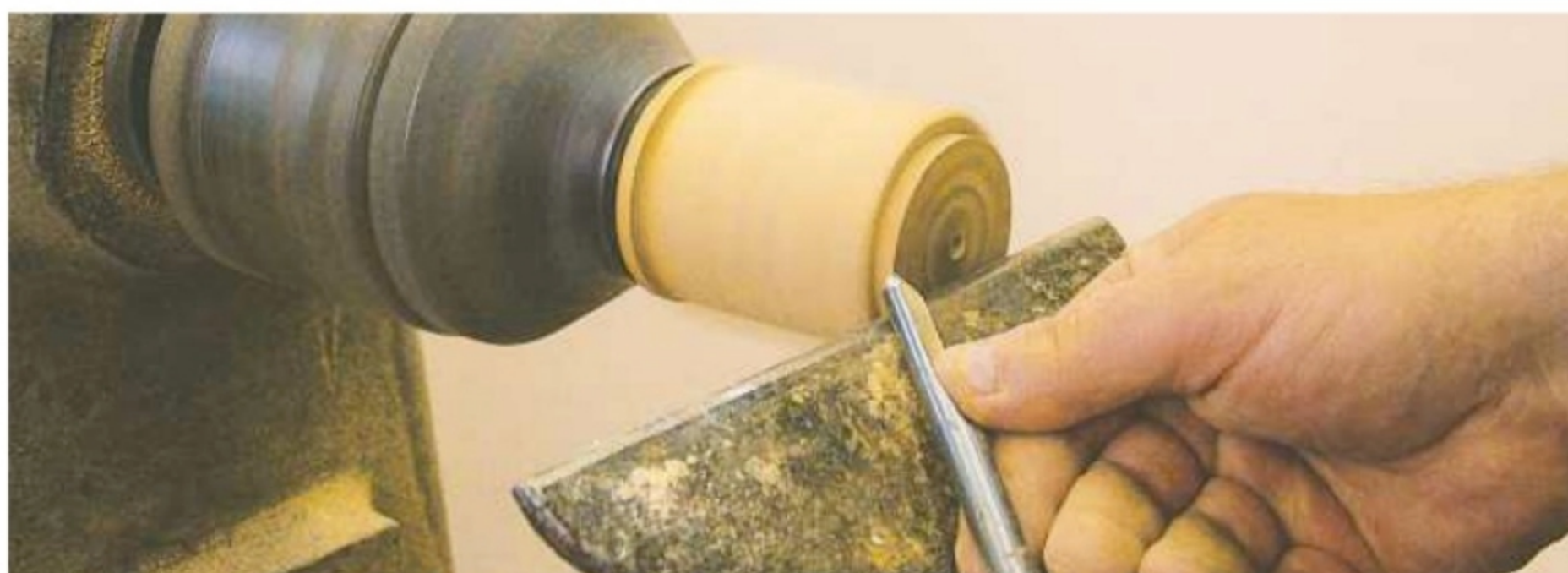
16. Reverse the base onto a jam chuck so you can remove the spigot on its underside using a spindle gouge
