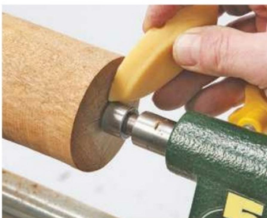
11. If the ring centre gets hot, apply a tiny amount of wax to it
