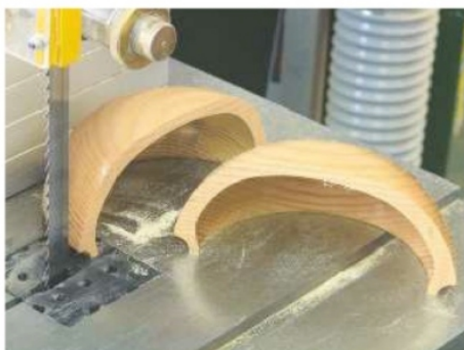
21. Set the fence to half this distance from the blade and cut the bowl in half
