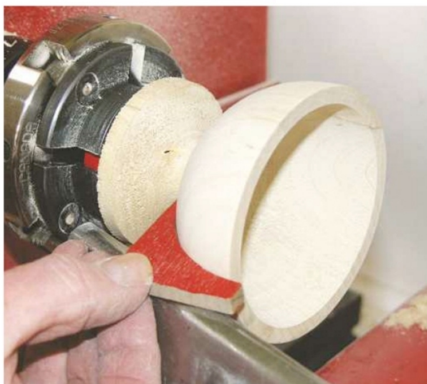
5. Use the external template (see below again) to check the progress of the outside curve
