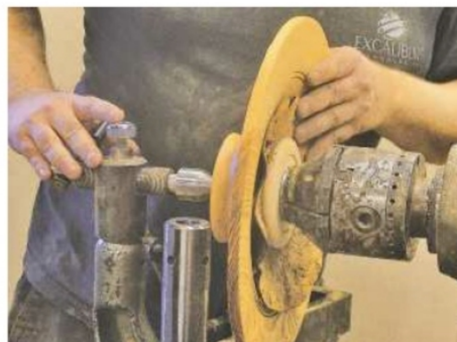
16. This shows the set-up I used to turn off the chucking spigot
