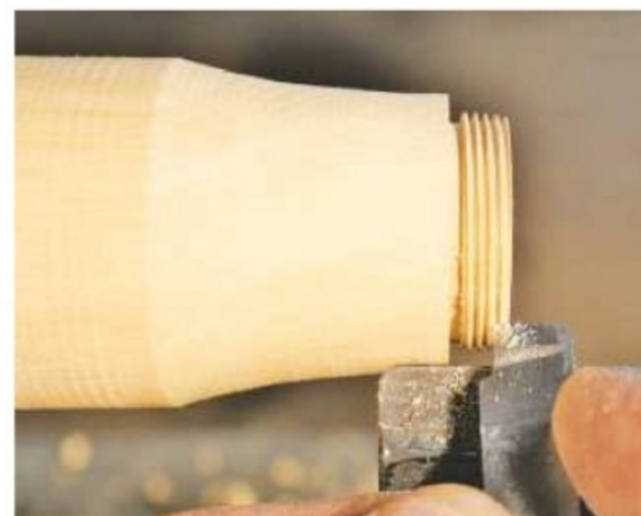
12. Start the cut with gentle sideways pressure on the side of the tool
