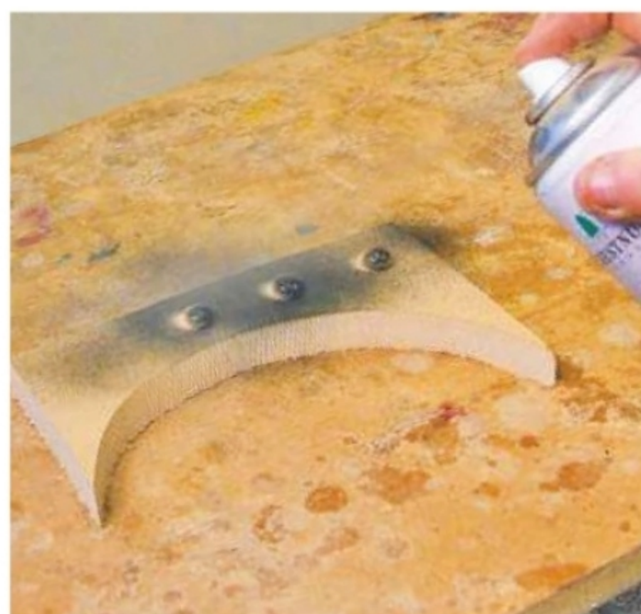
16. Mount the feet in holes drilled in some scrap wood and spray them black
