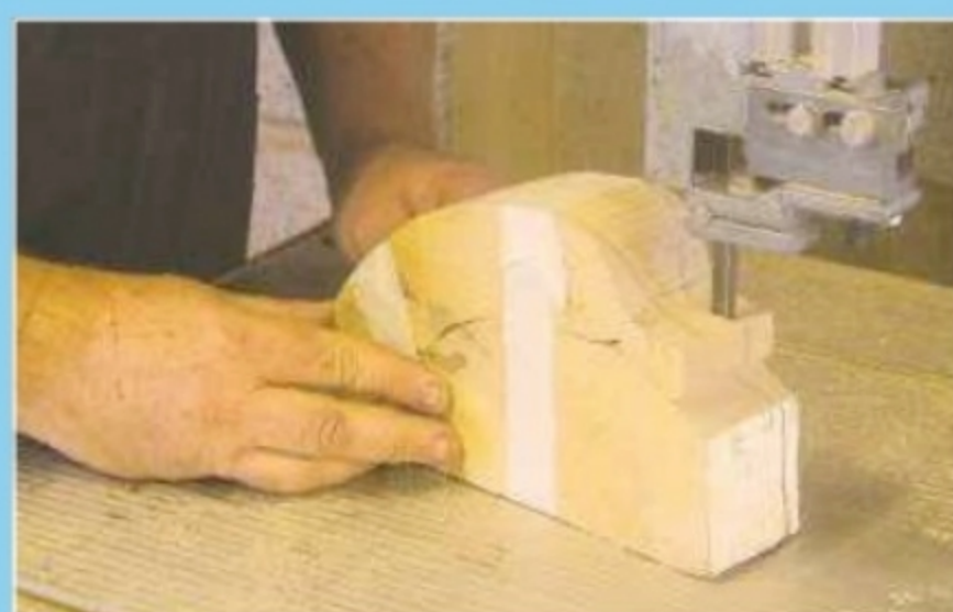
D. Make these shaping cuts using the taped-on offcut as a support
