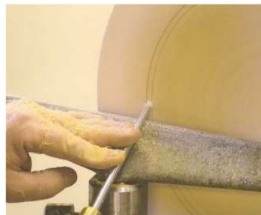
15. I cut this small decorative bead with a home-made beading tool
