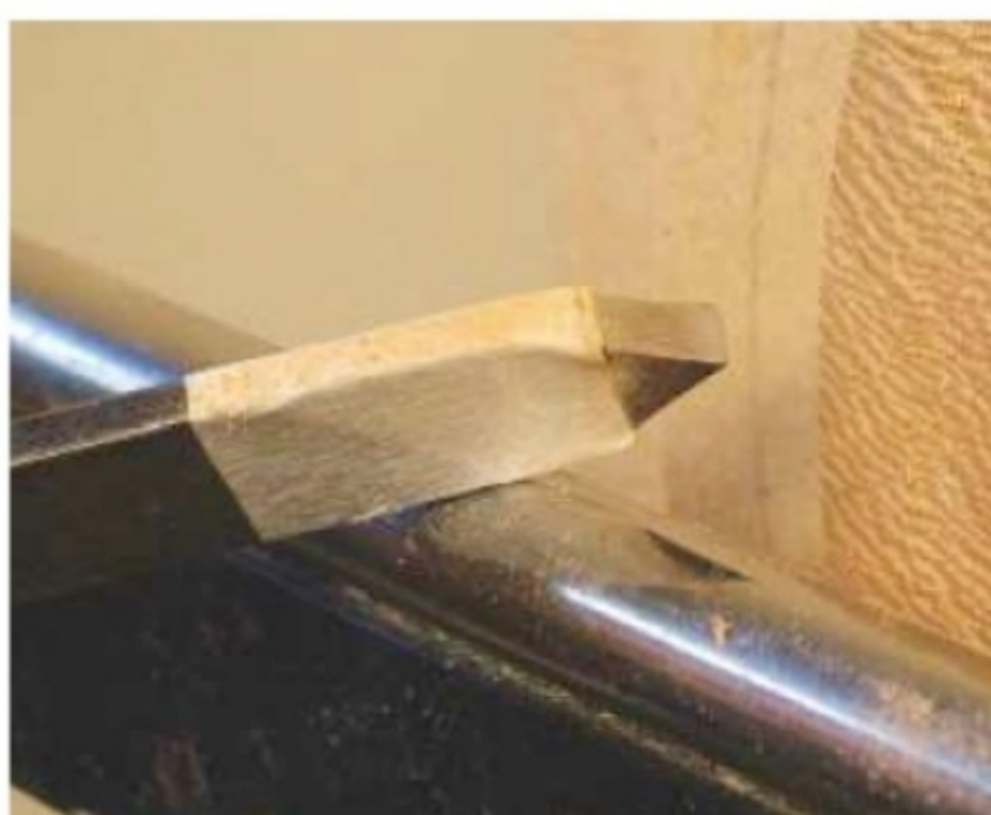
8. Use tape on the blade as a witness mark to gauge the groove depth accurately
