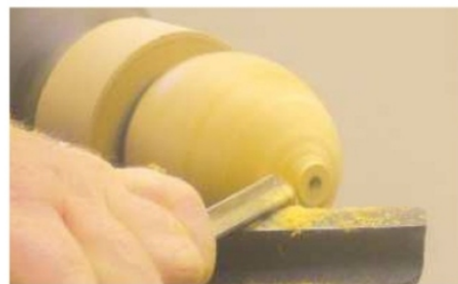
8. Use the \frac{3}{8} in spindle gouge to shape the bottom of the apple
