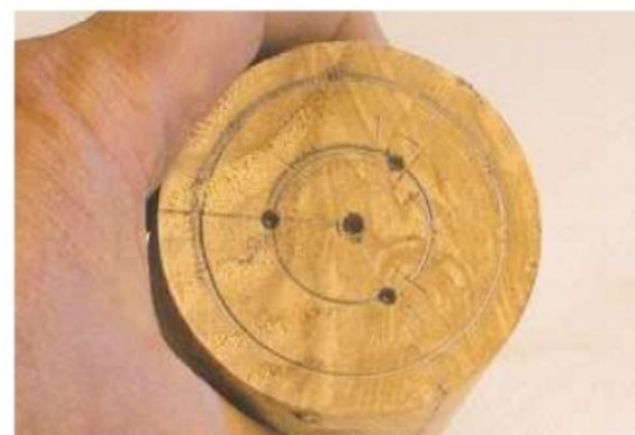
4. Centre-punch holes where the three radial lines cross the inner circle, then number them
