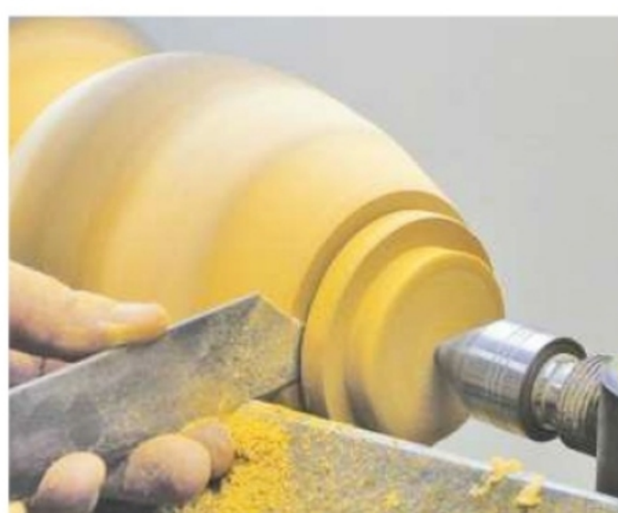
5. Part off the plug section next to the spigot using a narrow parting tool
