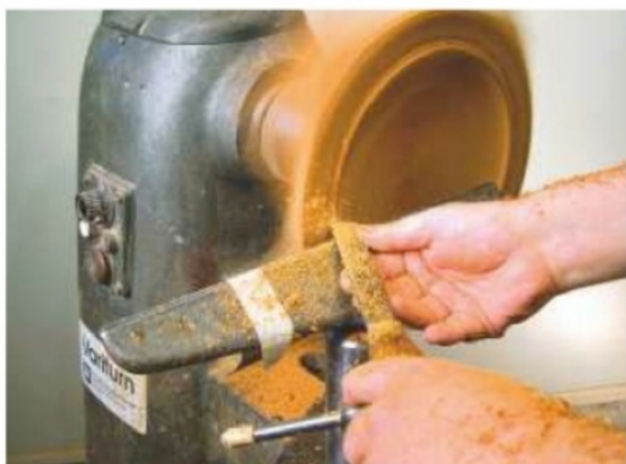
15. Flat down between coats, apply pastewax and buff up to a high sheen
