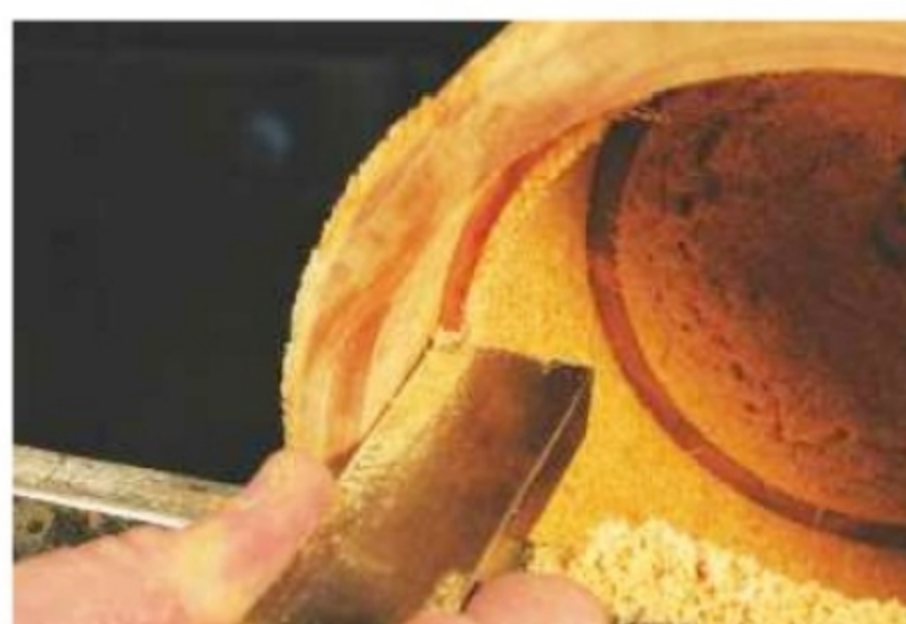
12. Remove the rest of the waste by widening the hole with a square scraper
