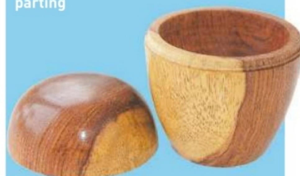
The box is polished before the final parting
