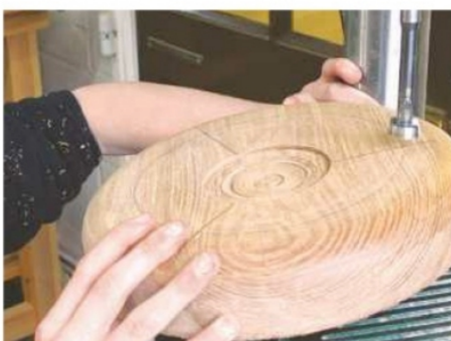
12. Align each marked line in turn by eye with the shank of the drill bit
