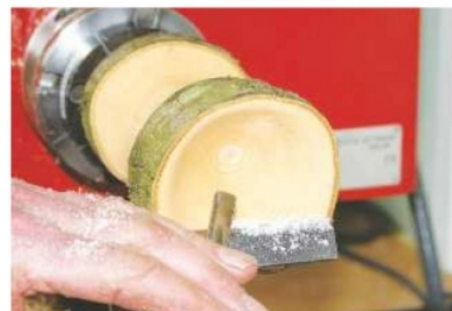
8. Withdraw the tailstock and hollow out the goblet carefully using a 9mm bowl gouge
