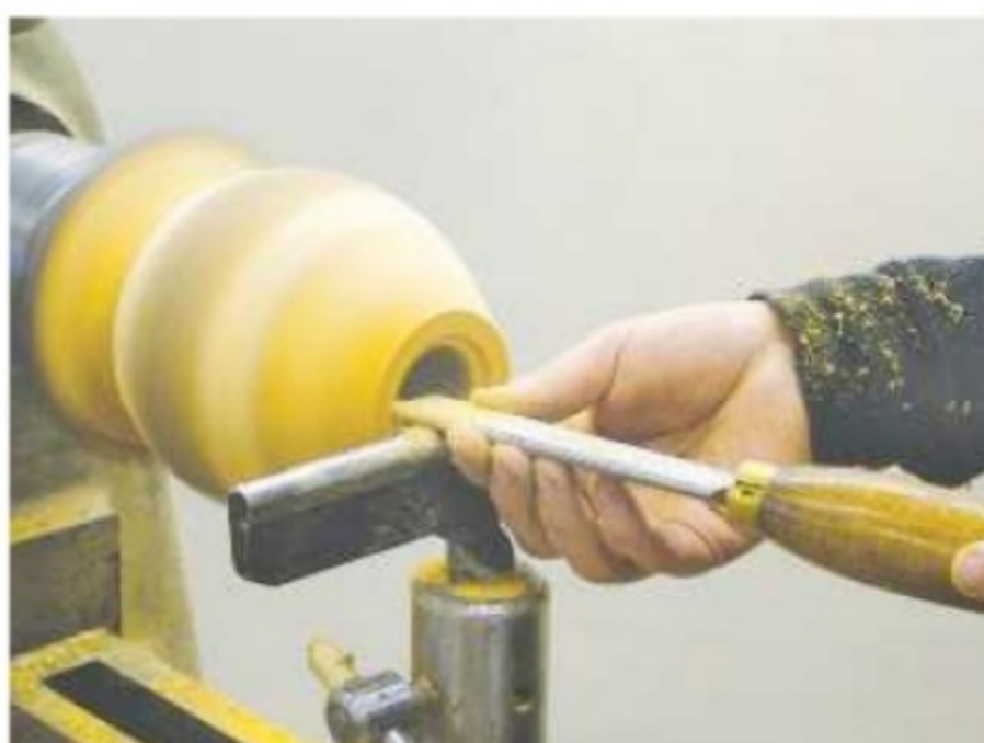
12. Use a skew chisel to cut a parallel-sided step in the base for the plug
