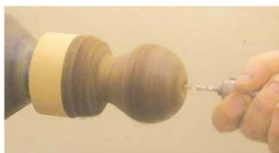
14. Bore a hole in the bottom of the pear with a hand-held drill bit
