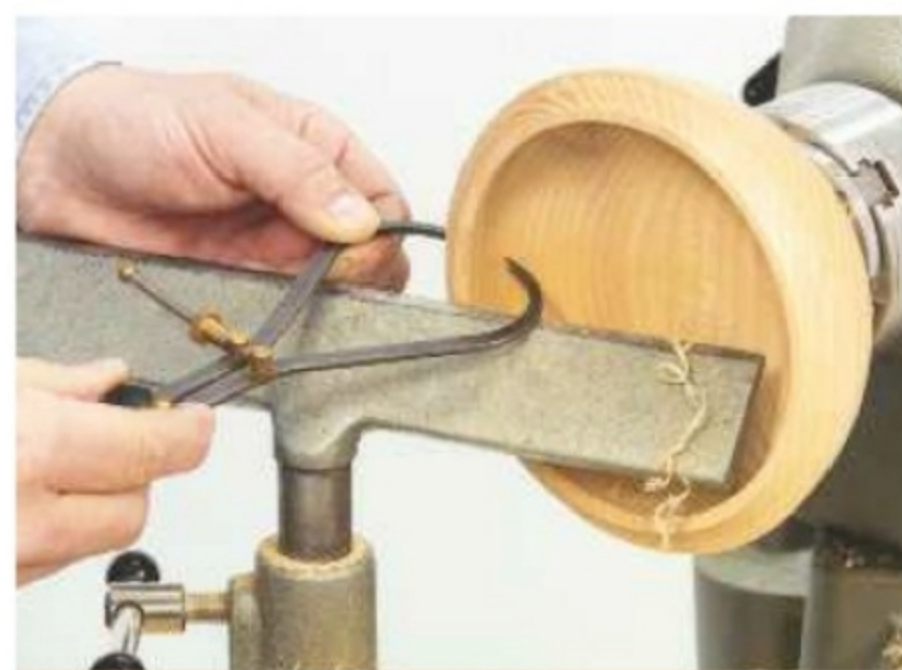
11. The key to success is in creating an even wall thickness; check this with callipers
