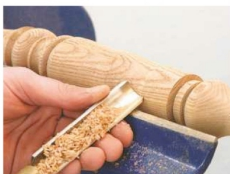
23. Form the details on the leg using a variety of gouges and a parting tool
