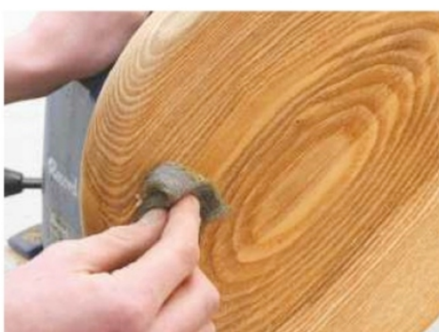
18. Polish the top with pastewax, applied over cellulose sanding sealer
