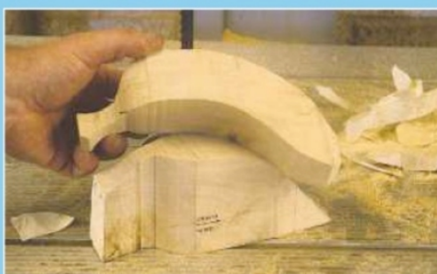
E. You now have a three-dimensional banana shape with four sides
