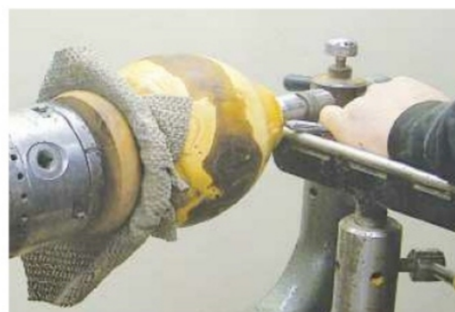
19. Reverse-chuck the vase onto a padded dolly and bring the tailstock up to apply pressure
