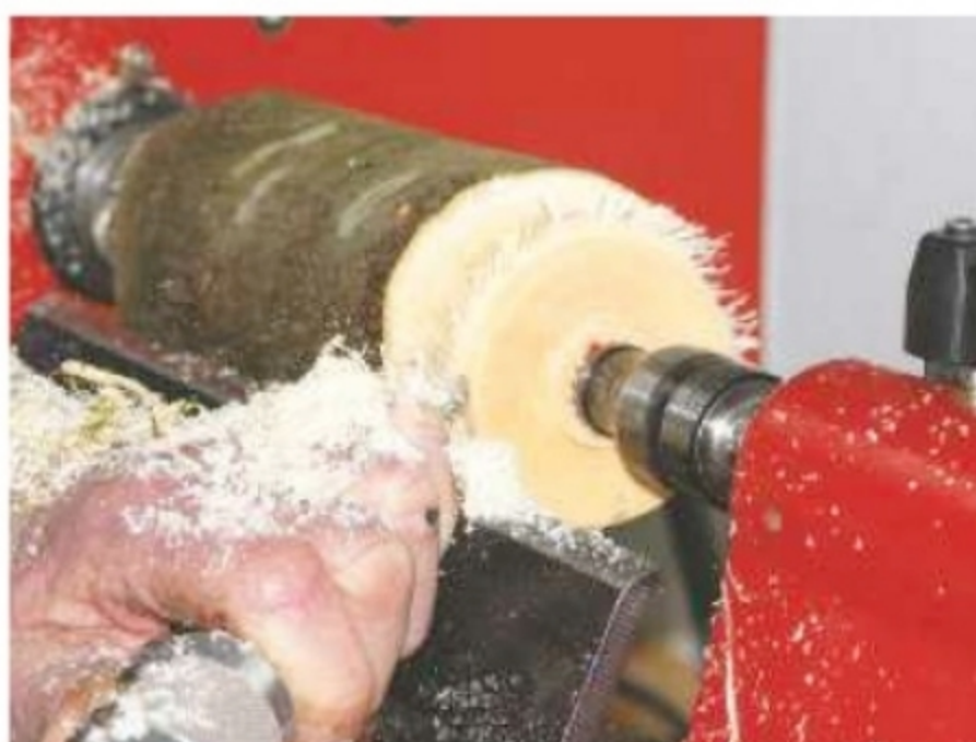
4. Start turning a spigot to suit your chuck jaws. Note how the wet shavings peel off the wood
