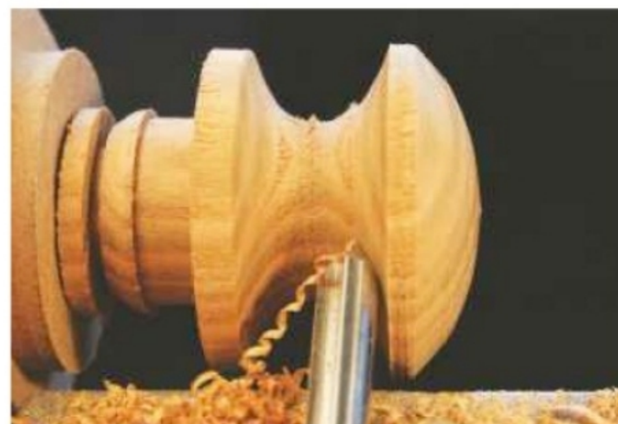
17. Use a small spindle gouge to form the profile on the body of the knob...
