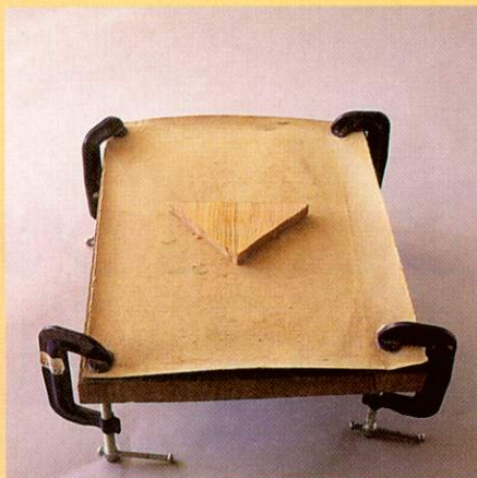
Sanding table is useful to remove burrs from sawn sections.
