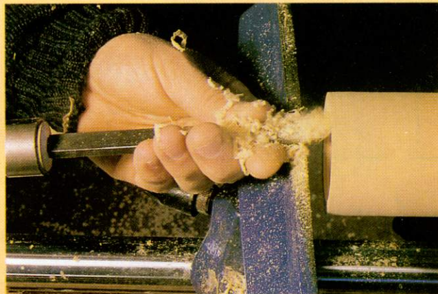
Hollowing out the end of the scoop with a round nosed scraper.
