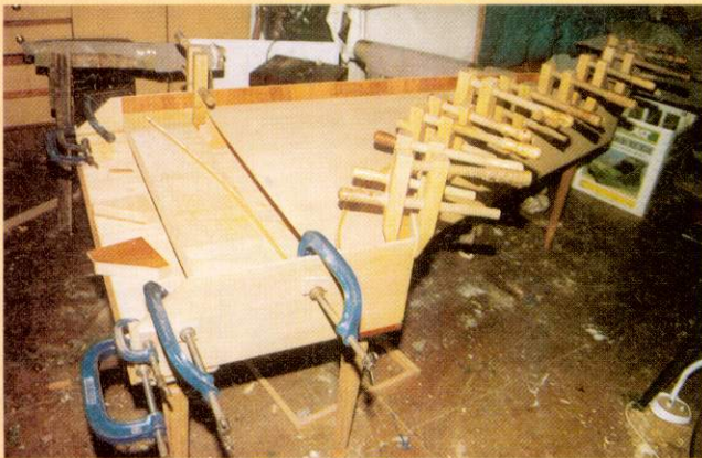
The carcass of a harpsichord is glued and held together with old-fashioned wooden cramps. Using lots of cramps enables Chris to apply more pressure as it is spread out across the carcass.
