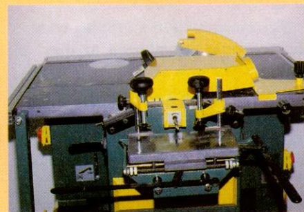
6. The mortising attachment in place.
