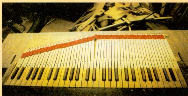
The keyboard is made using one large panel of lime which will be cut and fronted with boxwood after drilling.
