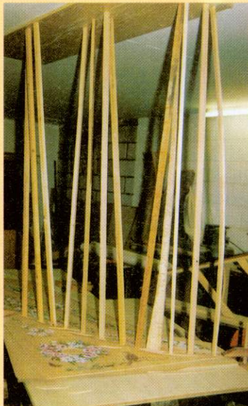
Wooden rods or 'go-bars' are sprung at a high pressure between the ceiling of Chris' workshop and the beech bridge whilst it is glued to the soundboard.
