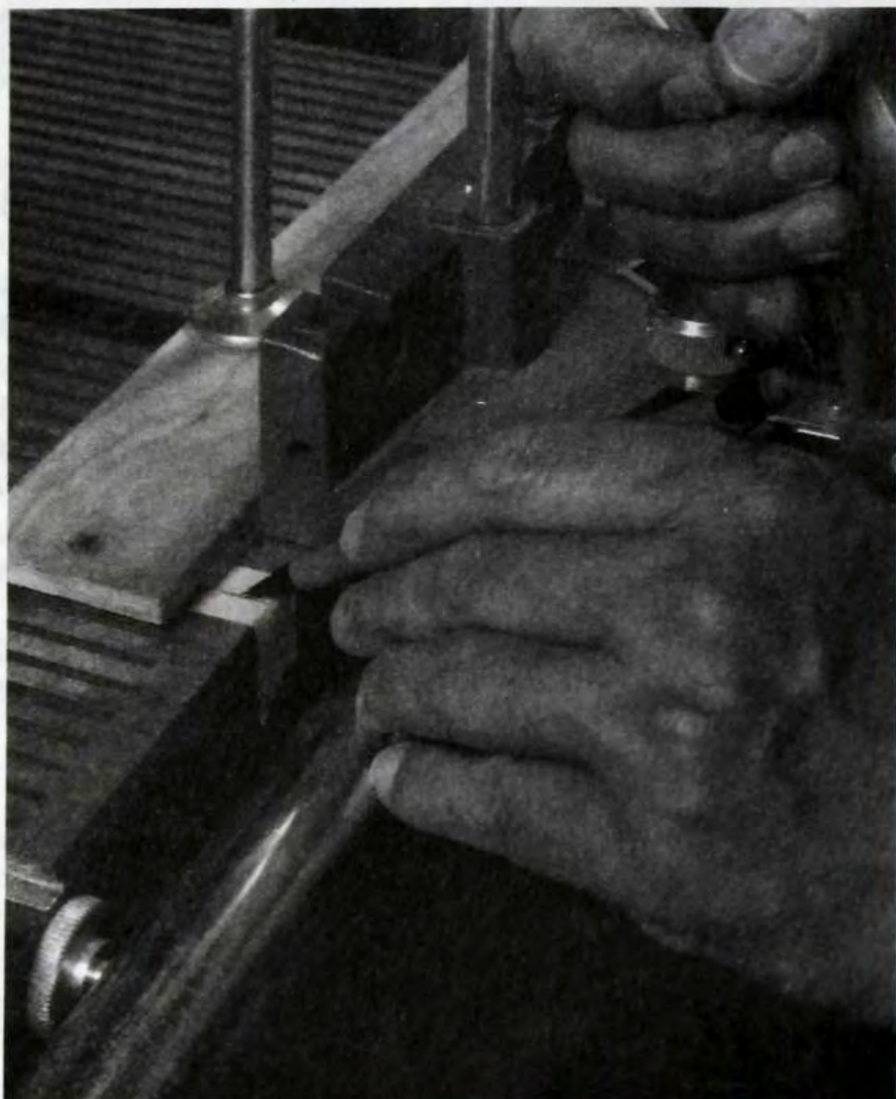
Figure 3. Make repetitive cuts in the half-lap areas. Use a pencil mark, placed on tape, to help you position the stock for dadoing.
