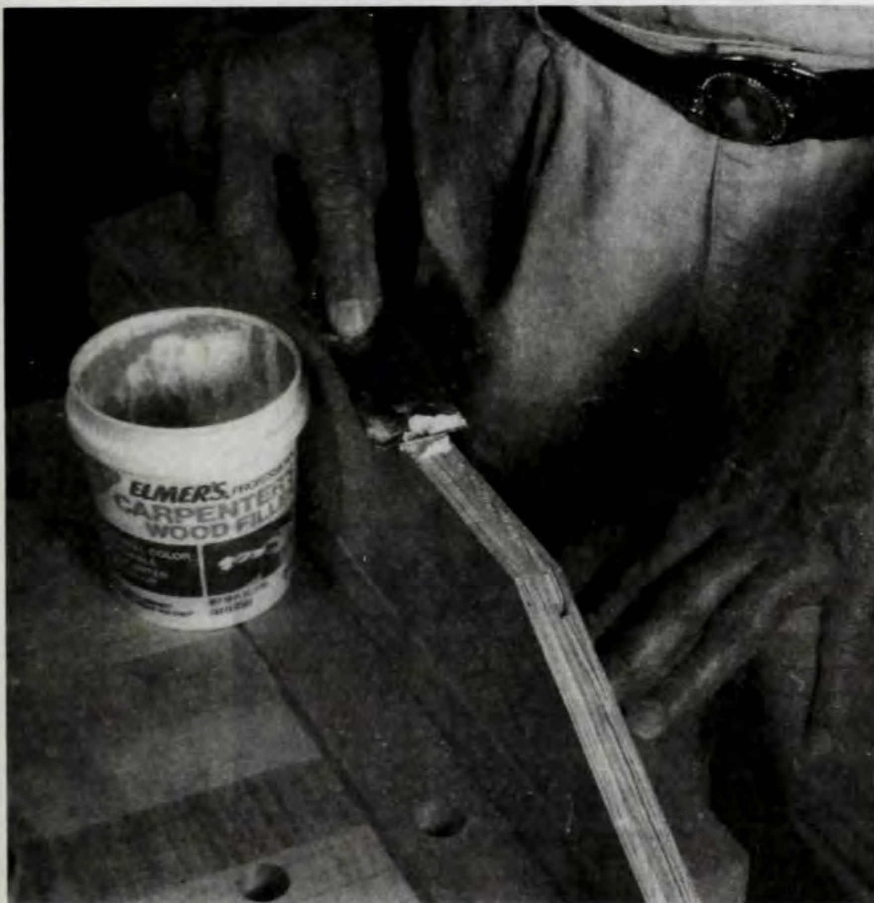
Figure 2. Fill in all blemishes with a nontoxic wood filler. Then sand flush with a belt sander.
