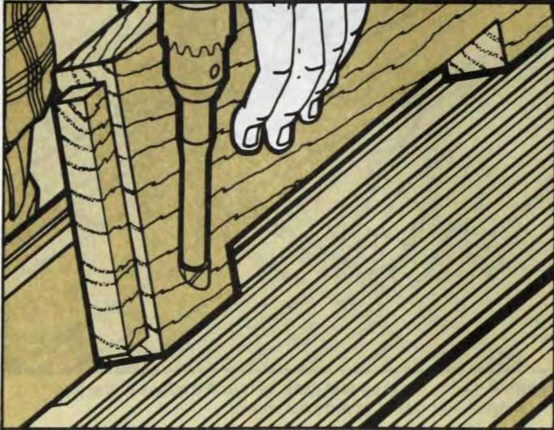
Figure 6. Drill screw pockets in the sides (B). Drill at a 10 degree angle, with a 1/2 in. Forstner bit, to within 3/8 in. of the bottom. Use a 1/4 in. brad point bit to make pilot holes for the No. 12 round head screws. For clarity, guards not shown.
