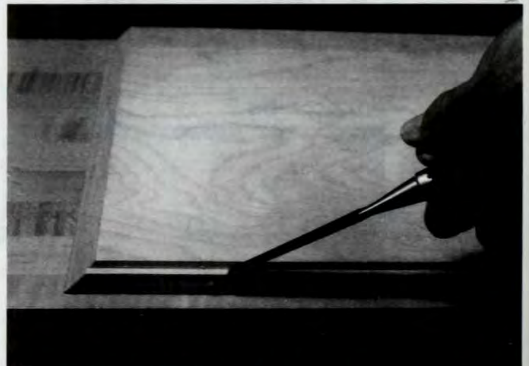
Figure 4. Clean out the rabbeted area (see previous photo) using a sharp wood chisel. Always clamp the workpiece to prevent one hand getting in harm's way in case of a slip.
