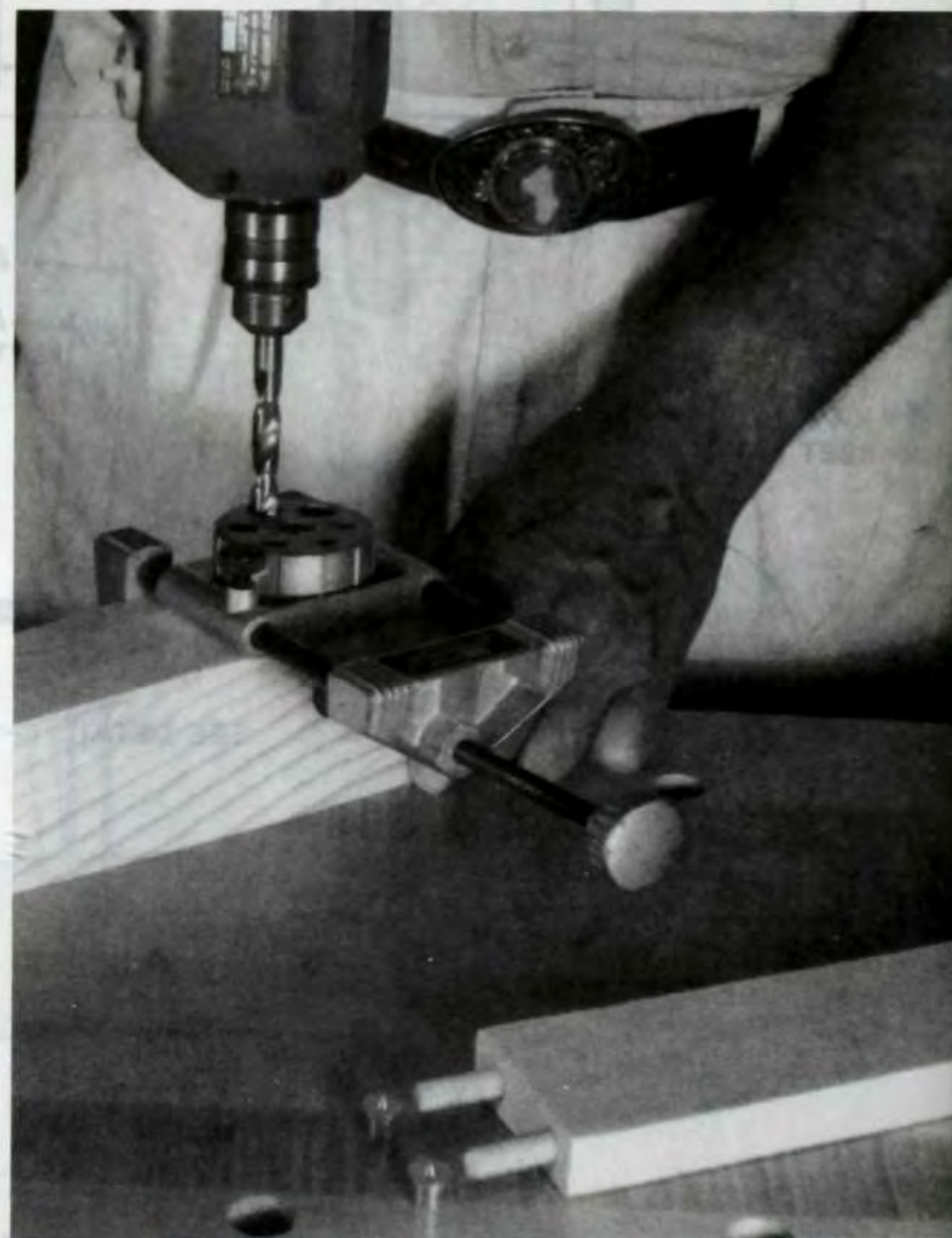
Figure 4. Drill dowel holes into the legs (F) and insert dowel centers to help mark the adjacent desk rails (E, G) for drilling.
