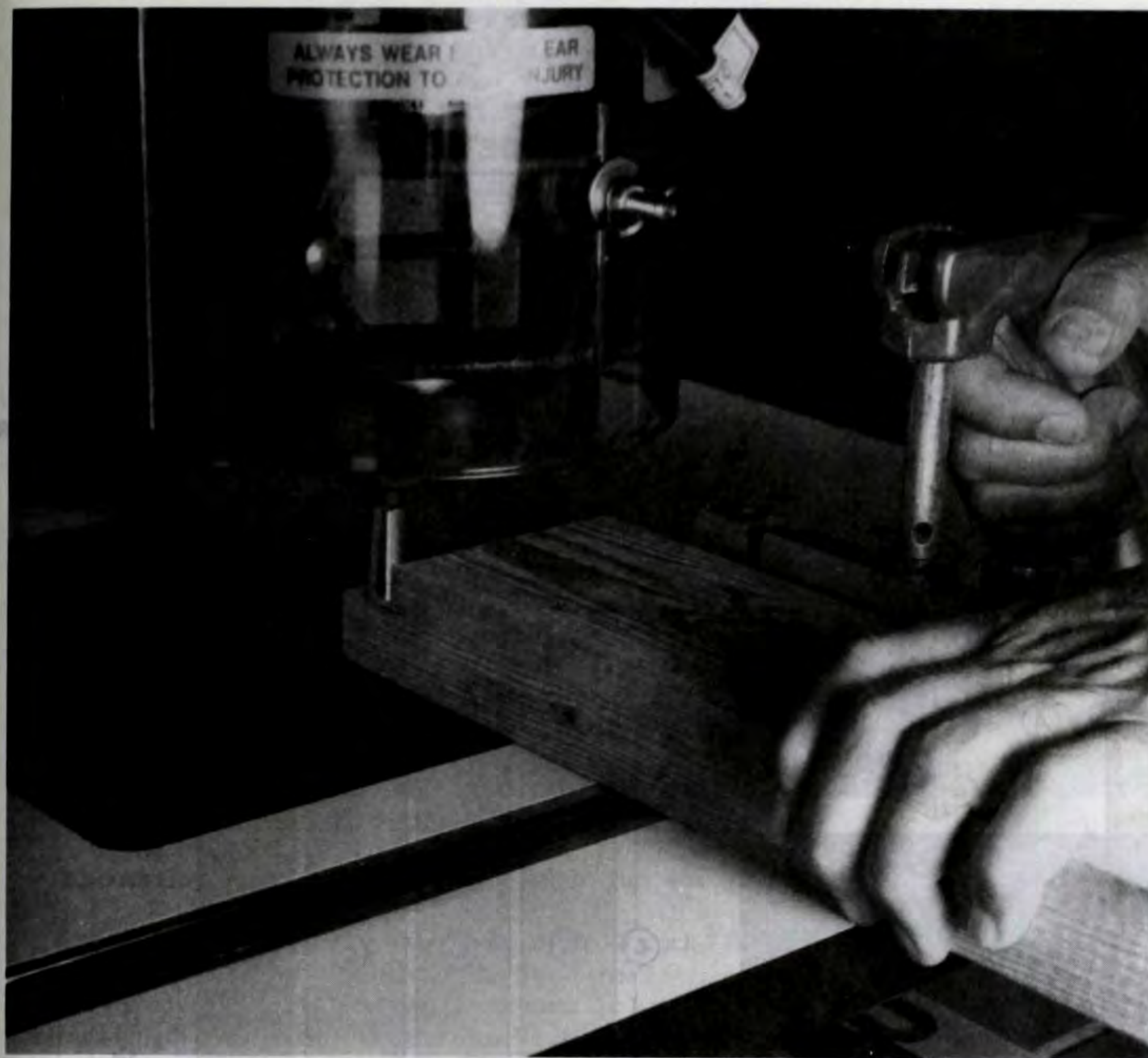
Figure 1. Cut the rabbets on your router table. Do not make the cut in one pass; make progressively deeper cuts on each pass. Use a miter gauge to hold the material for cutting.
