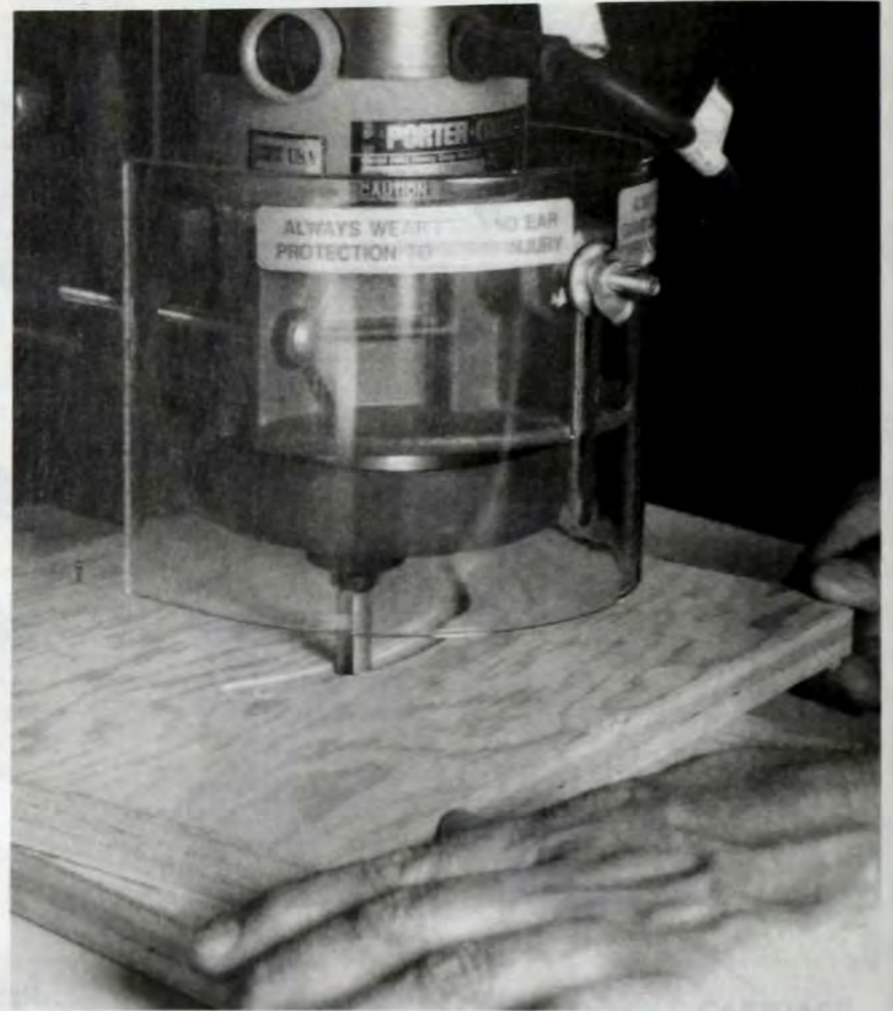
Figure 4. An overhead router is ideal for making the slot into the pivot support. Drive nail at the pivot point and lower the overhead router into the wood at the proper starting point. Then rotate the workpiece. Make only 1/8 in. deep passes until you achieve final depth. Then drill out the pivot point with a drill press.
