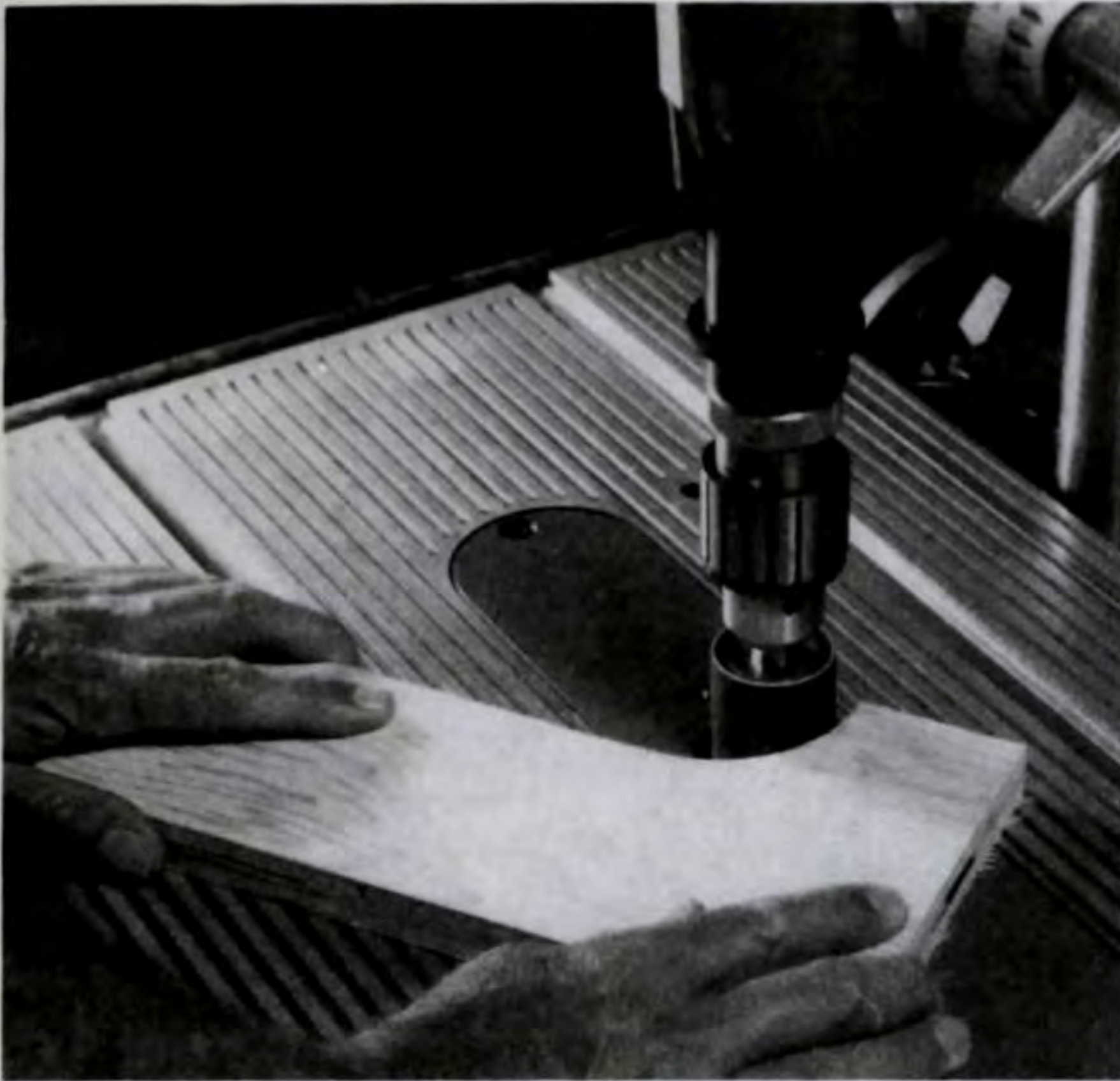
Figure 2. Sand the contours with a drum sander installed in a drill or drill press. The drum should rotate into the workpiece.
