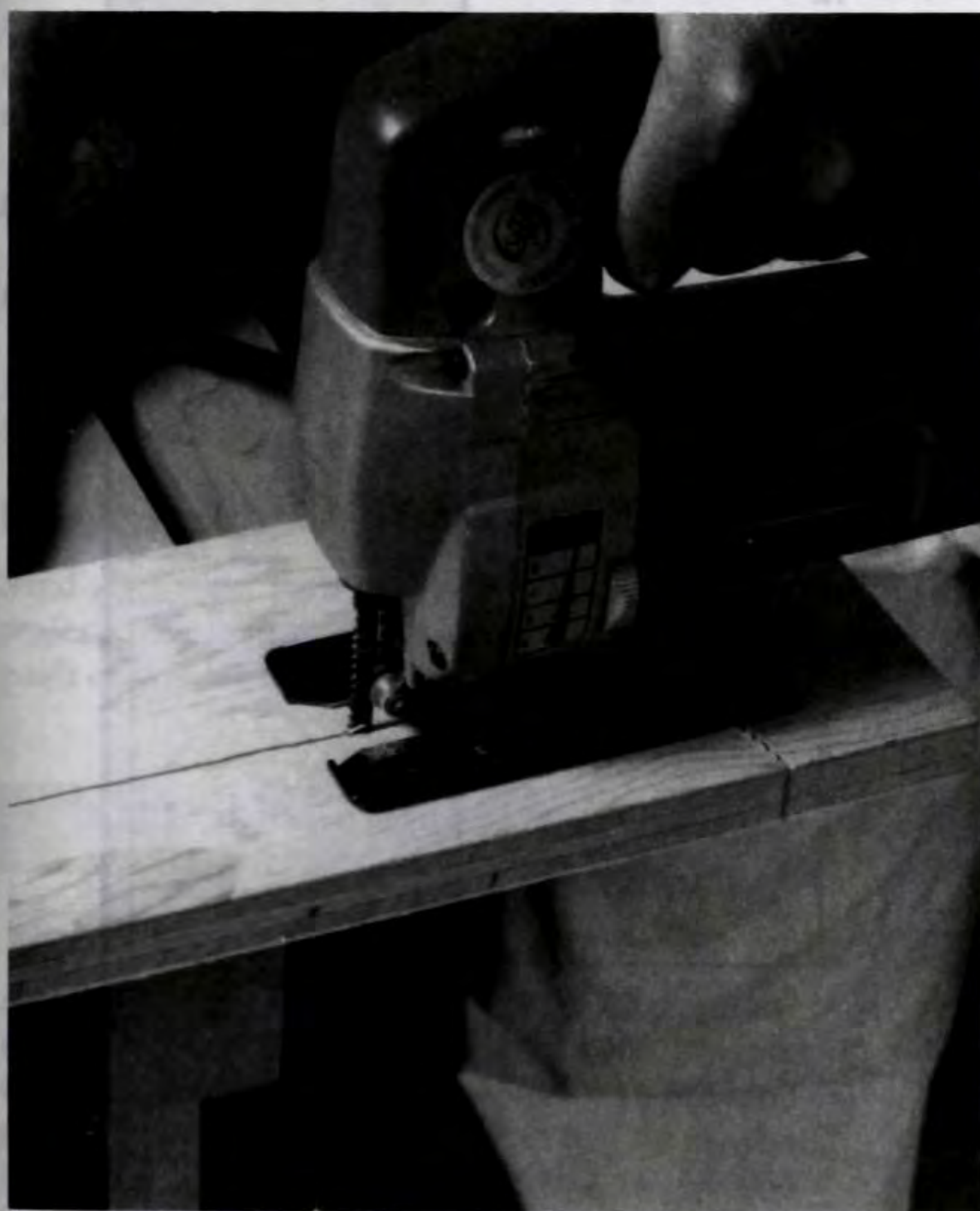
Figure 1. Cut out the contours in the rails (E) and sides (A) with a saber saw. Cut with the good side down and use a plywood cutting blade.
