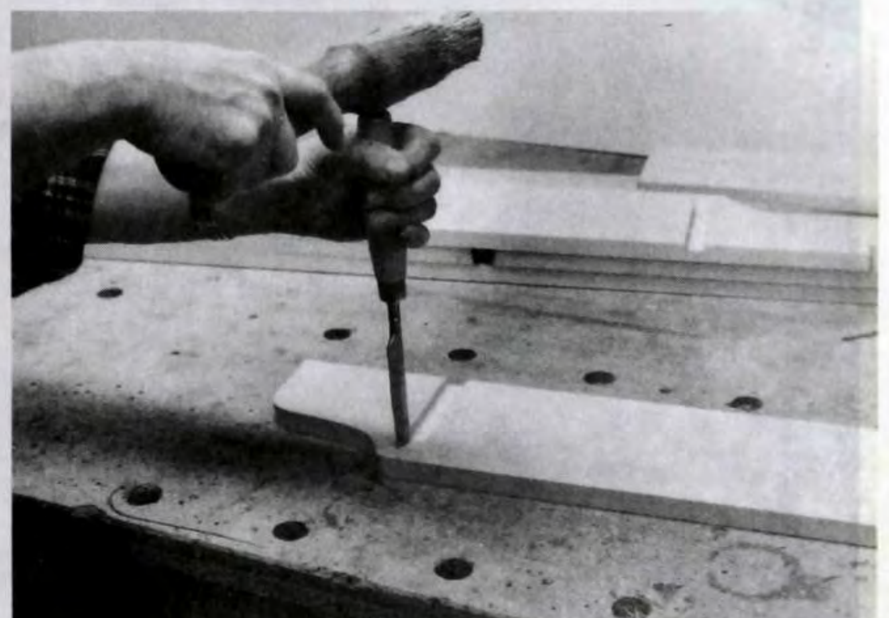
Figure 4. Trim the stopped dado with a sharp wood chisel. Strike the chisel lightly with a wood mallet.
