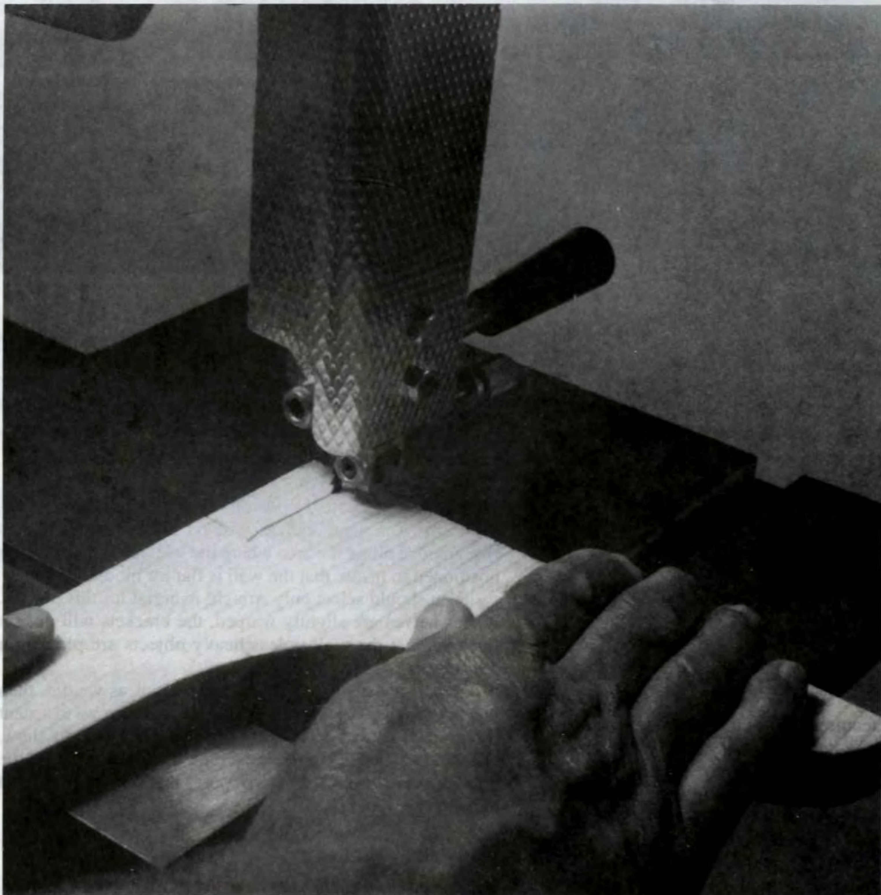
Figure 2. Cut out the bracket (C) with a saber saw equipped with a fine-tooth blade. Work slowly and hug the cutting line.
