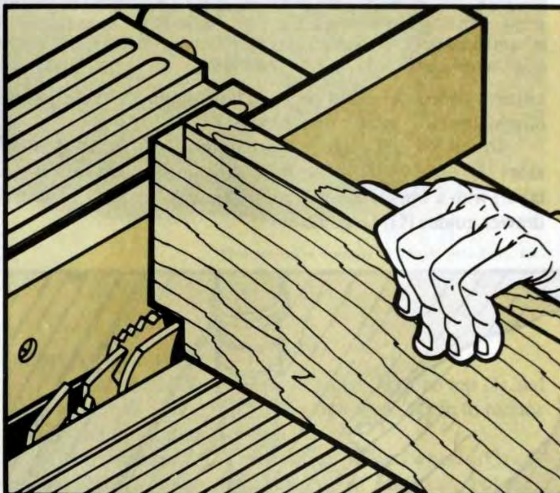
Figure 4. Use a dado installed in your table saw to cut the tenons (note the use of extension fence).
