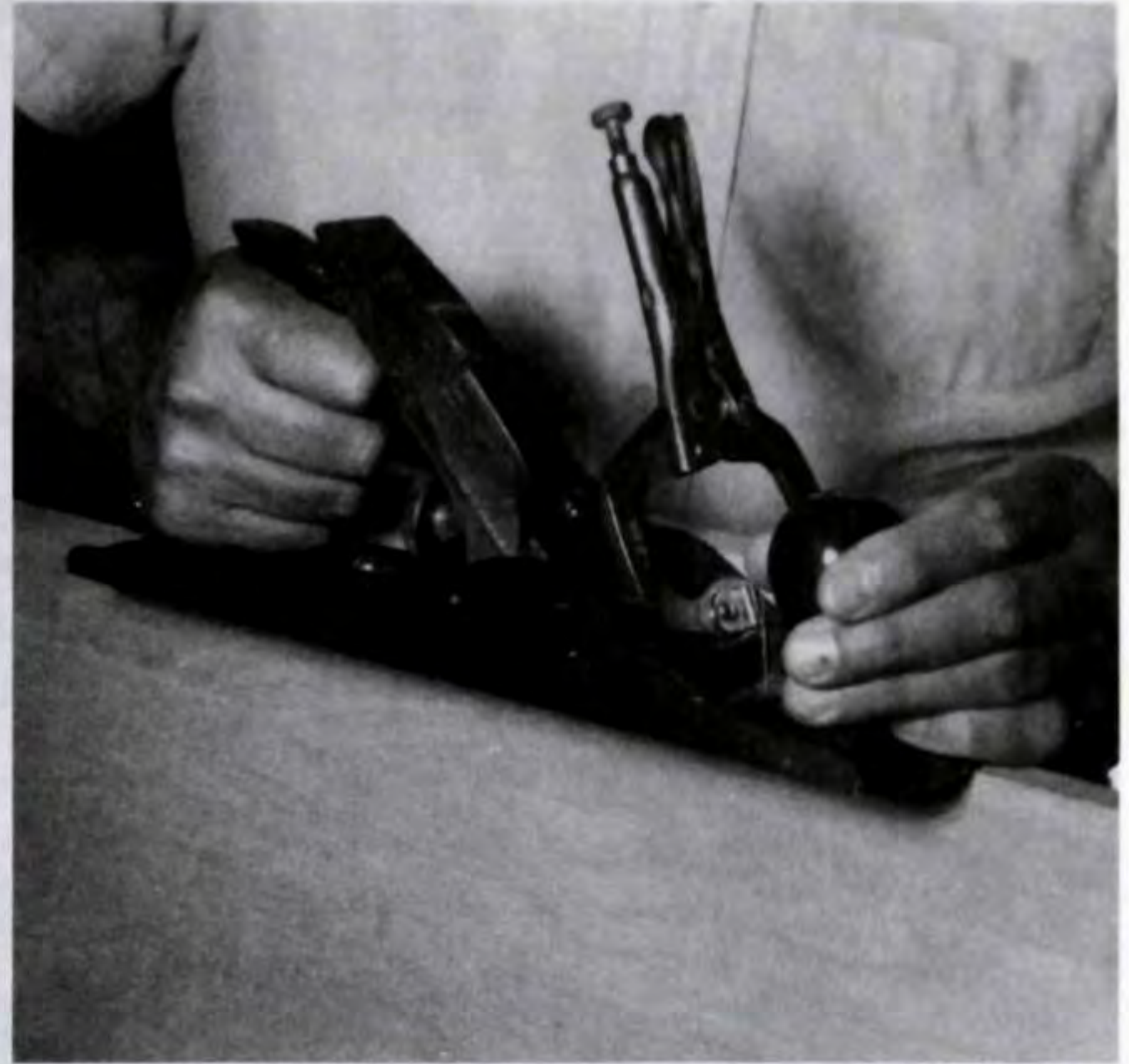
Figure 3. If you do not have a jointer or power hand plane, use a bench plane. Clamp a piece of scrap wood for an edge-guide, as shown. Take long, shallow passes.
