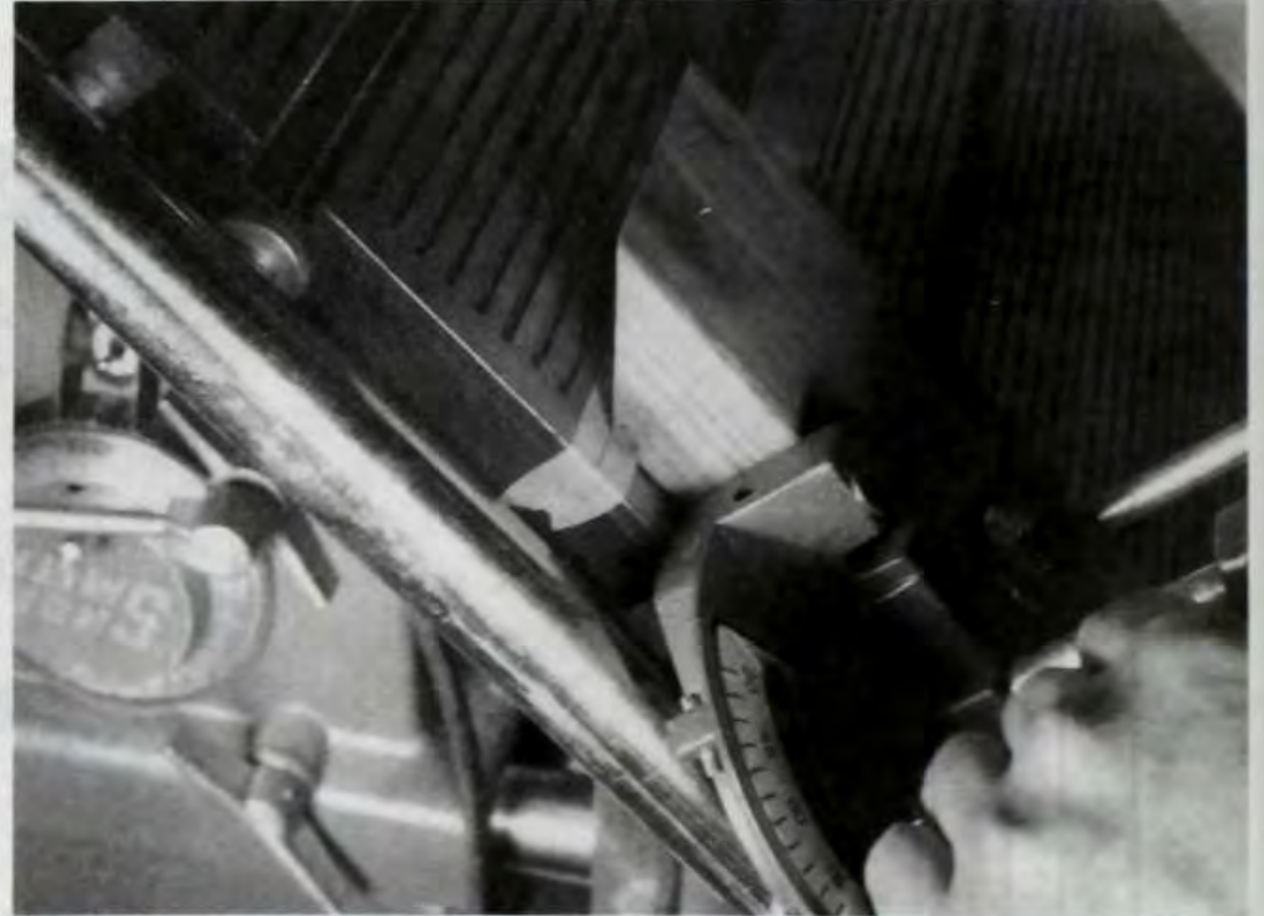
Figure 2. Mark the location where the cut is to begin by placing a piece of tape on the table saw. Make sure the tape is well away from the blade so you can position the next piece for cutting.
