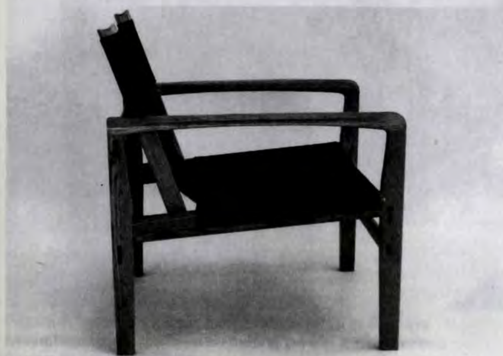
Figure 5. Assemble the chair with carpenter's glue and plenty of clamps. After the assembly is tightened, drive in wedges into the slotted tenons.
