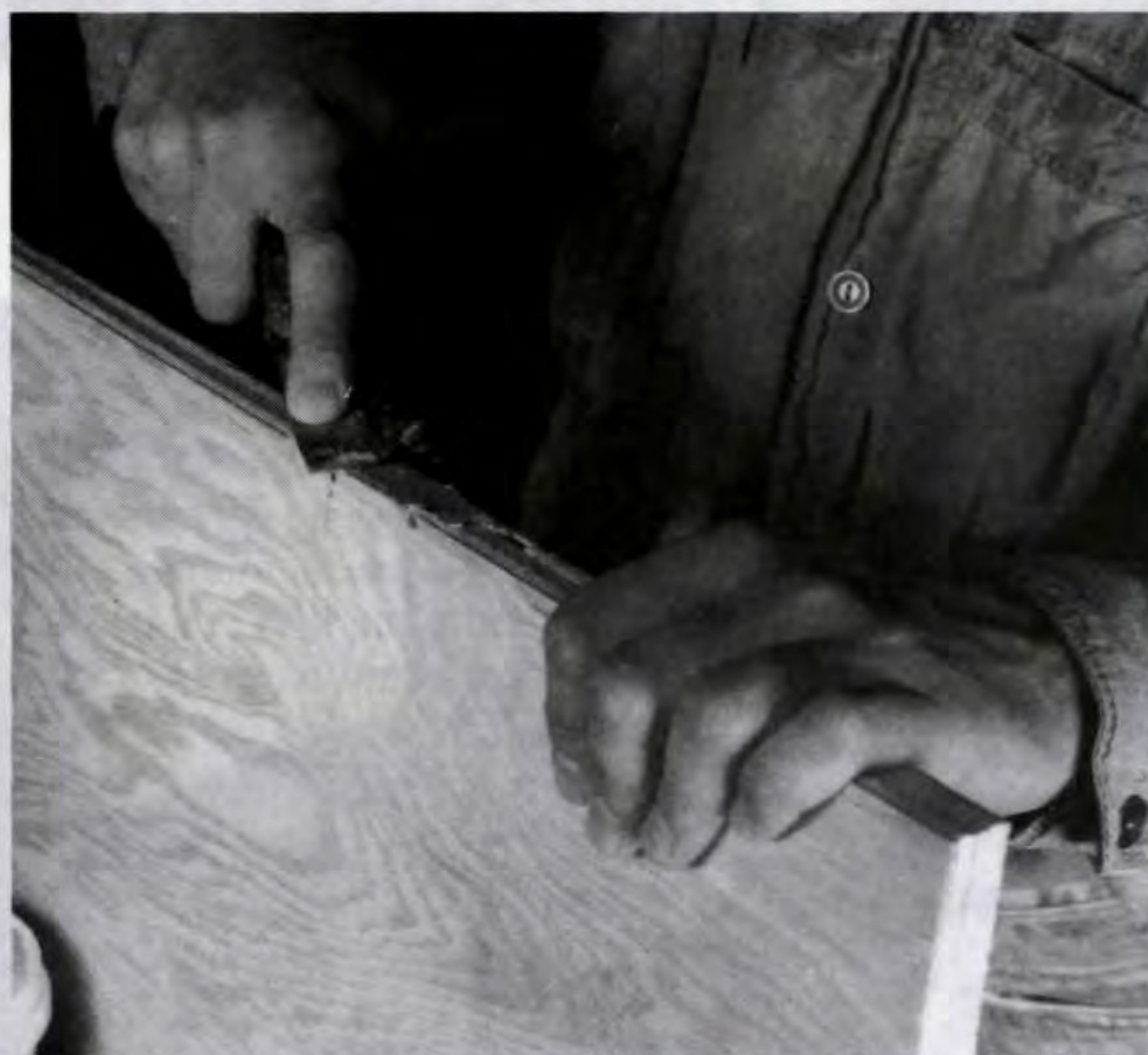
Figure 4. Fill in any blemishes with a nontoxic wood filler. Make sure the filler goes on smoothly.
