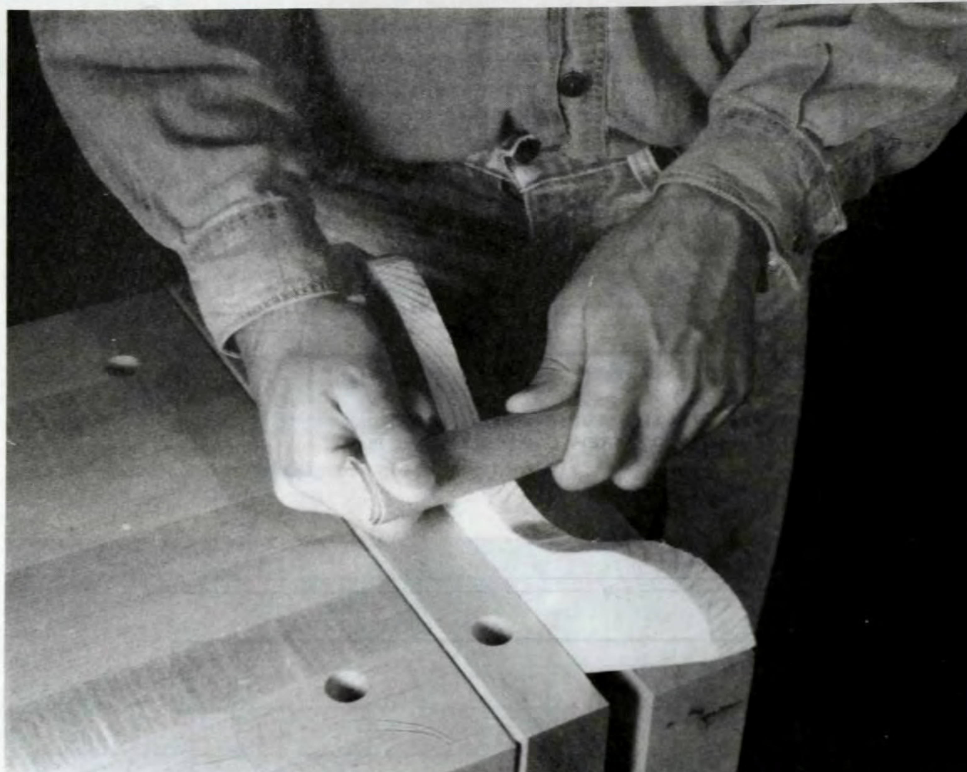
Figure 3. Finish sand the edge of the bracket (C) with a half-round file or dowel wrapped with sandpaper (as shown).
