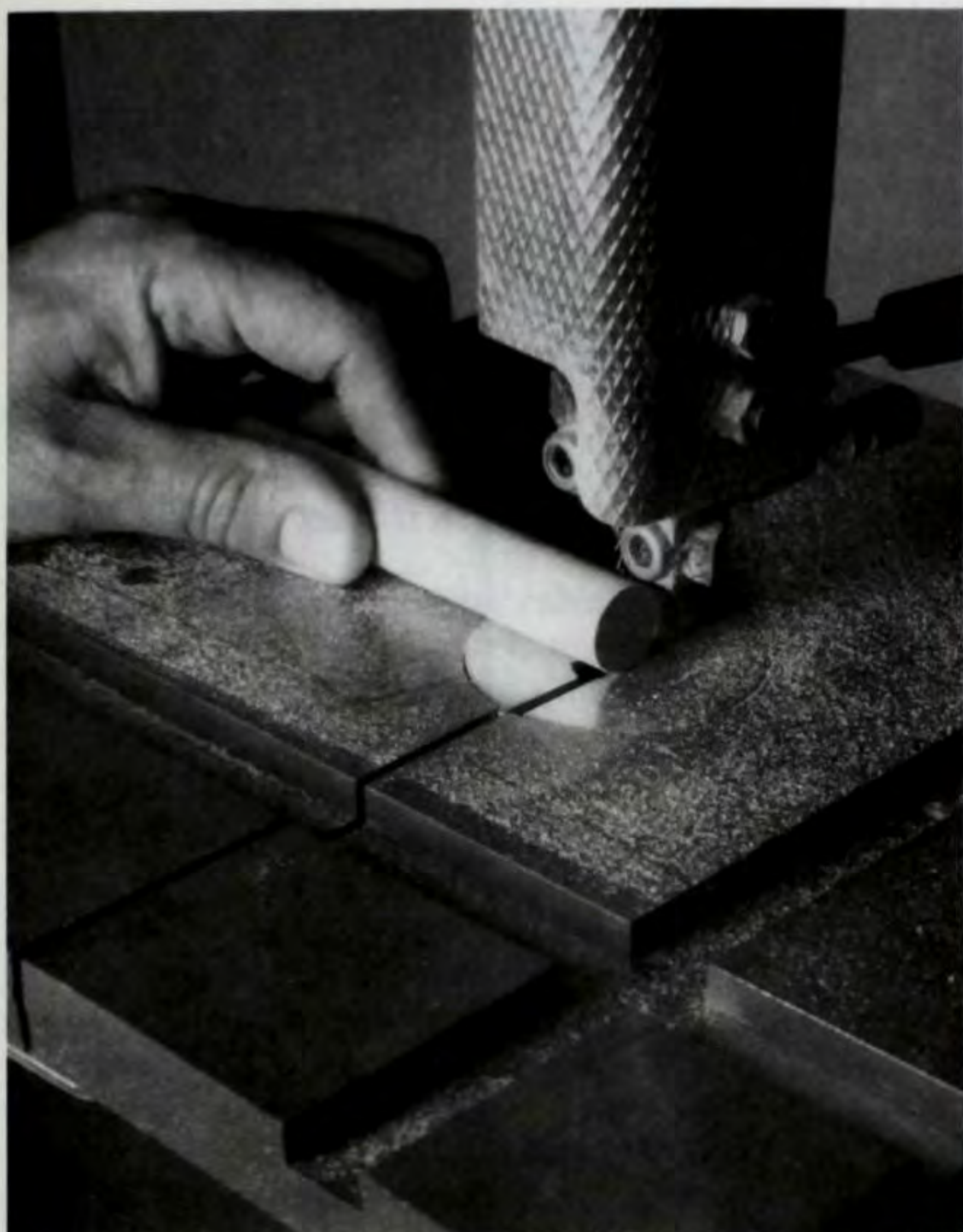
Figure 1. Cut the dowels for the logs (F) to length on your band saw. Hold the dowel firmly while cutting to prevent it from turning and binding.
