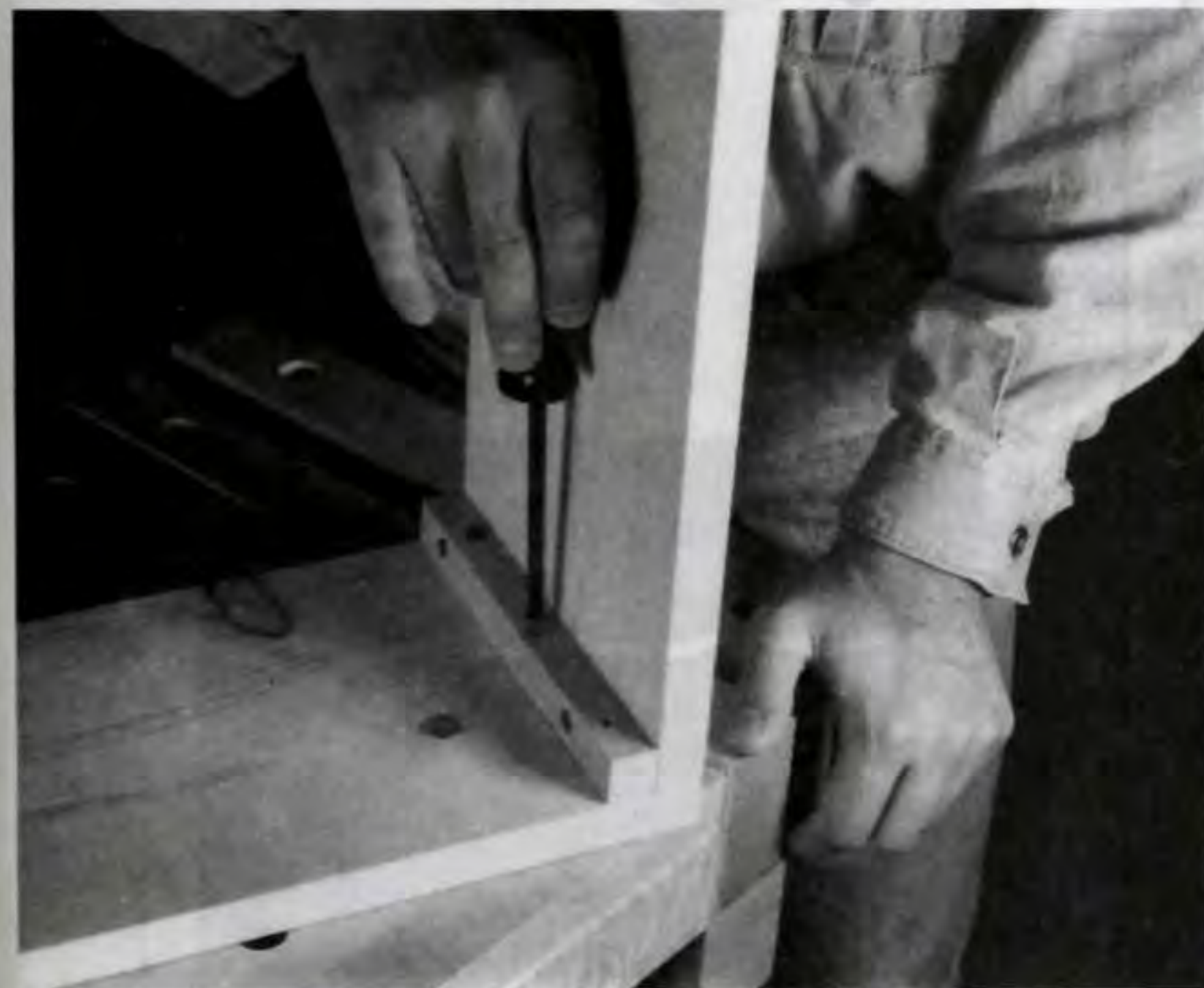
Figure 1. Assemble the sides (A) by driving drywall screws through a corner cleat, into the sides. Pre-drill these holes to prevent the cleat from splitting.
