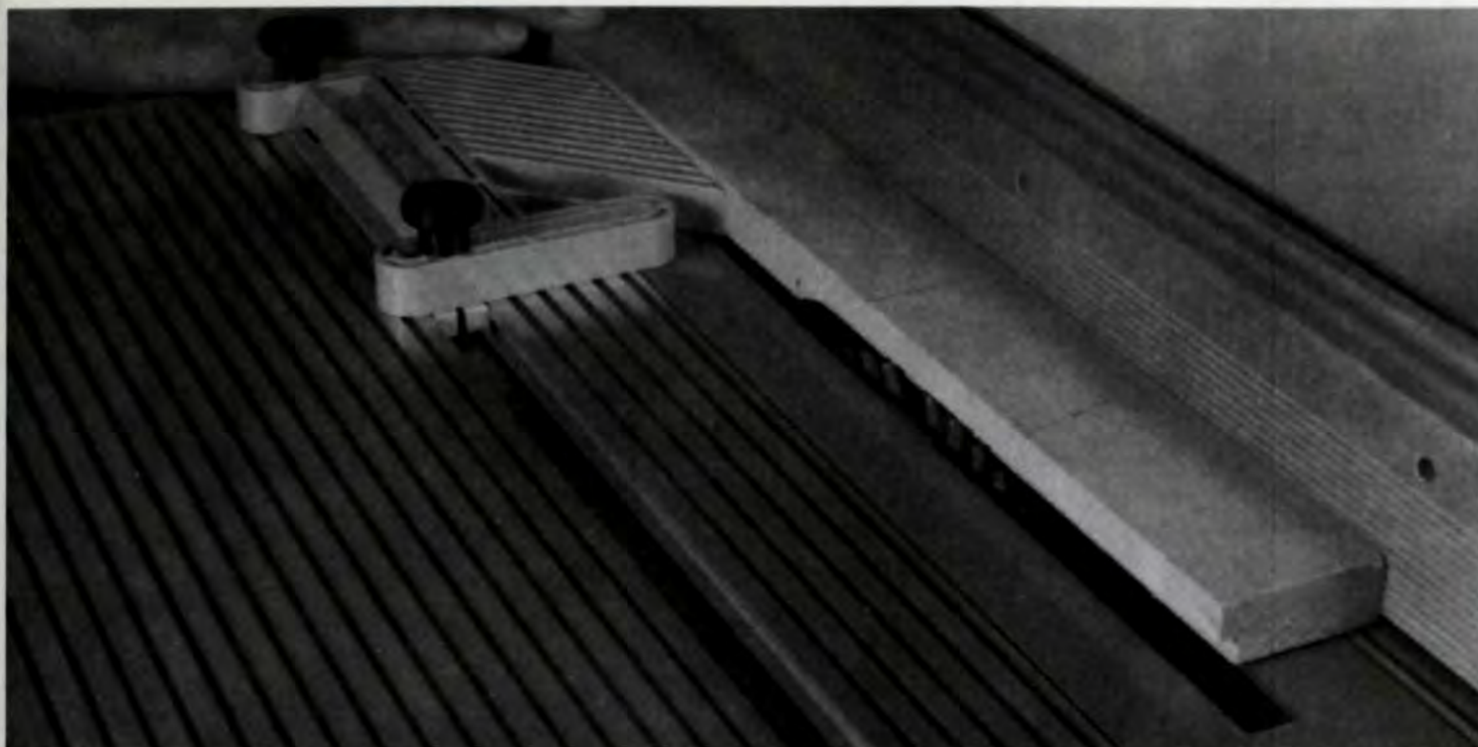
Figure 1. Rabbet the sides (D) on your table saw using a dado blade. Work from a long length of material, since short lengths can be difficult to mill on a table saw.
