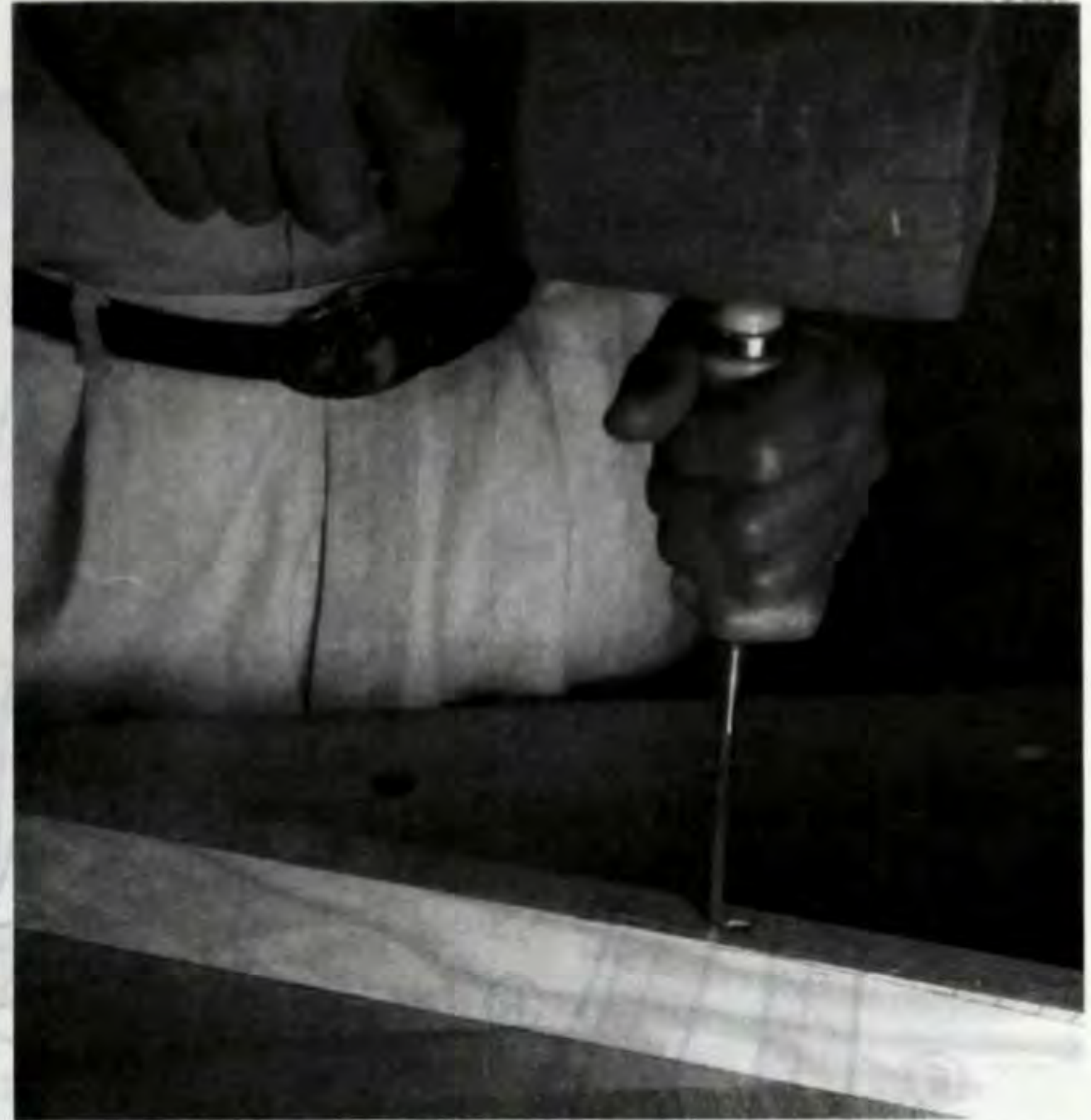
Figure 2. Lay out and then cut the mortises into the legs (A). Use a sharp wood chisel and stay short of the cutting lines when making your rough cuts. After the hole is rough cut, finish to the cutting line with your wood chisel.
