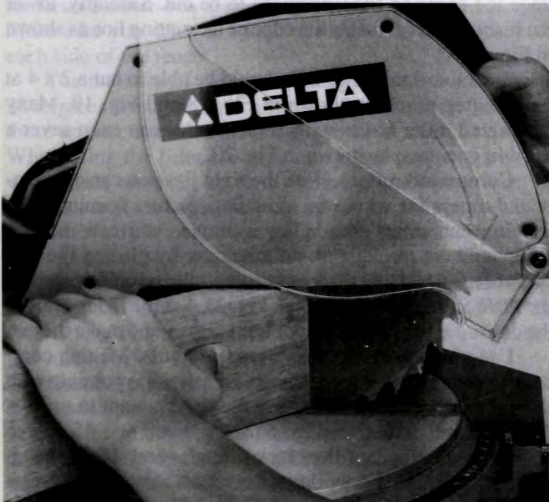
Figure 19. Mitering a 2 x 4 placed upright.
