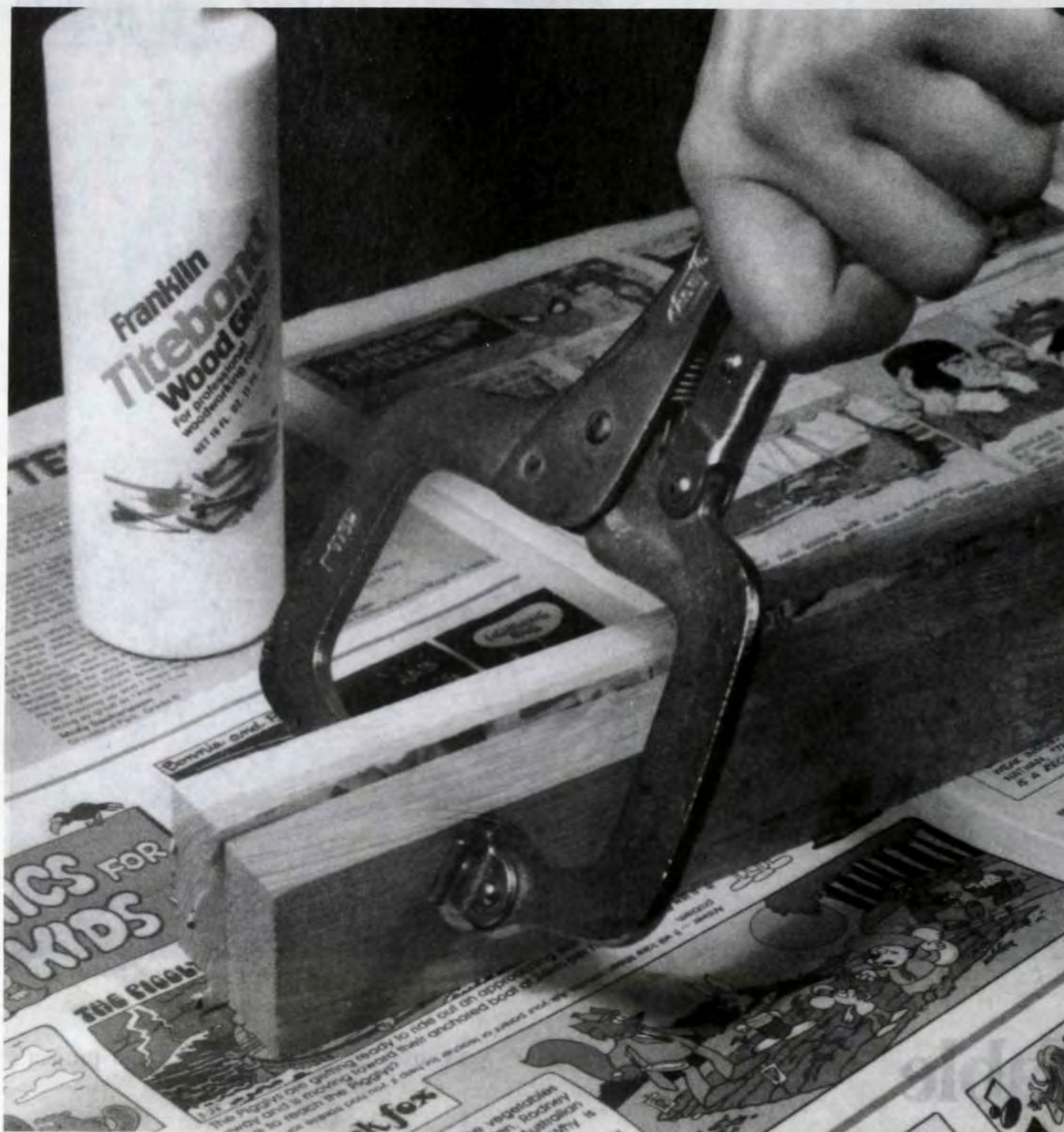
Figure 1. Surface glue two pieces of stock together with newspaper sandwiched in between to turn the half-round leg caps (I).
