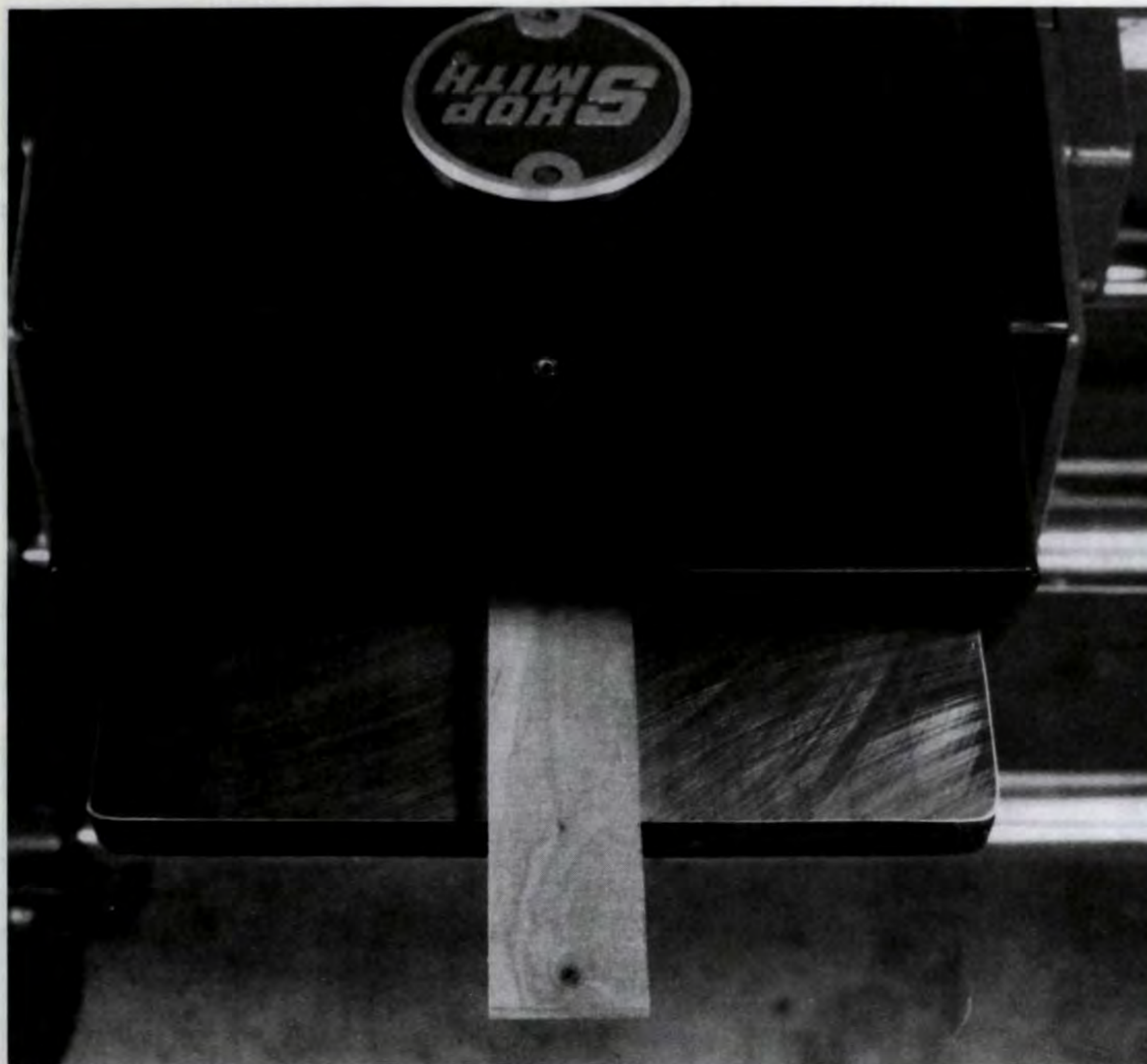
Figure 1. Use a thickness planer to thickness the material. Make light passes to reduce excessive wood tear.
