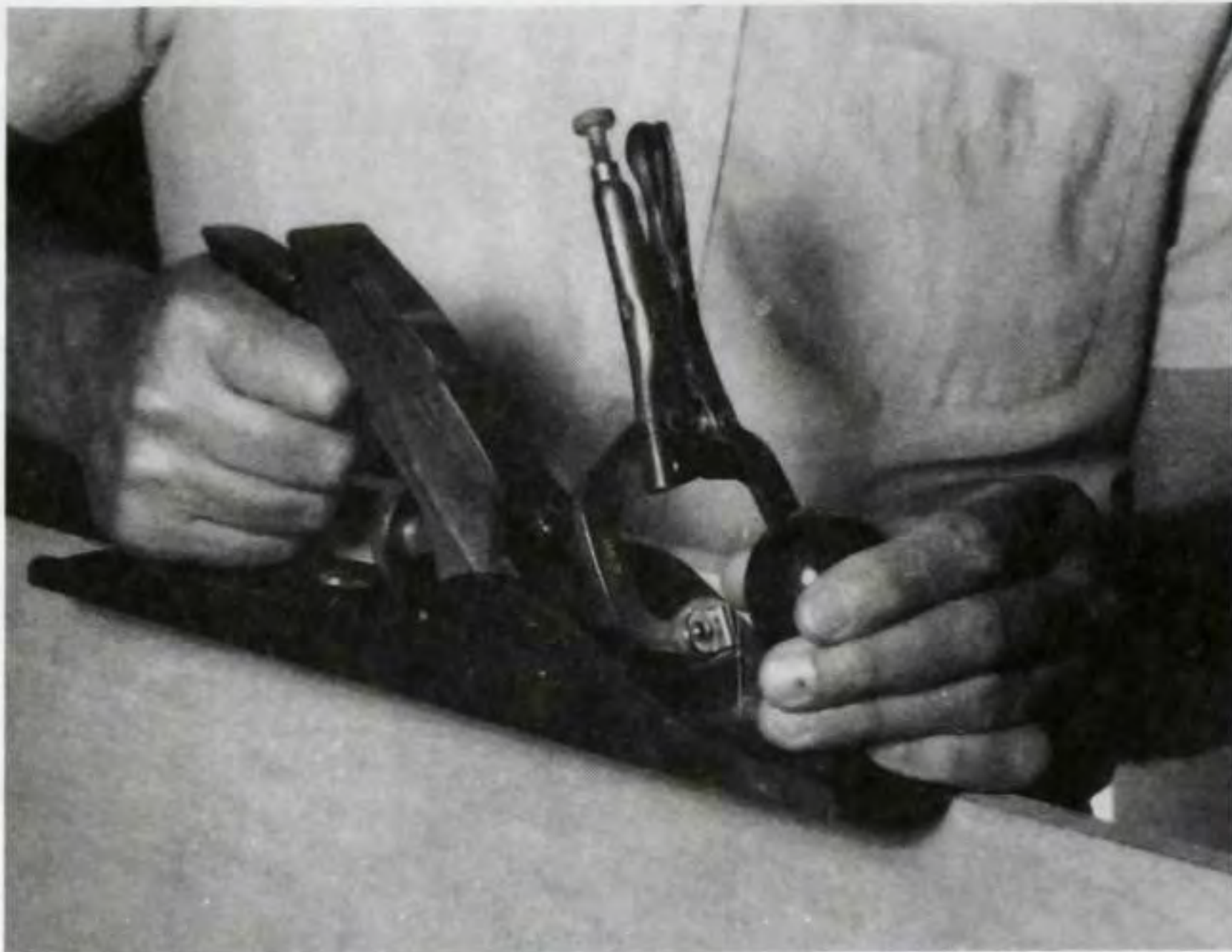
Figure 1. Use a portable hand plane to joint the plywood edges. Use the tool's edge-guide to keep the jointer perpendicular to the wood's edge.
