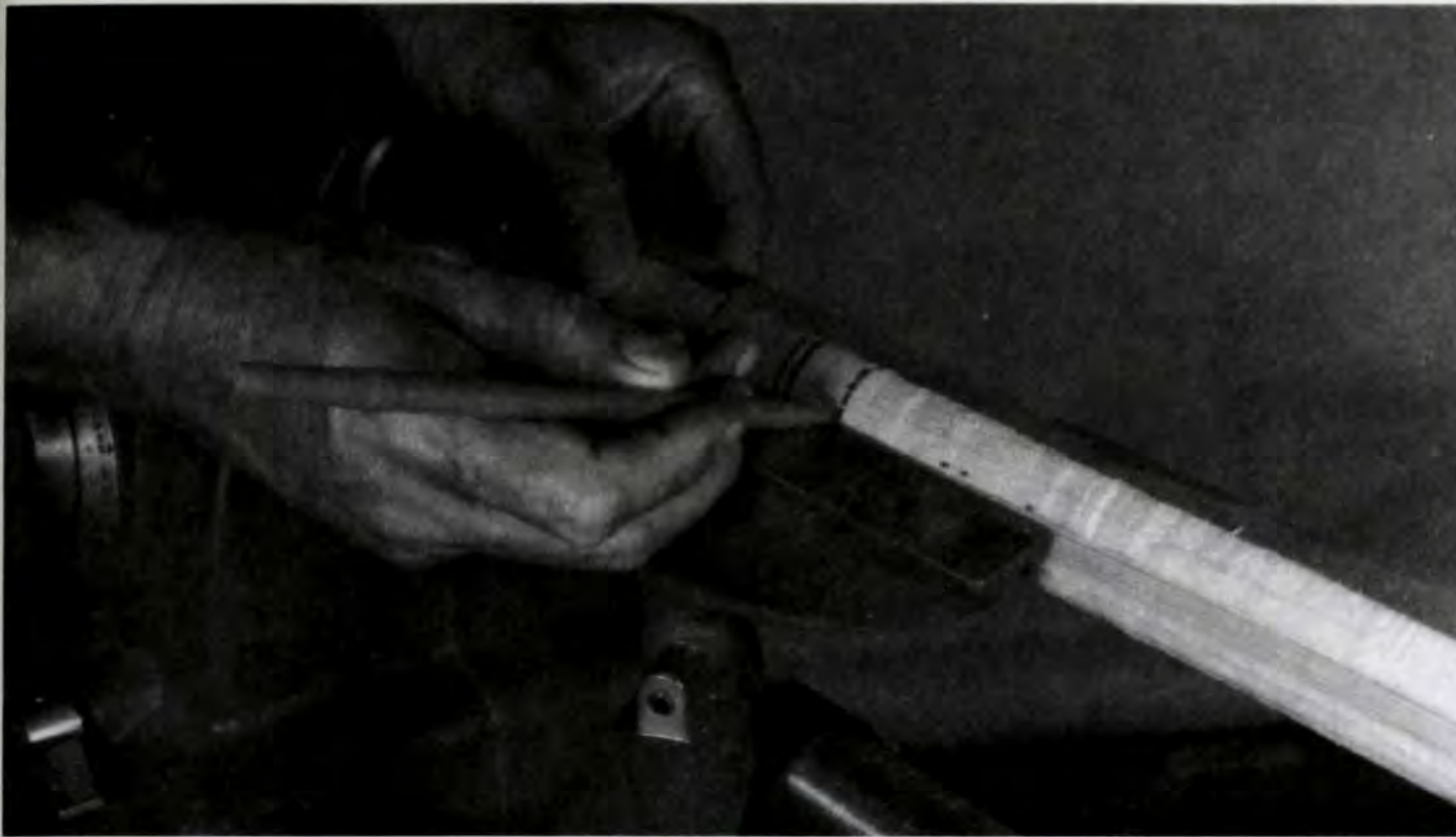
Figure 2. Mark the turning points on the legs (B) after turning the legs to a cylinder.
