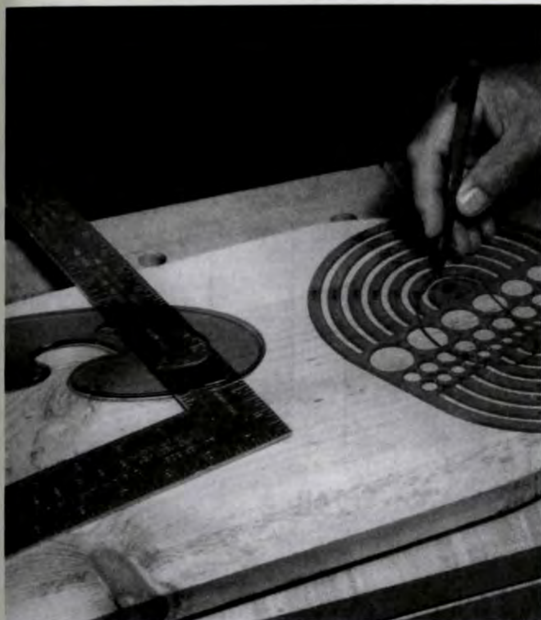
Figure 1. A radius template is ideal for laying out the handholds in the sides (A). Draw the curves of the sides with a bar compass.
