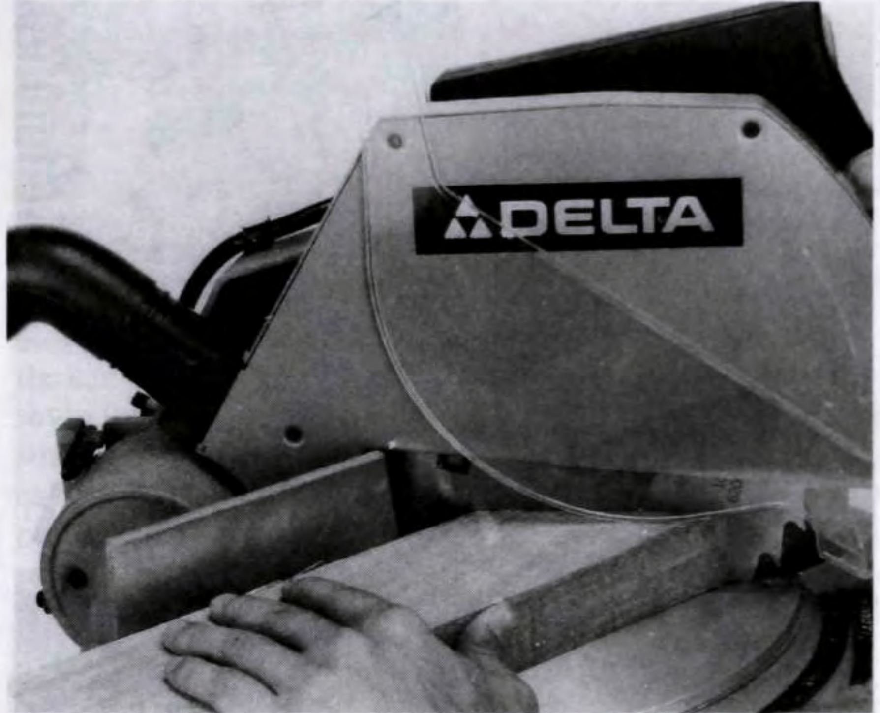
Figure 18. Mitering a 2 x 4 laying flat.
