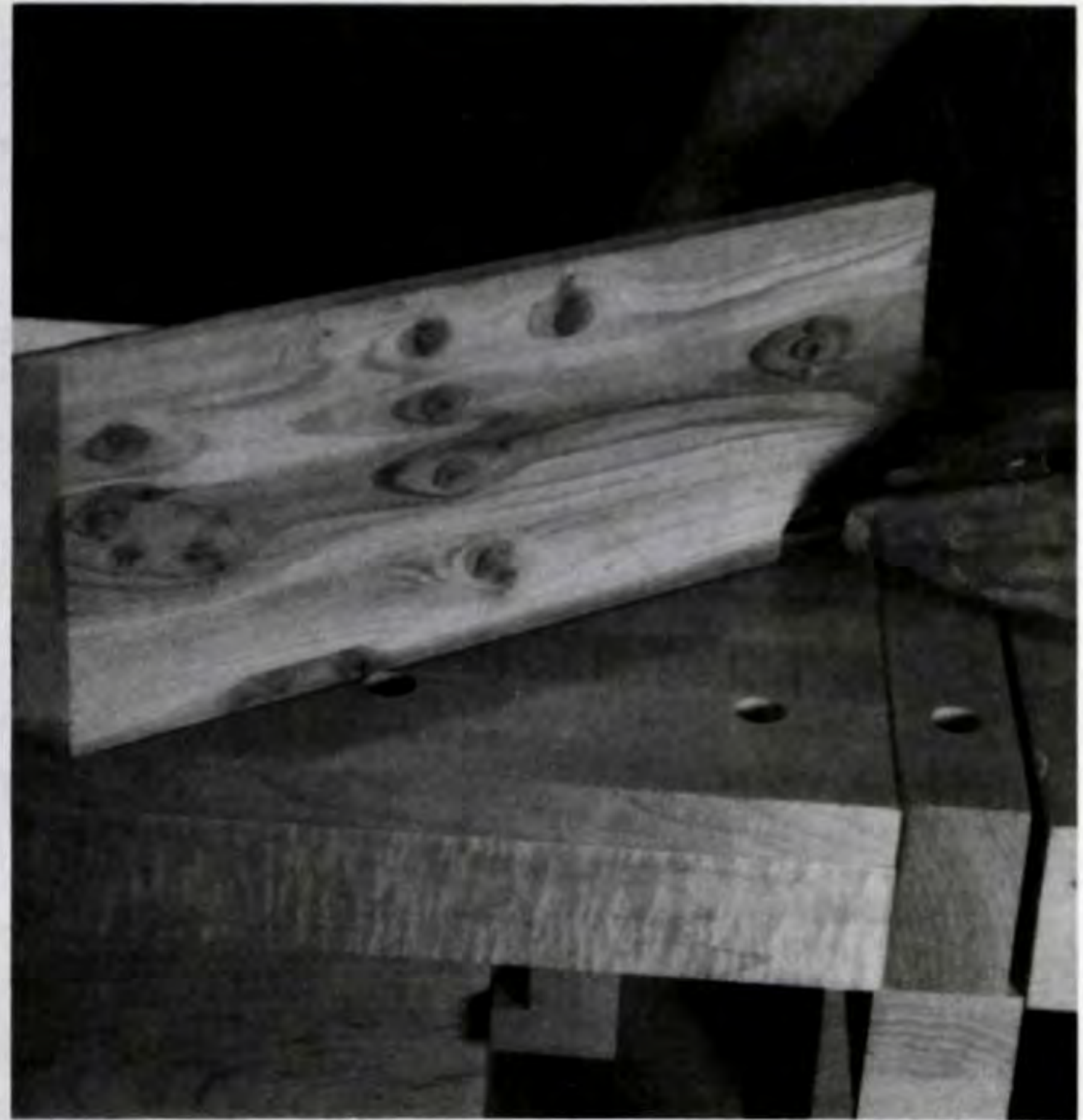
Figure 2. Cut the sides (C) oversize and make a 45 degree miter with a saber saw. Then position the side workpieces next to the front as shown. Mark the sides to their correct length and cut.
