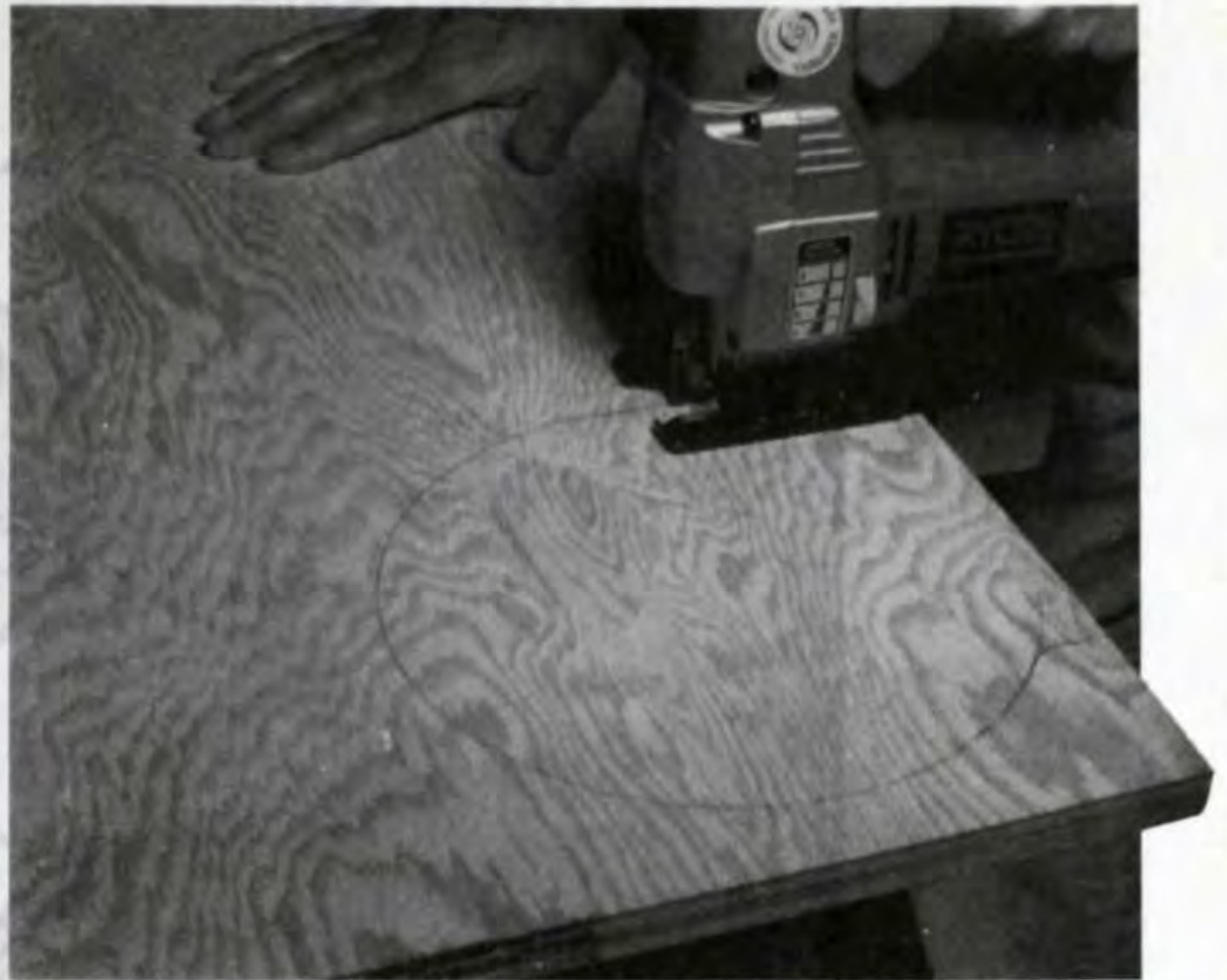
Figure 2. Cut out the design with a saber saw equipped with a plywood cutting blade. Work slowly.
