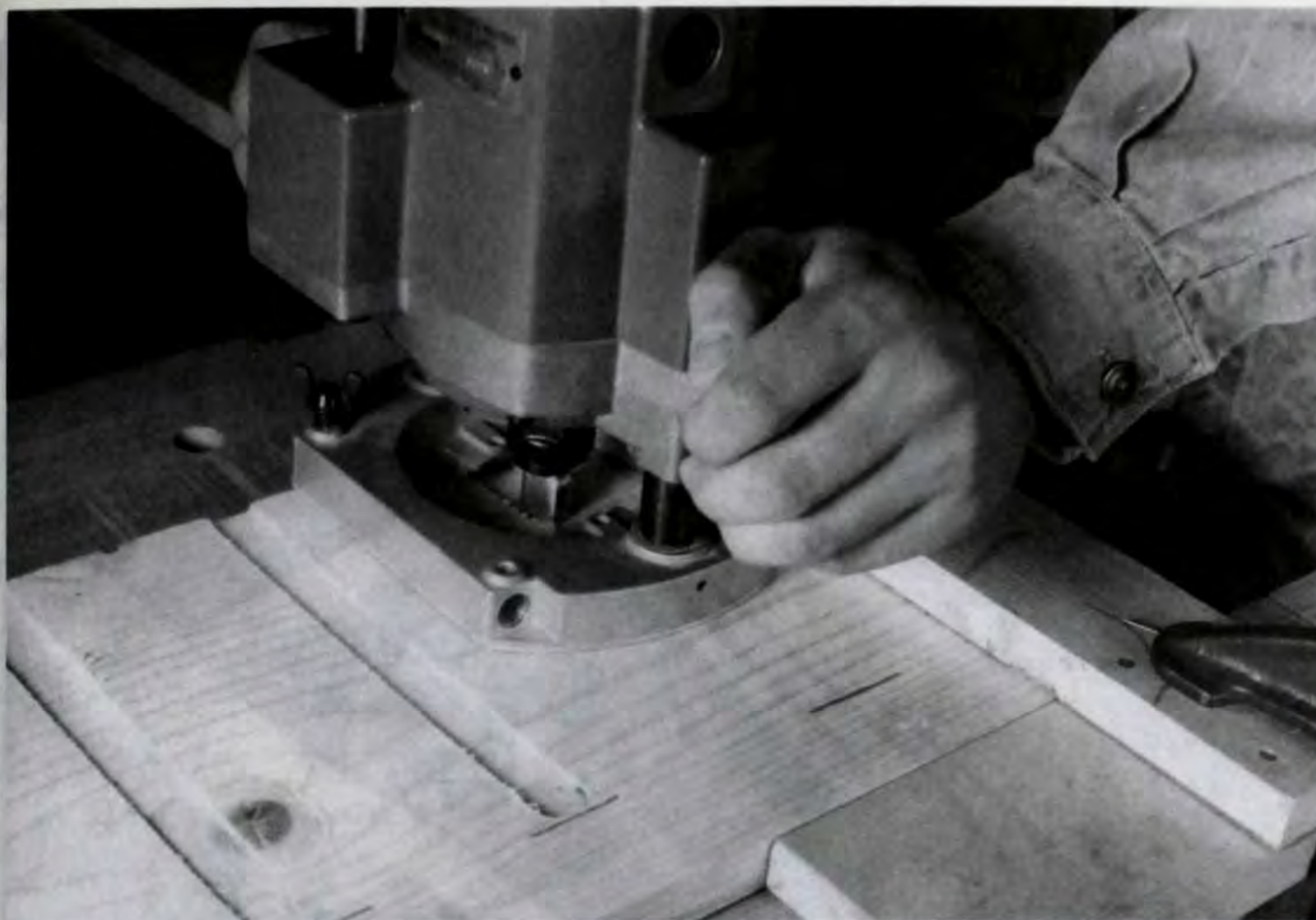
Figure 5. Cut the dados in the cabinet top (R). If you do not have a radial arm saw, use a T-square guide to help you align a router equipped with a \frac{3}{4} in. straight bit.
