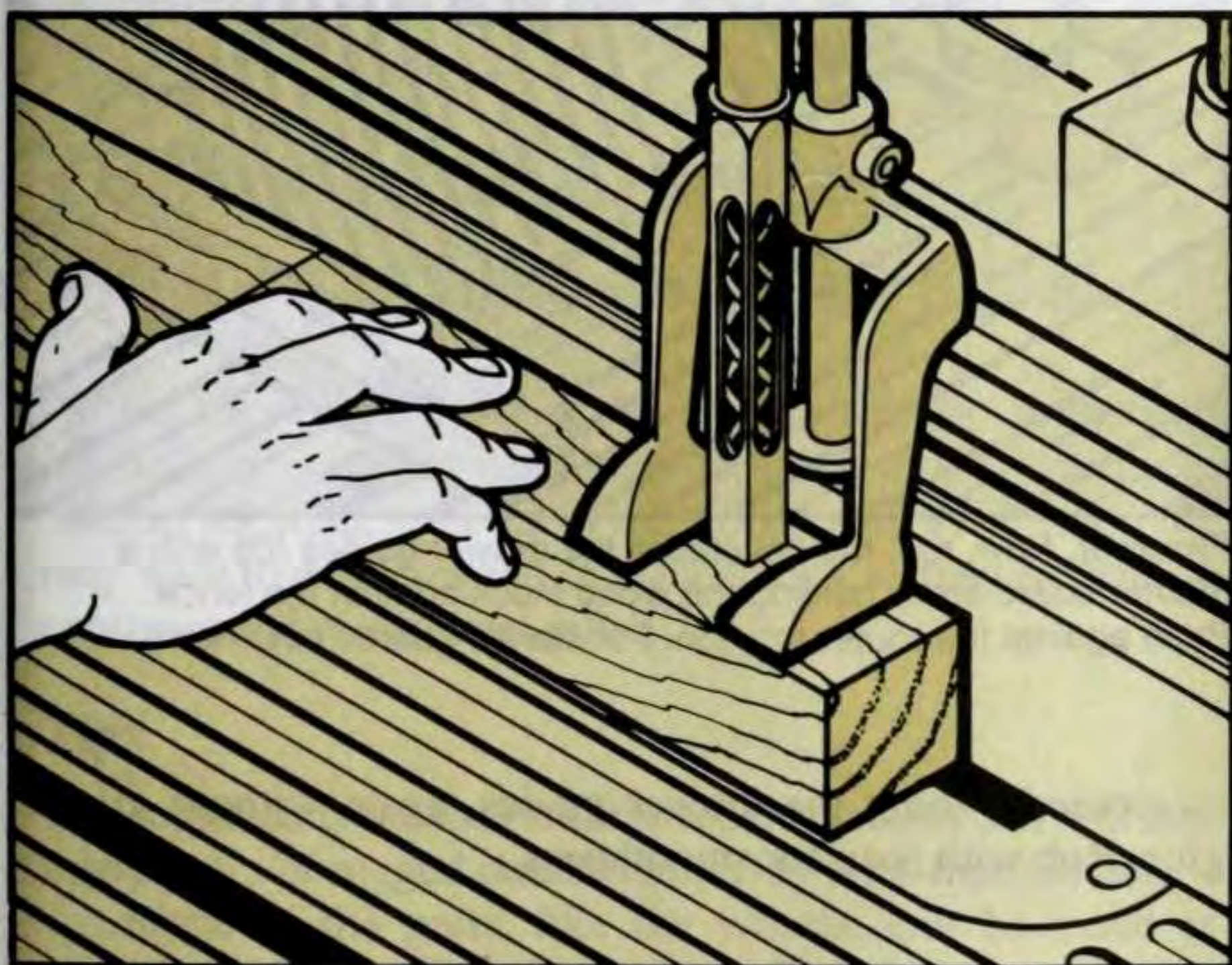
Figure 3. Cut the mortises in the legs (A) with a sharp \frac{3}{8} in. mortising bit/chisel.
