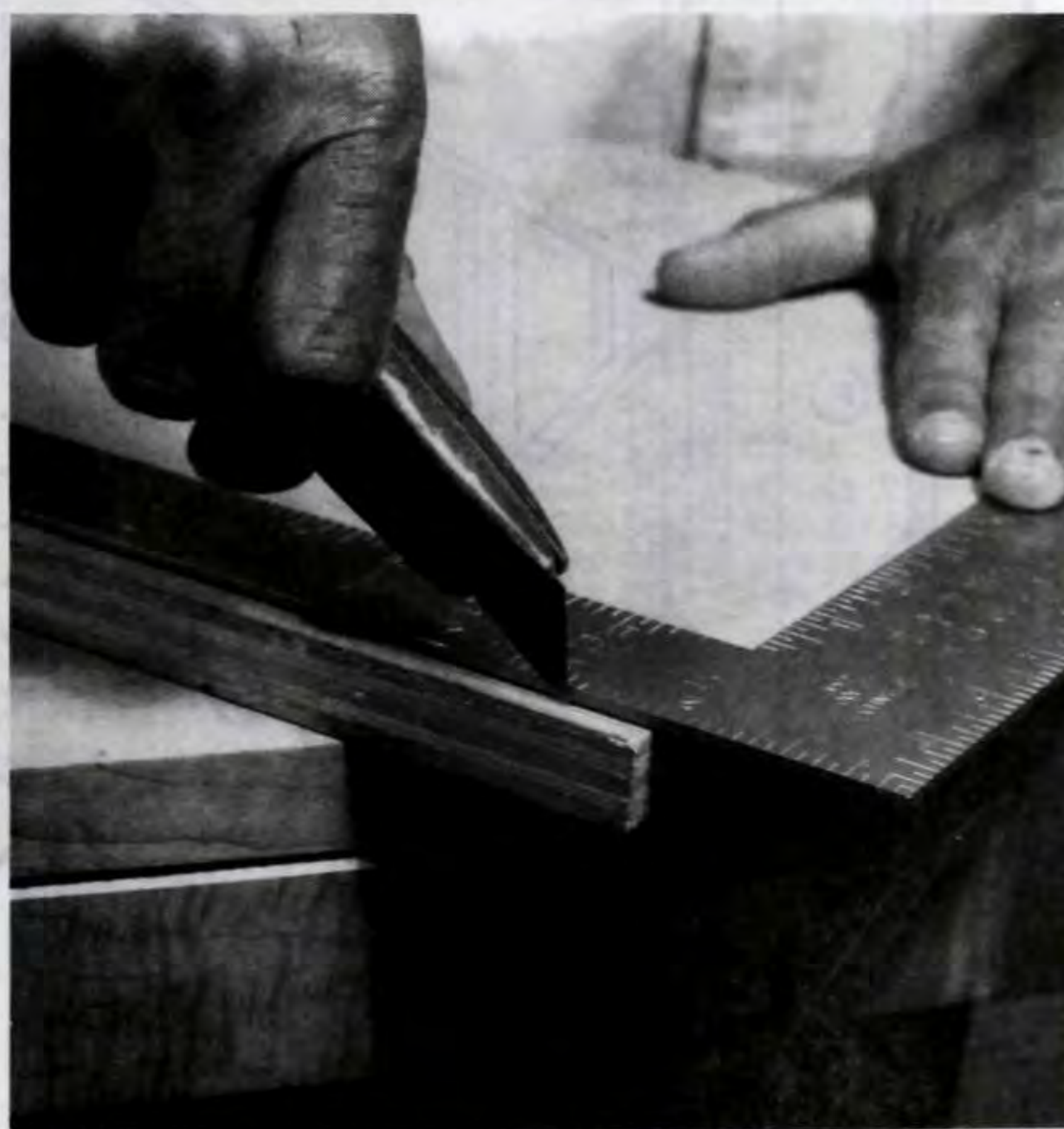
Figure 2. If your blade causes too much wood tearout, run a utility knife along a clamped carpenter's square. Then cut up to this line, not on it, with your saw. This scored line must be on the tearout side of the blade.
