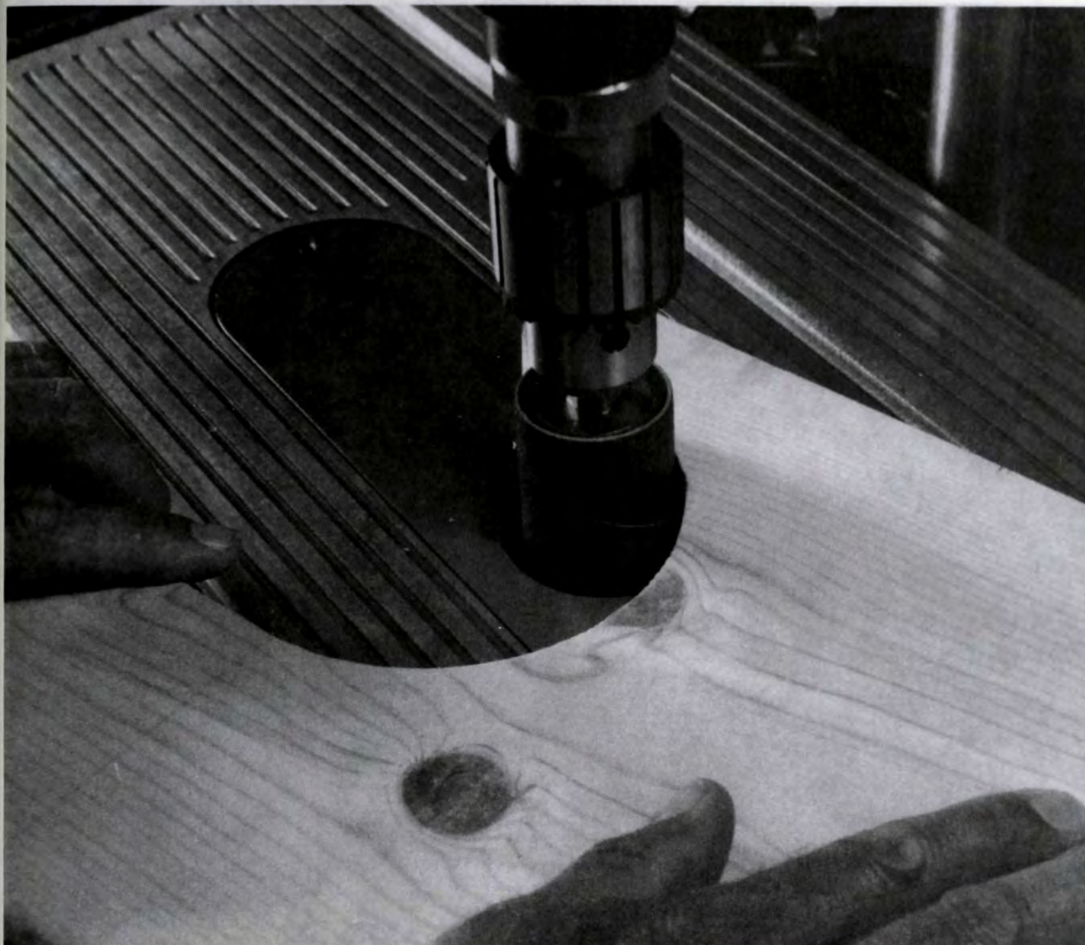
Figure 4. Sand the circular areas of the sides with a drum sander installed in your drill press. Use fine grit sandpaper and move the wood into the rotating drum.
