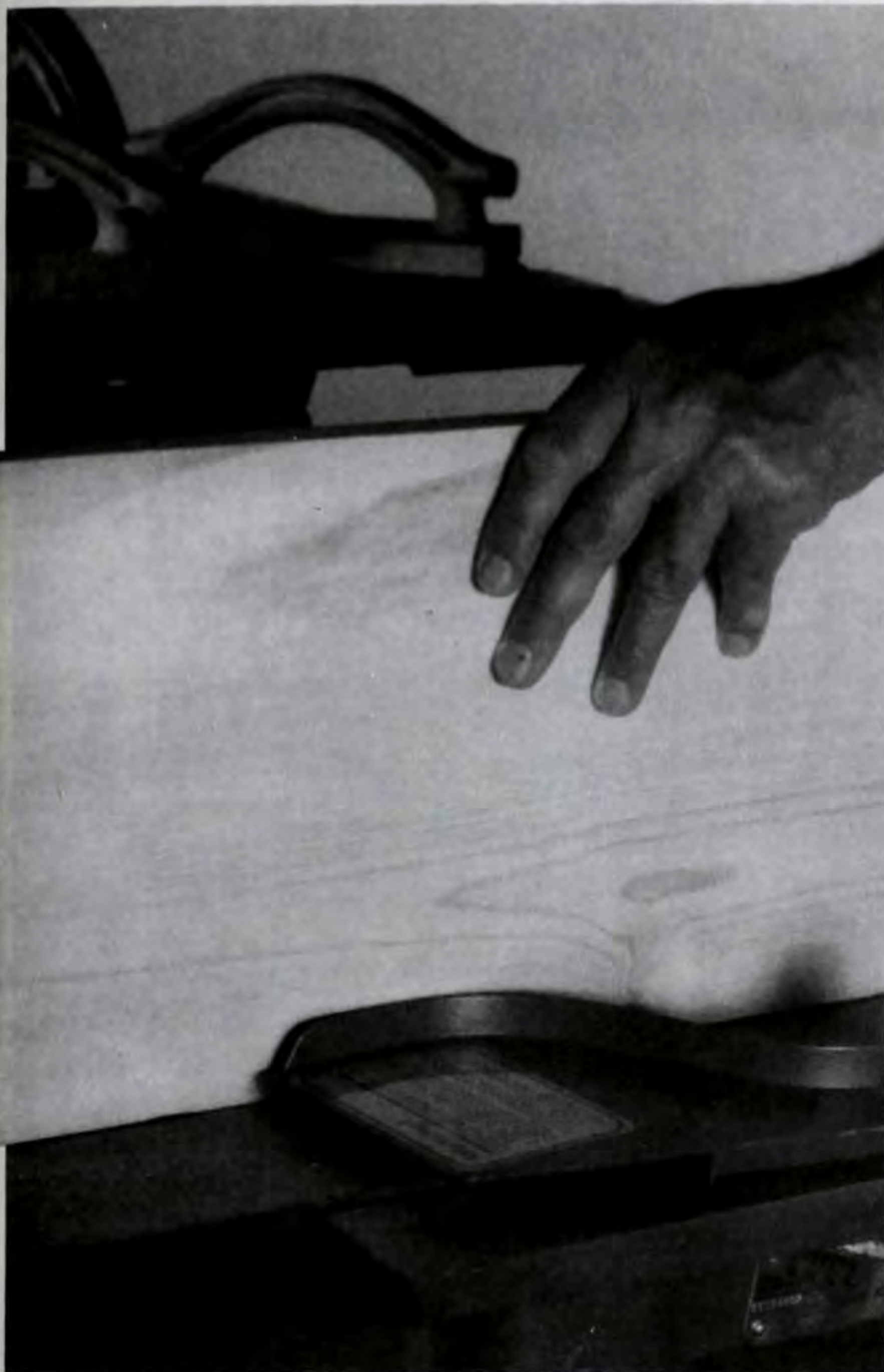
Figure 1. Joint the lumber to be edge-glued to form the sides (A). Use a stationary jointer and make a smooth continuous pass. Keep fingers well away from the cutters.
