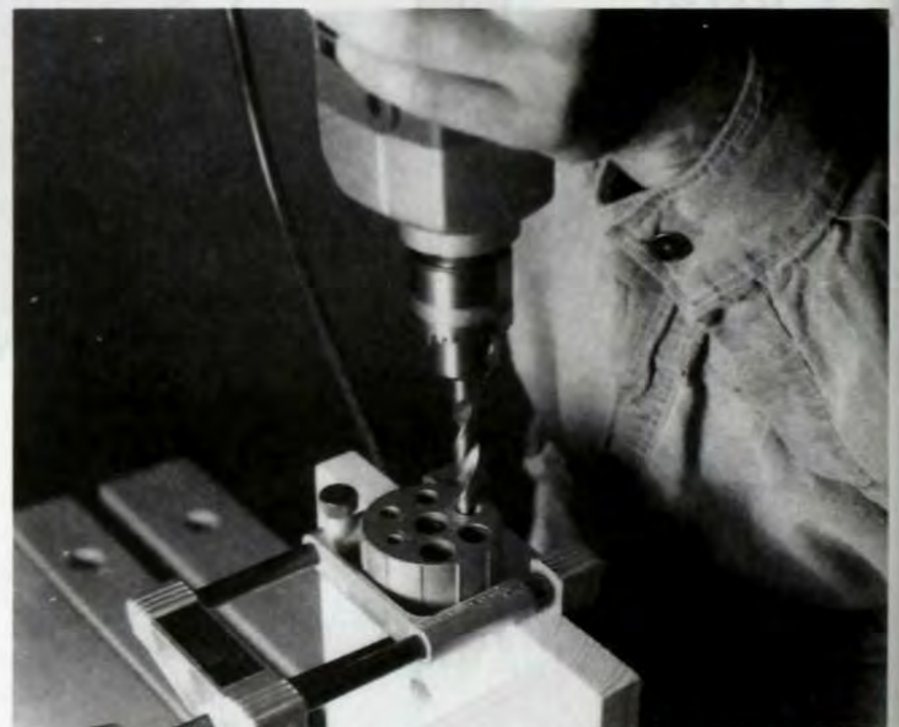
Figure 3. Use a doweling jig to position and drill all dowel holes. Use a spur point drill bit.
