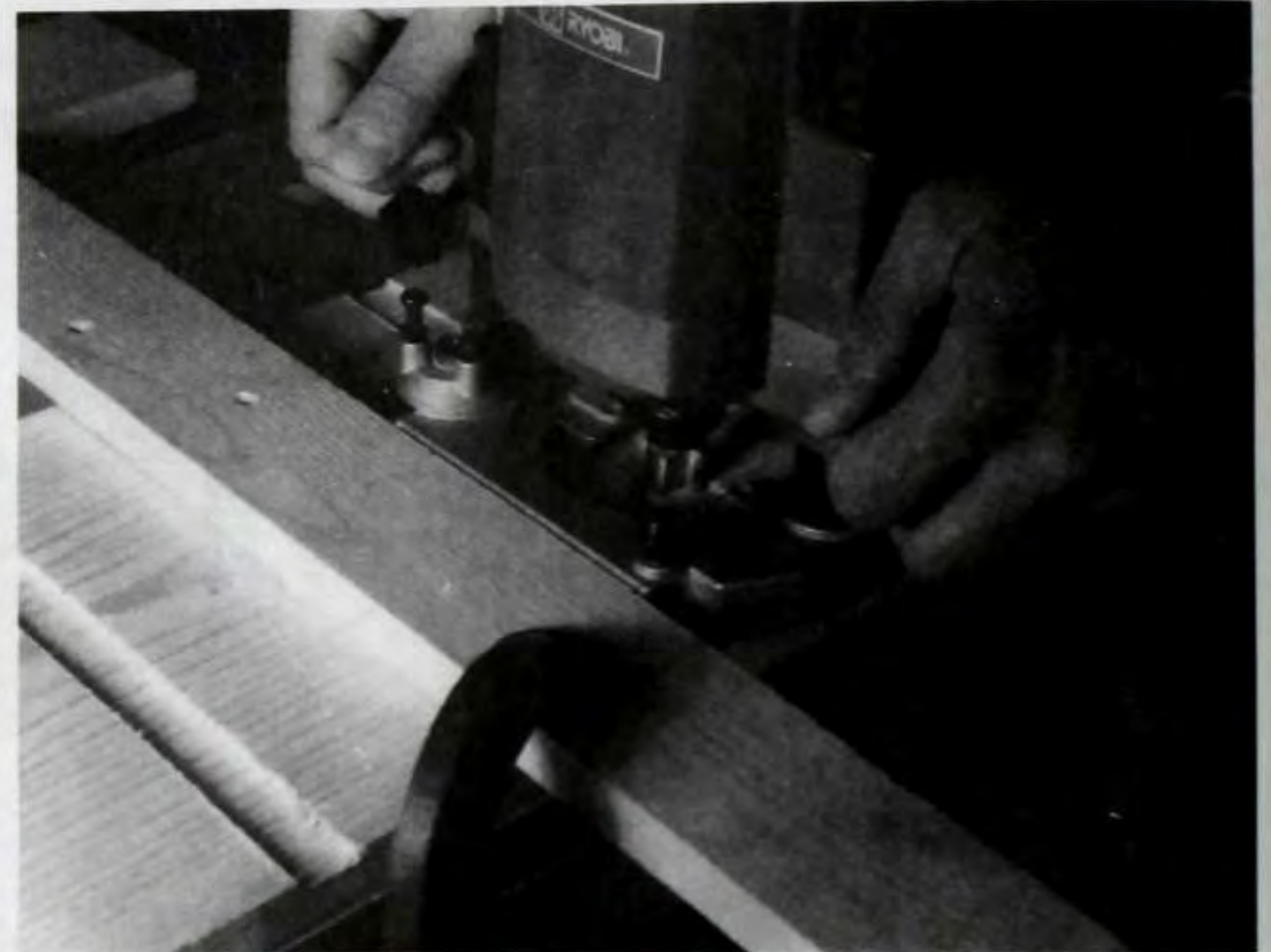
Figure 2. Use a router equipped with a straight bit to cut dados into the sides (B, K). Make progressively deeper passes with the router until it reaches final cutting depth.
