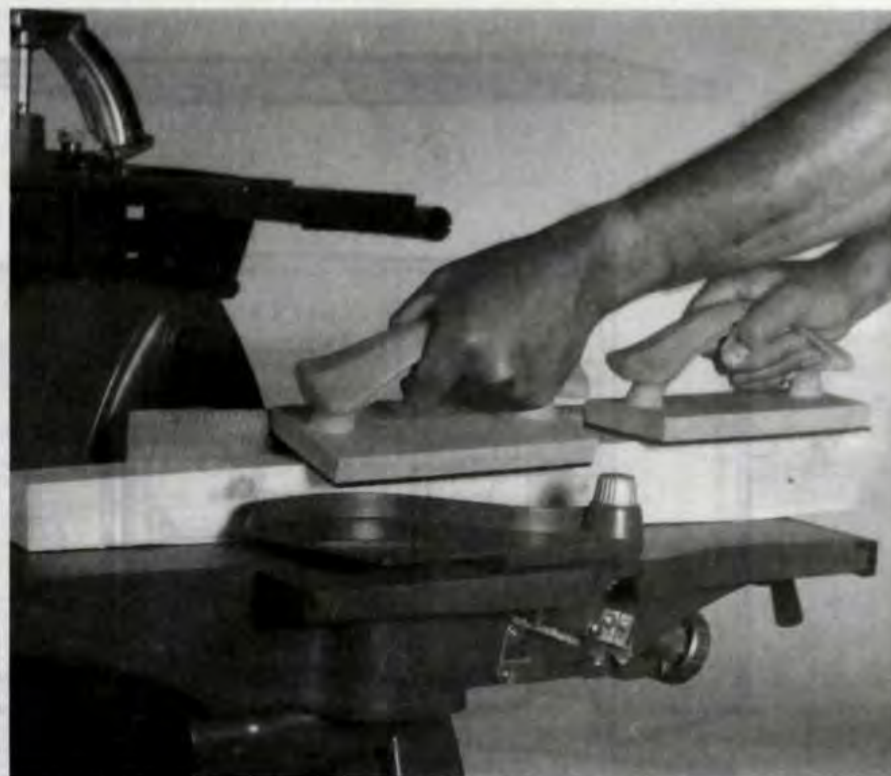
Figure 2. Joint the leg tapers on your jointer. Use a holding jig to prevent your fingers from inadvertently slipping into the cutterhead. Make light 1/32 in. or less passes.
