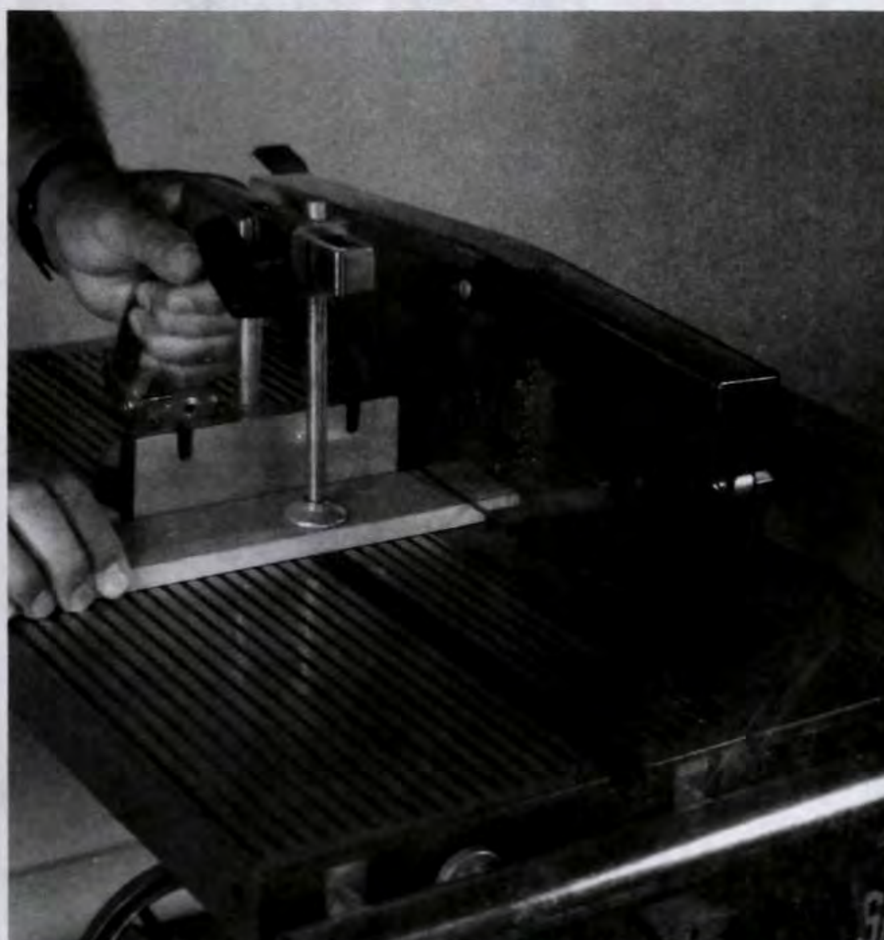
Figure 2. Cut half-laps into the edges of the stiles (A) and rails (B) with your table saw set to one-half the wood's thickness. Use a dado blade to make these cuts.
