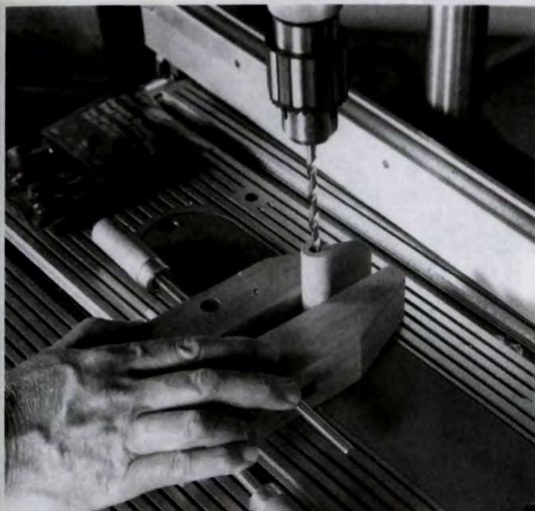
Figure 2. Drill \frac{5}{16} in. diameter holes into a length of \frac{3}{4} in. diameter dowel, held in place with a wood clamp. Then cut the spacers (C) to length on a band saw.
