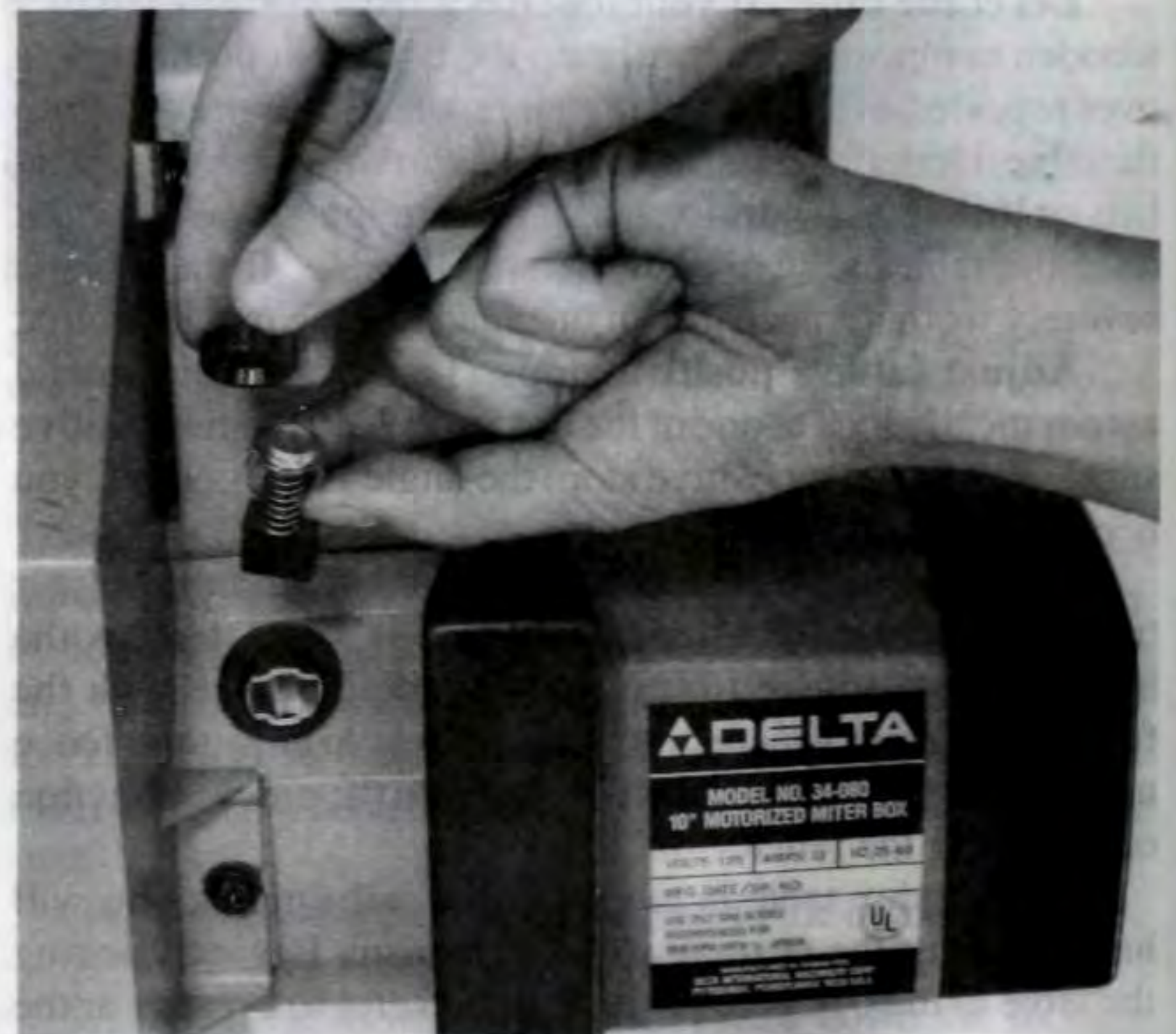
Figure 14. Inspecting the motor brushes.
