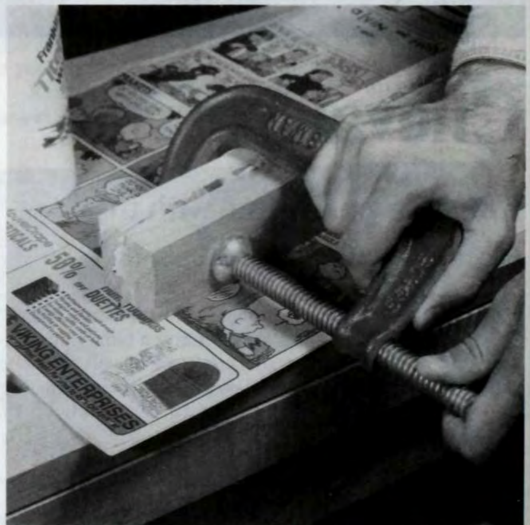
Figure 4. Surface-glue long pieces of material to form the spindle stock (A). Use carpenter's glue and secure the stock with C-clamps.
