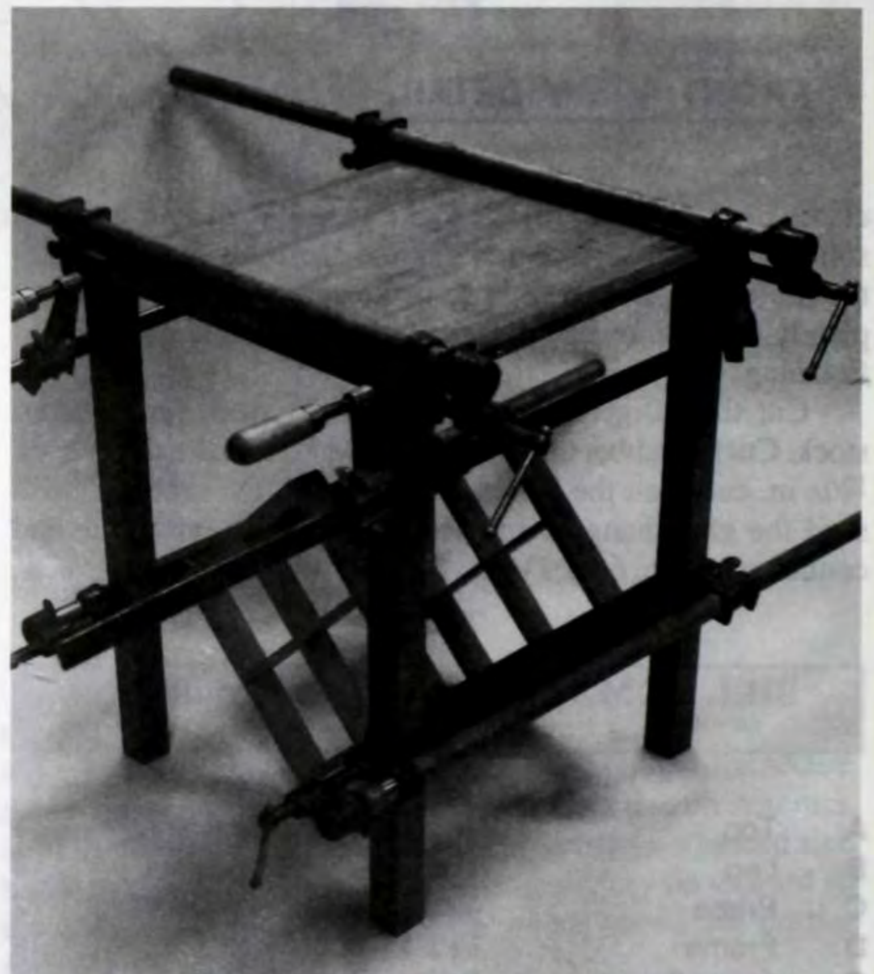
Figure 7. Glue the entire assembly, making sure the legs sit solidly and the unit is square. Allow the glue to cure for at least 24 hours.
