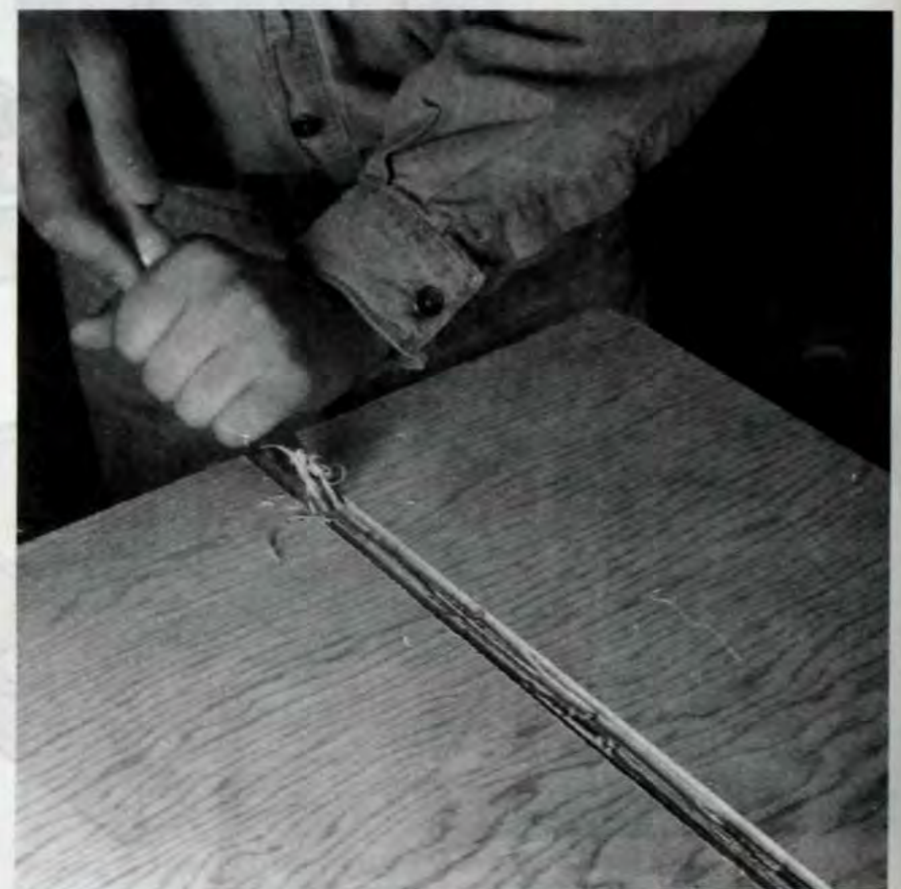
Figure 5. Finish the dado cut with a sharp wood chisel. Never put your hand in front of the area you are cutting.
