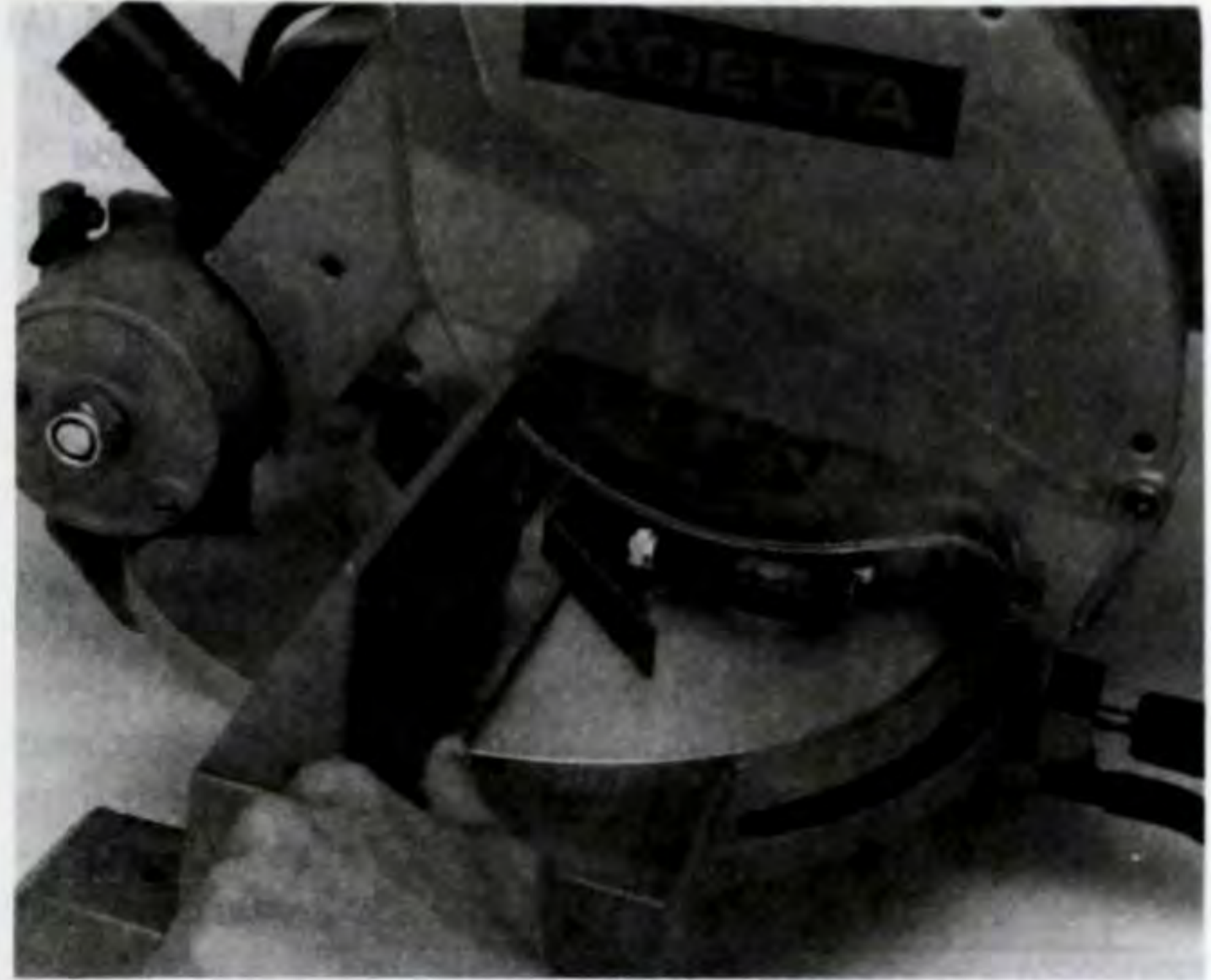
Figure 3. Checking to make sure the blade is 90 degrees to the fence.
