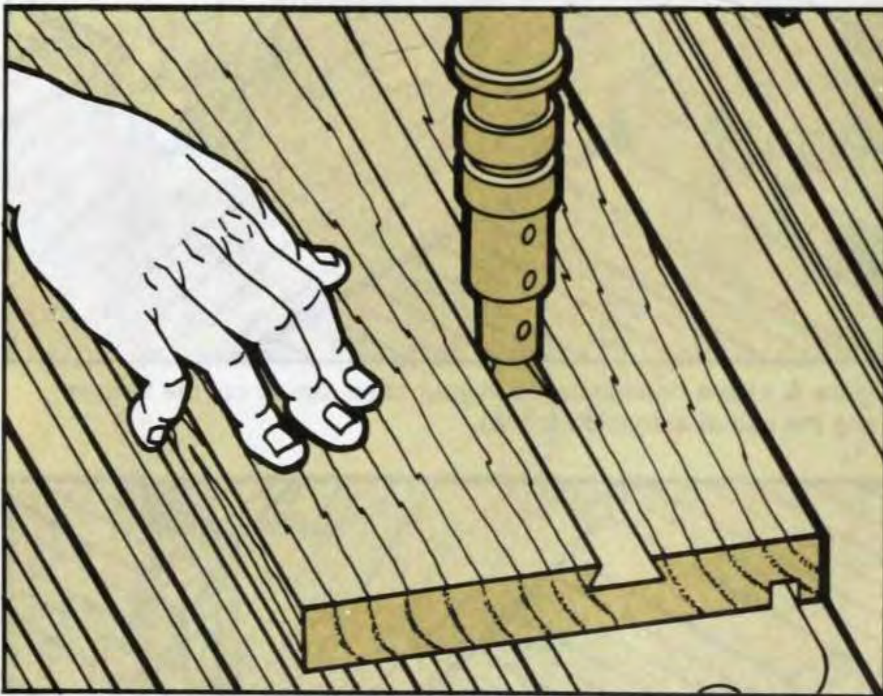
Figure 8. Also rout a dovetail slot into the drawer sides (J). Two passes are needed, both at a full 1/4 in. depth. For clarity, guards not shown.
