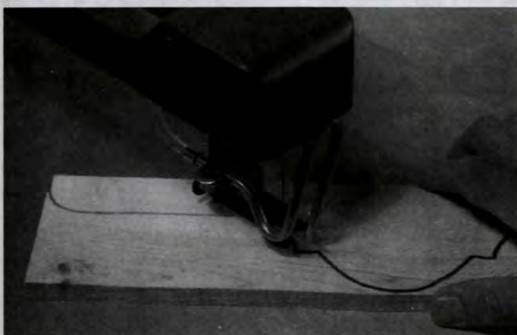
Figure 2. Lay out the design for the upper back (E) and cut out with a scroll saw. Keep the blade guard \frac{1}{8} in. or less above the wood.
