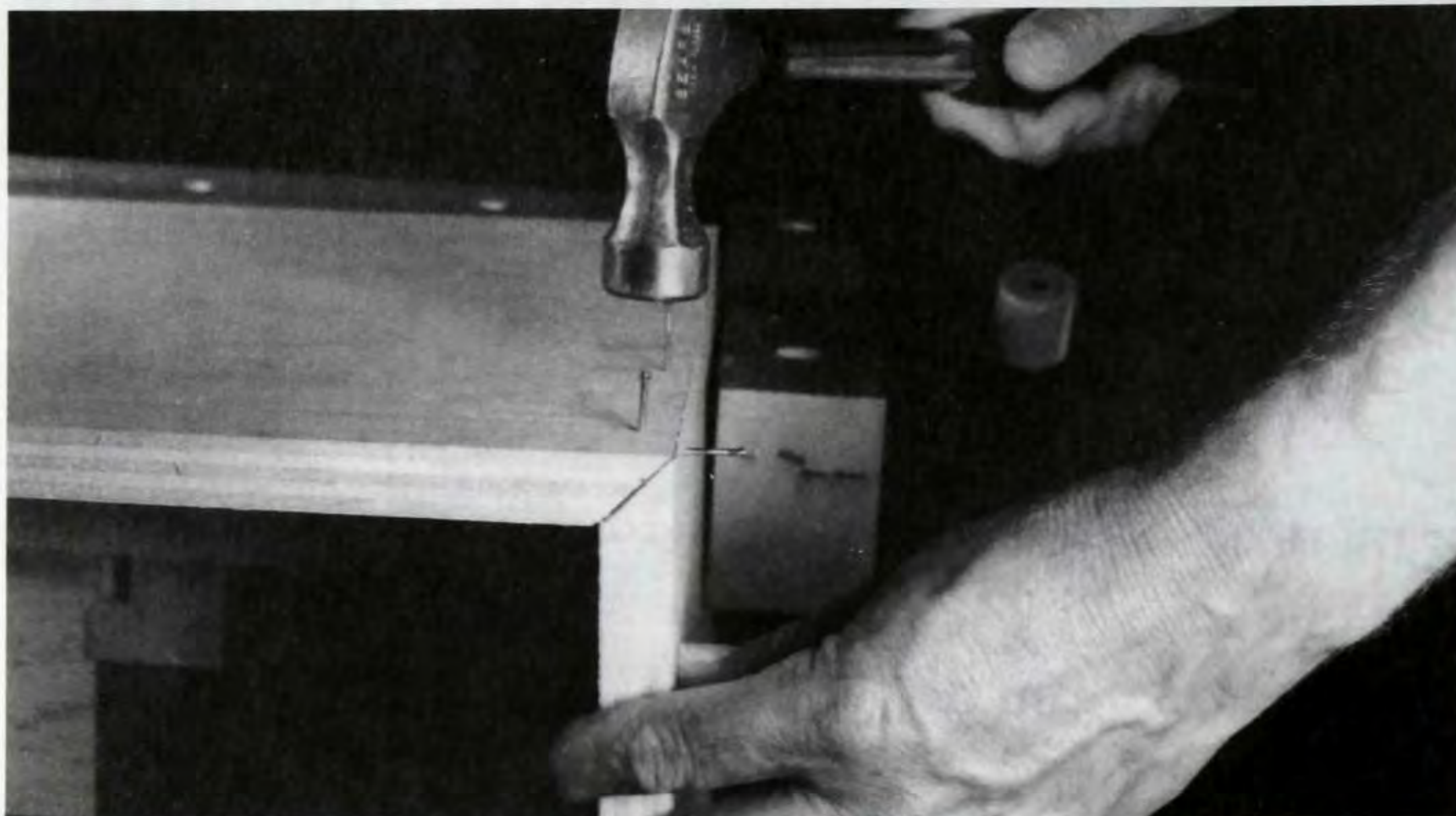
Figure 1. Drive finishing nails into the side's mitered edges while alternating nail placement, as shown. This makes a stronger joint. Don't forget to add glue.
