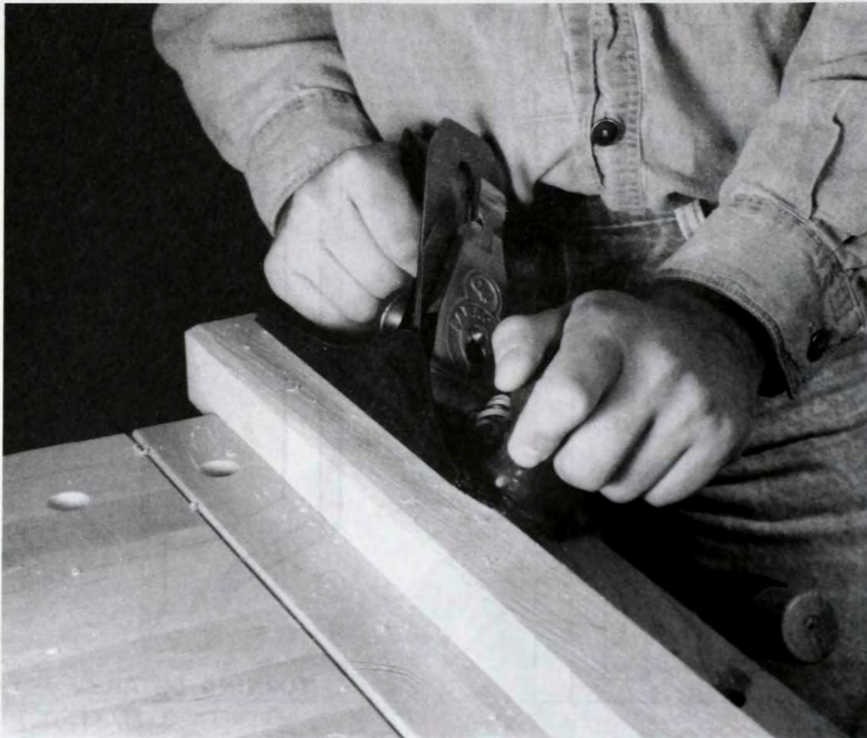
Figure 5. Taper the spindle stock (A) with a bench plane. This saves time and wear on your lathe tools.
