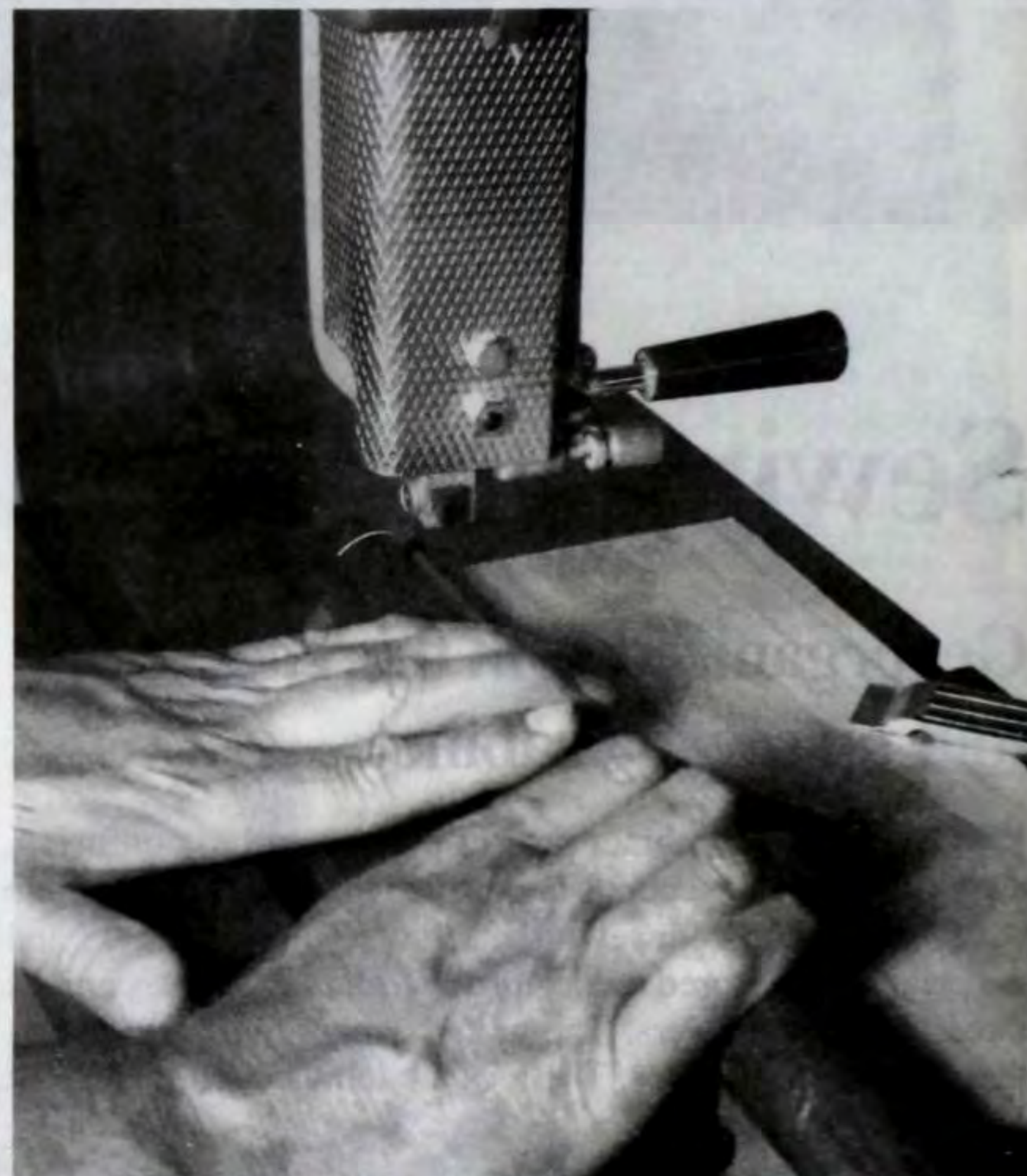
Figure 2. Now, move the leg into the blade and rotate the leg clockwise so the wood is moved into the cutting blade and not with the cutting blade. Hold the dowel firmly and keep fingers well away from the blade.
