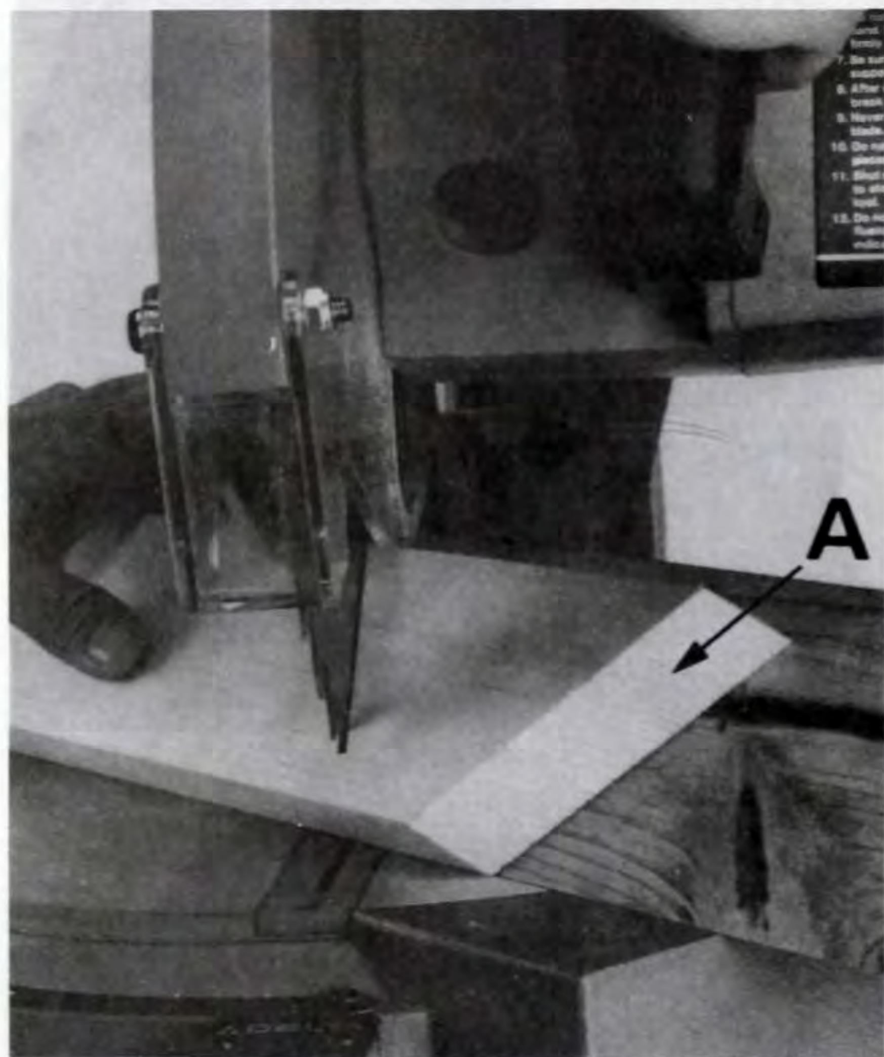
Figure 23. Cutting compound angle in rectangular material (A) against filler block.
