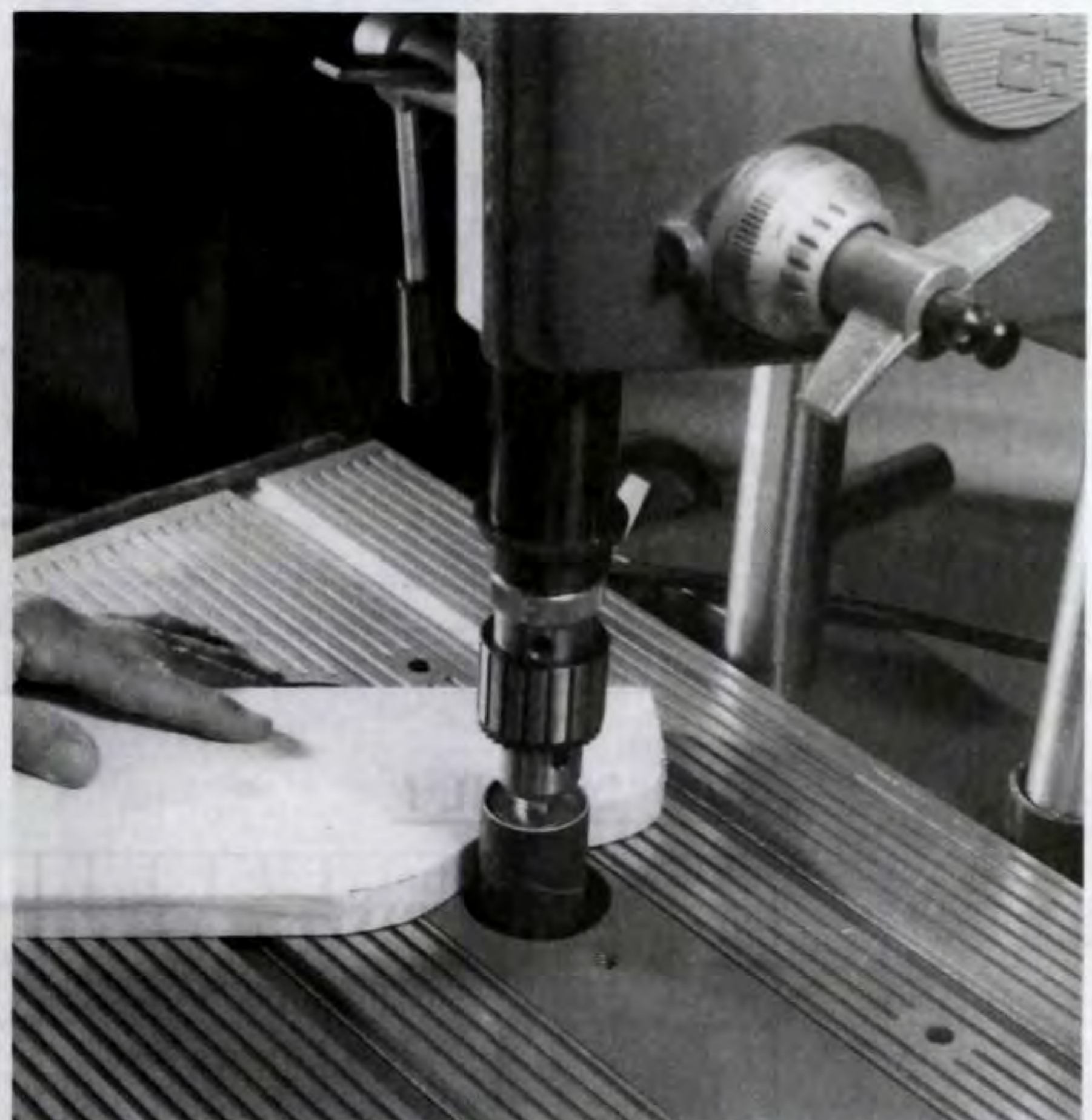
Figure 2. Sand the contours using a drum sander inserted in your drill press. Move the material into the drum.
