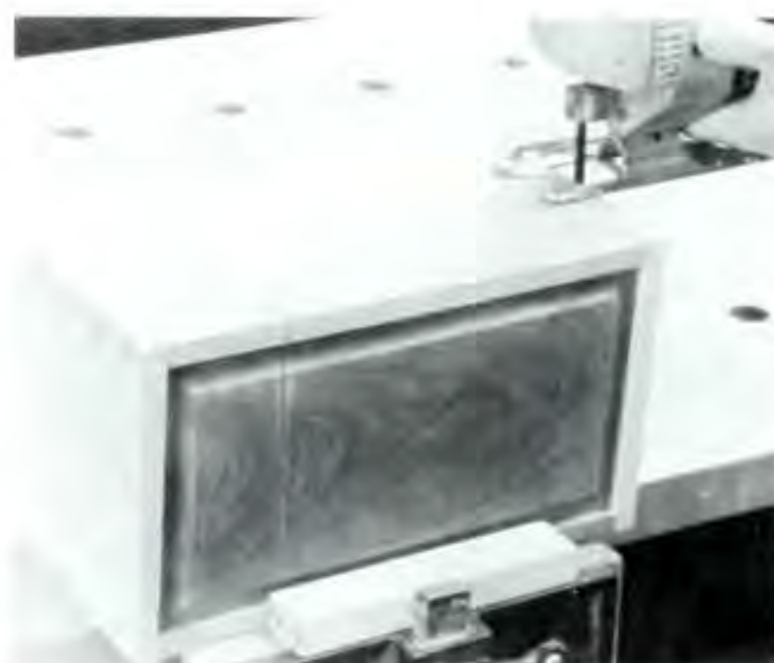
Figure 8. Cut the lid free from the box with a sabre saw. Use a fine blade for a smooth cut.
