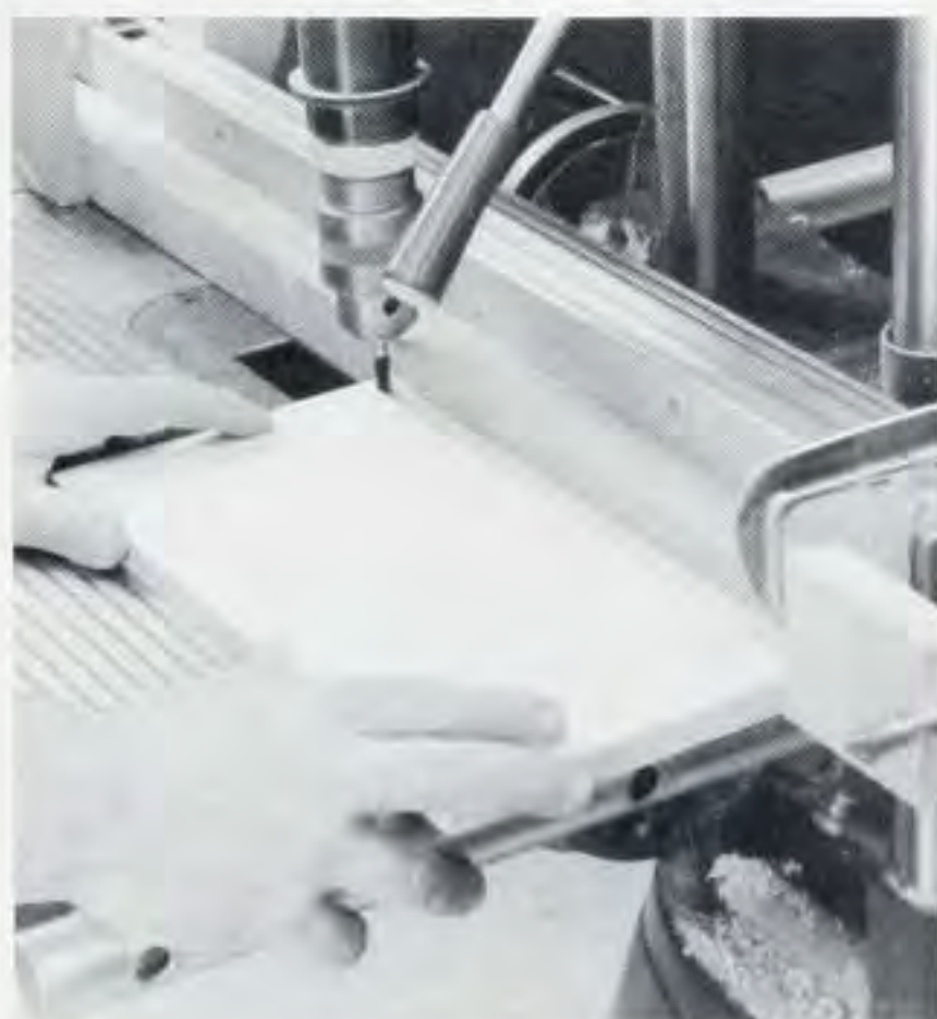
Figure 4. There are several special routing jigs that will help you cut through dovetails. In addition to the jig and a router, you also need a guide bushing, a dovetail bit, and a straight bit.
