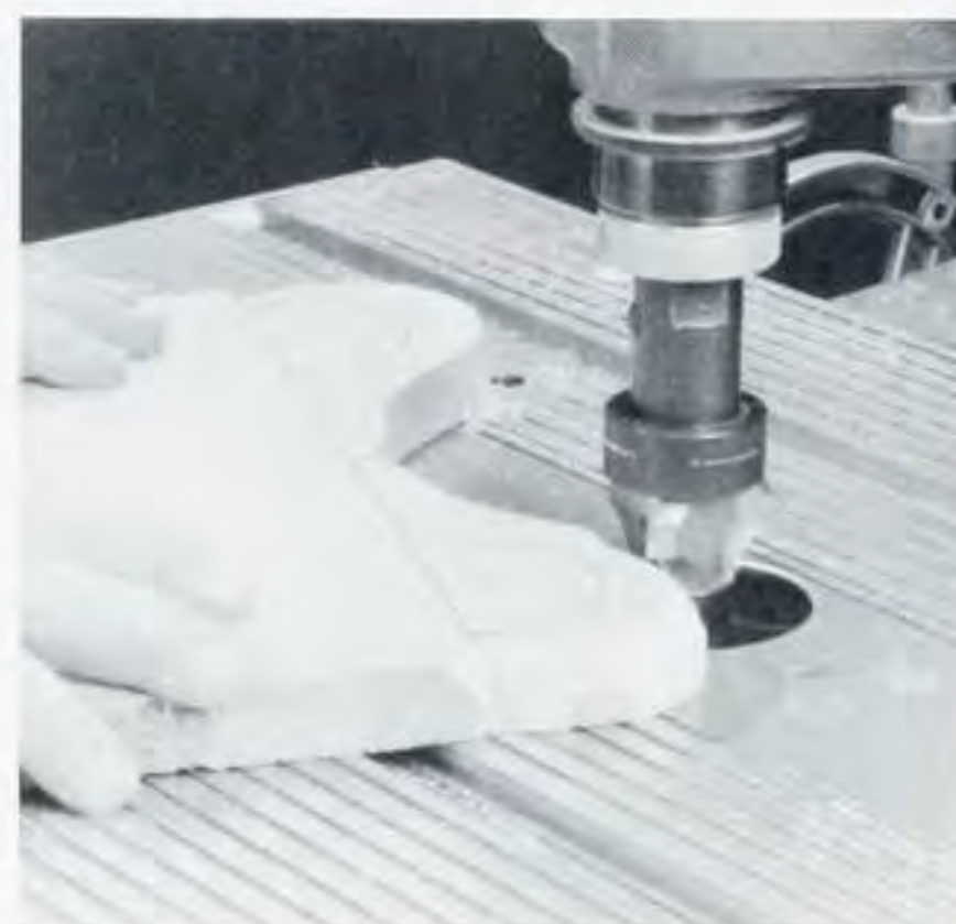
Figure 2. Round over the upper edge of the fender, then cut it free from the stock.
