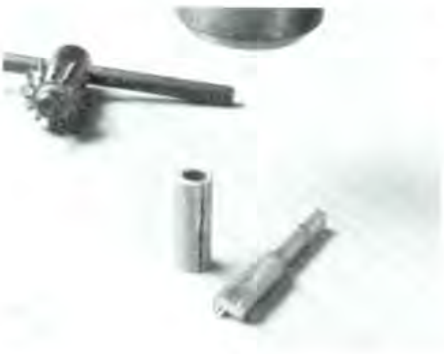
Figure 10. To rout safely on a drill press, make a collet from a \frac{1}{4} " I.D. bushing. With a hacksaw, cut a slot down the length of the bushing.
