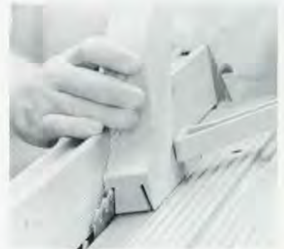
Figure 1. Cut the faces of the dovetail tenons with your table saw. Tilt the blade (or the table) at 10°.
