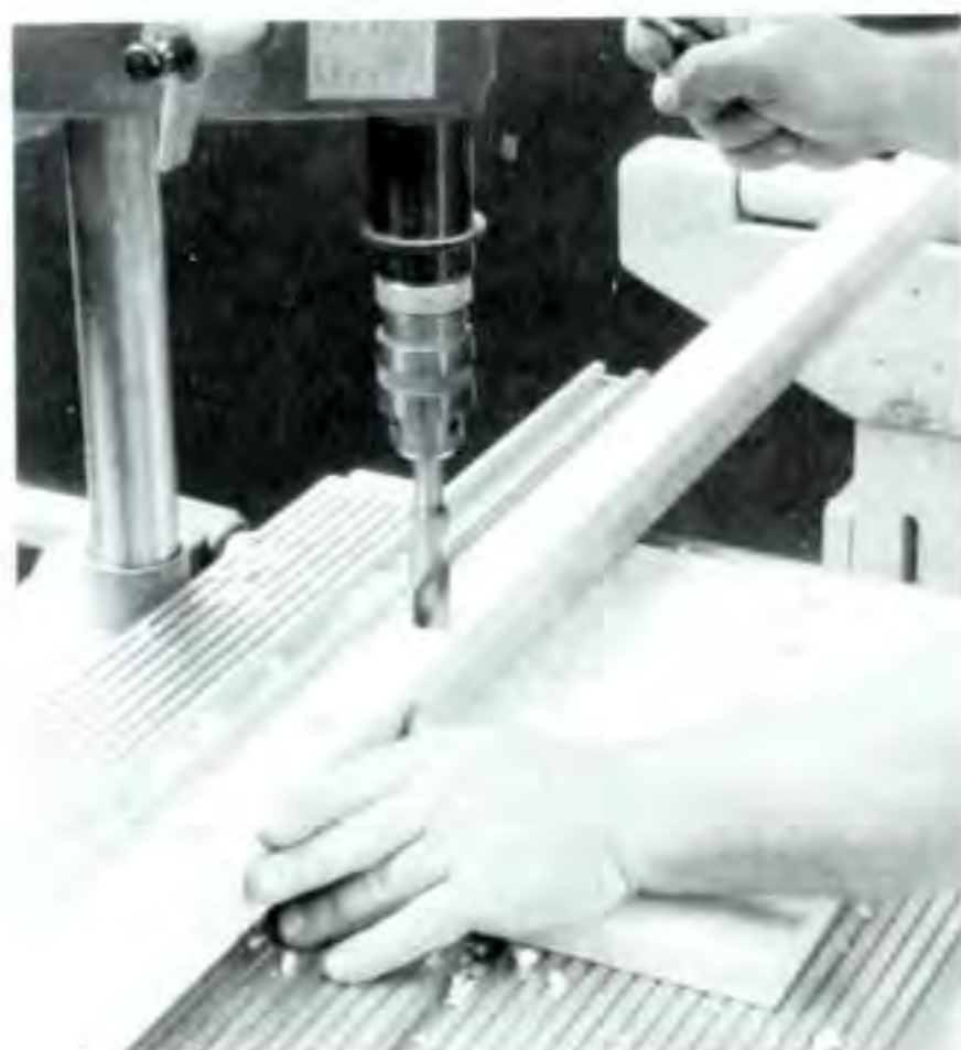
Figure 1. Stack up the uprights so that you can pad drill the holes for the dowels.
