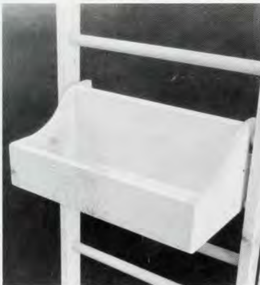
Figure 7. Certain parts of the hooks, shelving supports, and bin holders must be reinforced with finishing nails. To keep the thin wood from splitting, use a hand drill to spin the nails most of the way into the stock...
