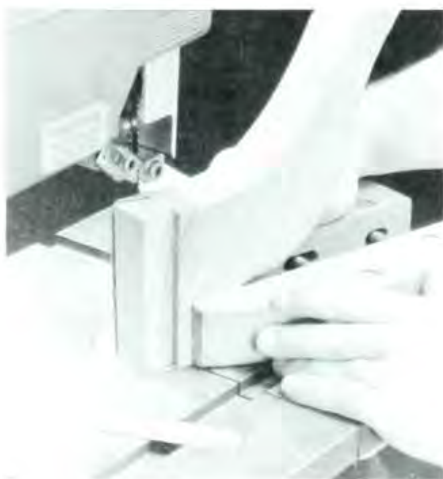
Figure 2. Remove the waste from either side of the tenons with a bandsaw. Clamp the legs in wood screws to hold them upright.
