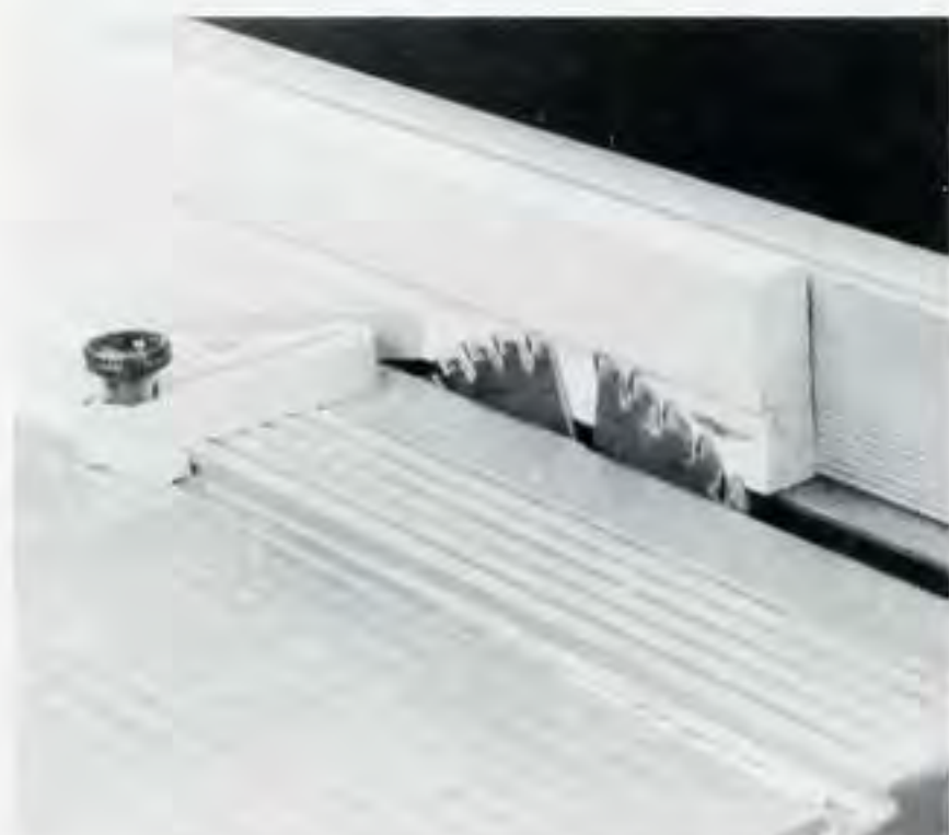
Figure 3. Cut the molding shape in a wide board, then rip the molding from the board.
