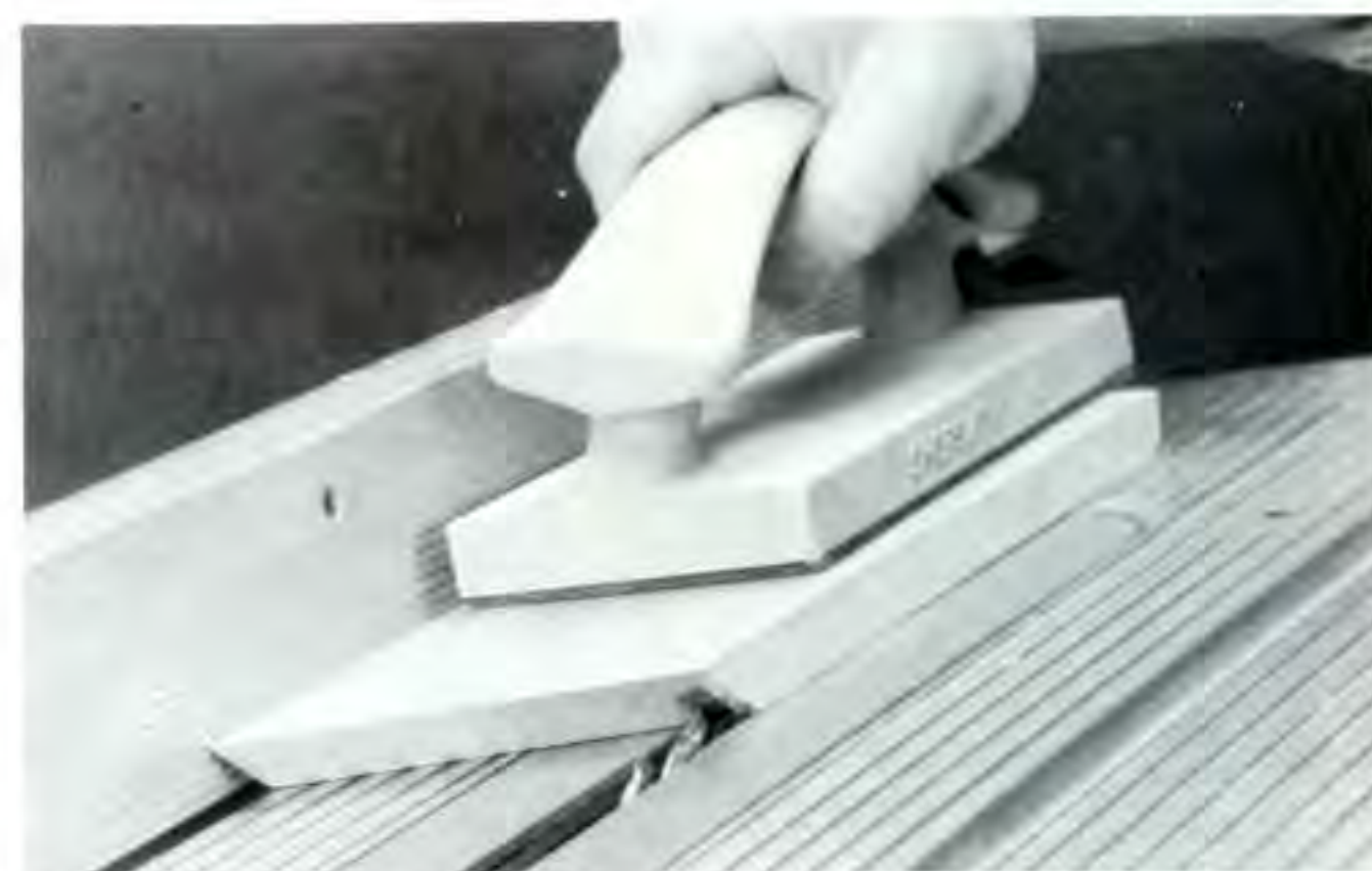
Figure 2. Cut the groove for the bottom at a 15^\circ angle.
