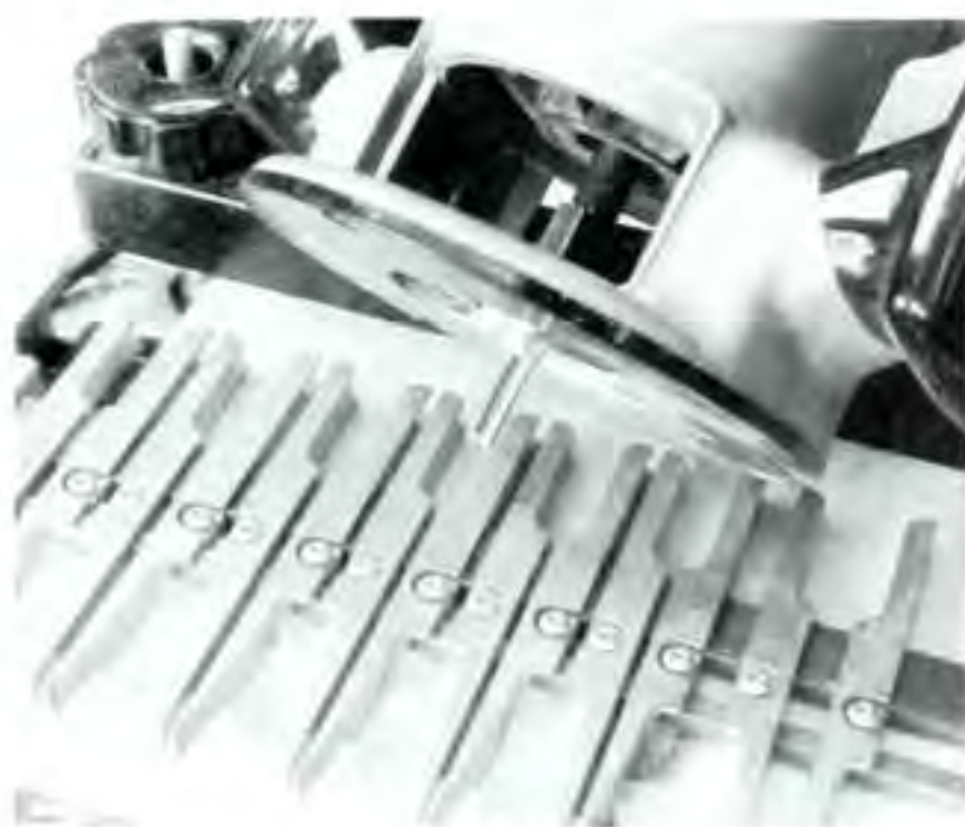
Figure 6. Cut the pins with the straight bit and the other portion of the jig.
