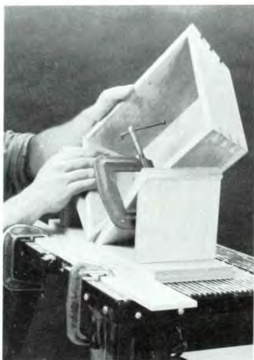
Figure 5. Cut the dovetail slots in the corners of the assembly with a special jig. You can build this jig from scraps of plywood.
