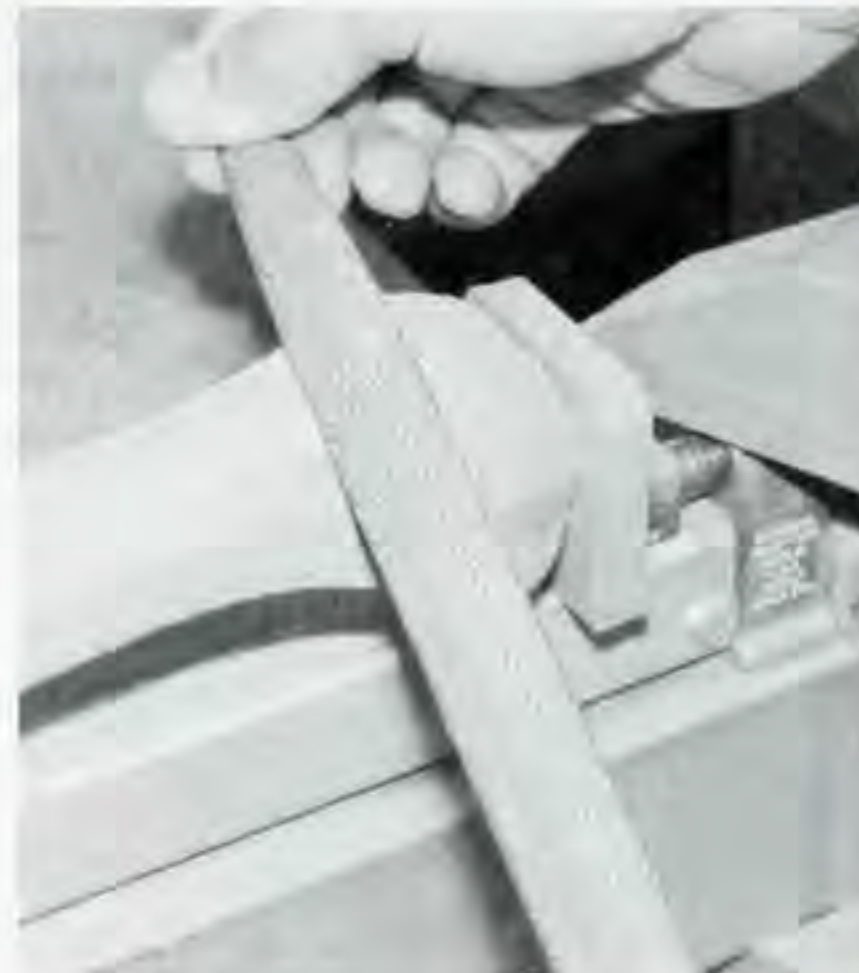
Figure 10. After sculpting the cabriole shape with the router, remove the millmarks with files and rasps.
