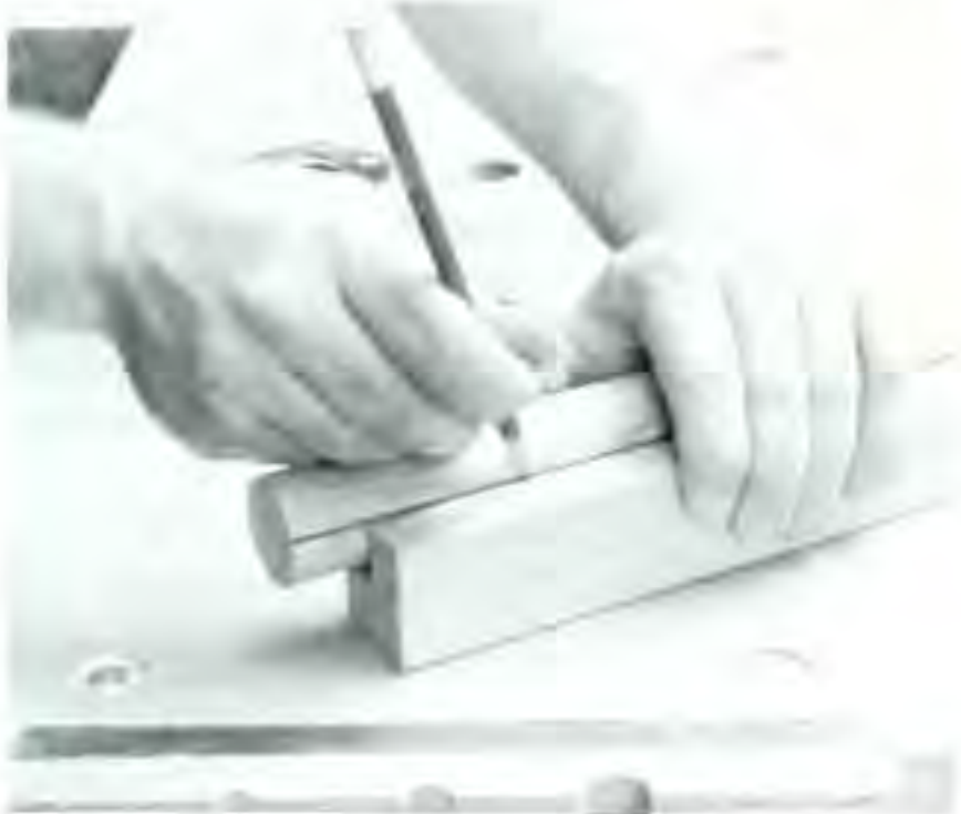
Figure 8. Use a V-jig as a straight-edge to mark the "lines" of mortise holes on the legs.
