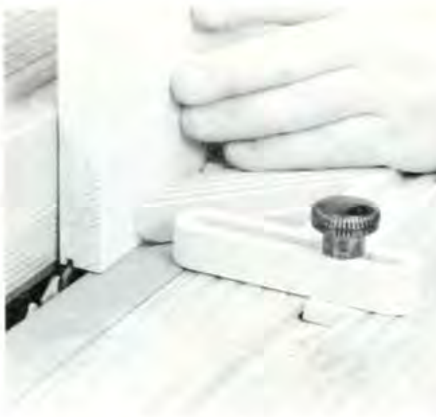
Figure 4. To make the extension ladder uprights, first cut a kerf in the edge of the stock.
