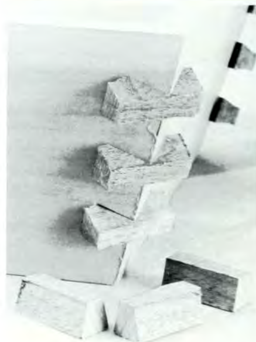
Figure 7. Glue the keys in the slots, cut off the excess wood, and sand them flush with the surface of the carry-all.
