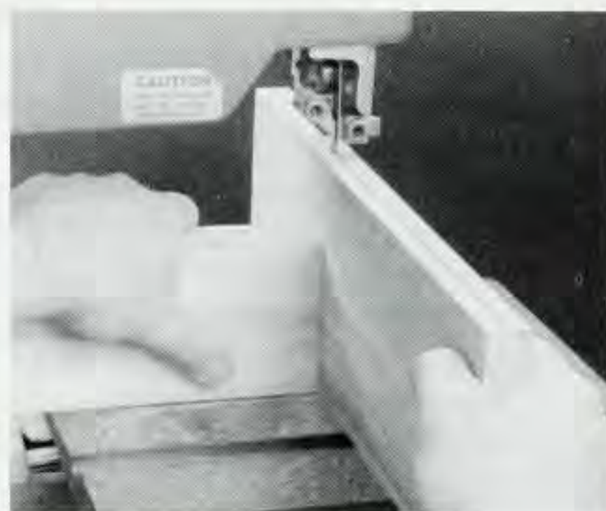
Figure 5. When resawing free-hand, use a large scrap of wood as a guide block. One end of this scrap must be cut off at 90°. This helps to keep the wood square to the table.
