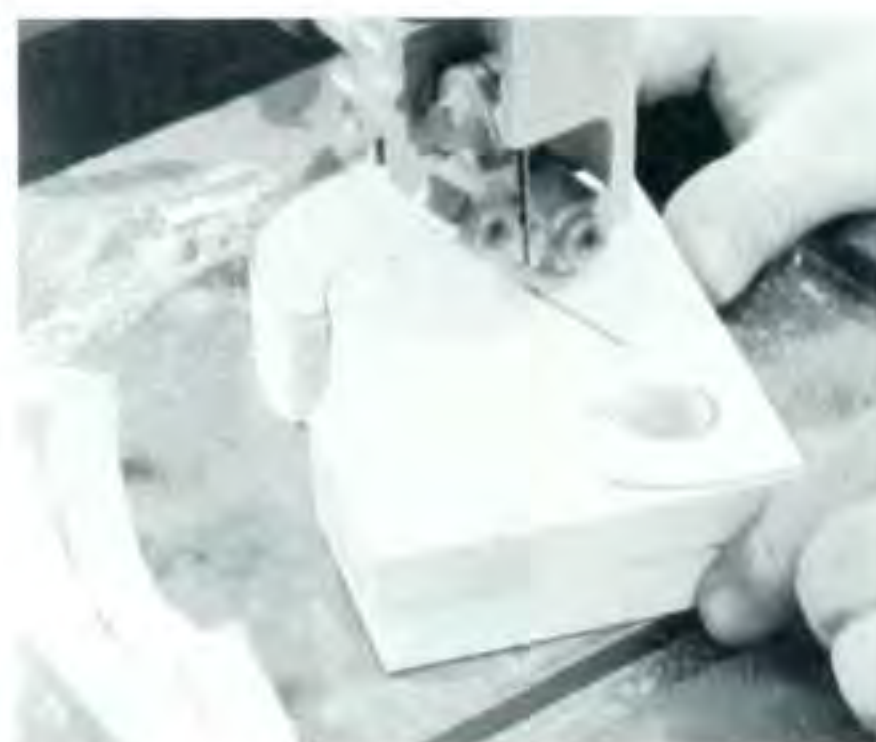
Figure 9. You can make several hooks, shelving supports, or bin holders by pad sawing the shapes on a bandsaw.
