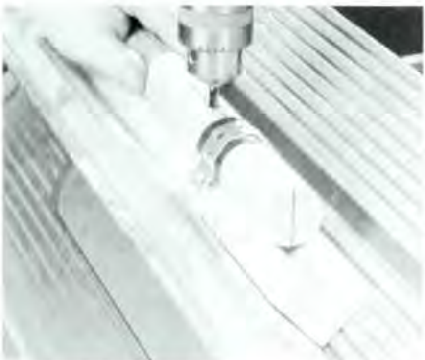
Figure 9. Secure the legs in the V-jig to cut or drill the mortises. Use scraps of leather to prevent the metal straps from marking the wood.
