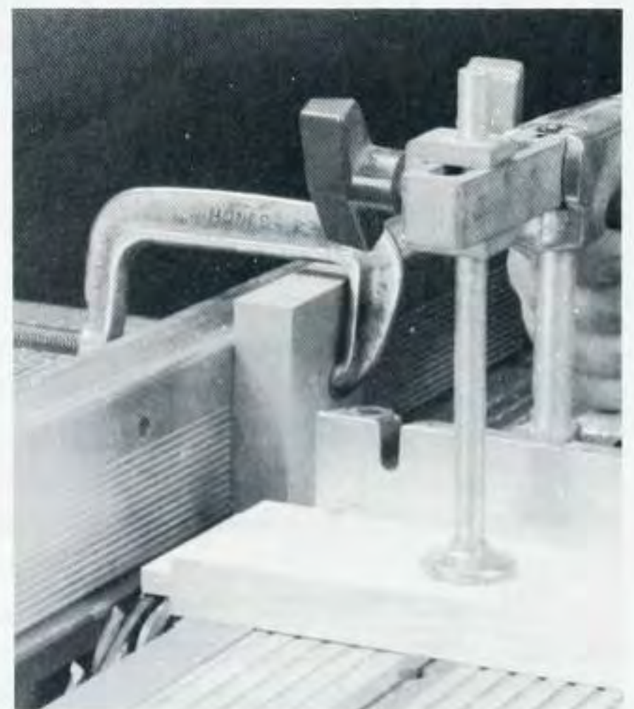
Figure 2. Make matching tongues, \frac{1}{4} " wide and \frac{3}{8} " long, in the ends of the web frame stiles.
