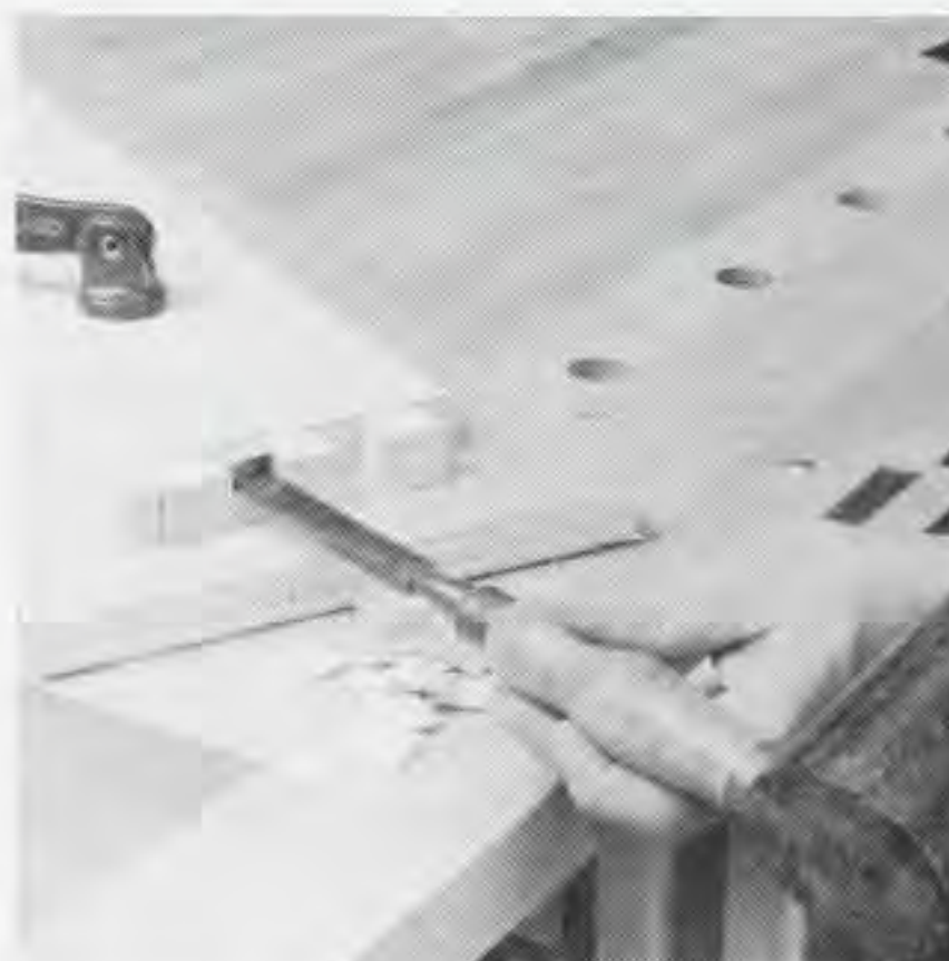
Figure 3. If the waste won't split off when you pry out, you may have to split it off from the edge of the board.
