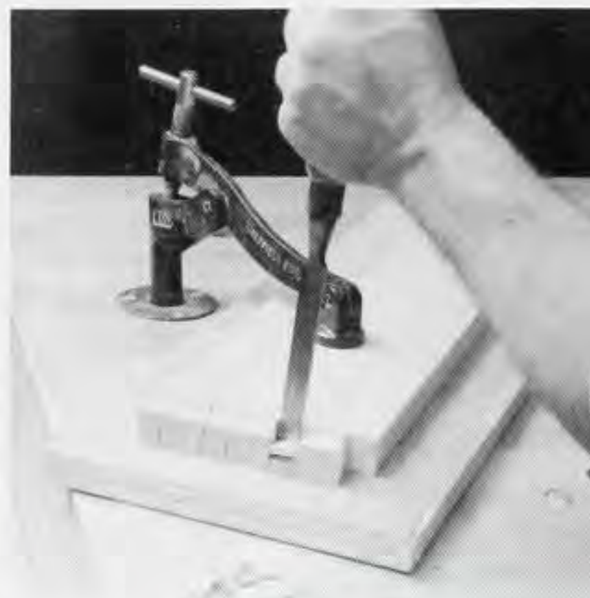
Figure 2. Remove the waste with a sharp bench chisel. Cut down about \frac{1}{16} ", then pry off a sliver of waste. Cut half the waste from between the tails, then turn the board over and do the other half.
