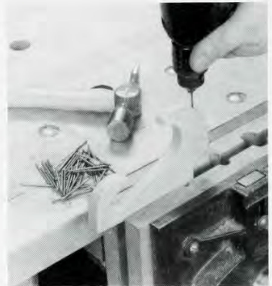
Figure 7. Certain parts of the hooks, shelving supports, and bin holders must be reinforced with finishing nails. To keep the thin wood from splitting, use a hand drill to spin the nails most of the way into the stock...
