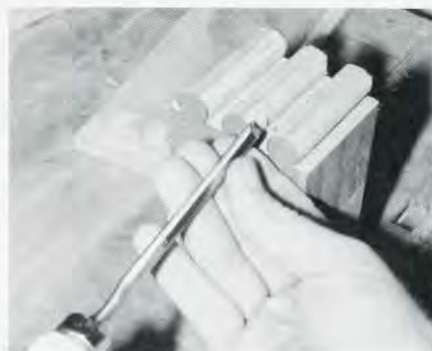
Figure 15. After you saw them to their rough shapes, use a chisel to shave all the beaver tails, fitting them to the sockets.
