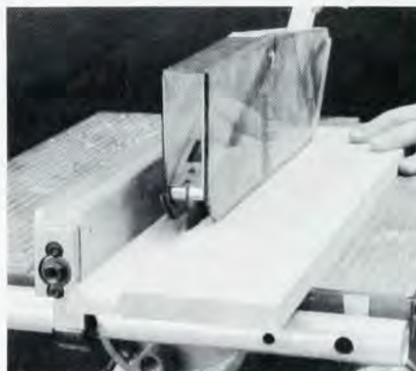
Figure 3. Cut the molding shape in a wide board, then rip the molding from the board.
