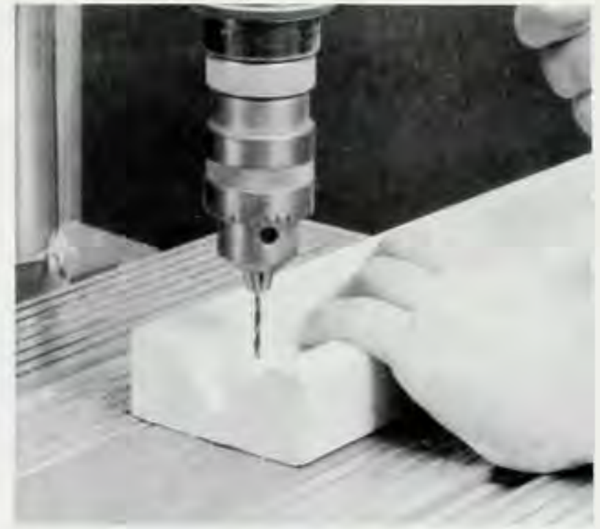
Figure 1. Use a long V-block to drill the holes in the wooden bead and the maypole.
