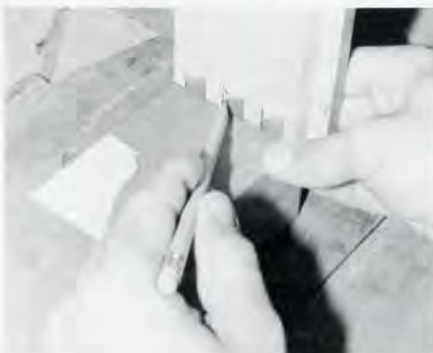
Figure 16. In the center of each beaver tail, drill a 1/4"-diameter hole for a dowel pin.
