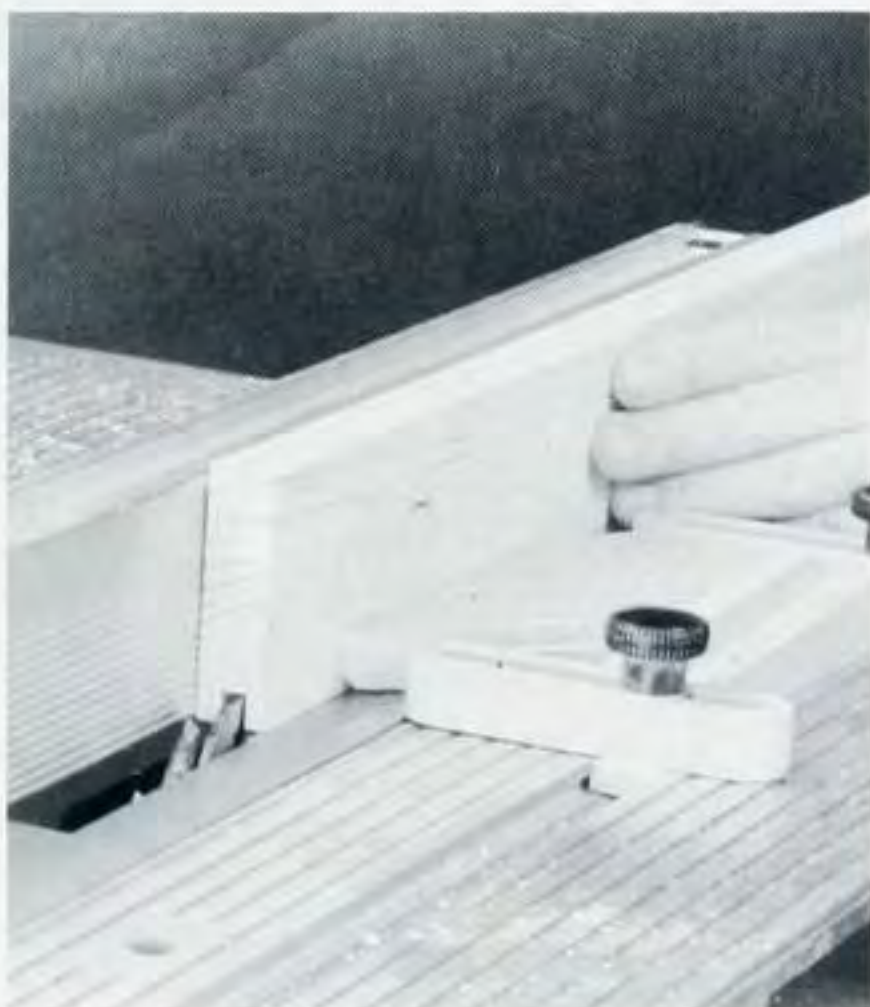
Figure 2. Make matching tongues, \frac{1}{4} " wide and \frac{3}{8} " long, in the ends of the web frame stiles.
