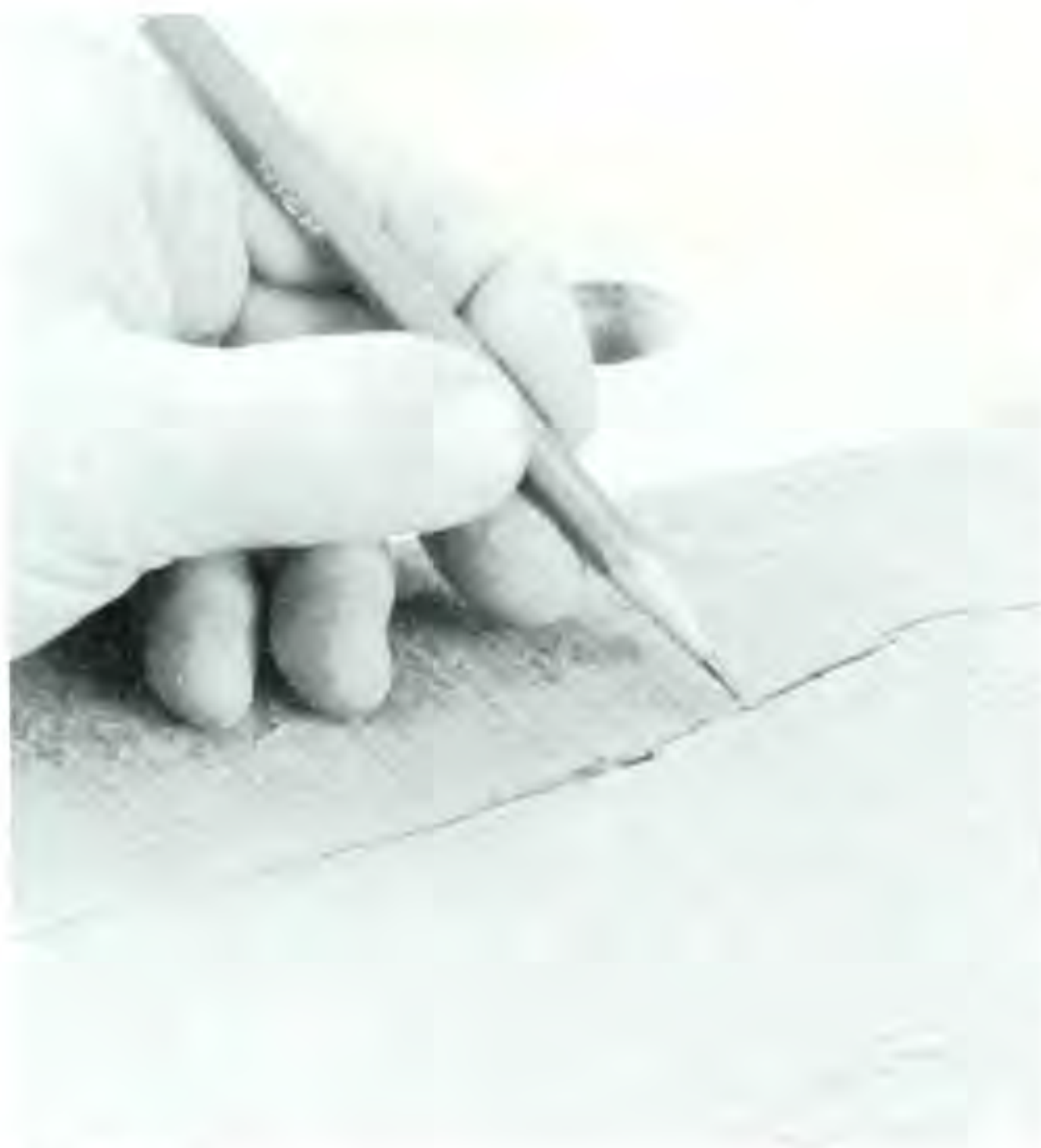
Figure 1. If the moisture is removed from a board too quickly, it will form surface checks. This is sometimes called 'case hardening'.
