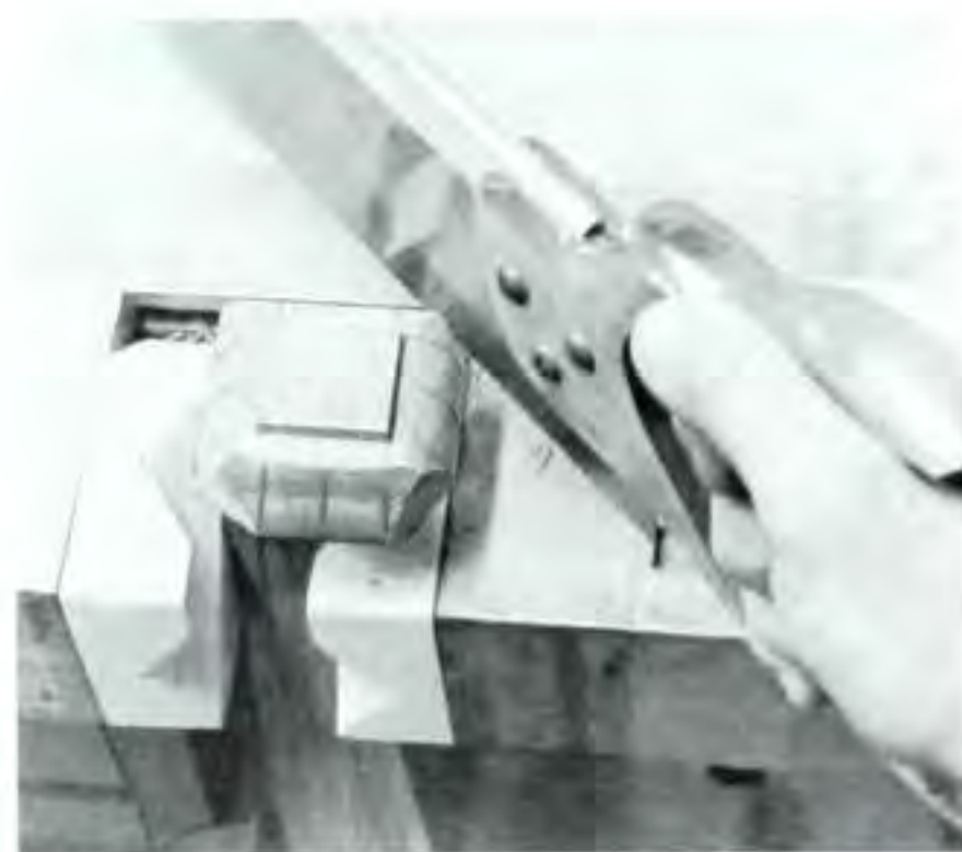
Figure 8. Using a back saw, cut off the three outside corners of the foot.
