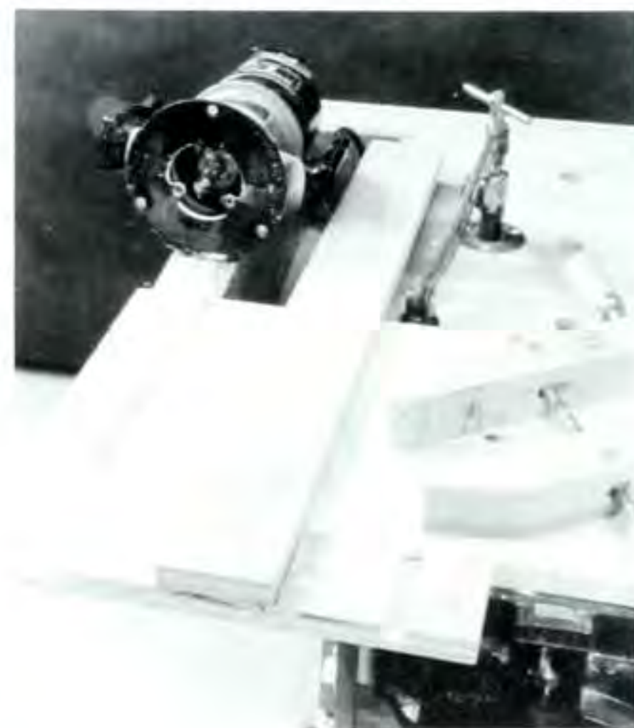
Figure 1. A large T-square makes a great routing guide for making dados and other simple joints.
