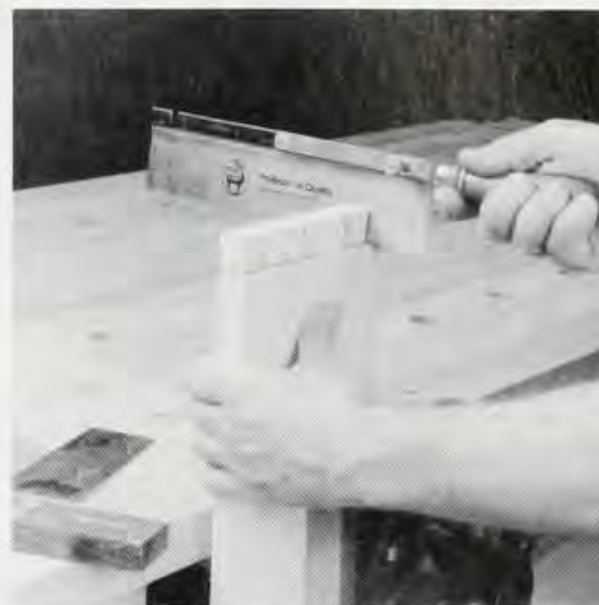
Figure 1. Cut the tails with a dovetail saw. If you want, use a square to help start the saw.
