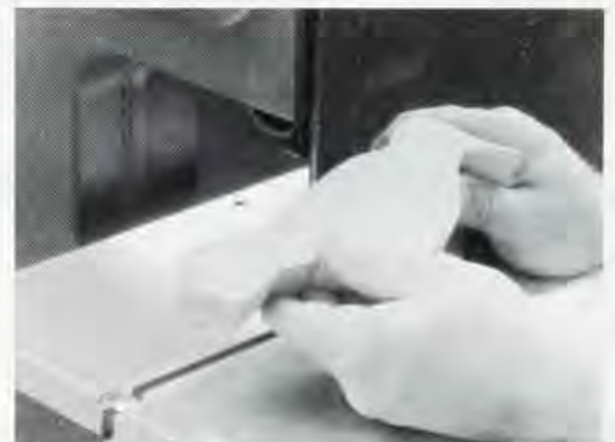
Figure 1. A strip sander makes short work of removing the saw marks from the sawn bird silhouettes.
