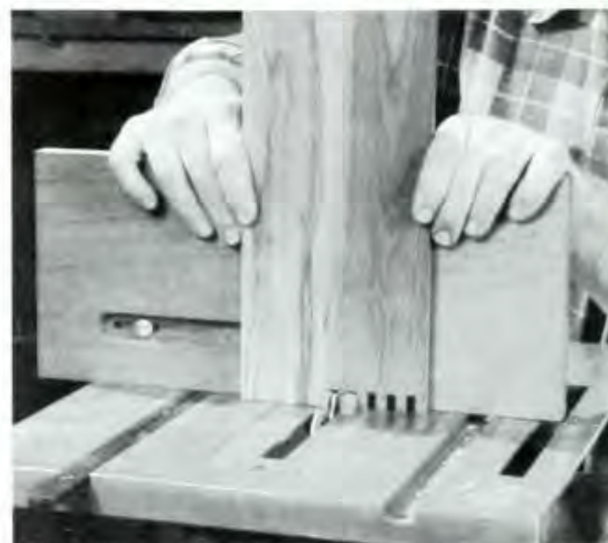
Figure 2. Cut the fingers with a finger joint jig attached to the miter gauge of your table saw.
