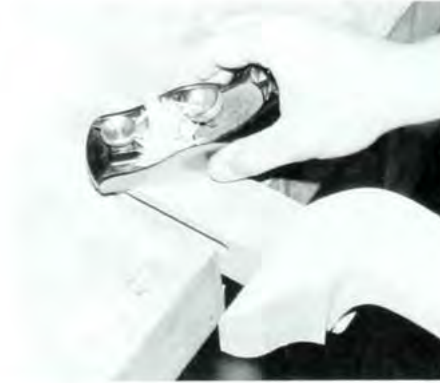
Figure 12. Smooth the leg post with a block plane.
