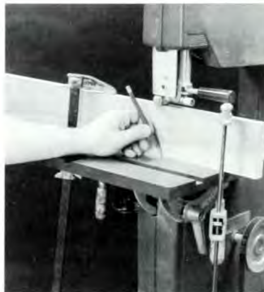
Figure 9. Use the scrap to draw a pencil line on the bandsaw table. Position your shop-made fence parallel to this line. This will help to compensate for the drift while you're resawing.
