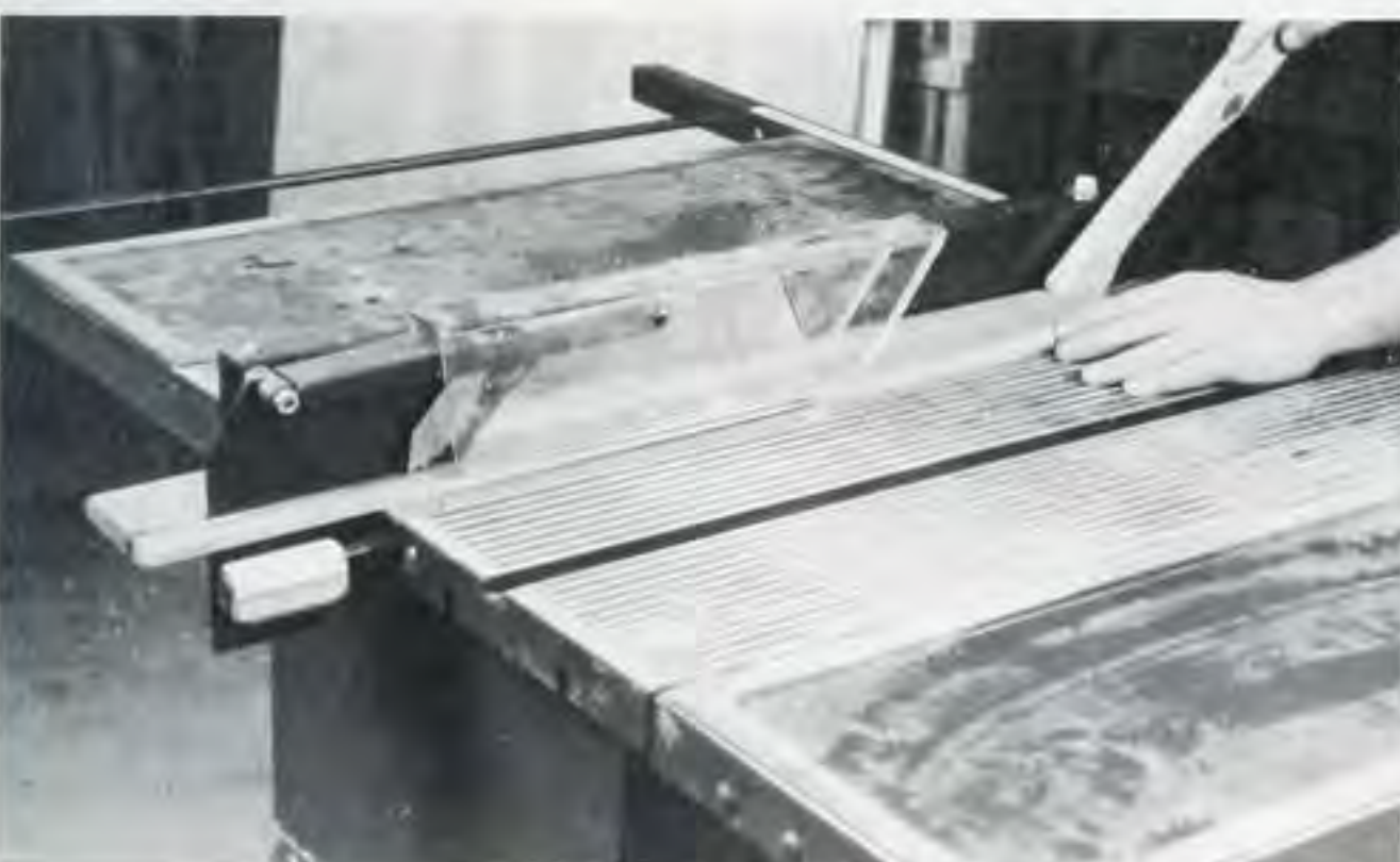
Figure 7. Cut the shape of the cove and the bead moldings in a large board, then rip the moldings free of the stock.
