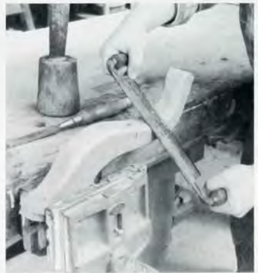
Figure 5. Shape the legs with a drawknife or a spokeshave, tapering them at the ankle so that the foot appears bulbous.
