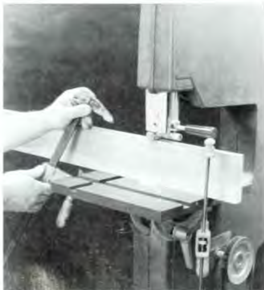
Figure 8. Before you can resaw with a fence, you must first find the "drift" of your blade. Scribe a straight line down the middle of a long scrap, and saw the line. As you cut, adjust the feed angle until the blade tracks the cutline accurately. Stop cutting and clamp the scrap to the table.
