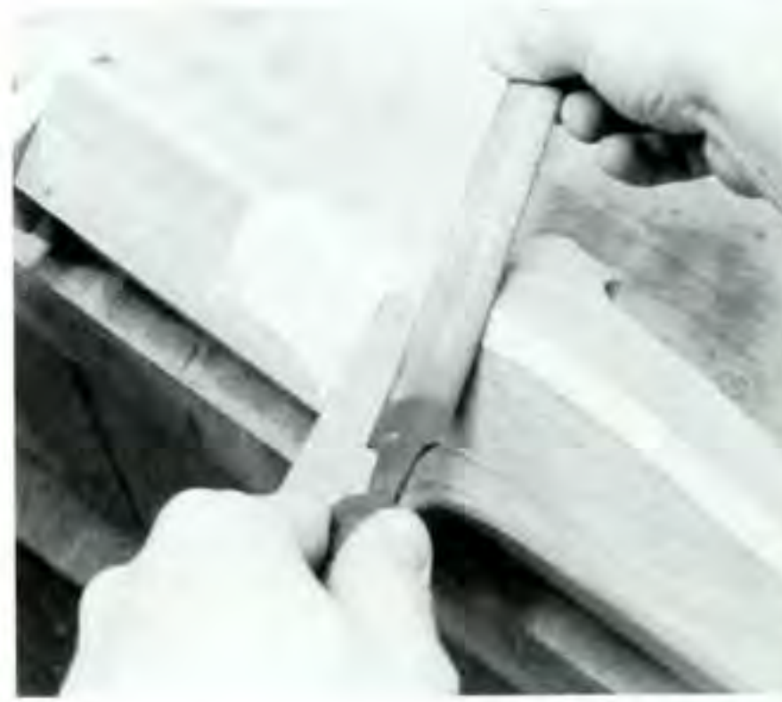
Figure 10. Chamfer the corners of the stock between the lines.
