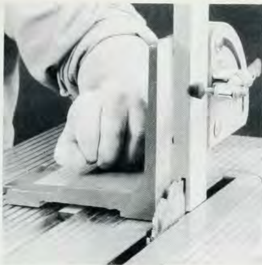
Figure 8. Cut the mortises and the tenons that hold the door frame together with a tenon cutting jig. The jig shown here is commercially-made, but you can easily make one from scrap wood.
