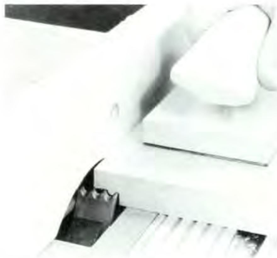
Figure 5. Use a molder to cut the bead in the left and right back panels.
