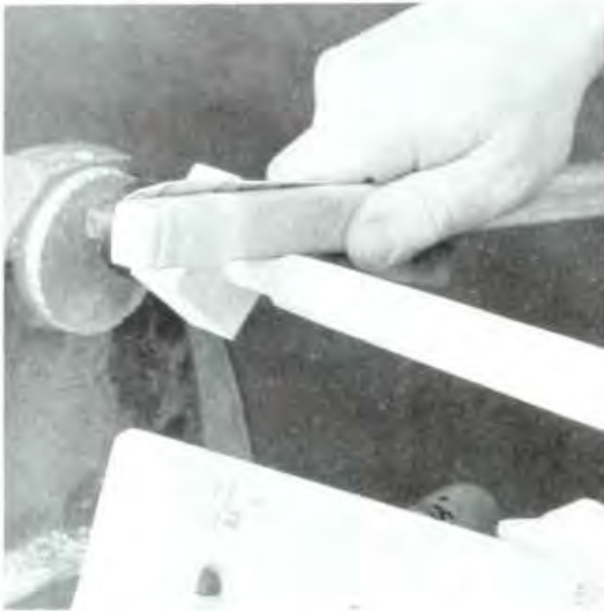
Figure 2. To remove stock slowly — so that you don't accidentally turn past the diameter — sand the tenon to the final dimension.
