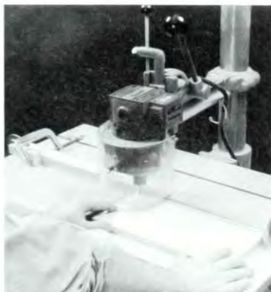
Figure 1. If you have one, use an overarm router to make the double-blind grooves. Two stops keep you from cutting through to the ends of the boards.
