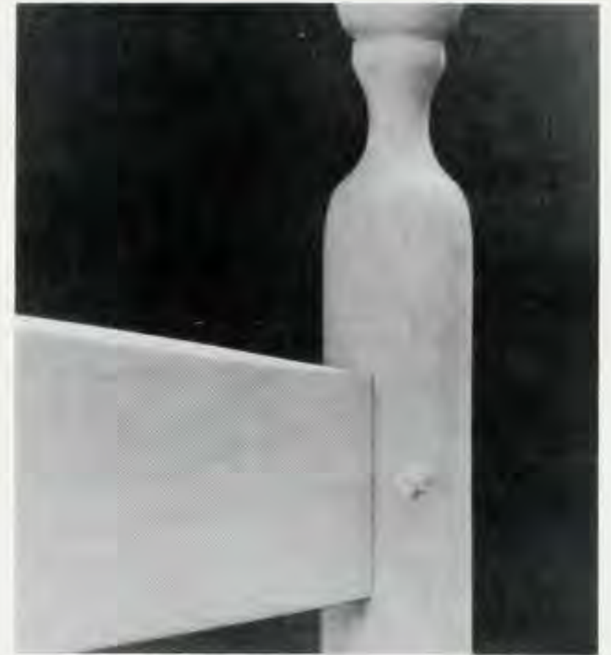
Figure 12. Peg the backrest in the mortises in the back legs. This will help hold the chair together even after the glue joints give way.
