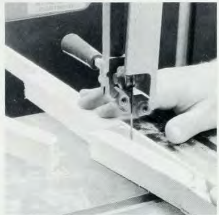
Figure 7. To make the bends in the top handle, thin out the stock with a bandsaw.
