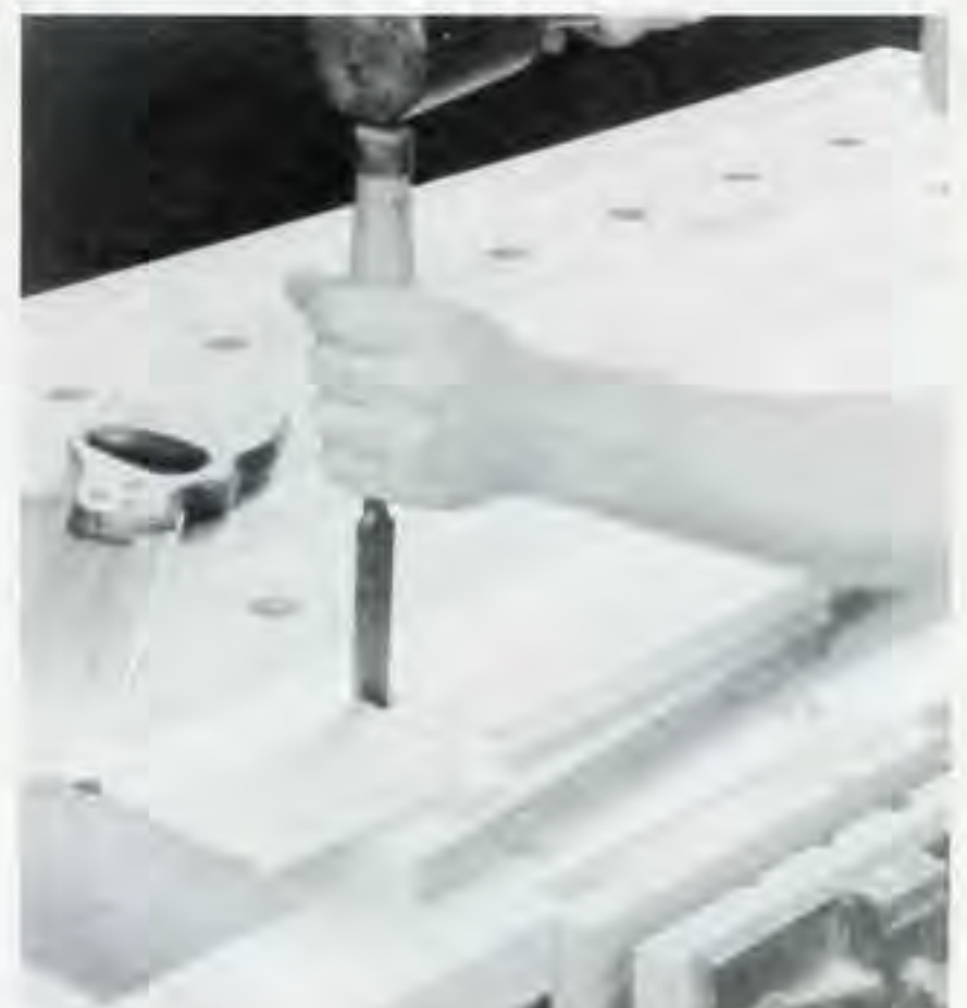
Figure 3. Then remove the waste with a bench chisel.
