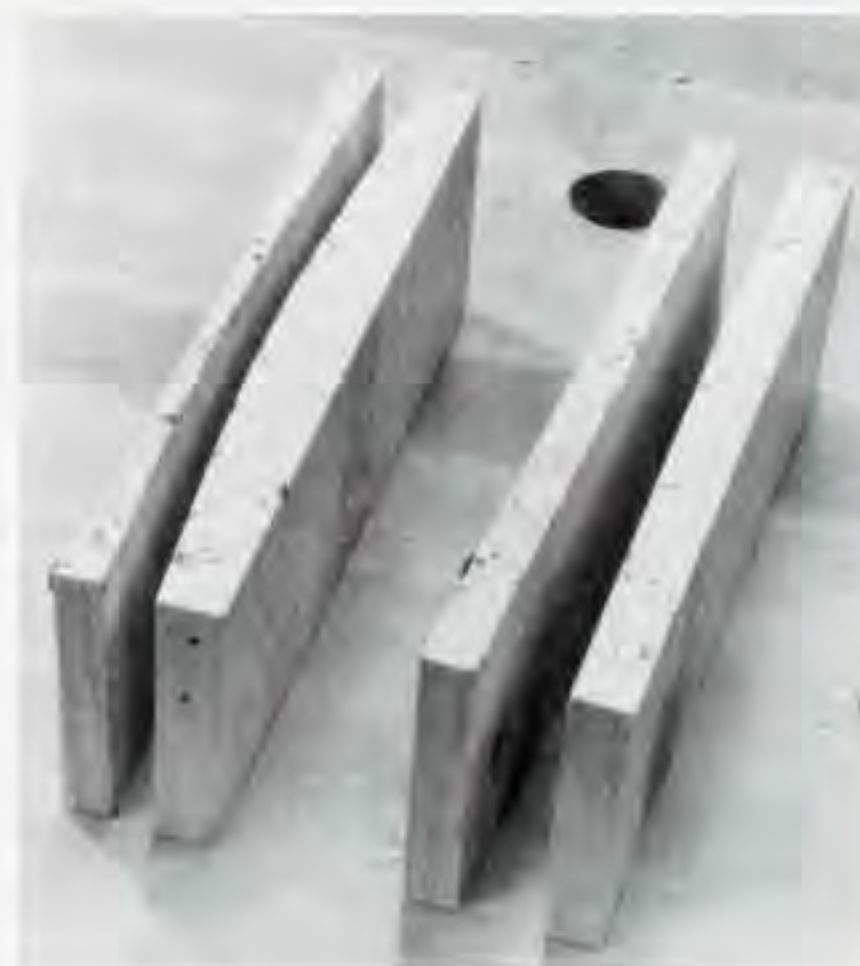
Figure 12. One of the most common resawing problems is “cupping” — the blade bows in the stock. Usually, this problem can be cured by increasing the blade tension. The piece of wormy chestnut on the left was cut with the tension too low. The piece on the right was cut after the tension had been readjusted.
