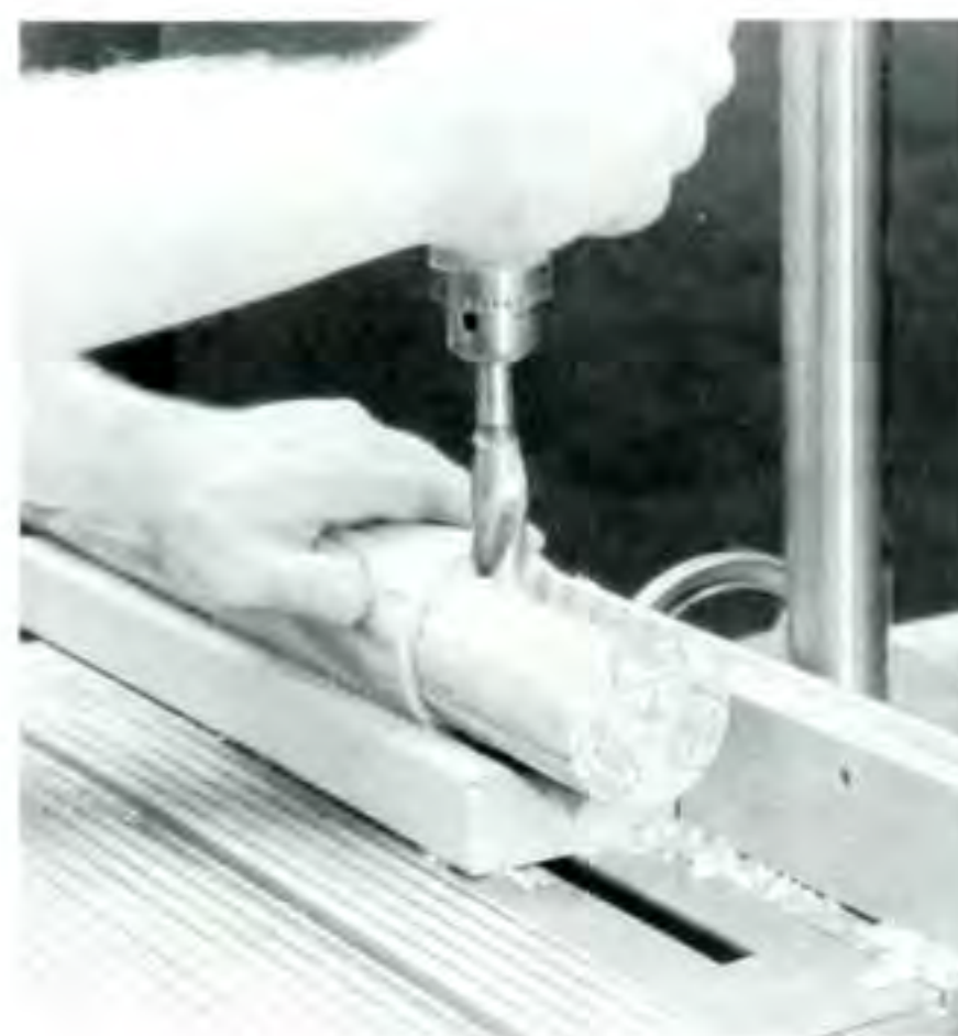
Figure 3. Drill a series of holes to remove as much waste as possible from the dovetail slots.
