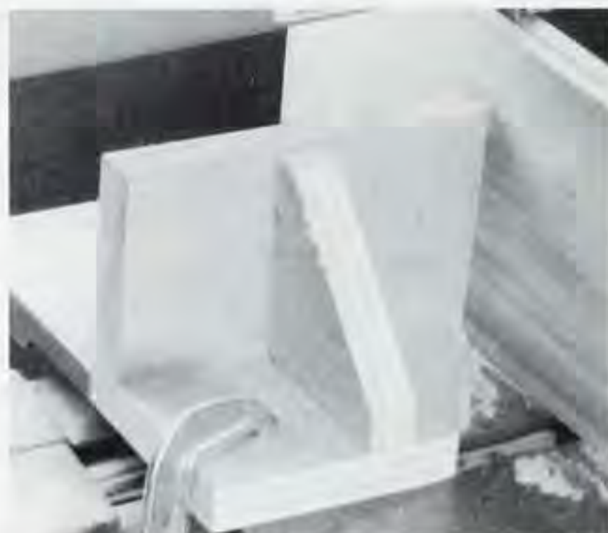
Figure 7. Clamp the pivot securely to the bandsaw table. The distance between the pivot and the blade determines the width of the cut. When you cut, keep the smooth (planed) face of the stock against the pivot.
