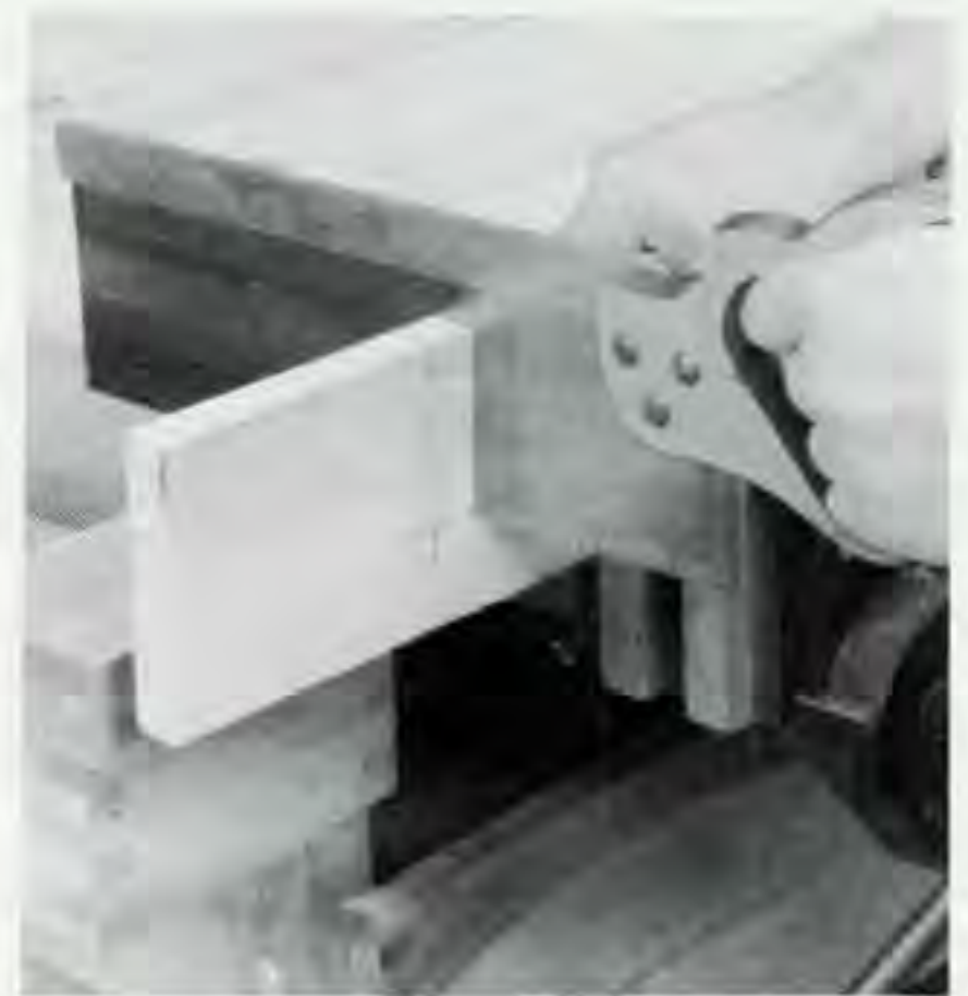
Figure 2. To make the notches in the canopy slats, first cut the sides of each notch with a handsaw.
