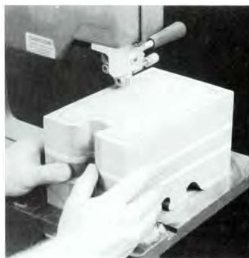
Figure 5. For the fourth and final cut, cut the waste from the inside of the box.
