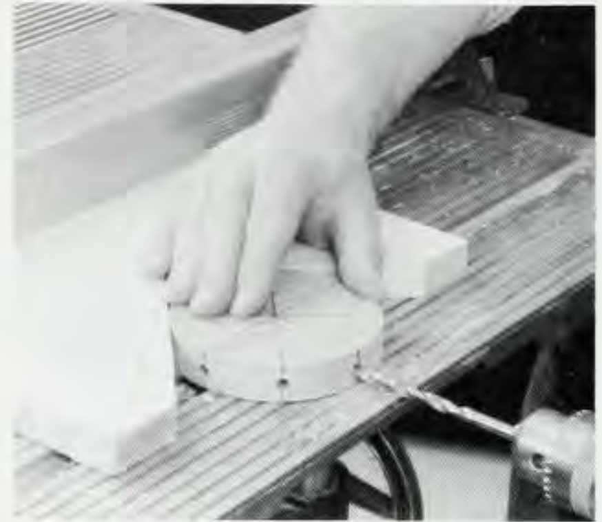
Figure 2. A "V" cut into a 3/4"-thick scrap of wood to make a flat V-jig helps to hold the hub while you drill holes in the edge.
