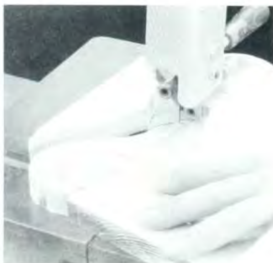
Figure 1. Cut the top edge of the fender shape in a long piece of stock. Don't cut the fender free until after you've shaped the edge.
