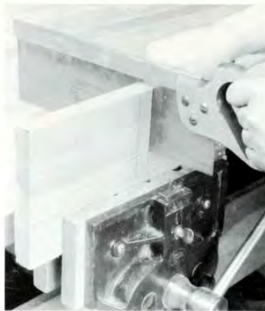
Figure 1. To make a cross lap joint, first saw the side of the joint.
