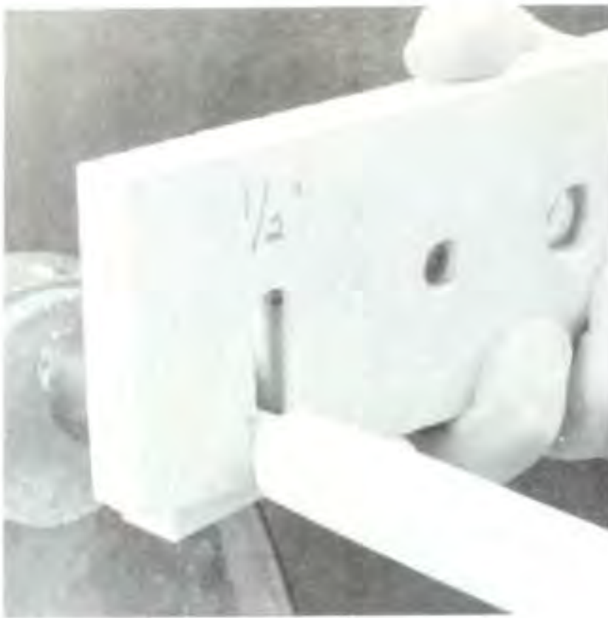
Figure 1. When the gauge slips over the tenon up to the jog or step, then you're nearing the final diameter.
