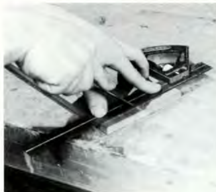
Figure 1. Lay out the finger joints on the inside surface, scoring the stock with an awl or marking knife. This will prevent tear-out.
