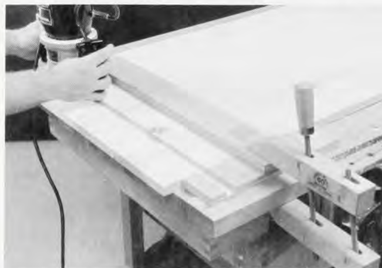
Figure 4. When you cut the dadoses, use a straightedge to guide the router.
