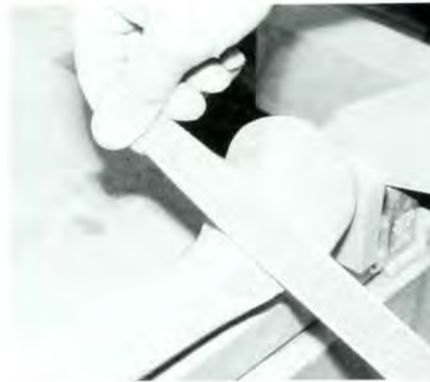
Figure 11. Feather the top of the foot to flatten it and blend the other surfaces of the leg with it.
