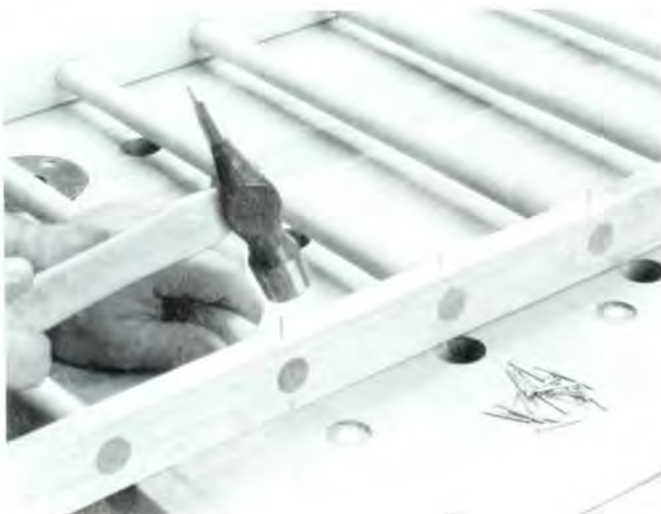
Figure 2. Pin the dowels in the uprights, driving brads through the edge of the uprights and into the ends of the dowels.
