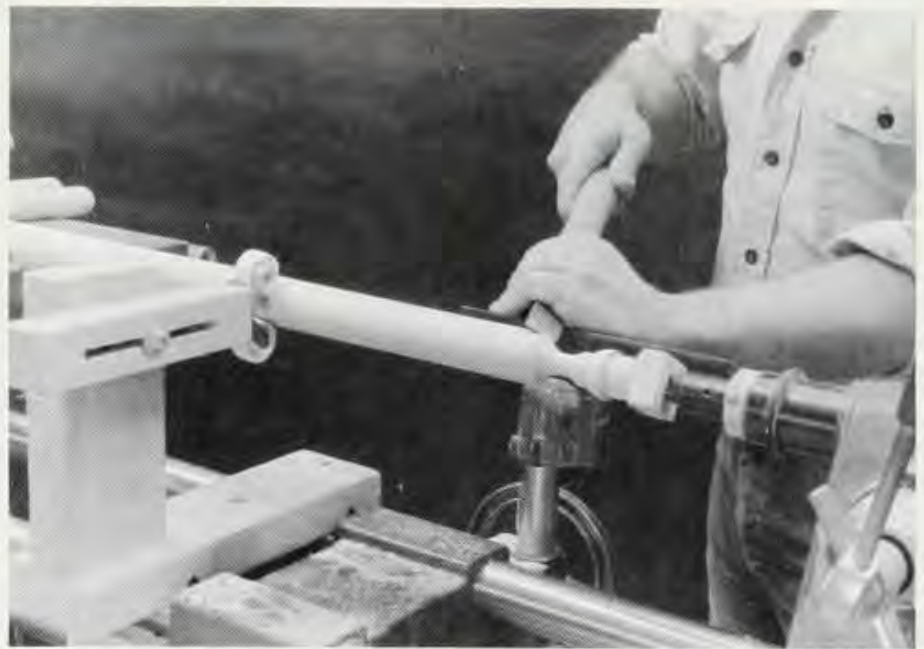
Figure 6. When turning the back legs, use a steady-rest to keep the long, slender turning from whipping on the lathe.
