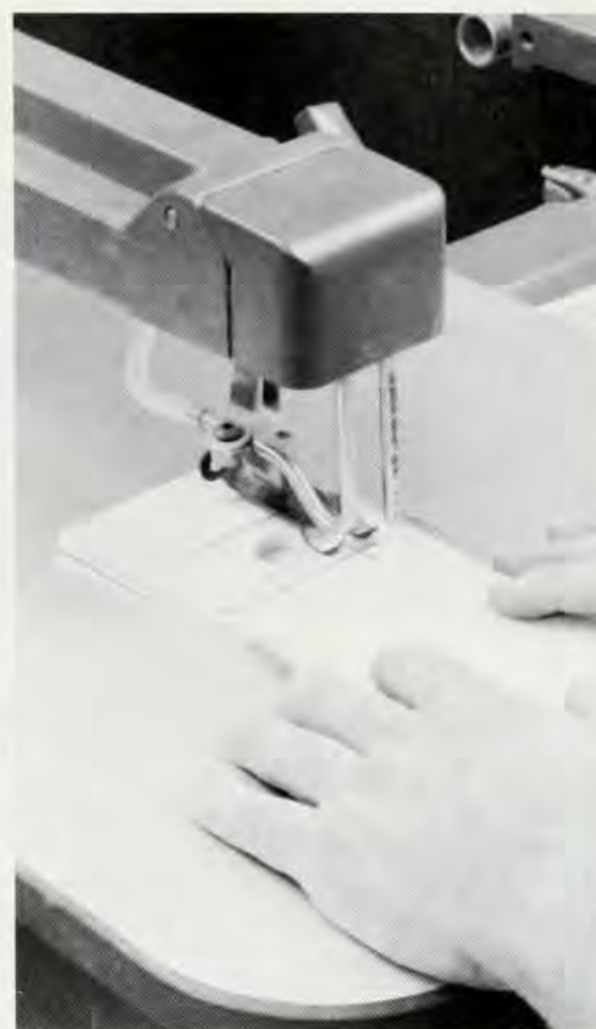
Figure 5. Make a piercing cut with a scroll saw to cut out the skylights in the roof halves.
