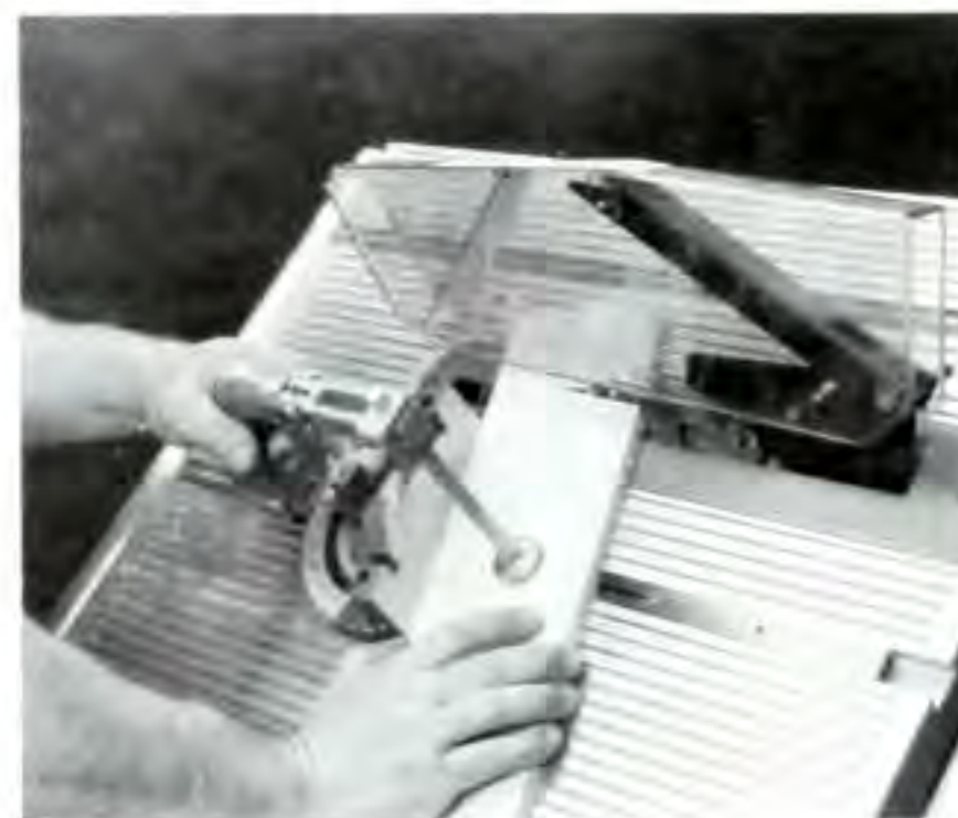
Figure 1. Join the sides and ends with a compound miter. Set the blade angle to 43\frac{1}{4}^\circ , and the miter gauge angle to 75\frac{1}{2}^\circ .
