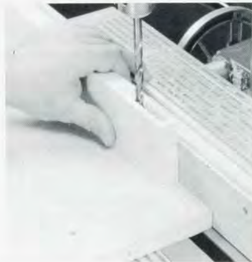
Figure 5. Make the mortises in the rails by drilling a series of holes, then cleaning up the edges with a chisel.
