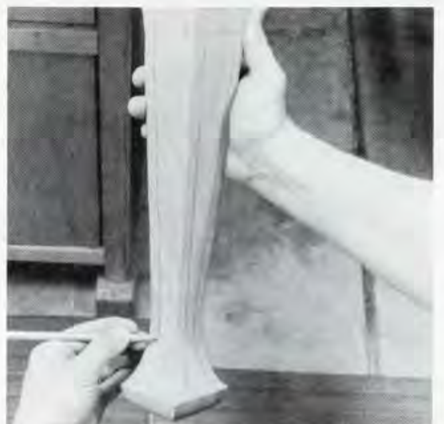
Figure 6. Divide the faces of the leg and foot into quarters, and mark the lines on the stock.
