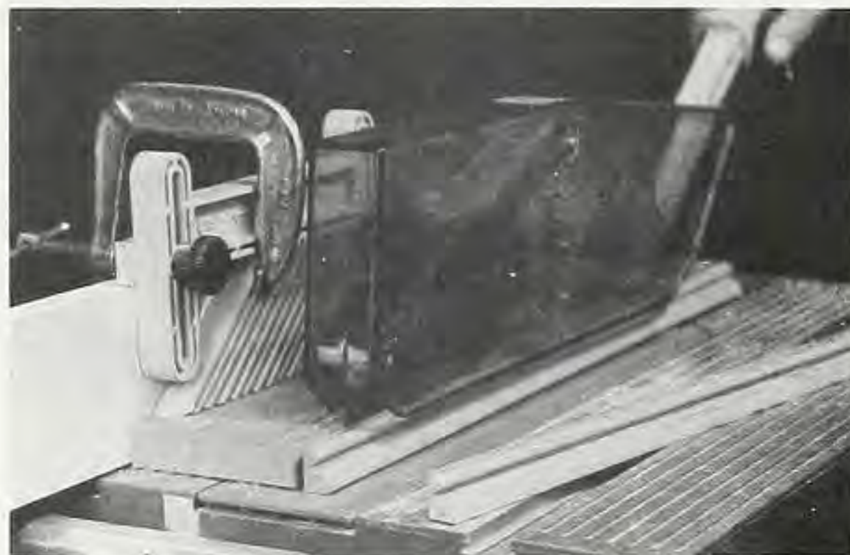
Figure 3. A wide extension fence, bolted to your rip fence, helps keep a board at the proper angle to the molding knives.
