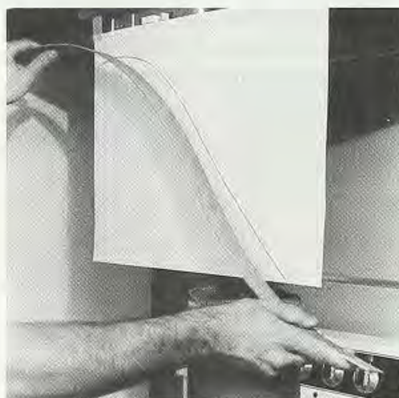
Figure 5. As you work, compare the wood you're bending to a full size drawing of the bend you want.
