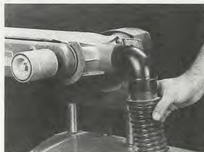
Figure 5. The rear housing on the belt sander has a port so that you can vacuum up the sawdust as you work.
