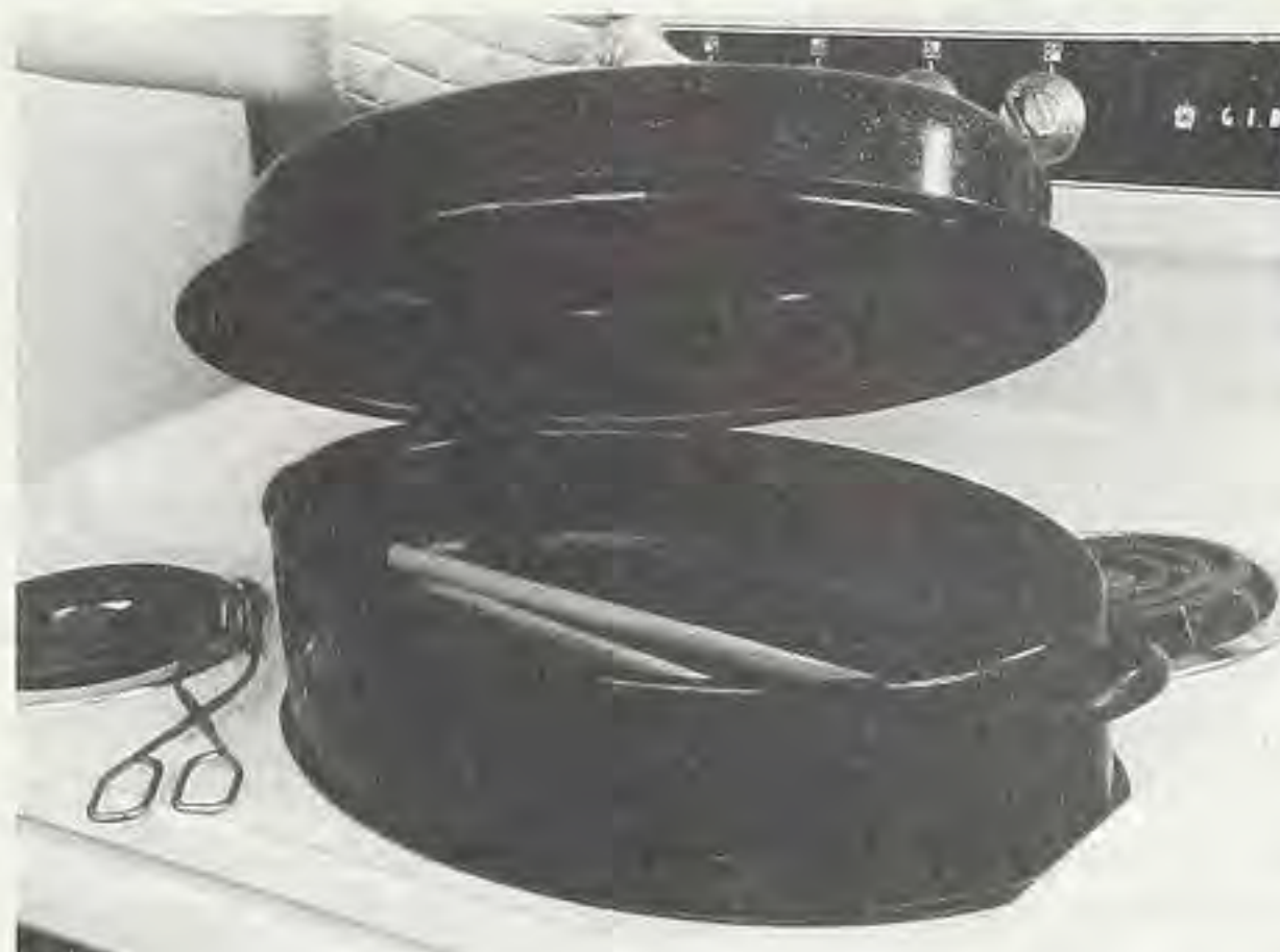
Figure 1. To heat the wood evenly, boil it. A roast pan makes a good boiler.
