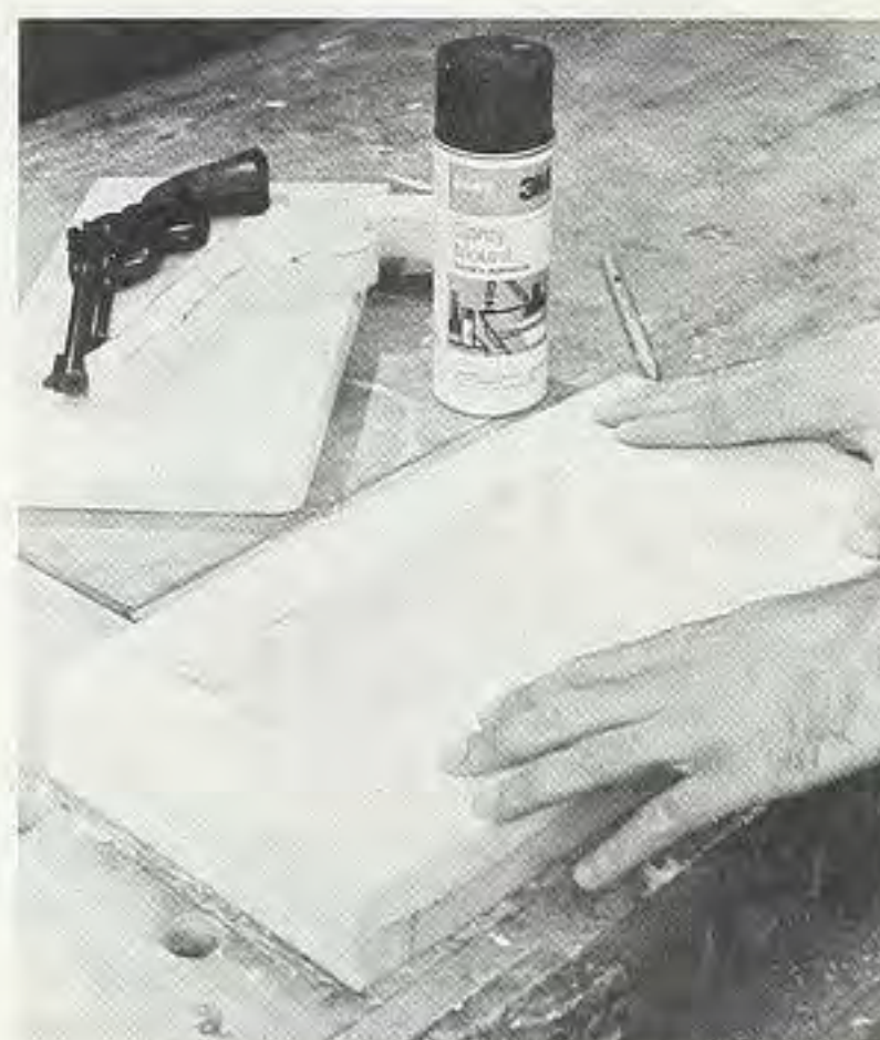
Figure 15. To make a foam cradle, trace the outline of the object you wish to display on a piece of foam. Cut out the outline, discarding the inside. Then glue the foam to a second, solid piece of foam.
