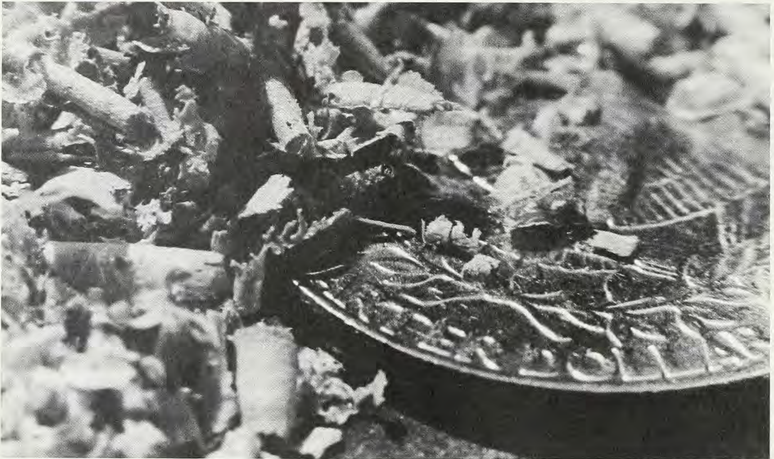
Jointer shavings magnified 25x.
