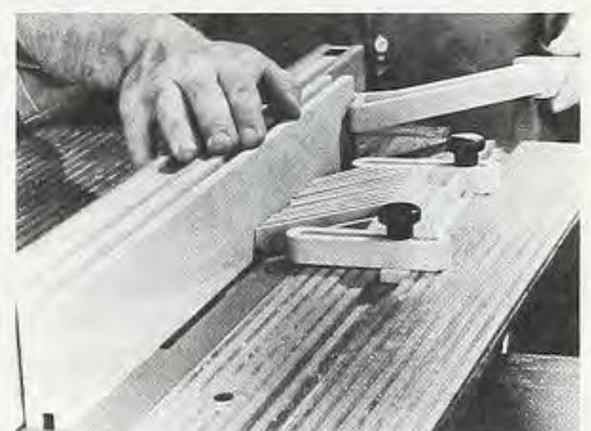
Figure 1. Cut the grooves on the insides of the web frame rails and stiles with a router or dado cutter. The middle stiles get grooves on both edges.
