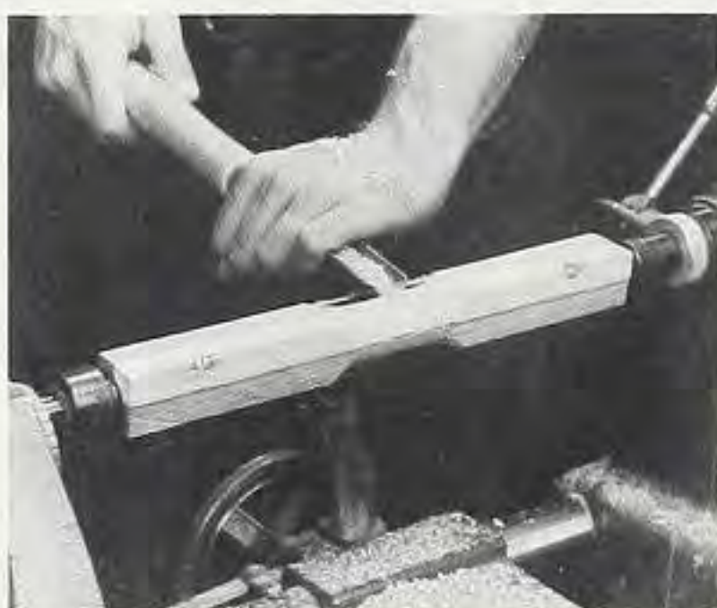
Figure 11. Turn the middle of the post first and wrap a piece of tape around it to help hold the strip in place.
