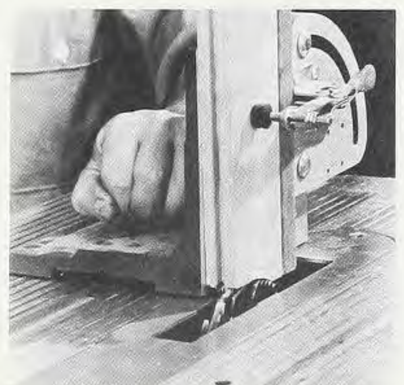
Figure 2. Use a tenoning jig to cut tenons in the ends of the web frame stiles.
