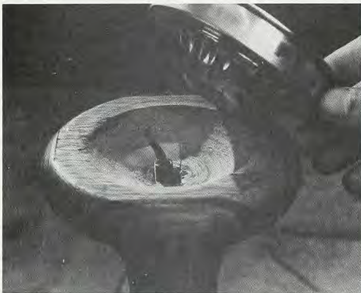
Figure 5. Some metal collars require that you turn a small bowl-shaped recess in the top cap, so that the collar will mount flush to the top of the turning.
