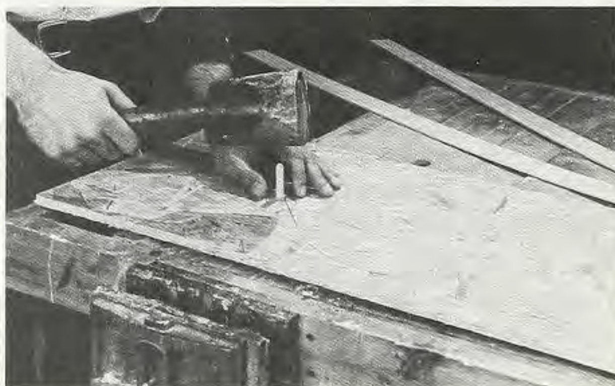
Figure 6. The first step in making a laminated bending is to make a bending jig. This can be nothing more than a few pegs in a sheet of plywood or particle board.
