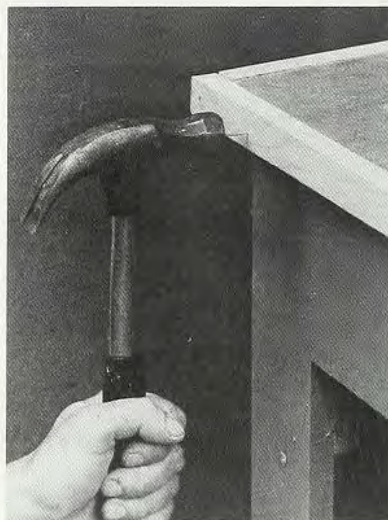
Figure 4. Trim the edges of the covered countertop with \frac{3}{4} " thick, 1" wide stock. This will hide the edges of the countertop and hardboard surface, giving the project a more 'finished' look.
