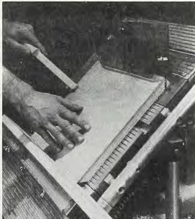
Figure 4. With the dado cutter, make a rabbet in the back edges of the tops, sides, and bottoms. These rabbets will hold the backs in place.
