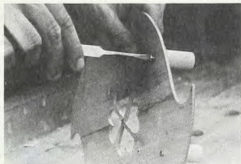
Figure 3. While you assemble the soundbox, hold the coupling posts in place on the top sounding board with small screws. Remove these screws after completing the soundbox.
