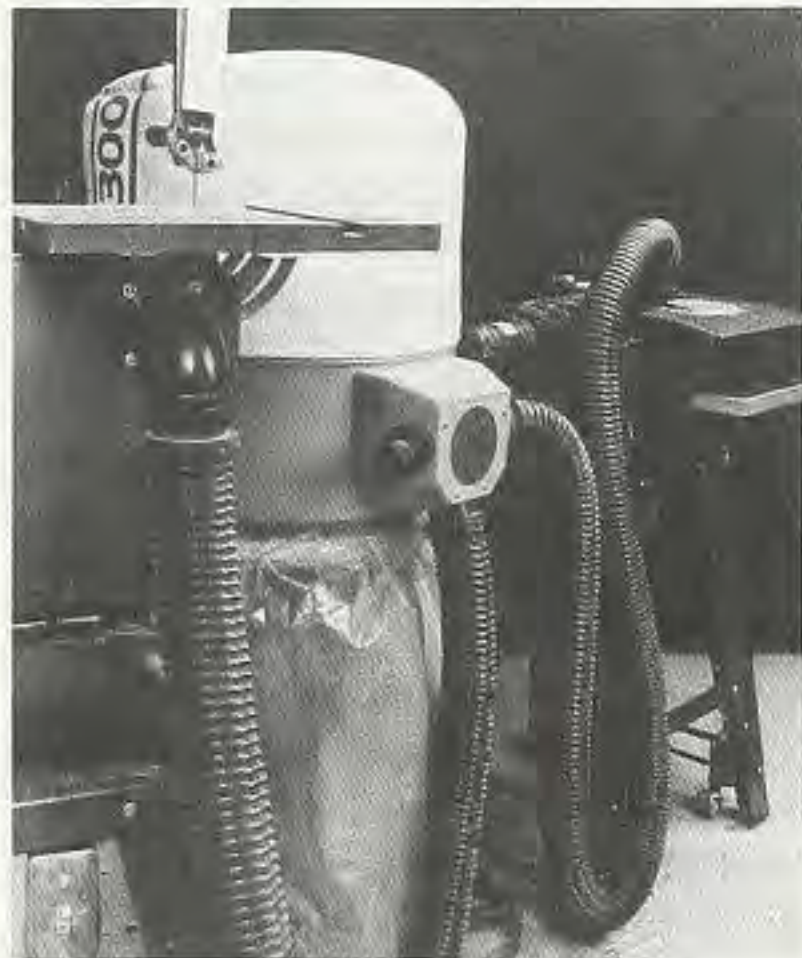
Figure 3. The new DC3300 will collect sawdust from up to three tools at a time.
