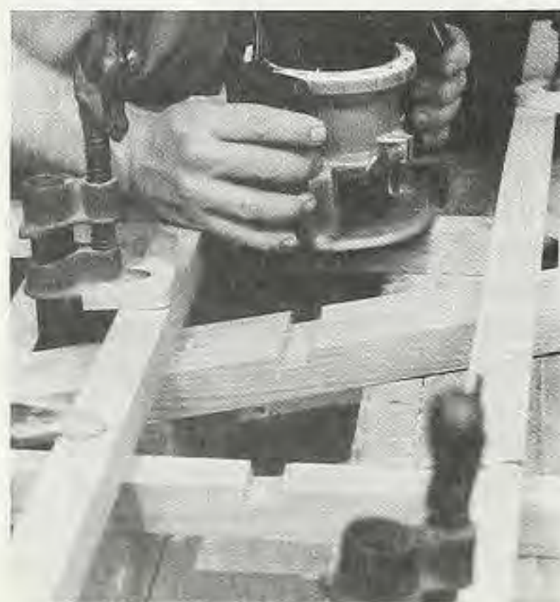
Figure 2. To rout the dadoes in the frames to hold the steps, clamp the side frames to your workbench. Use a straightedge to guide the router.
