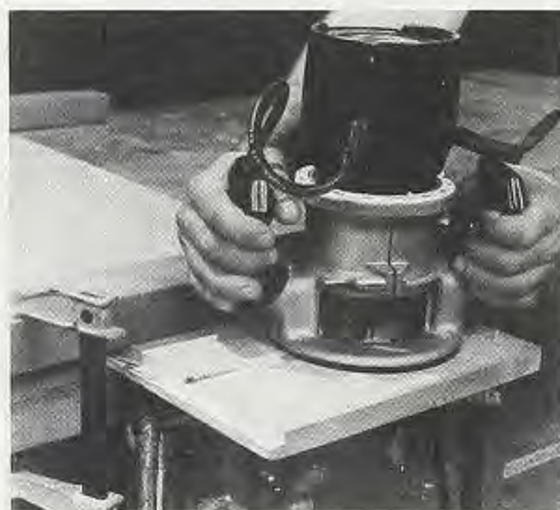
Figure 5. Raise the panels by cutting a rabbet in the edges of the panels, then cut a cove in the shoulder of the rabbet with a core box router bit.
