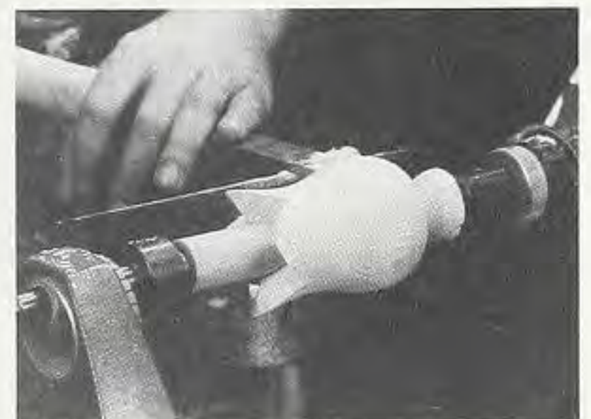
Figure 8. Turn the outside shape of the tulips on a lathe. Plug the tops with a dowel so you can mount the stock on the lathe.
