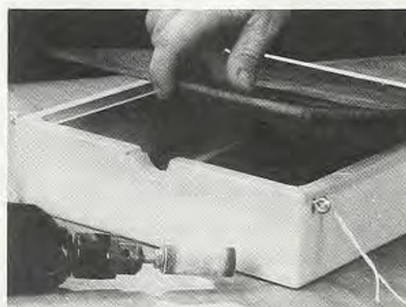
Figure 4. Rip the top from the base on a table saw. On the last cut, insert \frac{1}{8} " spacers in the kerfs and clamp them in place. This will keep the top from pinching the blade on the last cut.
