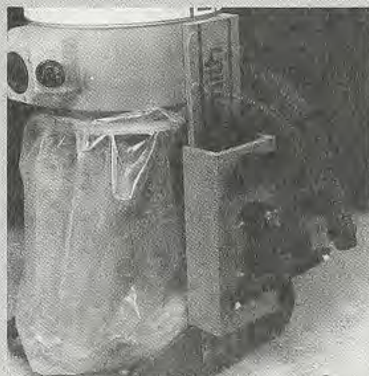
Figure A. A 'caddy' mounted on your shop vacuum keeps your vacuum accessories handy.
