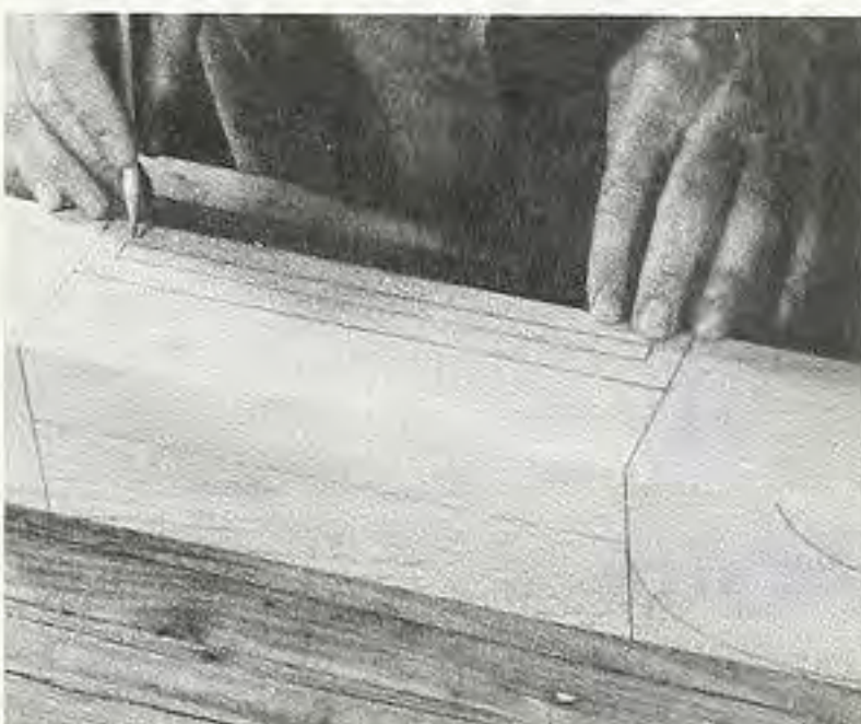
Figure 2. Mark the stiles and the mortises on the corners opposite the leg patterns.
