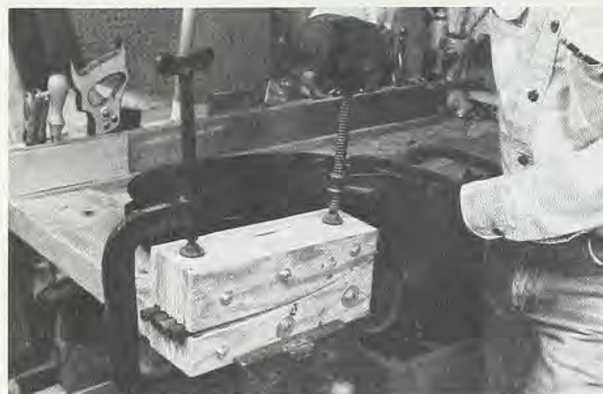
Figure 3. When the boiled wood is in place, clamp the parts of the mold together. Do this quickly, before the wood cools.
