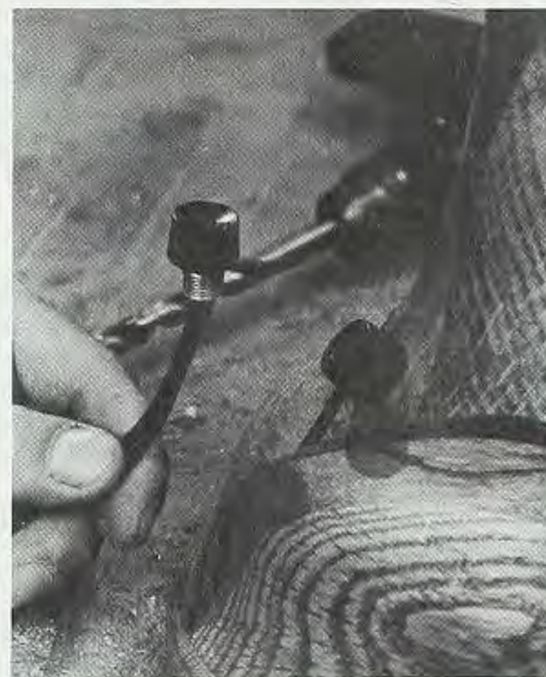
Figure 7. Install the switch by pressing it into a hole drilled in the turning. The hole should be slightly smaller than the threaded base of the switch. To prevent the switch from coming loose, rub some epoxy glue on the threads.
