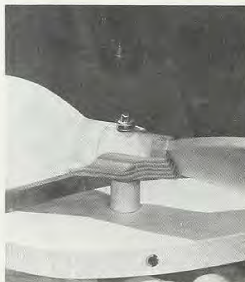
Figure 5. Hold the wings on the rod with cap nuts. These cap nuts are hammered onto the ends of the rods.
