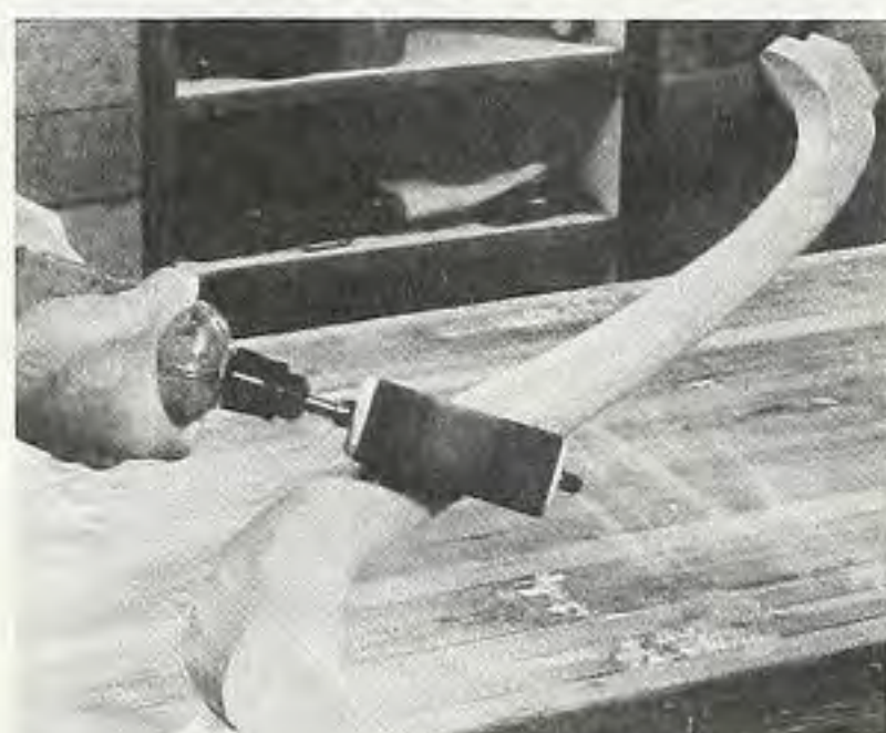
Figure 5. Use a pneumatic (or air-filled) drum sander to sand the cabriole legs.
