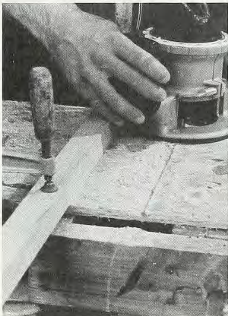
Figure 1. If you cut the dados with a router, use a straightedge to guide your work. Make each joint in several passes, cutting just \frac{1}{8} "- \frac{1}{4} " deeper with each pass.
