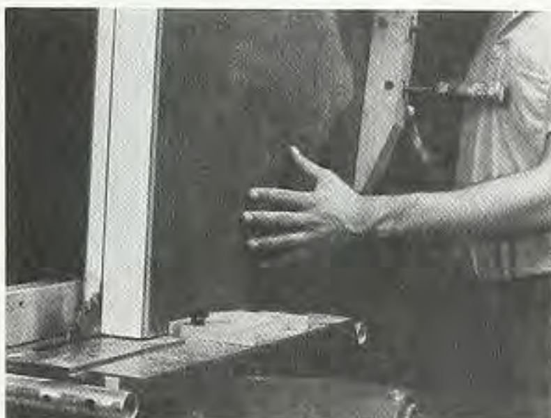
Figure 4. Rip the top from the base on a table saw. On the last cut, insert \frac{1}{8} " spacers in the kerfs and clamp them in place. This will keep the top from pinching the blade on the last cut.
