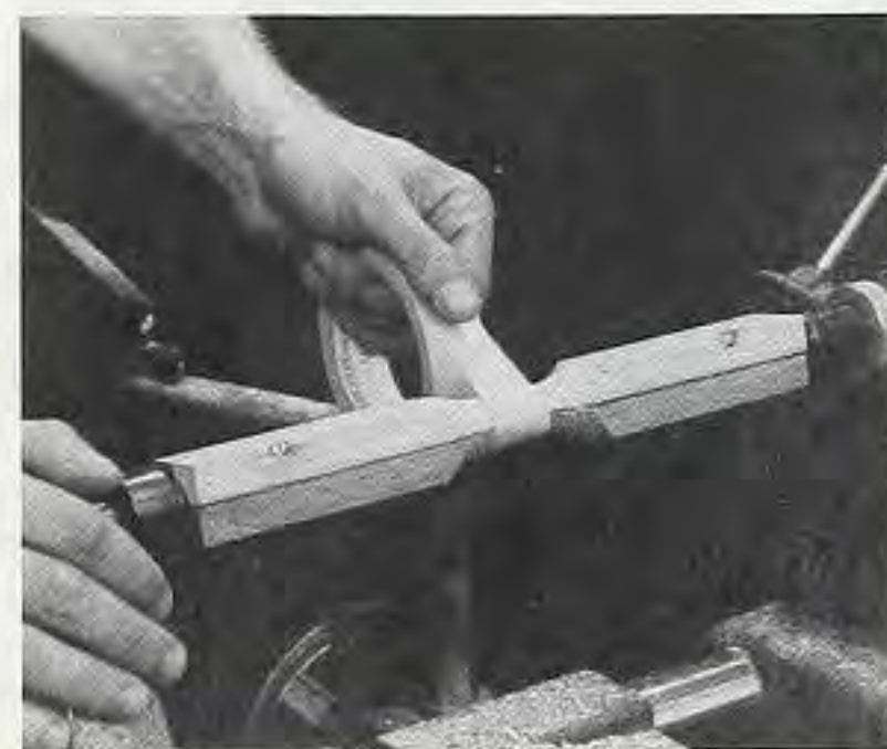
Figure 11. Turn the middle of the post first and wrap a piece of tape around it to help hold the strip in place.
