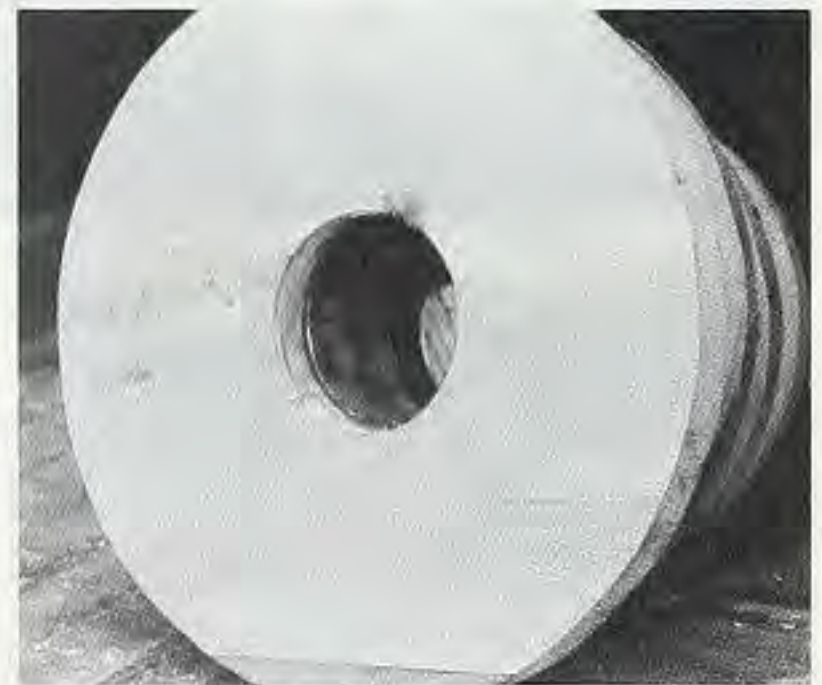
Figure 3. Leave a small shaft down the center of the turning blank and a cavity in the bottom of the lamp base to accommodate the necessary lamp hardware and wiring connections.
