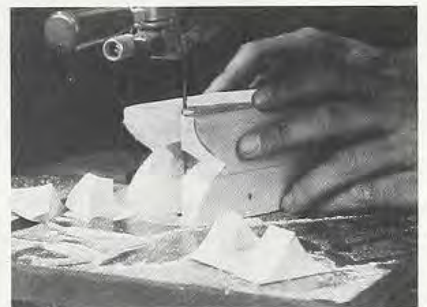
Figure 7. Cut the shapes of the tops of the tulips on a band-saw. Make two cuts, on two adjacent sides.
