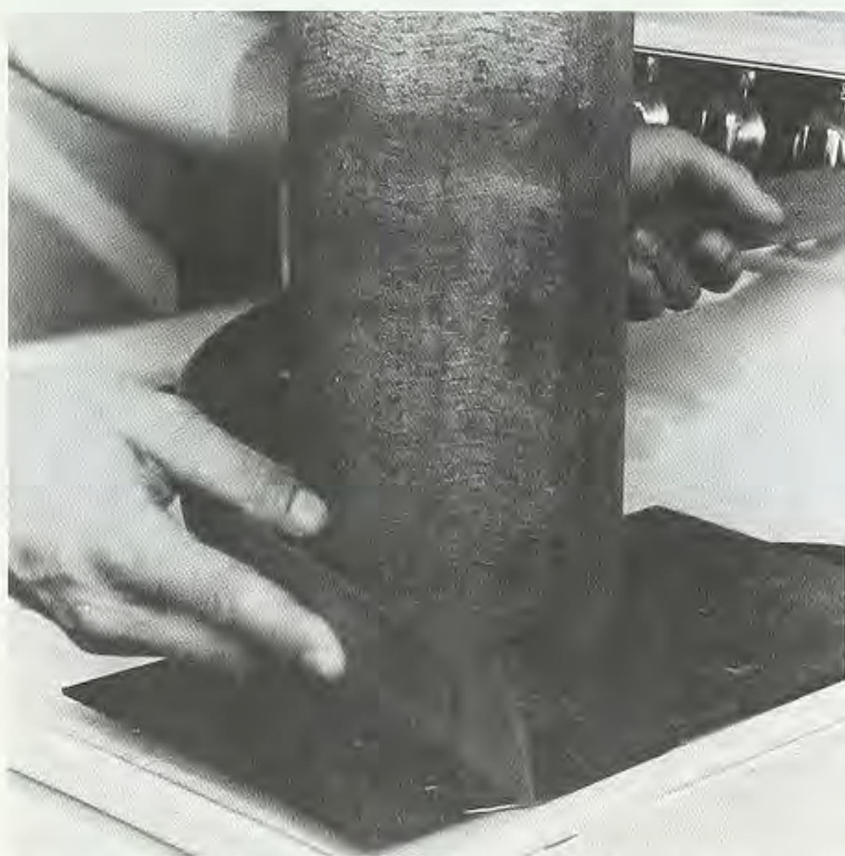
Figure 4. To use a bending iron, press the wood gently against the hot metal until it begins to 'give'. Be careful not to scorch the wood.
