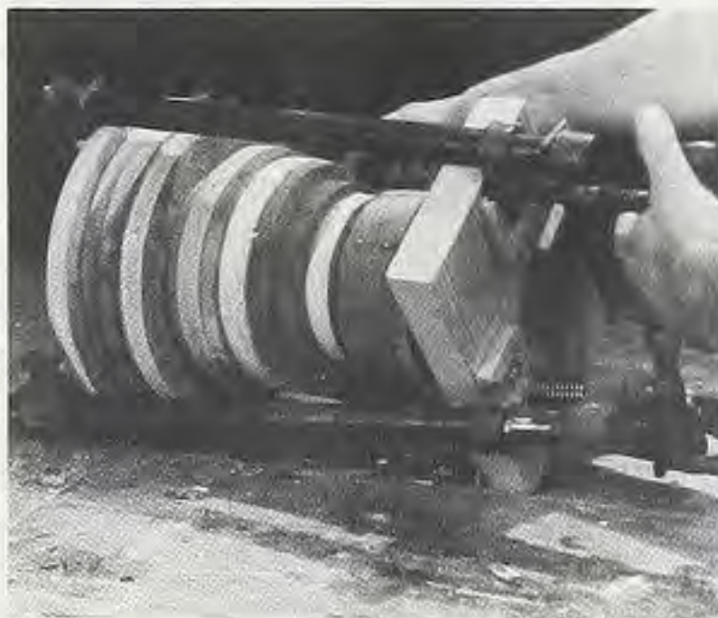
Figure 3. Leave a small shaft down the center of the turning blank and a cavity in the bottom of the lamp base to accommodate the necessary lamp hardware and wiring connections.
