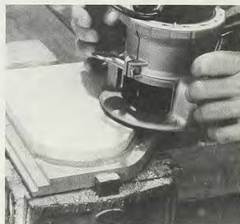
Figure 5. Cut the grooves in the sides with the router, keeping the router plate flat on the template and the guide bushing pressed up against the edge of the template.
