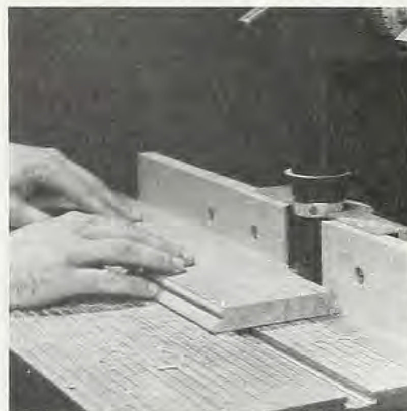
Figure 1. To make your own molding, first cut the shape in the edge of a wide board. Guard removed for clarity.
