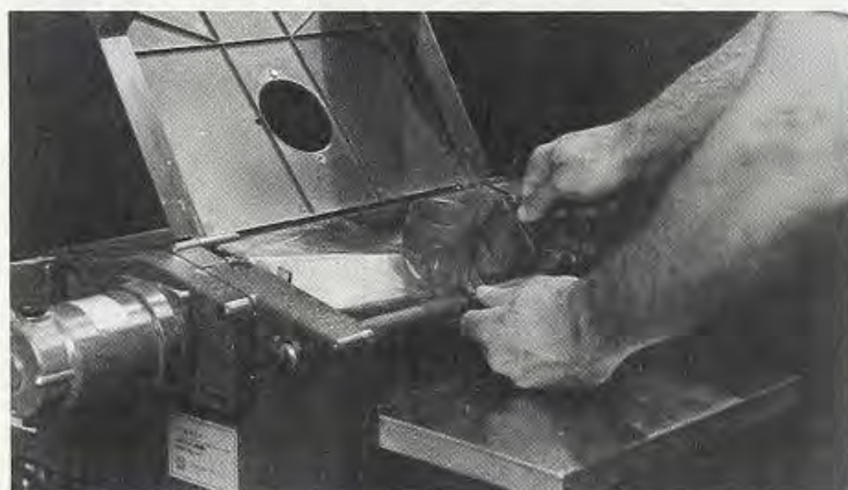
Figure 10. The planer pick-up fits under the outfeed housing, and the vacuum port comes up through the housing.
