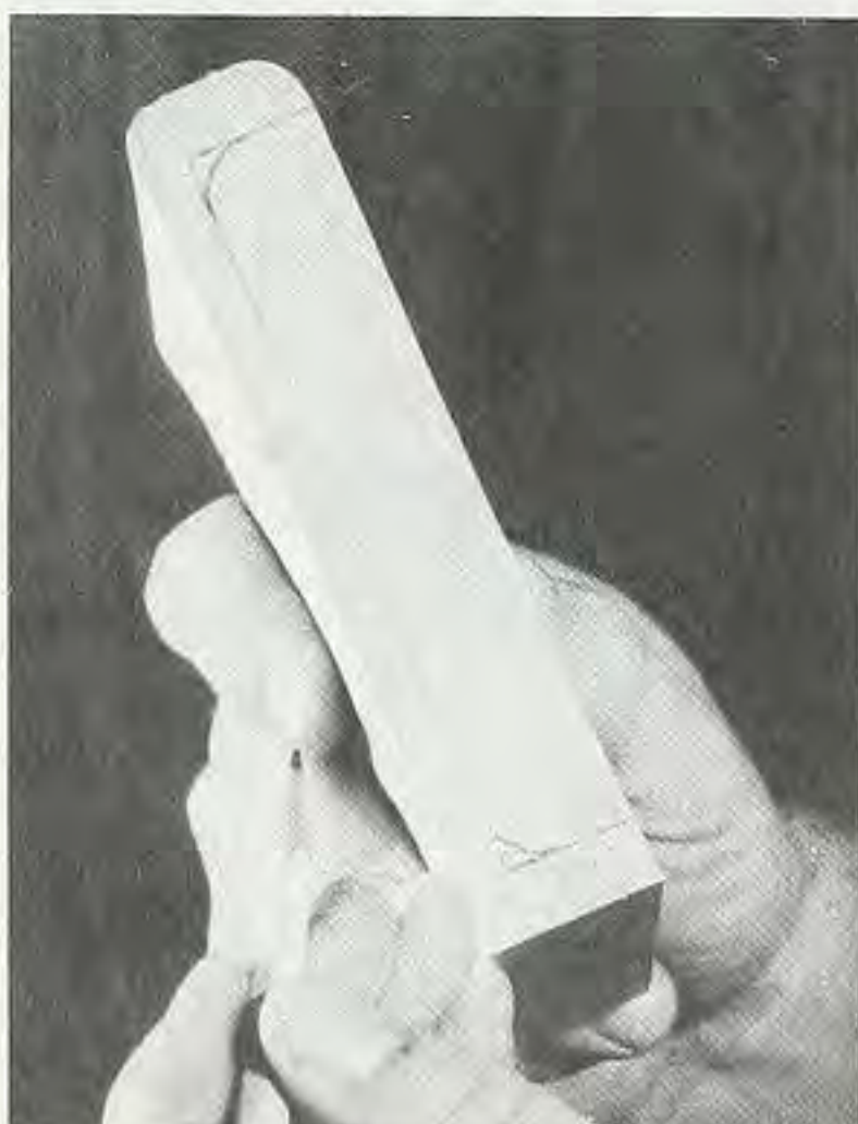
Figure 5. Cut the sides off the drawer blanks, in the same manner you cut the box sides.
