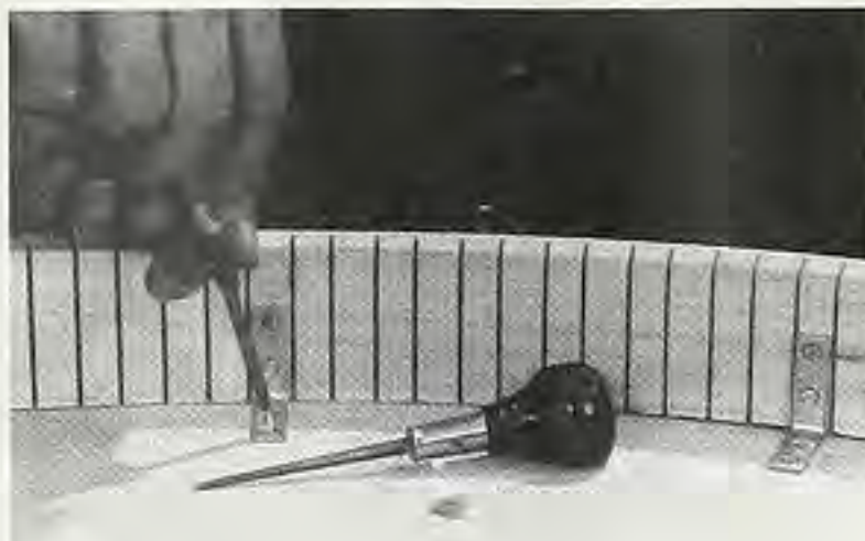
Figure 7. To keep the aprons in place, use small angle brackets, screwed to the back side of the aprons and the underside of the top halves, every 8"-12".
