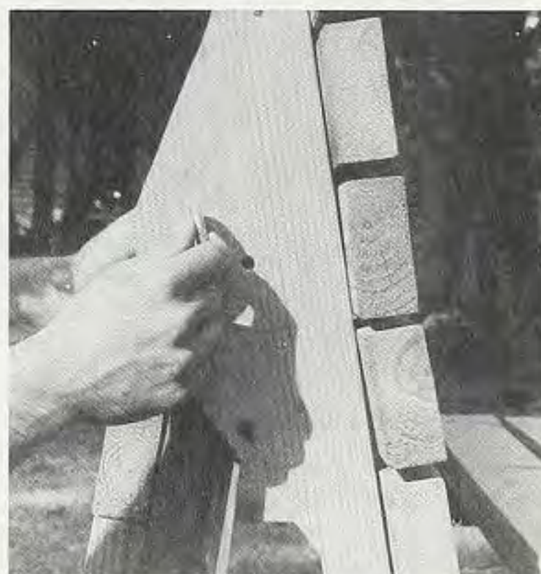
Figure 3. To lower the table top to the vertical (bench) position, remove the eye bolts and re-insert them in the second set of stop pin holes.
