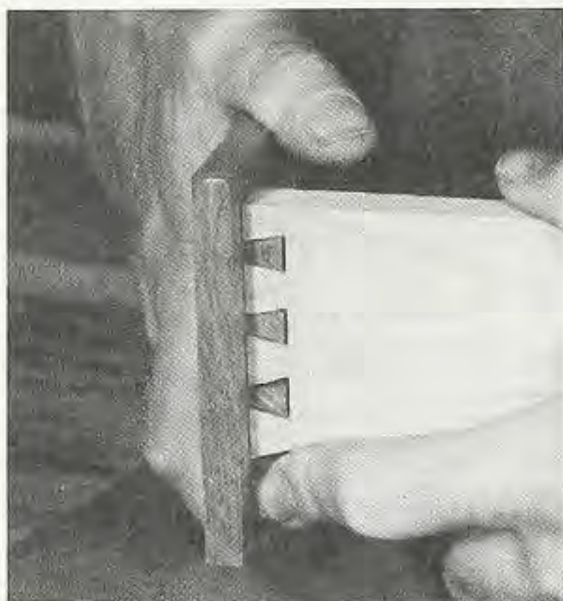
Figure 6. The fronts of the drawers are attached to the sides with half-blind dovetails — you can't see the joint from the front.
