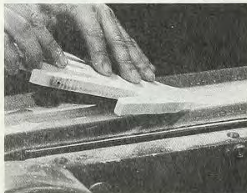
Figure 1. Taper the wrist with the aid of a belt sander.
