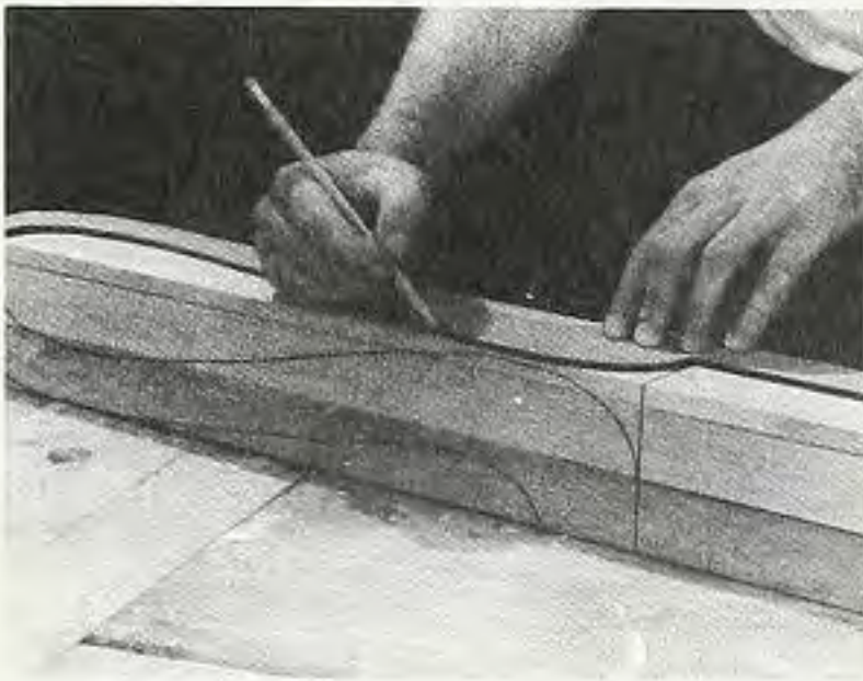
Figure 1. Mark the leg patterns with a cardboard or hard-board template. Be sure that the knees meet at the corner.
