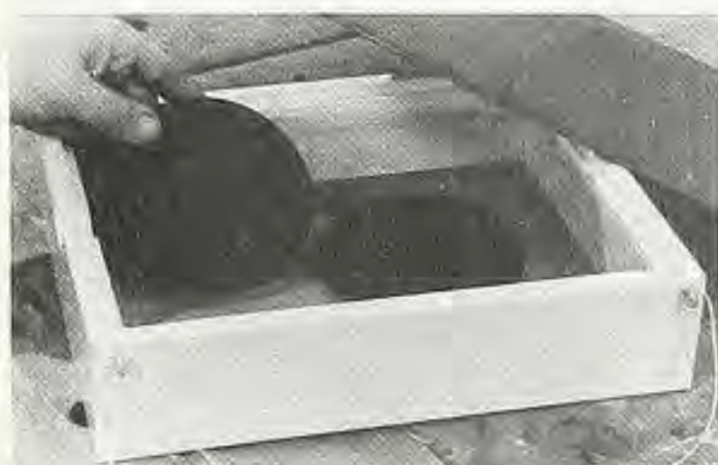
Figure 8. To enhance the pendulum action of the drawing board, place weights on the inside.
