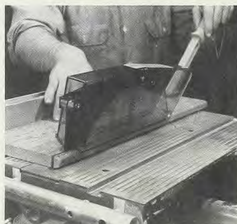
Figure 6. Round over the corners of the tambour stock; then rip the tambour from the stock.
