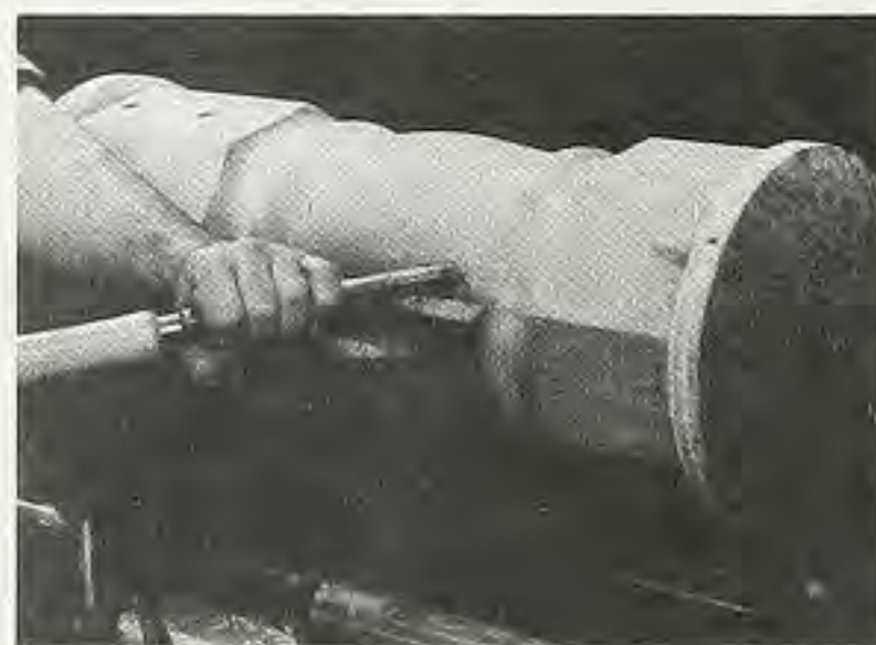
Figure 4. Temporarily, install discs of scrap wood at either end of the pedestal so that you can mount the hollow pedestal to the lathe.
