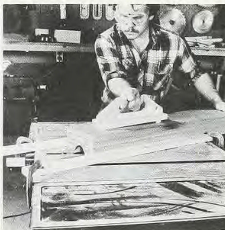
Figure 7. To shape the bracket feet, first cut a cove in the front face of the stock by passing the board across your table saw at an angle to the blade.
