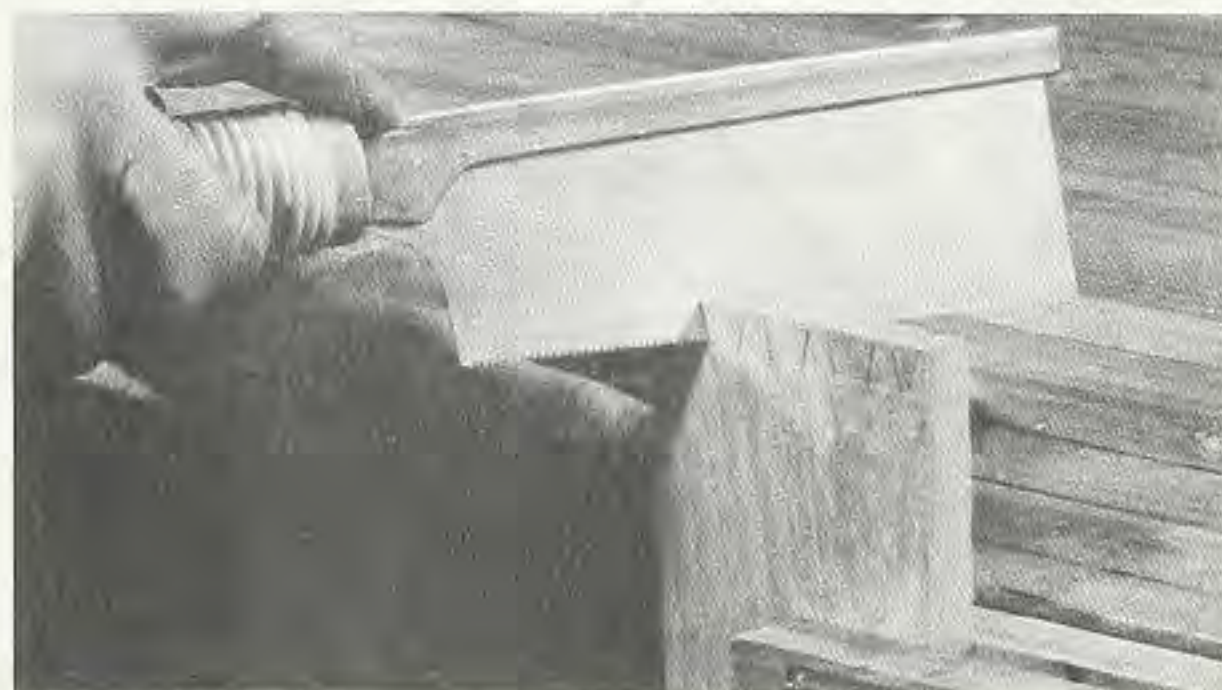
Figure 9. Carefully cut along the marks with a saw. A Japanese 'Dozuki' saw works best.
