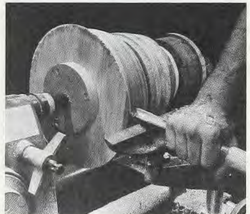
Figure 4. 'Cap' the ends of the turning blank so that you have someplace solid to mount the lathe centers. If you wish, these caps can become part of the turning.
