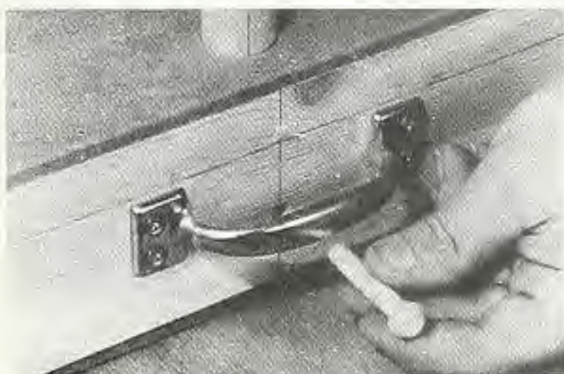
Figure 7. Use a toy 'axle peg' to pin the drawing arm support dowel in place.
