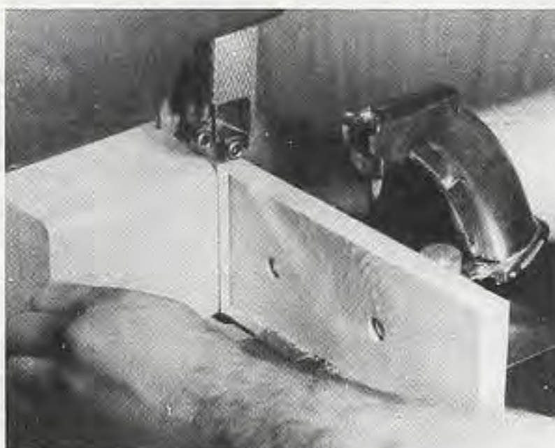
Figure 1. Using a rip fence as a guide, cut off the sides of the box stock.
