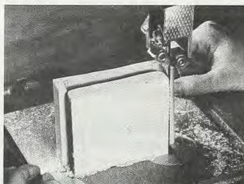
Figure 7. Cut out the drawer insides and discard them.
