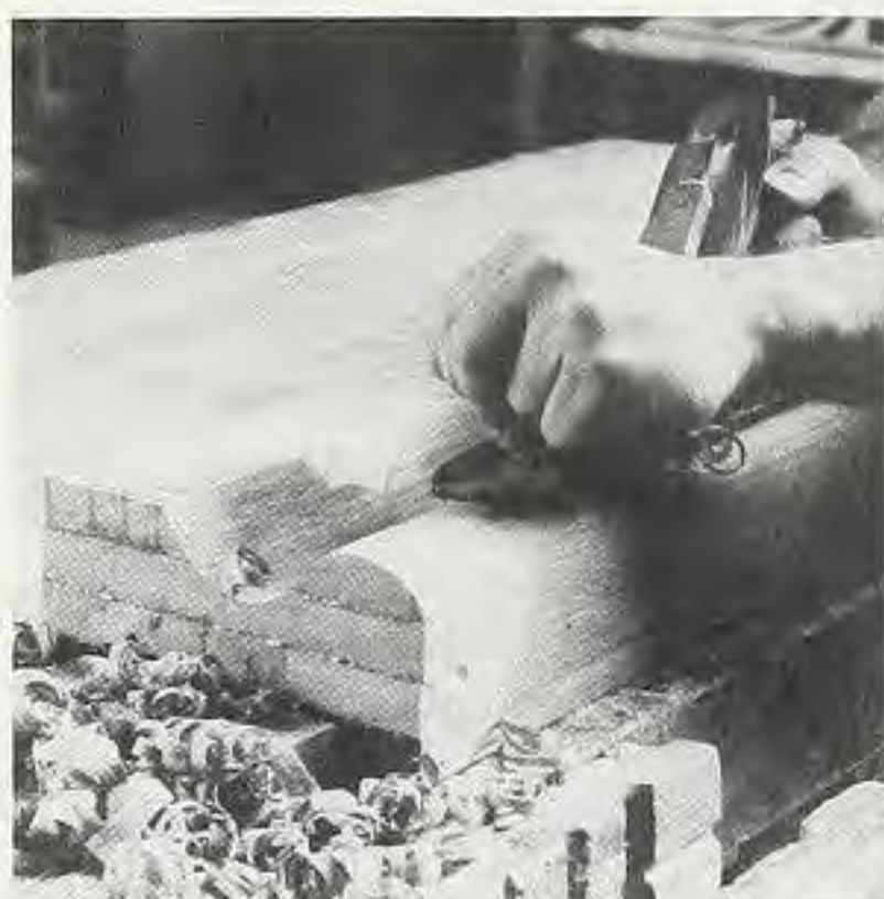
Figure 8. Then round the top portion of the front face with a hand plane, completing the classic cyma curve.
