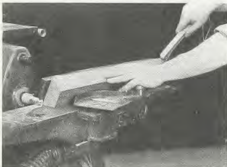
Figure 2. Join the edges of the pedestal parts at 22½°. Tilt the jointer fence in, towards the work.
