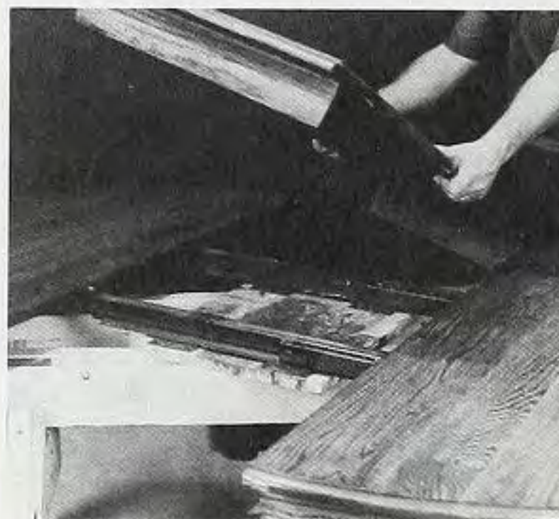
Figure 1. Using special 'equalizer slides', made especially for pedestal tables, the top halves slide apart so that you can install a leaf for more table space.
