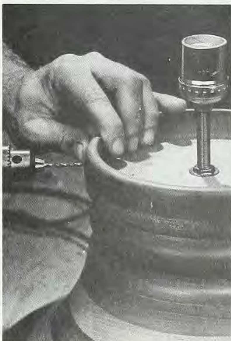
Figure 5. Some metal collars require that you turn a small bowl-shaped recess in the top cap, so that the collar will mount flush to the top of the turning.
