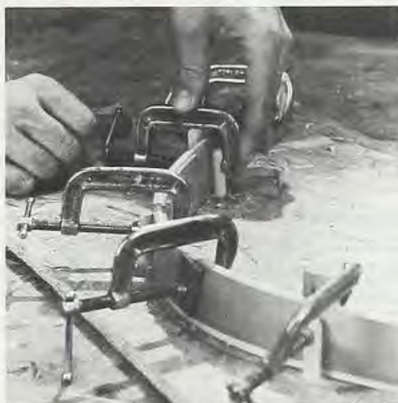
Figure 7. Glue the surfaces of the strips together in the jig. Use plenty of glue, and plenty of clamps — you don't want any gaps between the laminations.
