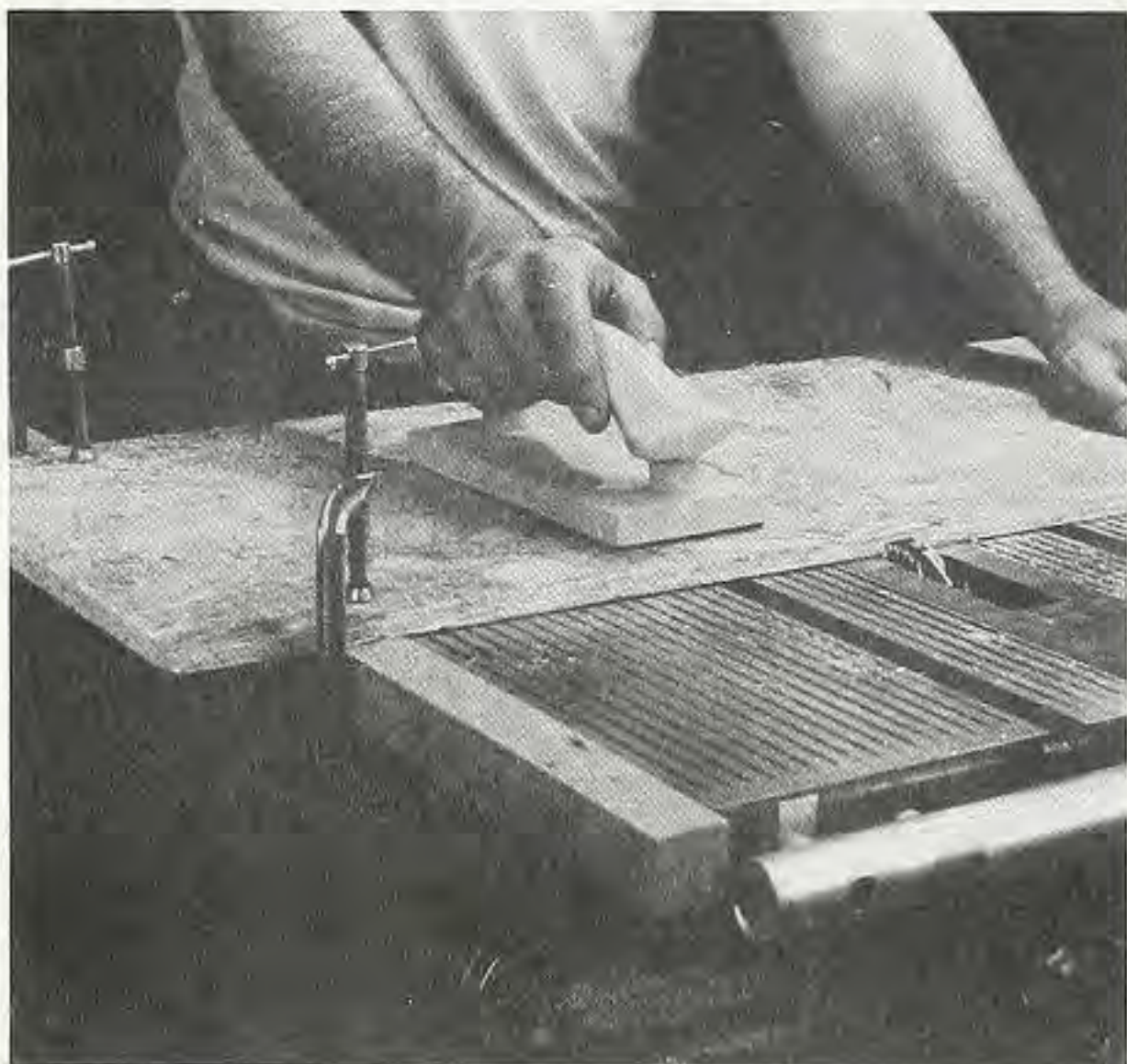
Figure 2. If you cut the dados with a table saw, use a straightedge (clamped to the underside of the stock) as an 'auxiliary fence' to guide the work. Keep the straightedge pressed up against the edge of the table saw.
