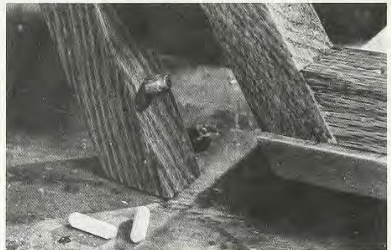
Figure 8. If you wish, install alignment pins in the slanting legs to keep the front and back frames halves properly aligned.
