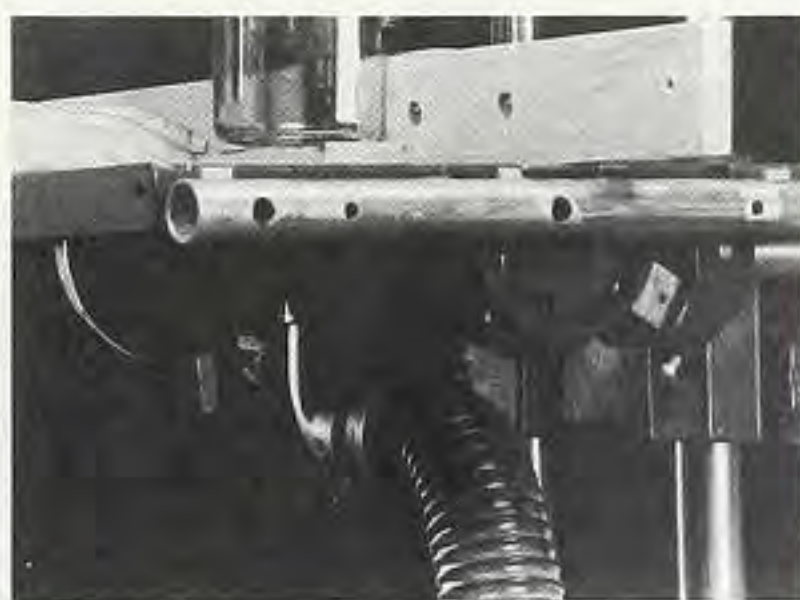
Figure 8. Both the shaper and the router accessories use the same pick-up. The pick-up bolts under the worktable.
