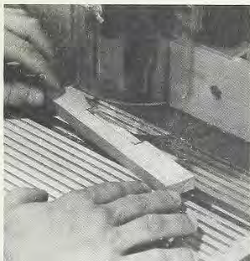
Figure 7. Rout the handholds in the lead tambour with a 3/4" straight bit.
