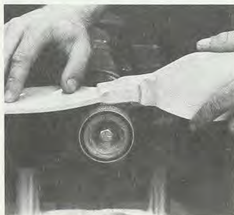
Figure 4. After you glue the wings in the bushing blocks, taper the blocks on a belt sander.
