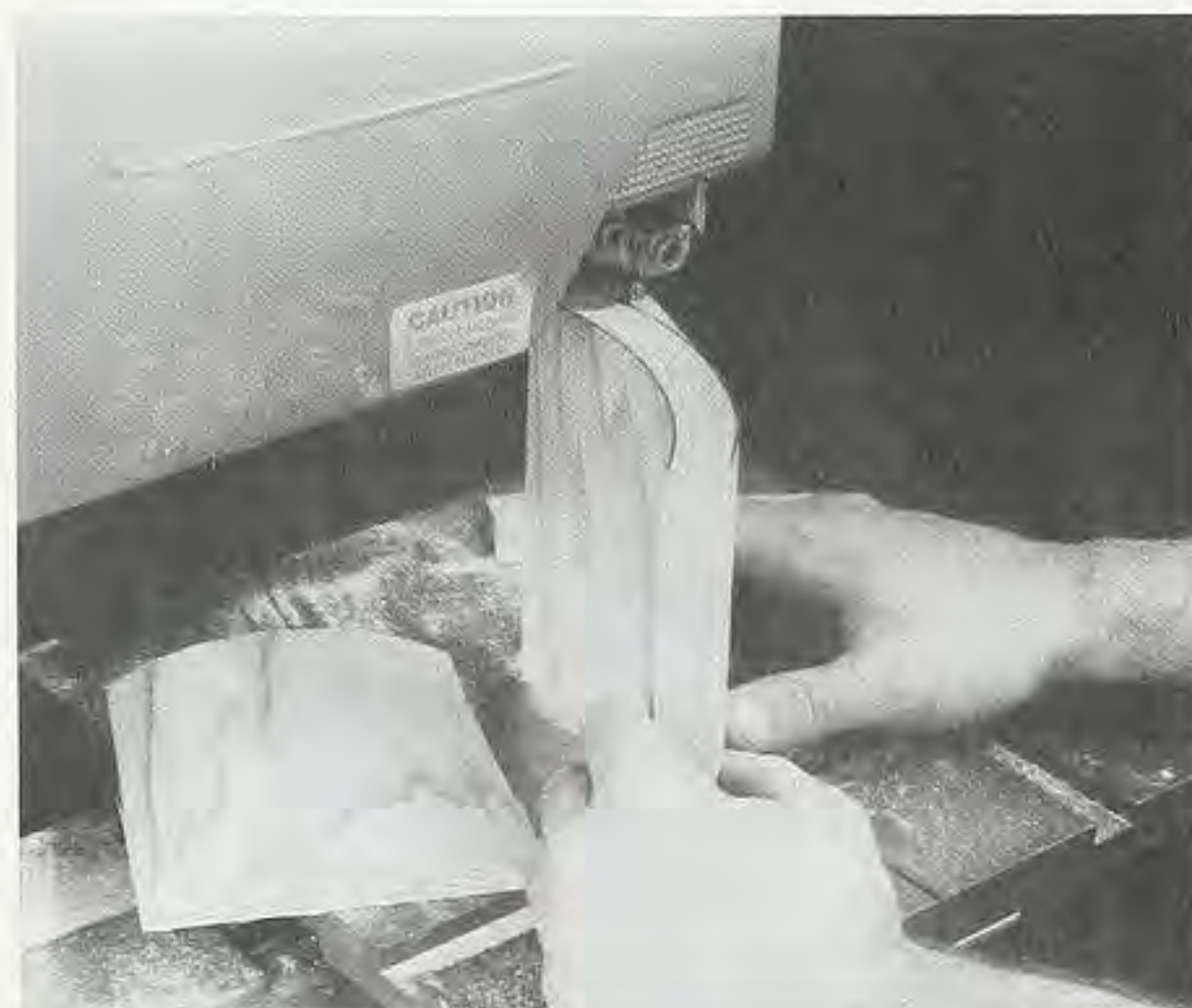
Figure 5. Cut the curved roof from thick stock. The curve must match the curve of the cab.
