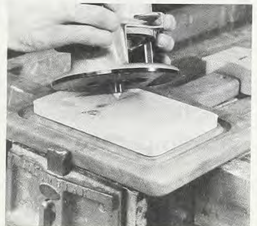
Figure 2. Cut the round-bottom grooves in the meat and vegetables side with your router. Keep the base flat on the surface of the template, and the guide bushing pressed up against the edge of the template.
