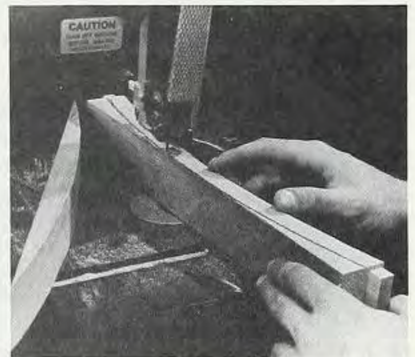
Figure 5. Using a bandsaw, cut the curved slats from thick stock.
