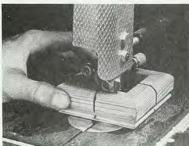
Figure 12. Using a bandsaw, cut the feet from a frame made with the foot molding.
