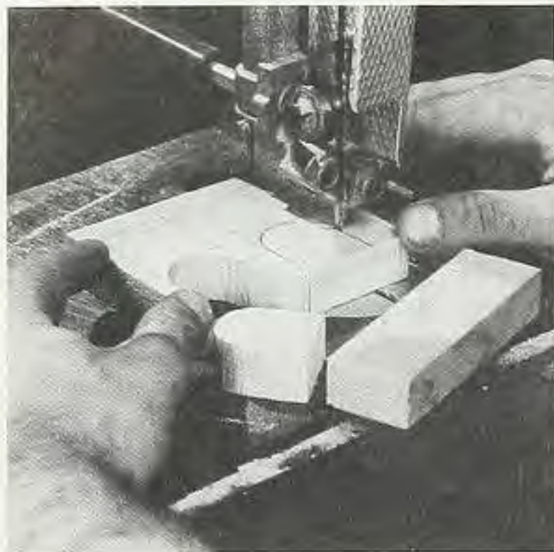
Figure 2. To cut the windows out on a bandsaw, first saw the cab sides in half. Cut the shapes of the windows in the upper half.
