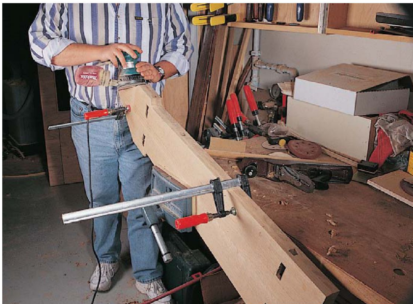
With the sides clamped together and mounted in my vise, shaping the sides simply took some sanding and planing.
