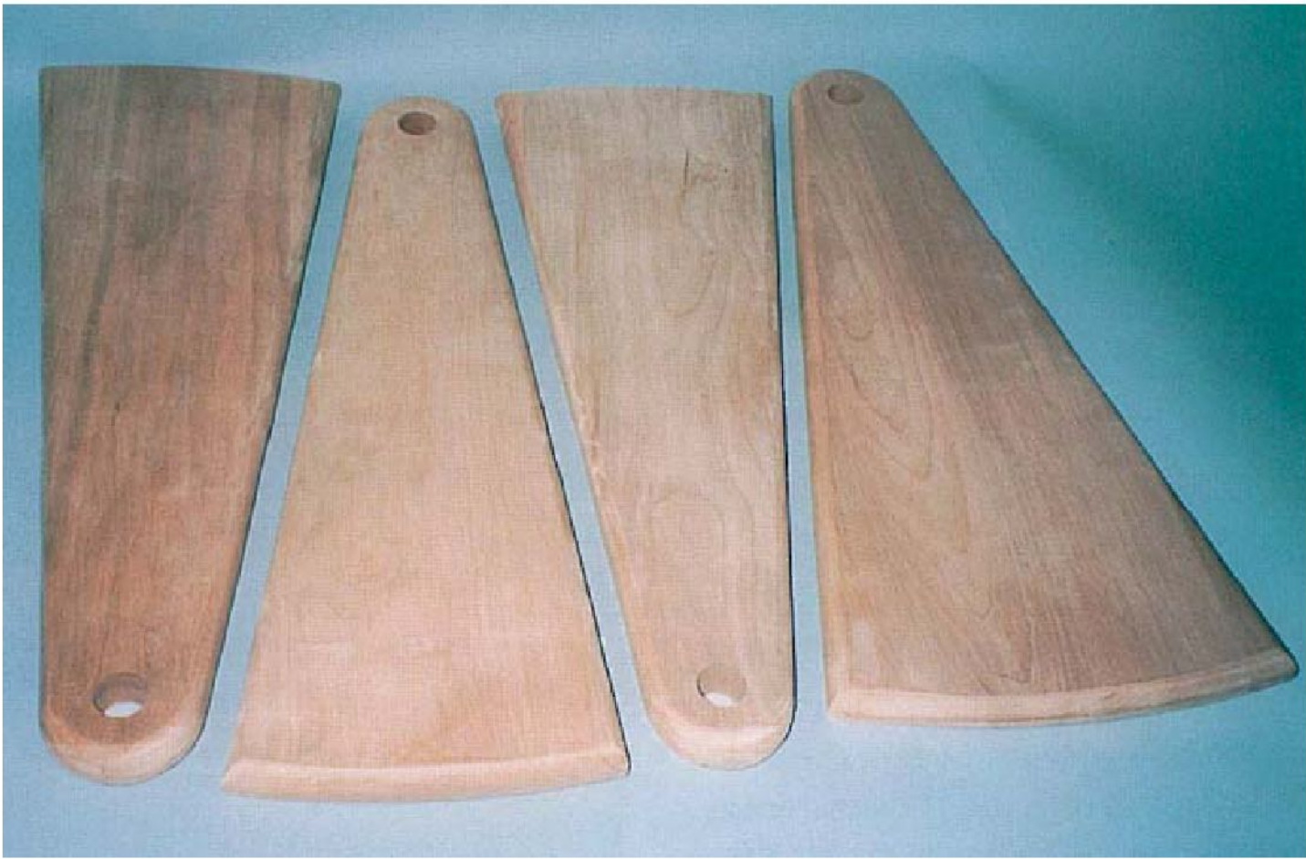
7 The completed stair treads. Remember that the top tread is slightly wider to accommodate a lamp.
