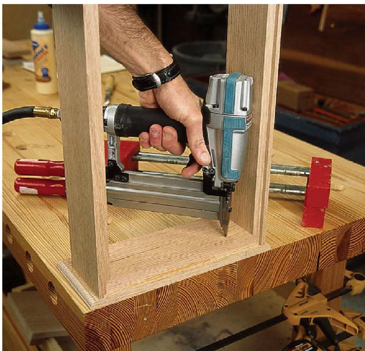
Above, you can see how a couple of well-placed nails keep everything in line as I apply the clamps. Whenever you can, use your bench to assist your clamping (right). It helps spread clamping pressure over a wider area.
