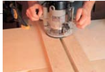
Here's the simple jig to rout the dadoes. It uses a bearing-on-top straight bit to guide against the edges of the jig. Clamp the jig right on the marked lines and rout the dado.
