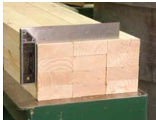
Silk purse. After drying, jointing and planing, this common material is now fit to use.
