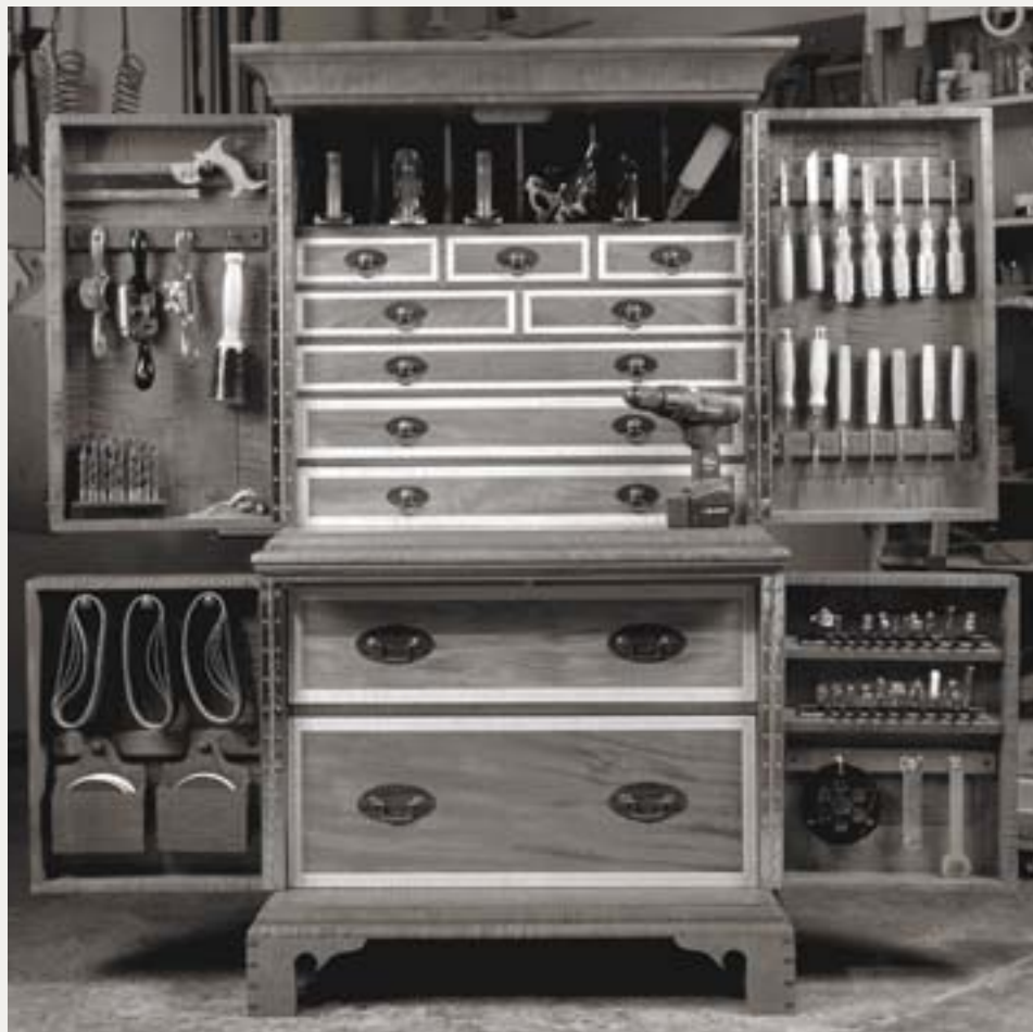
This tool cabinet, built by Malcolm and Glen Huey (owners of Malcolm Huey & Son, a custom woodworking shop in Middletown, Ohio) marries hand-tool and power-tool storage with drawers, deep-set doors, magnetic strips, cubbies, brass hooks, Shaker pegs and Shaker boxes.
