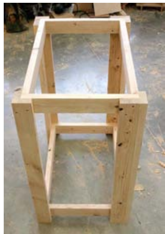
All together now. With the frames inside the leg assemblies, this table is ready for a plywood shelf and top.
