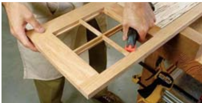
Install the horizontal muntins the same way. First glue a backing strip into the rabbet on the backside of the door. Then flip the door over and glue the muntin to that.
