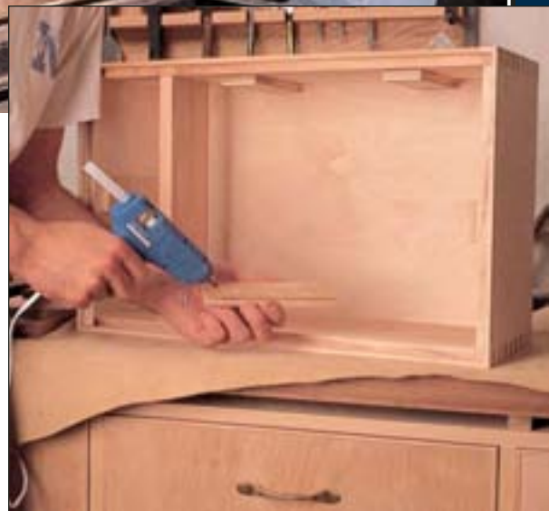
Use hot melt glue to attach 6"-long blocks that keep the saw kerf open when you cut the front off the cabinet (inset). After that, ripping the cabinet is almost cake.
