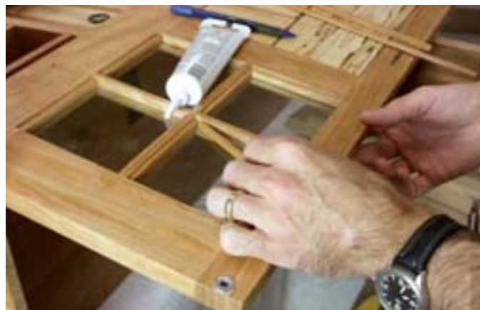
Once everything is finished, install the glass using small strips of cherry ( \frac{1}{8} " and \frac{1}{4} " thick). A few dabs of clear silicone and a couple small pins do the trick.
