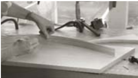
Two nails and a thin piece of offcut make a fine (and cheap) arc marker.
