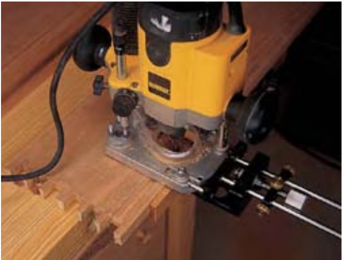
Cut the groove for the 1/2"-thick bottom in two passes using a plunge router outfitted with a straight bit and an edge guide. On the pin boards, you can cut the groove through the ends because it won't show.
