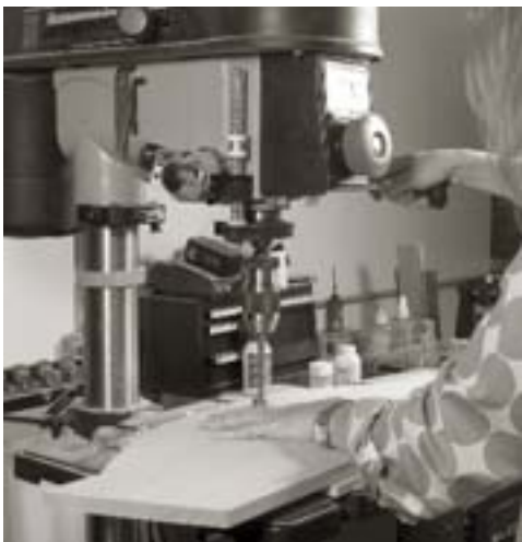
Use a drill press to cut the outside ends of your handhold, and a jigsaw to remove the remaining waste. You'll do the final shaping with a rasp and sandpaper.
