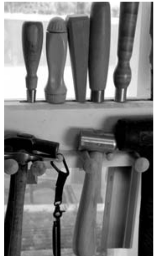
The two pieces are separated by \frac{1}{2} "-thick spacers, and tools drop into the space. This was a "sweet spot" for our tools and can be varied to accommodate your tools.
