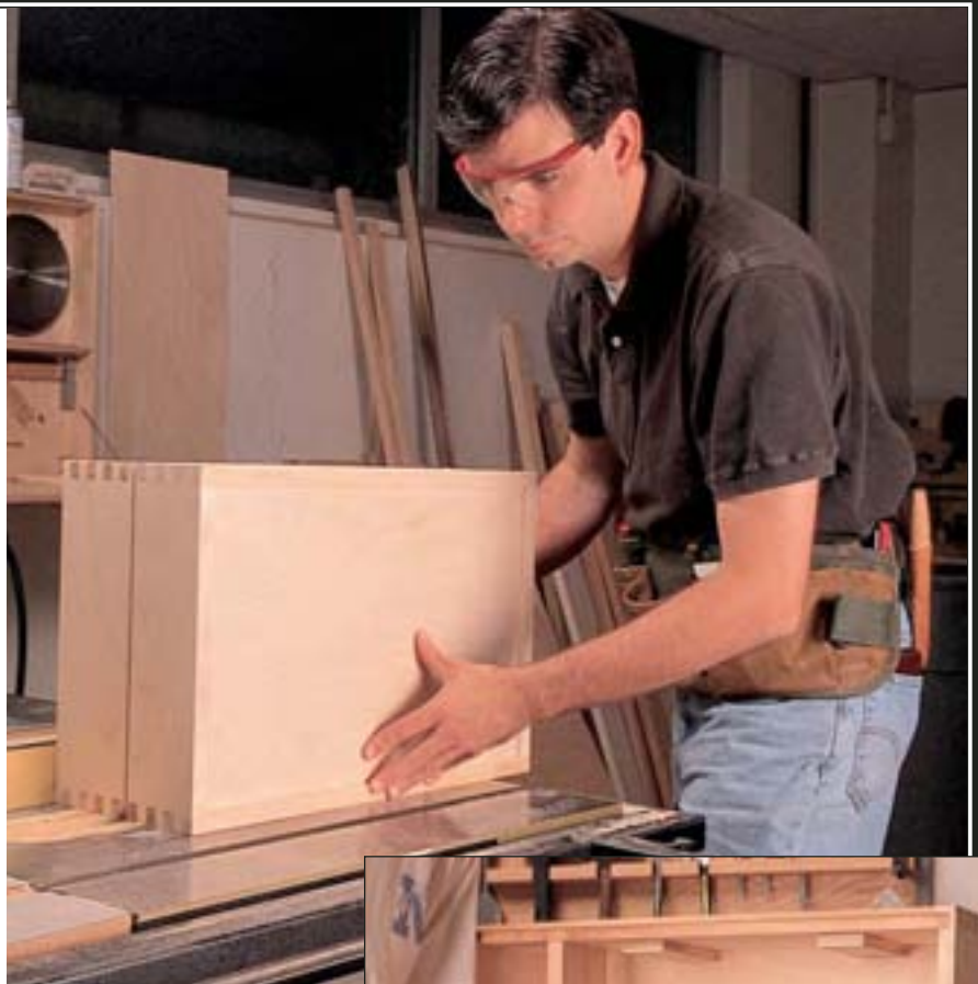
Use hot melt glue to attach 6"-long blocks that keep the saw kerf open when you cut the front off the cabinet (inset). After that, ripping the cabinet is almost cake.
