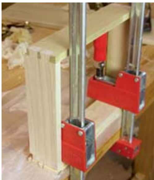
Build the drawers with through-dovetails. Then glue a piece of \frac{1}{4} "-thick veneer to the front.
