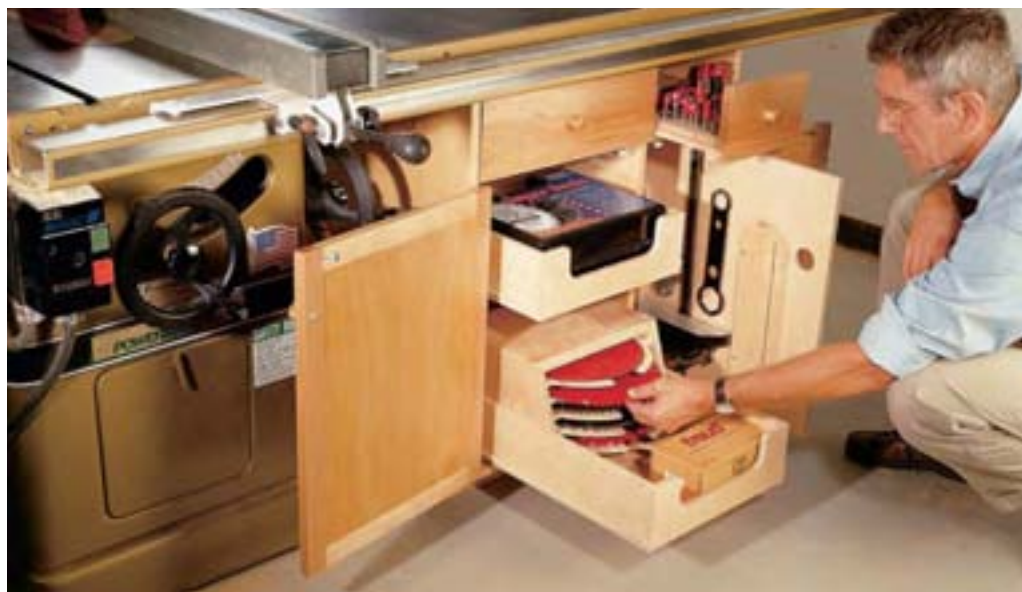
This saw blade box fits perfectly in the "Under-the-saw Cabinet" featured in the December 2002 issue. The cabinet is a great project for the small shop. It offers considerable storage beneath the wing of your saw – usually wasted space. For complete plans for the cabinet, order the back issue (issue #131) by visiting our web site at popwood.com or calling 888-419-0421.
