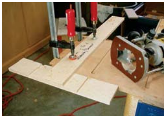
Here you can see how you use the dado cut into the jig to line up the jig with your layout lines. Using a router with a flat side on its base is more accurate than using a router with a round base.
