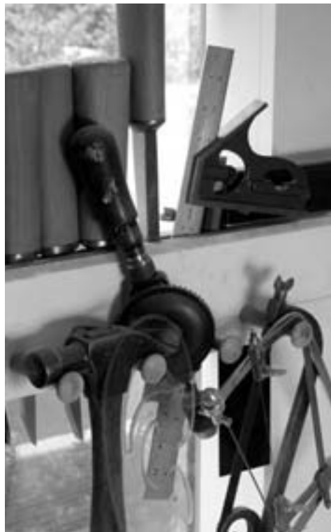
The simple start is two pieces of wood, \frac{3}{4} " thick x 3\frac{1}{2} " wide, of a convenient length. The back piece is longer than the front by a few inches to allow fastening to the wall. The rack is wide enough to hold tools securely, and provides a place for Shaker pegs for hanging tools.
