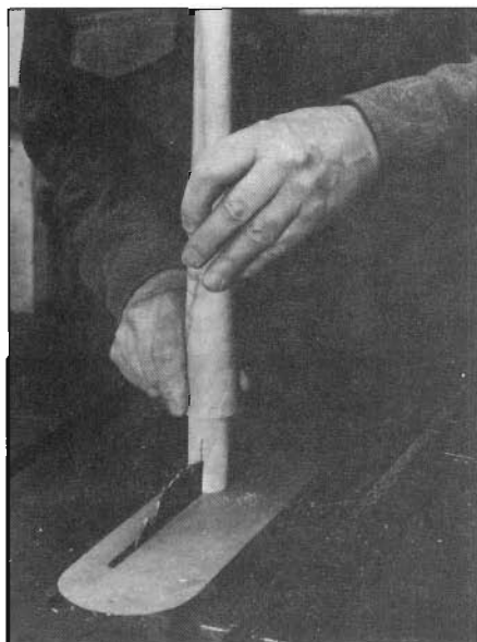
Carefully cut the notch for the wedge freehand on the table saw.
