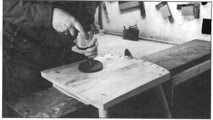
Clamp a plank to the top of the workbench to support the seat while you work on it. Saw the ends of the tenons, and finish the surface with a rotary sander followed by a pad sander.
