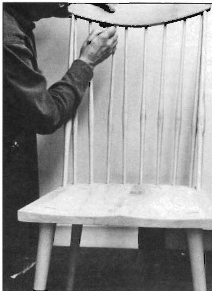
Fit the back rail onto the brace spindles to mark its position on the back spindles.
