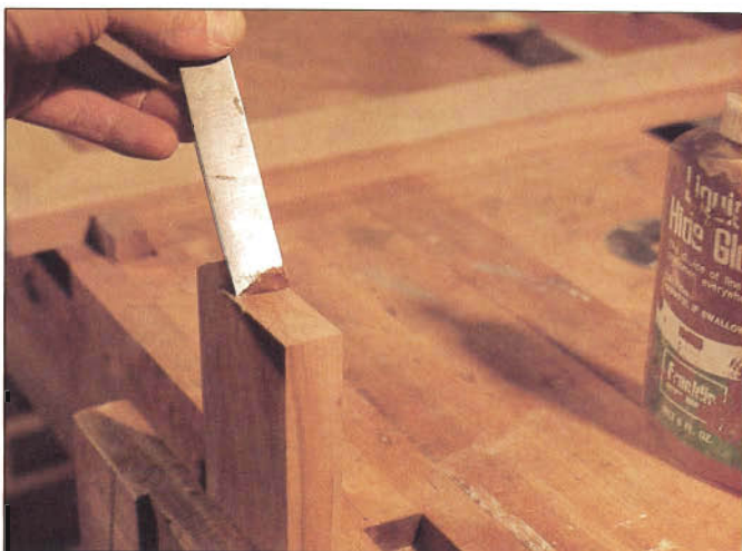
Put a single drop of liquid hide glue on the end grain. After scraping, apply the glue to the flawed area with the chisel.
