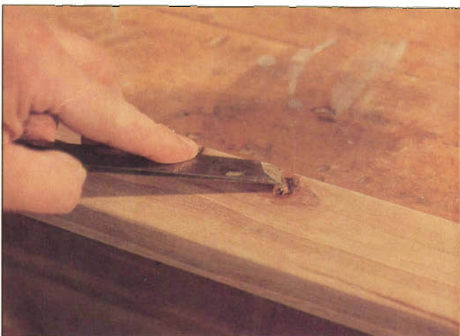
Put a single drop of liquid hide glue on the end grain. After scraping, apply the glue to the flawed area with the chisel.
