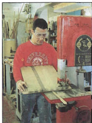
For the smaller pieces, a shop-made miter gauge with a 12° ramp proved to be an effective way to make band saw kerfs that established the bottoms of the sockets; however, this setup was too cumbersome to use for the long pieces.
