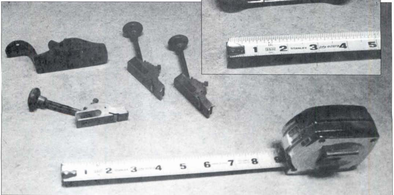
The Kunz palm plane and the Conover finger planes shown below are excellent for precise work on small pieces.
