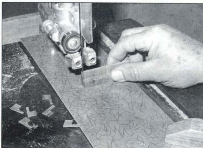
Bandsaw individual flags from the L-shaped stock. Plastic laminate fitted around the blade will keep the tiny pieces from falling through.
