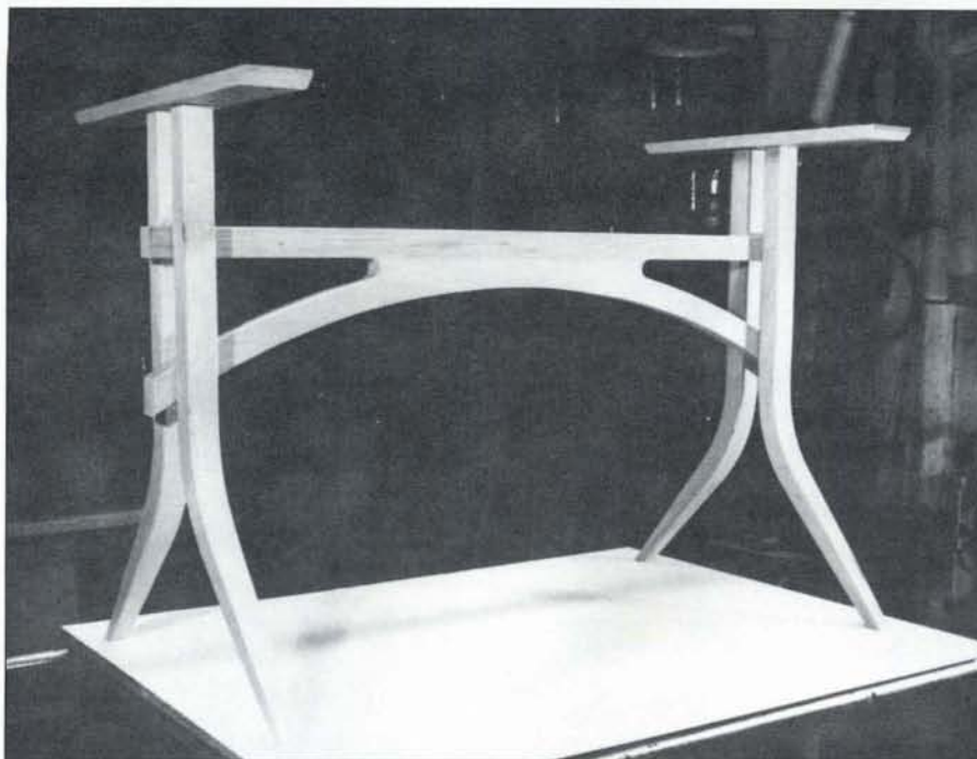
Dry-assemble the base with the dowels connecting the legs and the spreader, and check that the assembly sits flat and straight.
