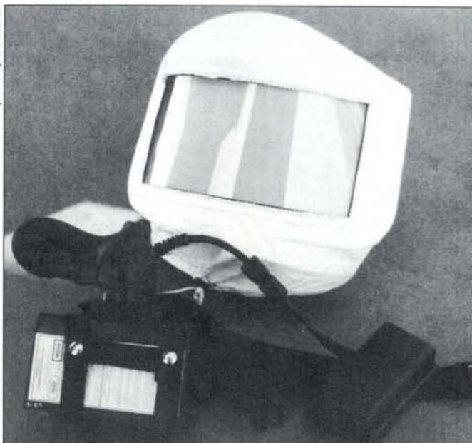
The fan, filter and batteries of the Neoterik Mini-Breezer are worn on the belt and connect to the Tyvek® hood via an air hose.
