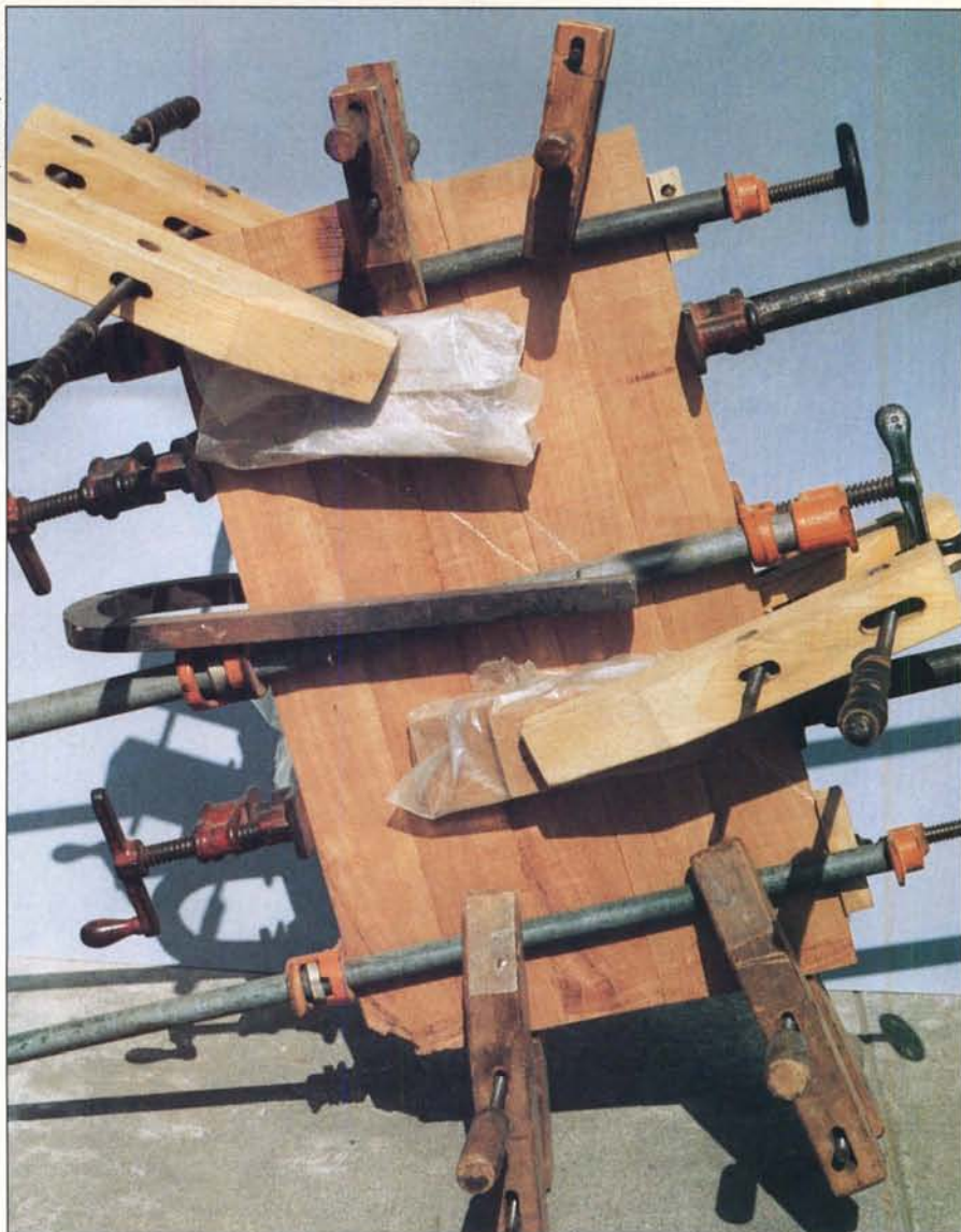
The photo and the illustration show the bottom panel glued and clamped. Note how the panel is clamped to prevent buckling.
