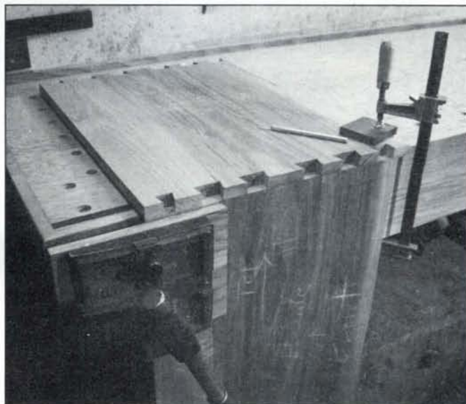
Secure the top and a side to the bench with their back edges aligned, and use a knife to mark the pins by tracing the tails.
