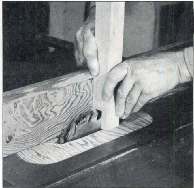
Cut the open mortises slightly thinner than the thickness of the side panels, and pare them with a chisel for a snug fit.
