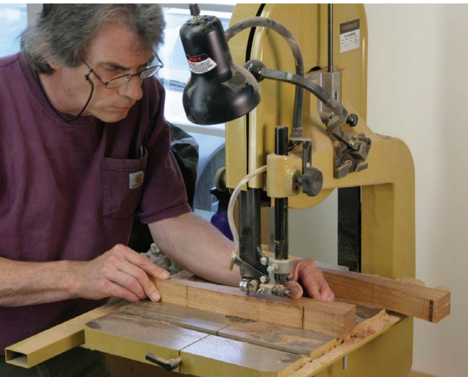
A stack of four blanks held together with double-sided tape yields eight matching corbels.
