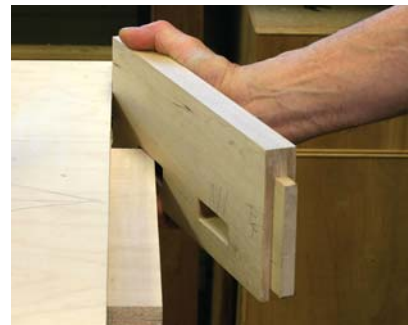
When a corner can be forced into the mortise, the thickness is close. Then it's time to cut the edges of the tenons.
