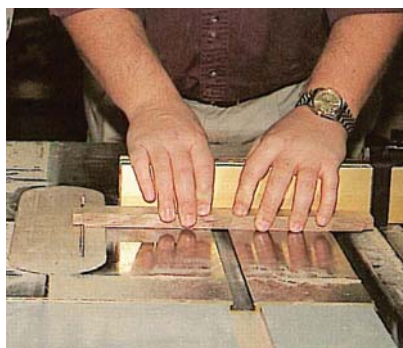
Use a simple stop block clamped onto the miter gauge to set the tenon shoulder depth.
