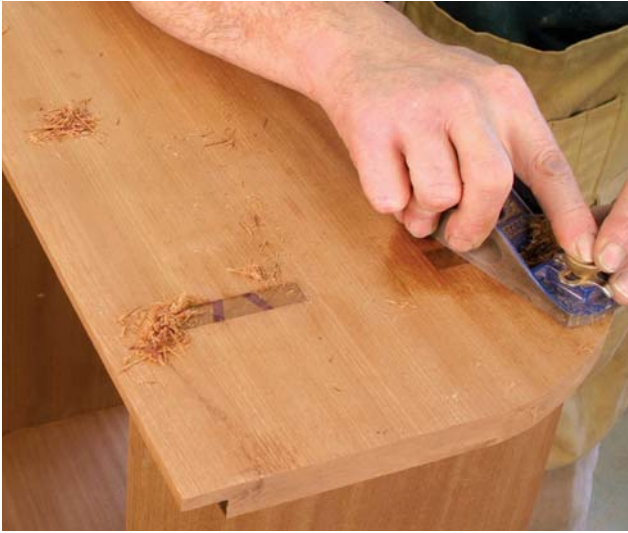
After sawing off the wedges, the joints are soaked with paint thinner to make it easier to trim the end grain flush.
