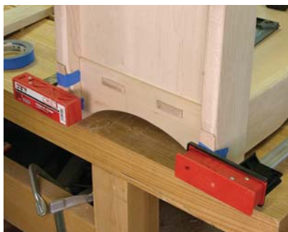
Offcuts from tapering the legs are taped in place to provide a flat surface for the clamps.
