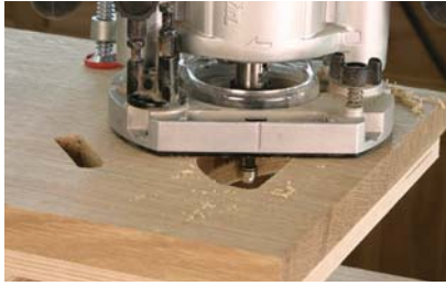
Cut close to the lines with a jigsaw and use the router to trim the opening at the top.
