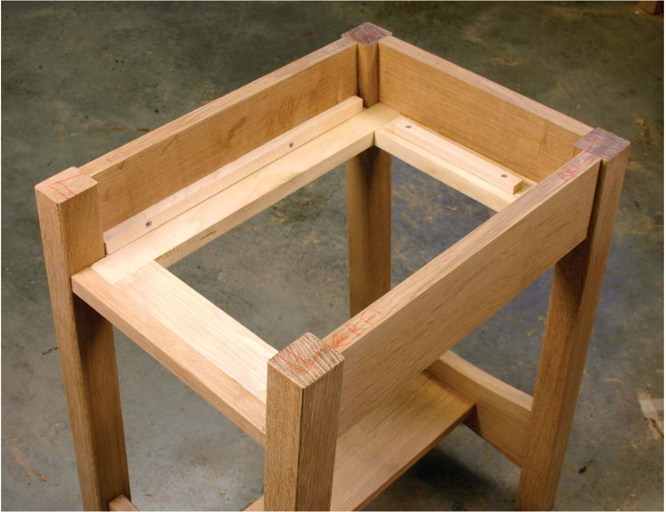
The assembled web frame is notched around the legs. After fitting the drawer runners between the legs, they are screwed in place, and the drawer stop is also attached with screws to the frame.
