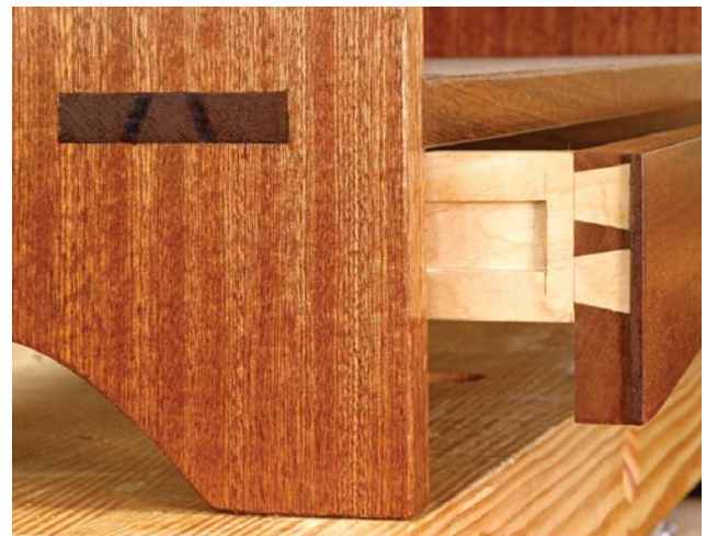
The rabbet in the end of the drawer front provides clearance for the sides, while allowing a narrow margin to be trimmed easily.
