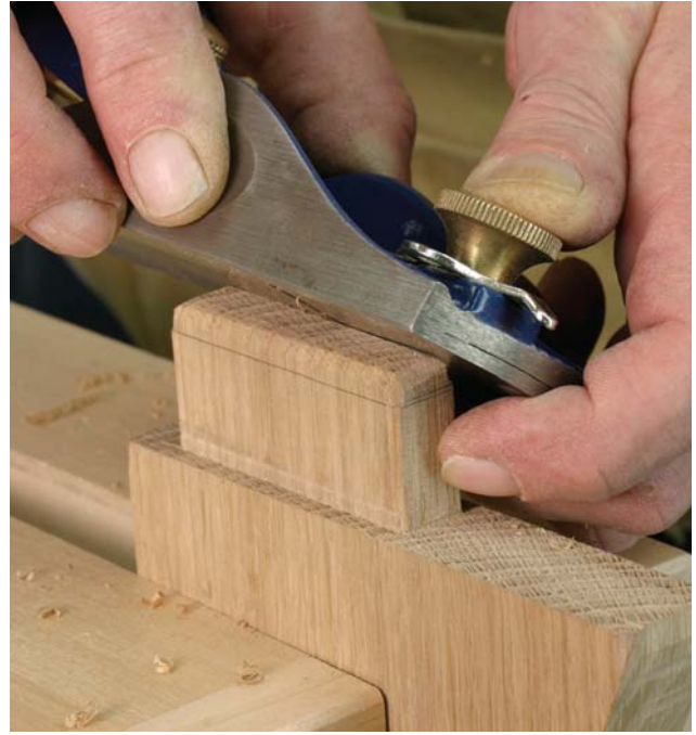
After the tenons are trimmed to fit with a shoulder plane and scraper, the exposed ends are rounded with a block plane.
