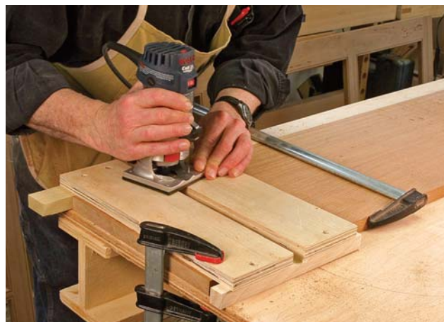
This dado jig is made to fit the thickness of the shelves, and utilizes a flush-cutting bit with the bearing on top.
