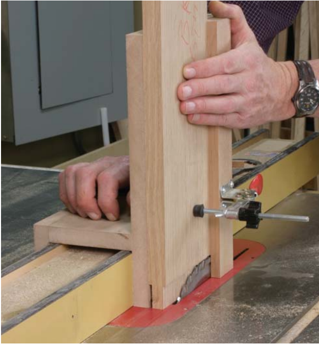
The long mortises on the ends of the rails are cut with this tenoning jig that rides along the table saw fence.
