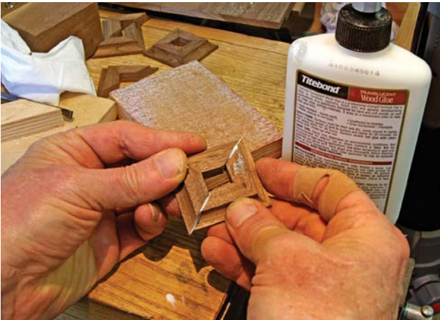
Each half of a foot is put together, then two pairs are assembled to fit the tenons on the ends of the legs.
