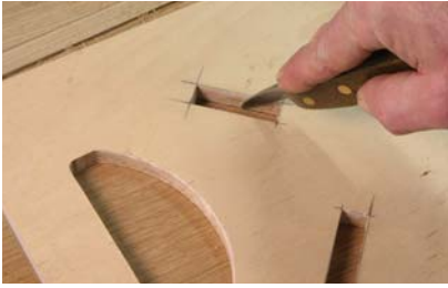
Prevent tear-out by scoring around the openings before cutting with the router.
