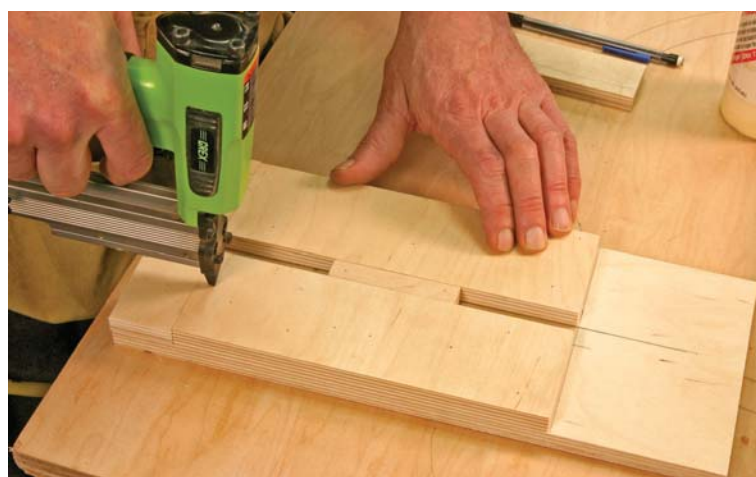
This jig for the through-mortises is made by assembling small pieces to a backer. The openings are then cut with a router and a locating fence is added.
