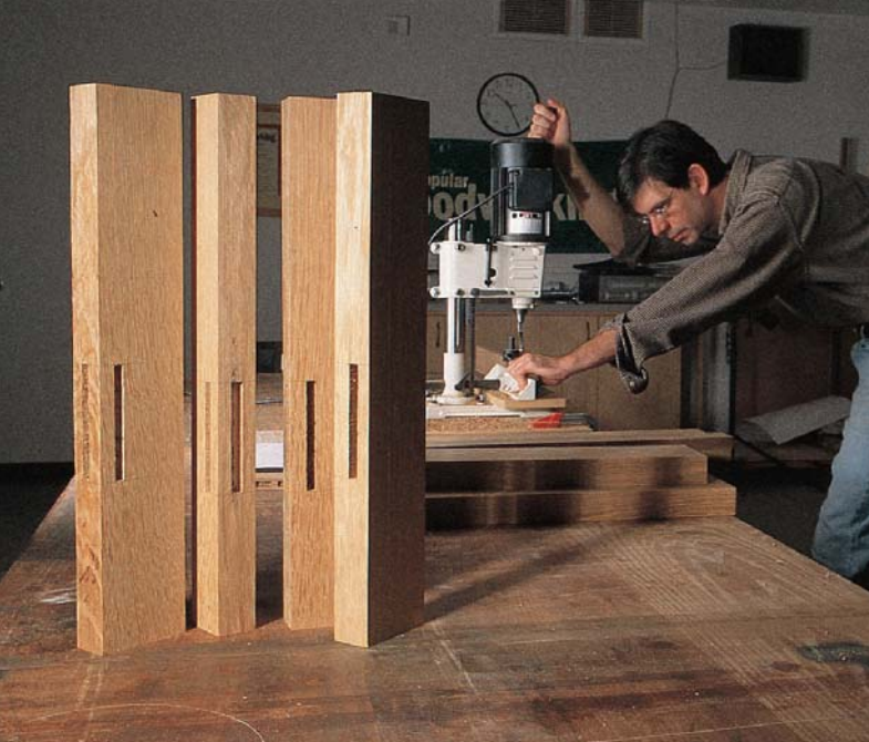
Mortises (made using a mortiser, left) and tenons (as shown being made on the table saw, above), create the mortise-and-tenon joint that is a staple in Arts & Crafts furniture.
