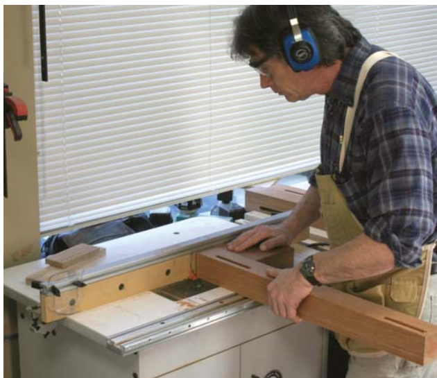
Just a portion of a 2"-radius roundover bit shapes the bottoms of the legs.
