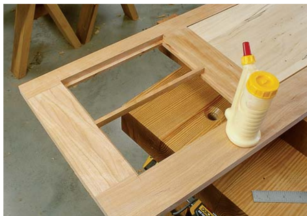
Glue one backing strip into the rabbet in the door on edge. Then flip the door over and glue a mullion onto the backing strip. Then use spring clamps to hold everything while the glue dries.
