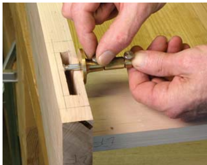
Setting the marking gauge directly to the edge of the mortise ensures exact alignment of the rail and leg.
