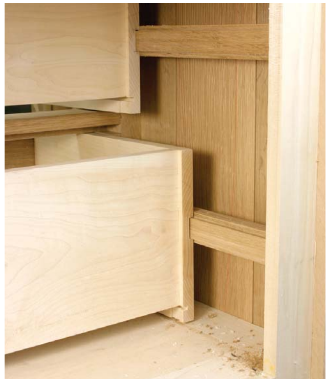
The back of the drawer runner is screwed to the back leg after being squared to the front of the cabinet. A groove in the side of the drawer box lets the drawers slide nicely.
