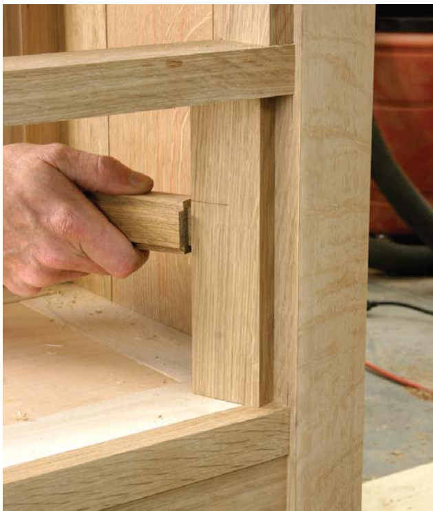
The drawer runners have a tenon on the front end that fits in a mortise in the stile. These are placed in position before the stile is glued in place.
