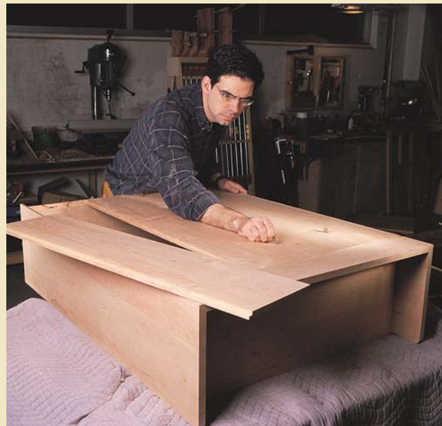
Shiplapped backs allow for solid wood movement.
