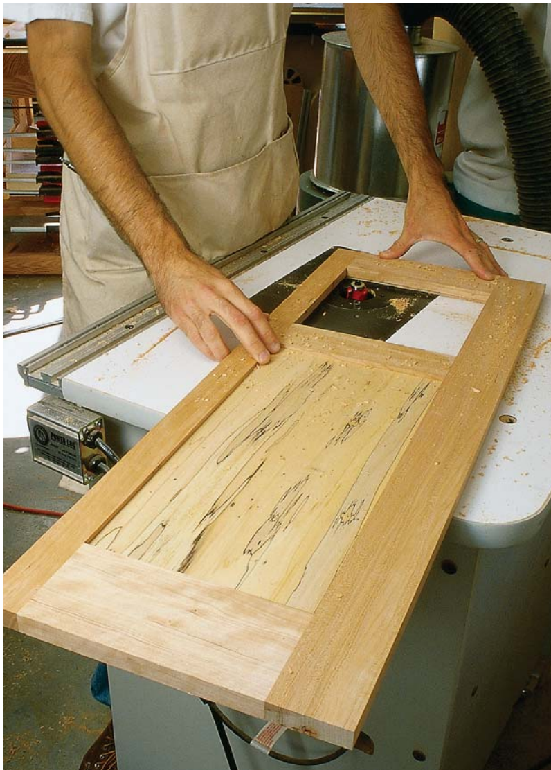
Cut the rabbet on the backside of the door using a rabbeting bit in your router table. With a large tabletop such as this, it's simple work.
