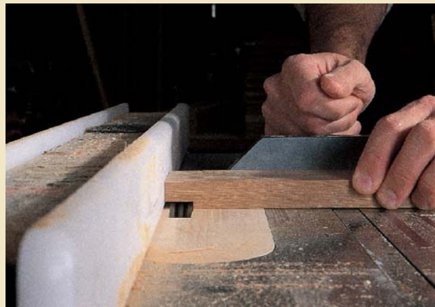
Mortises (made using a mortiser, left) and tenons (as shown being made on the table saw, above), create the mortise-and-tenon joint that is a staple in Arts & Crafts furniture.
