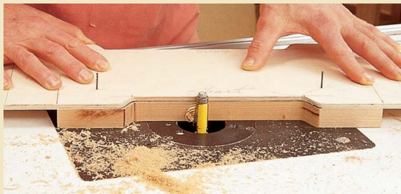
Pattern-routing a cloud lift for a Greene & Greene project.
