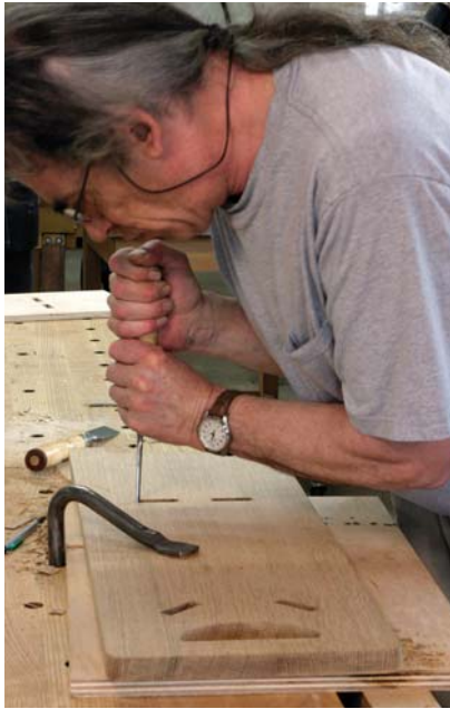
Press the back of the chisel against the mortise wall, then rotate the edge down to the corner to maintain a straight edge.
