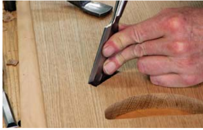
Press the back of the chisel against the mortise wall, then rotate the edge down to the corner to maintain a straight edge.
