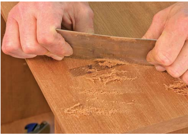
Following the plane, a scraper is used to smooth the exposed tenon ends and the cabinet sides.
