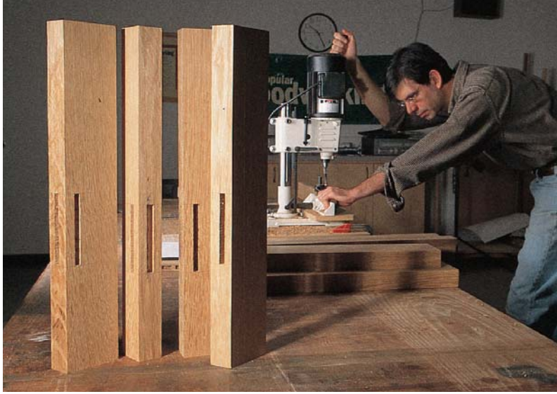
Make the mortises in the legs before you shape the curve near the bottom or make cutouts on the top.
