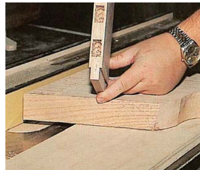
A featherboard provides stability and safety while cutting the tenons.
