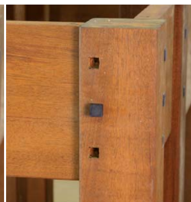
A small, flat riffler is used to clean up the edges of the square holes. A slight chamfer on the back of the oversized square plugs gets them started in the holes before they are driven home with a dead-blow mallet.
