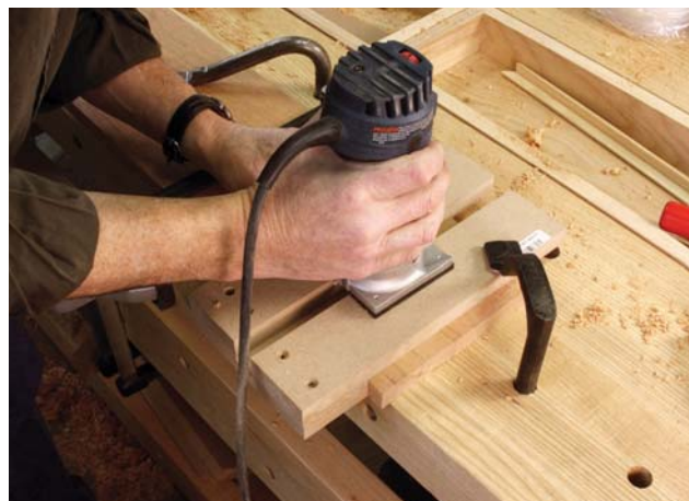
A pencil mark indicates the end of the dado, and because the router will leave rounded ends, I stop just short of the mark.
