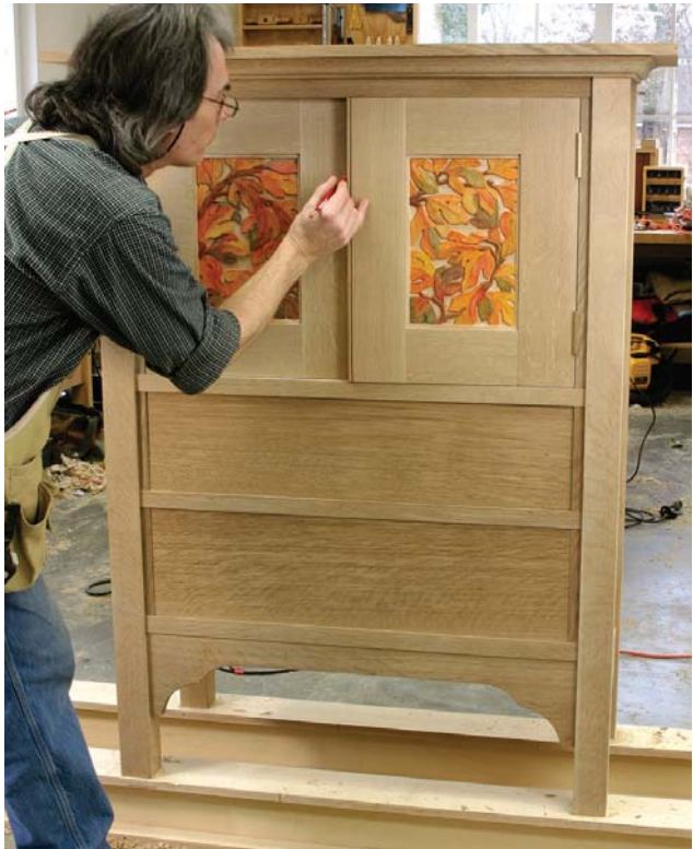
The drawers and drawer fronts are fit before finishing the cabinet. After hanging the doors, I mark where the right door overlaps the left before cutting the rabbet.
