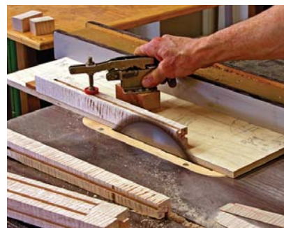
This jig takes only a few minutes to assemble, and provides a safe method to taper the legs at the table saw.
