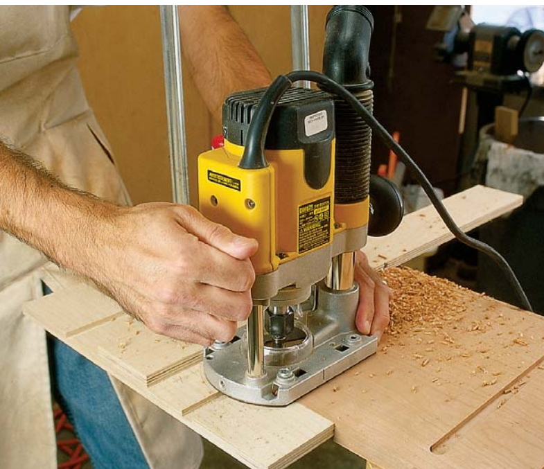
The shop-made T-square jig and a plunge router make quick work of the dados.
