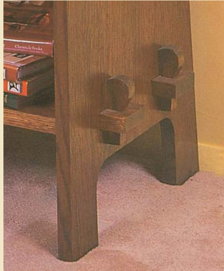
Through-mortise and wedged tenon.
