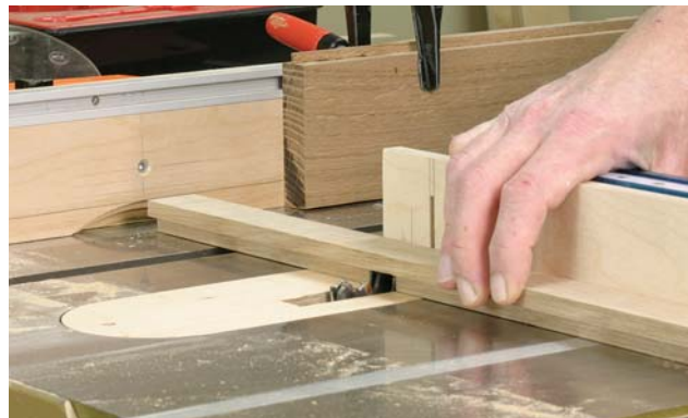
The half-lap joints, as well as all of the tenons for the door, were cut with the dado head on the table saw as you can see here. The block clamped to the saw's fence locates the cuts without trapping the parts between the dado cutter and the fence.
