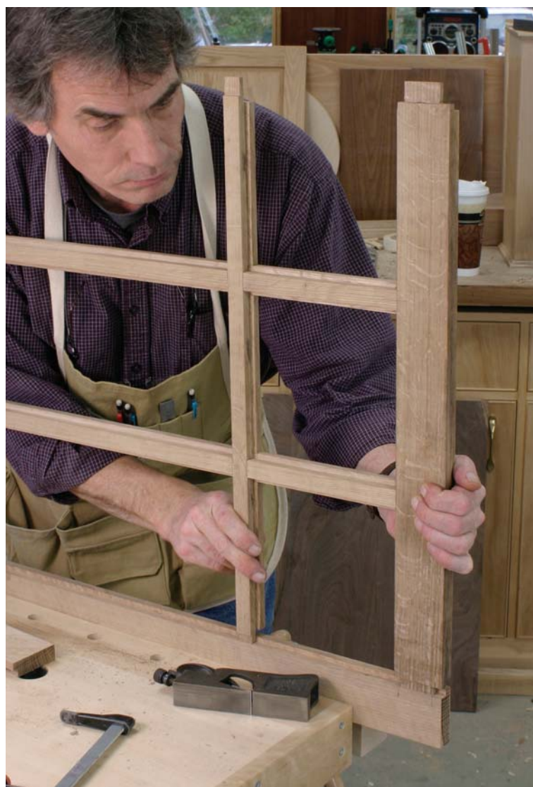
I assemble the door in stages. Here I'm placing a subassembly of the intermediate stiles and rail to one of the door stiles. The remaining stile will be placed on top and clamped.
