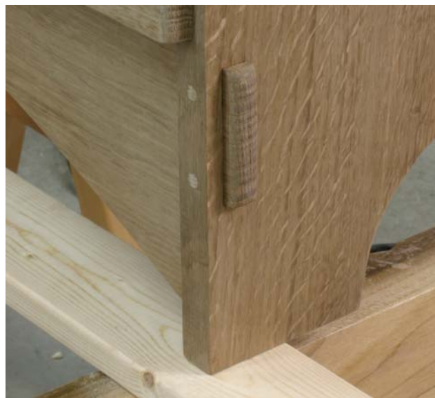
After exposure to ammonia fumes for 24 hours, the oak has turned a grayish brown color.
