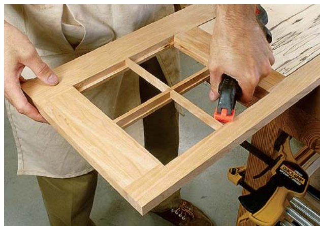
Install the horizontal muntins the same way. First glue a backing strip into the rabbet on the backside of the door. Then flip the door over and glue the muntin to that.
