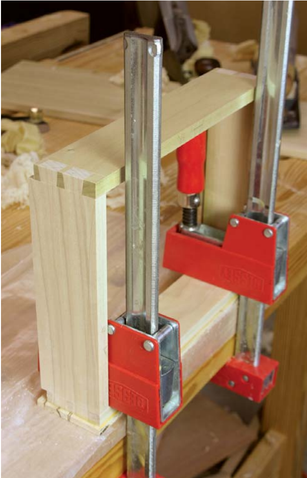
Build the drawers with through-dovetails. Then glue a piece of 1/4"-thick veneer to the front.
