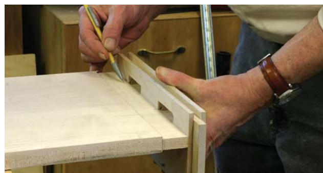
Marking the tenons directly from the mortises is faster and far more accurate than measuring.
