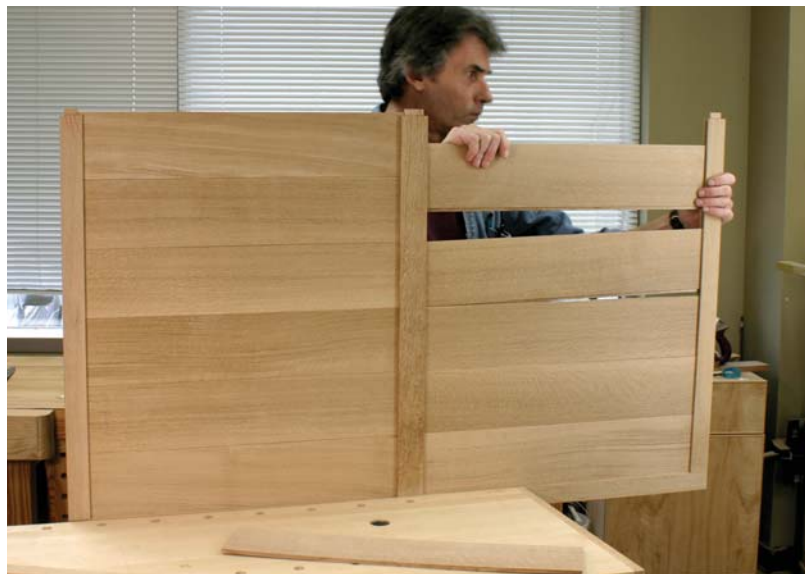
With the rails already glued to one stile, the shiplapped boards for the back panel are slipped into the groove in the rail. When they were all in place, I glued on the remaining stile.
