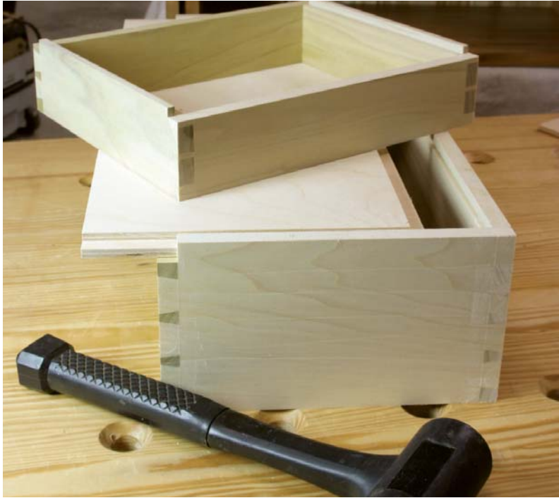
Here you can see the two different ways of installing the drawer bottoms. The bottom in the top drawer rests in a rabbet in the sides. The drawer bottom for the larger drawers slides into a groove.
