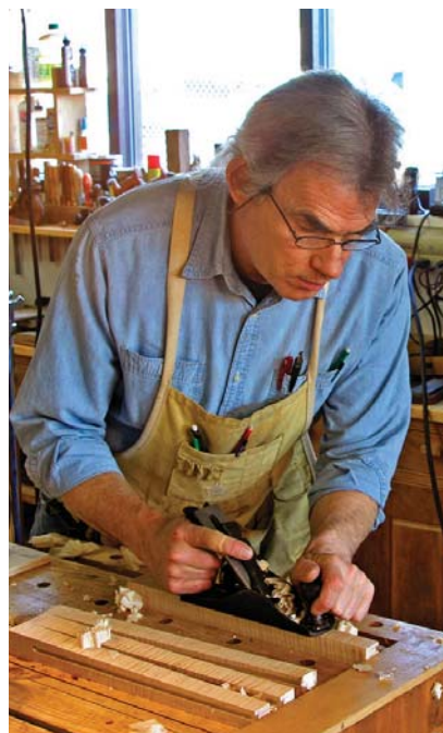
A handplane quickly removes the machine marks from the columns and it leaves a flat, smooth surface.
