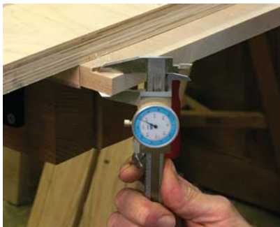
Measuring with calipers reveals the exact thickness of the tenon and how far to set the depth of the router bit.
