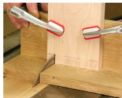
Place the pencil line next to the kerf in the guide to cut just inside the line.
