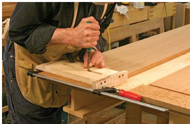
After routing, the mortising jig also serves as a guide for the chisel to square the corners of the through-mortises.
