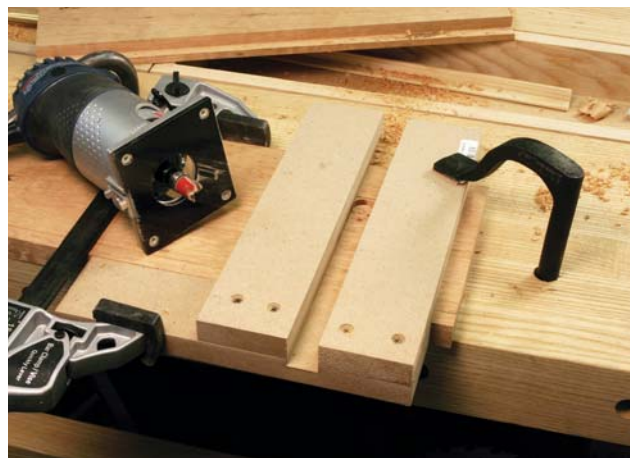
The dado-routing jig is made by clamping the two guide rails on either side of a shelf. The top-mounted bearing on the router bit then cuts the proper-width dado without measuring or fussing.
