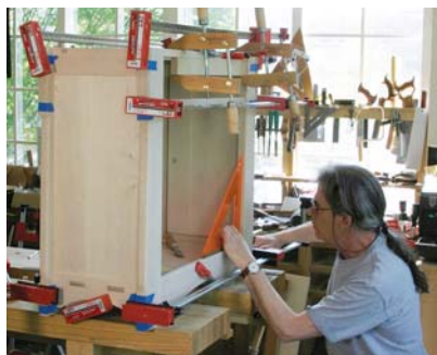
Start all the mortises and get the parts close with a rubber mallet. A few clamps close the joints side to side.
