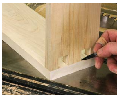
After cutting the first set of fingers, place the end of a side on the drawer front to mark the matching parts of the joint.
