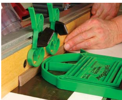
The first cut of the cornice moulding is made with the wood on edge.
