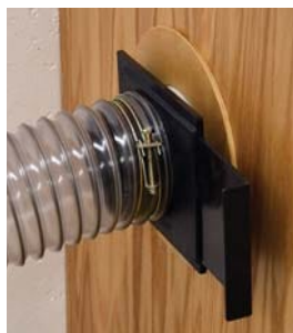
LEFT A 4" hose leads from the Large CO 2 engraver to the blast gate on a base cabinet in the work center.
