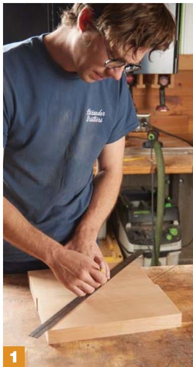
1 The seat starts by marking the center. Using a straight edge, cross the corners to locate the center.
