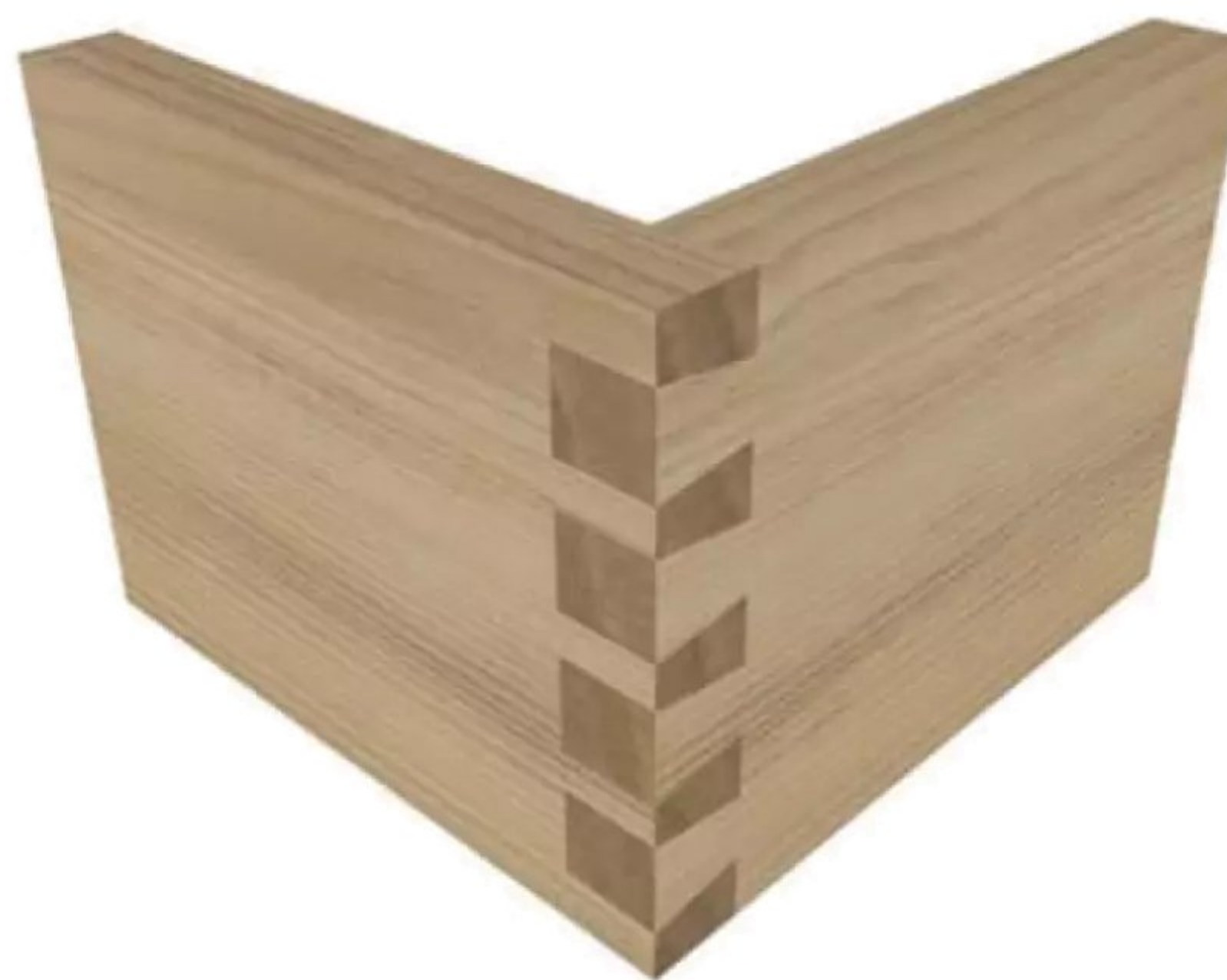
A rendering of a through dovetail. Even stronger than a box joint, a dovetail takes advantage of wedge-shaped joinery to provide a mechanical lock – the glue is just insurance here. Use when strength is absolutely necessary, or when you just want a very attractive looking joint that shows off your woodworking skills.
