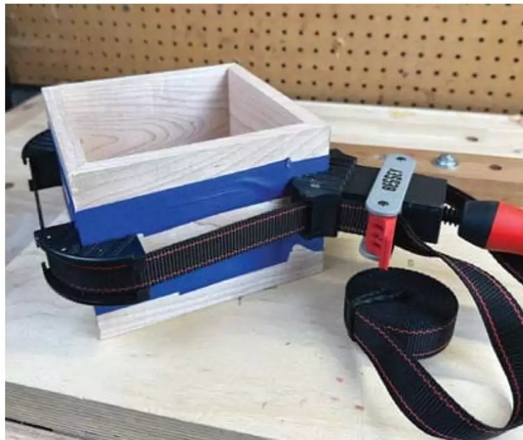
One method for securing miters during glue-up is to use a strap clamp.
