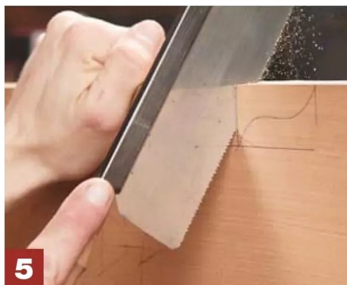
5 Define the ends of the chamfer with a hand saw.
