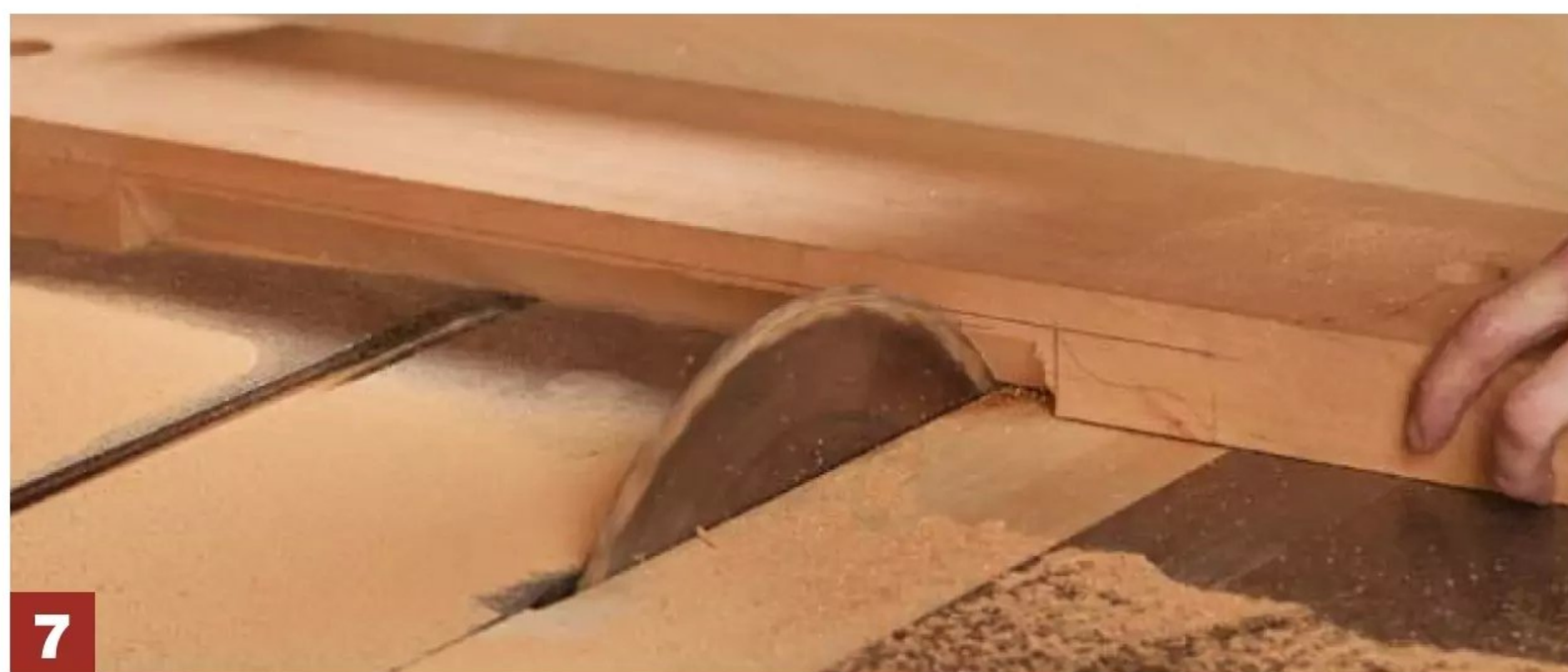
6-7 Wasting away the chamfer is done at the table saw. You'll set the blade to the appropriate height, then slide the workpiece left and right to nibble away the waste in several steps. This leaves a small "hollow ground" chamfer that is easy to clean up with hand tools.
