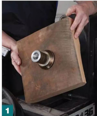
1 Mount the blank on a screw chuck.
