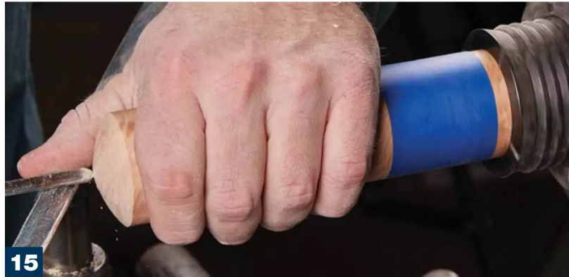
15 Dome over the top of the lid. Blue painter's tape holds the two halves together as you make this cut.
