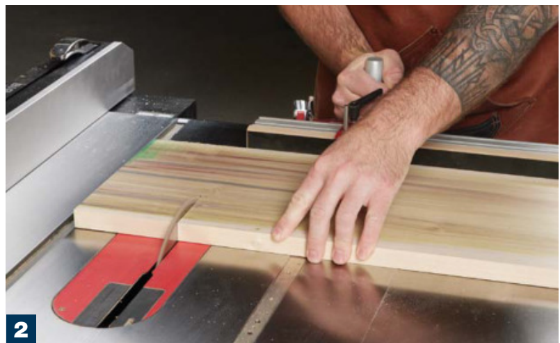
1-2 Start this saw till off by breaking stock down for the sides. Poplar is available in wide boards, but you could glue up stock if you need to.
