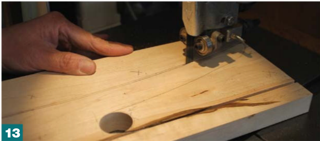
13 Mark two lines and shoot between them, making it less likely to drift past the waste line.
