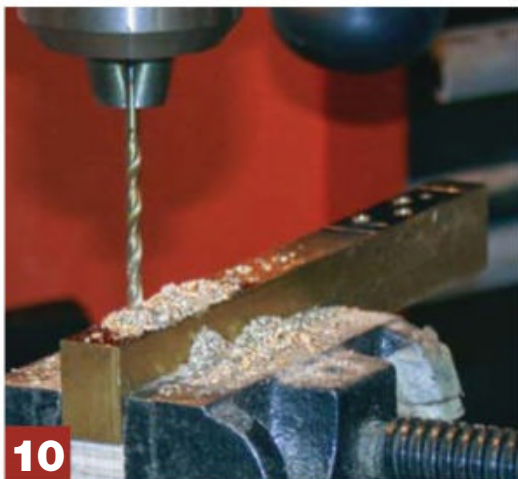
10 Drill the small cross-holes.
