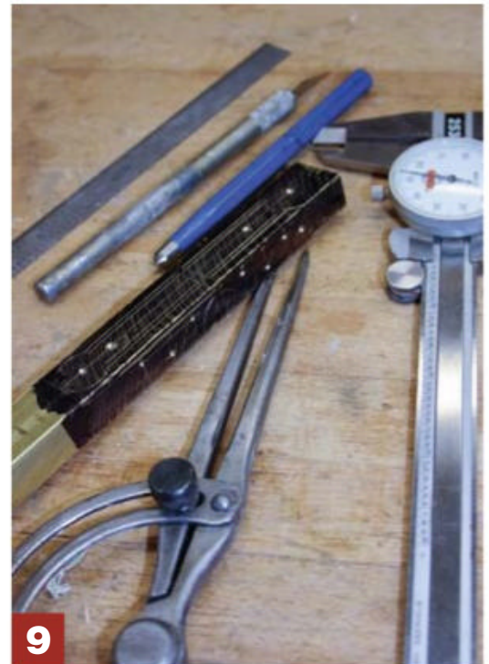
9 Mark the bracket holes and the profile. Using layout fluid or a marker increases visibility.
