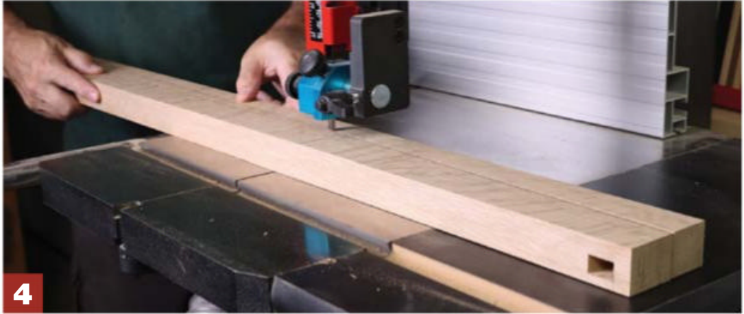
4 Bandsaw close to your line to establish the basic shape of the tapered leg. Cut the long and short inner taper.
