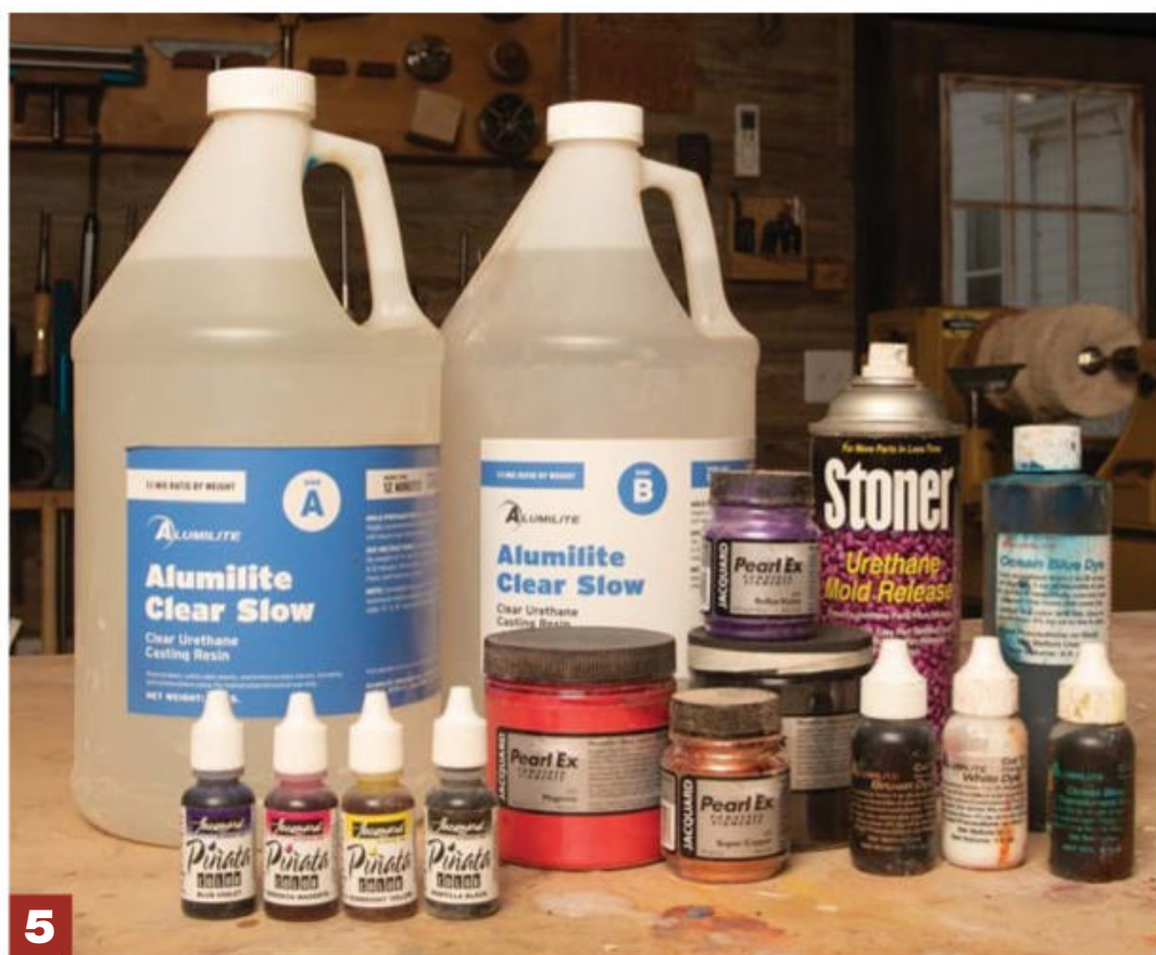
5 Alumilite Clear Slow is my resin for choice in turning, and is measured 1:1 by weight.
