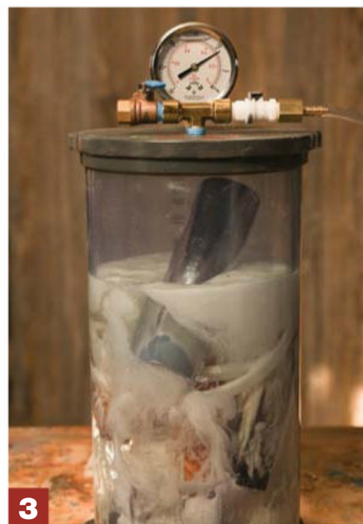
2-3 The vacuum chamber removes the air from the wood so the stabilizing resin can penetrate. Glass Vac (left) and TurnTex JuiceProof (right) are two commonly used vacuum chambers.
