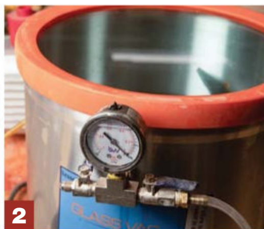
2-3 The vacuum chamber removes the air from the wood so the stabilizing resin can penetrate. Glass Vac (left) and TurnTex JuiceProof (right) are two commonly used vacuum chambers.
