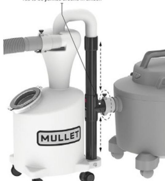
Rigid PVC connection to vac allow M5 and vac to be yanked around in unison
