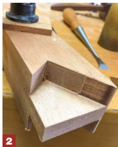
1 A template for the bird's mouth. Once I dialed in the exact angles, this template helped me mark out and cut the joint on the six rafters.
