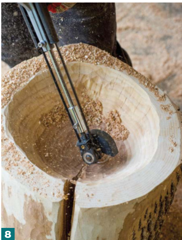
8-9 The multicutter with extension arm on an angle grinder is used to hollow out base of table.
