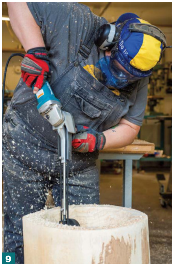
8-9 The multicutter with extension arm on an angle grinder is used to hollow out base of table.
