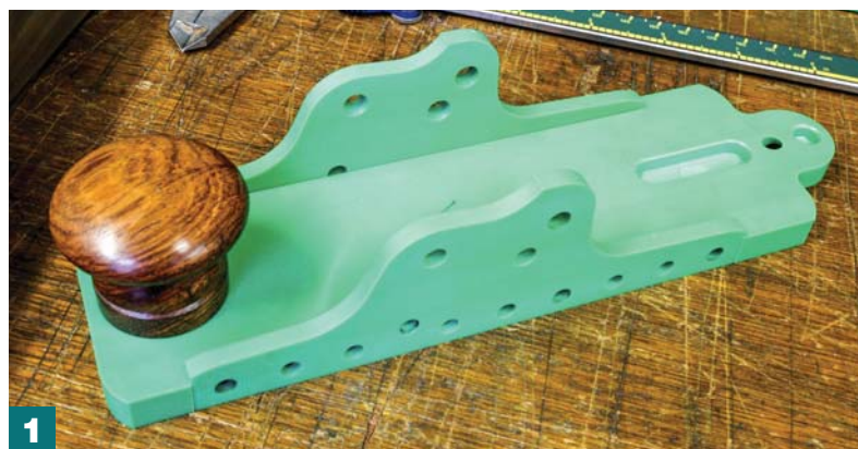
1 Plastic prototype for the 985 smoothing plane.
