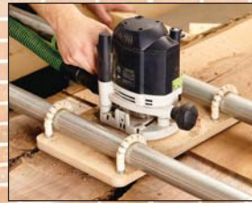
Hardware assembles easily on plywood pieces.
