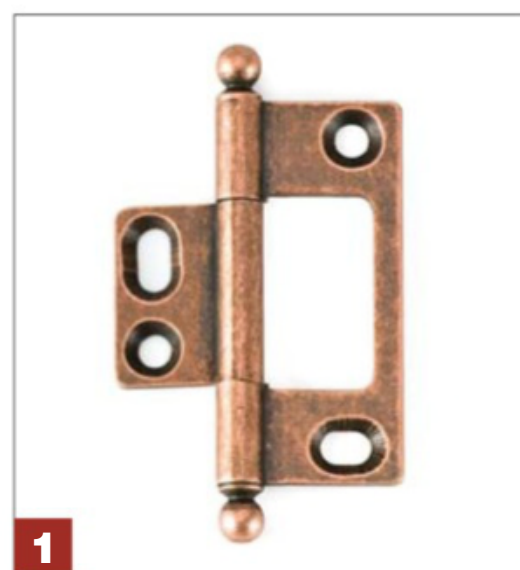
1 The elongated mounting holes in this non-mortised hinge give some adjustability after installation.
