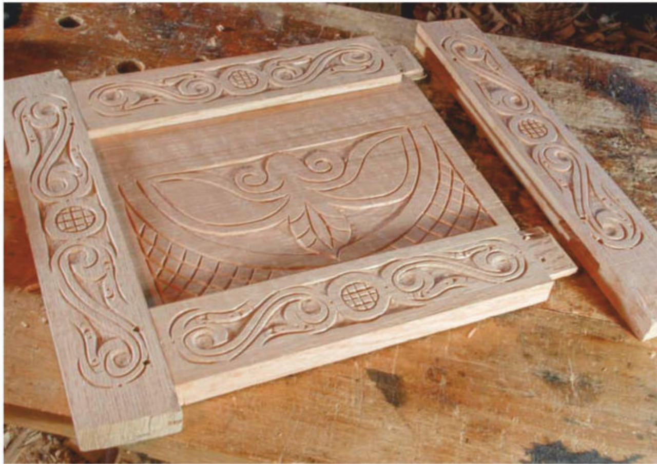
This partially assembled door shows its tell-tale components: the mortise-and-tenon joints, with a panel groove running along the stile.
