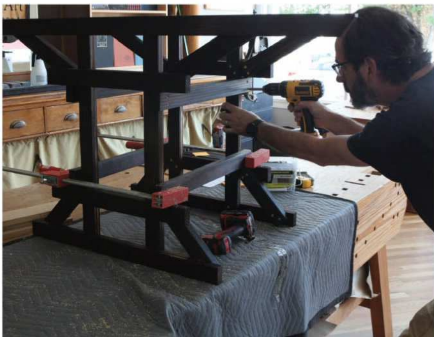
That escalated quickly. The base comes together fast when you screw the four horizontal braces (D) in place. If you don't have clamps, a helper can do that work as you drive in the screws.
