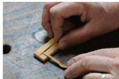
Weave. Start the weaver under one part of the slit section. Wrap it over the next part, then push it in tight to the bottom end of the sheath.
