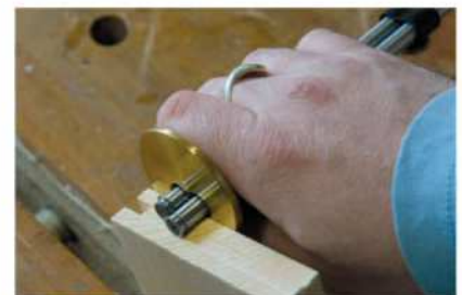
In the groove. Layout the tenons with a marking gauge set to the dimensions of the groove.
