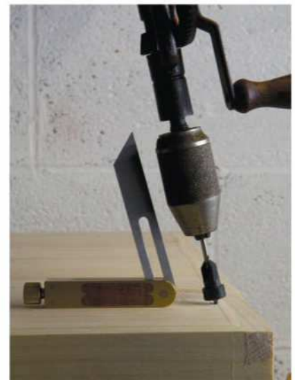
Drill reference. A small bevel helps to sight the angle the pilot hole for the cut nails on the backboards.
