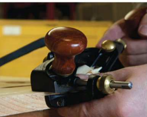
Rabbets by hand. A rabbet or moving fillister plane makes quick work of the rabbets for the casework.
