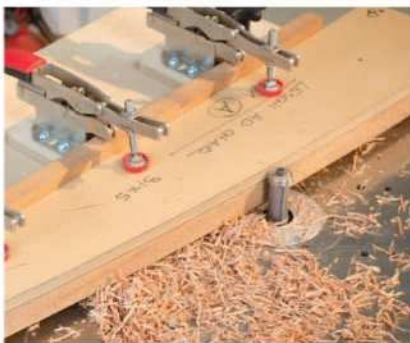
Route with a top-bearing bit. A router table, a simple jig and a straight bit with a top bearing are all that's needed to safely route your pieces to size with patterns.
