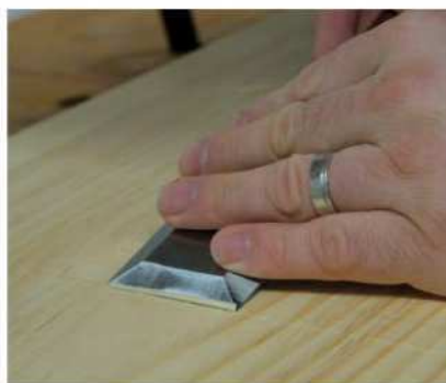
Saw guide. For a first-class saw cut, pare a channel into your knife line to guide the saw.
