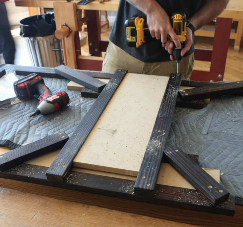
Spacers at work. The MDF spacer jigs allow you to line all your parts up without a lot of measuring. Mostly you are ensuring all the parts are centered on the legs.
