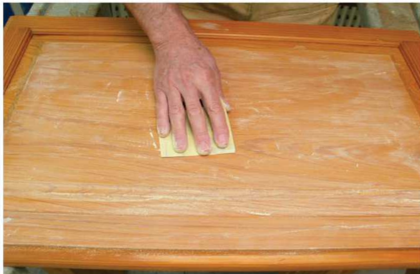
Sanding sealers. These are available for alkyd varnish and lacquer for the purpose of speeding production because these finishes gum up sandpaper; sanding sealer powders when sanded. To understand this product, put the emphasis on "sanding," not on "sealer."
