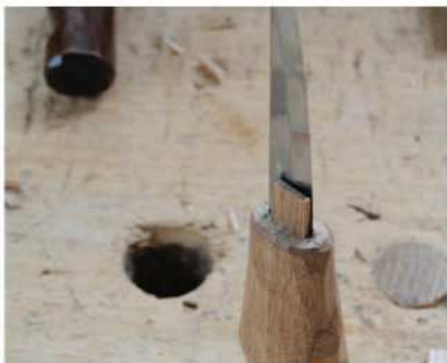
No glue required. I don't bother gluing the blade into the handle, nor the wedges, but gluing won't hurt. The bevel around the handle's end is carefully cut with the tip of a slöyd knife.
