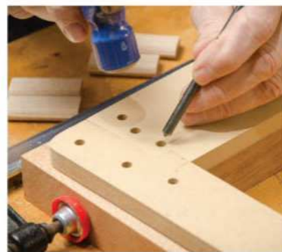
With a tap and a .250" machinist center punch, locations for holes and plugs are transferred through the pattern holes.
