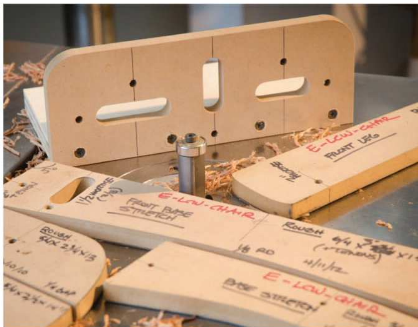
Taking it one more step. Sometimes I add router joinery templates right into my patterns. I mill \frac{5}{8} " router bushing slots at joinery locations.
