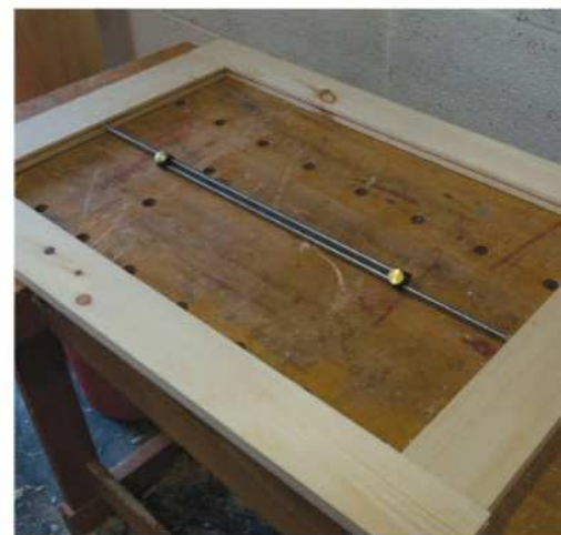
Make middle stile to fit. A bar gauge measures the internal length of the frame for the middle stile.
