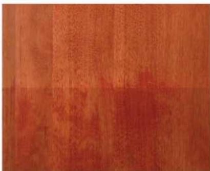
Washcoat. A washcoat is a highly thinned finish applied to blotch-prone woods (see top half of birch panel above) to partially seal the pores to reduce the blotching. A washcoat can be made from any finish. Wood conditioner is a washcoat made by thinning oil or varnish. The trick for having success with it is to let it dry thoroughly before applying a stain.
