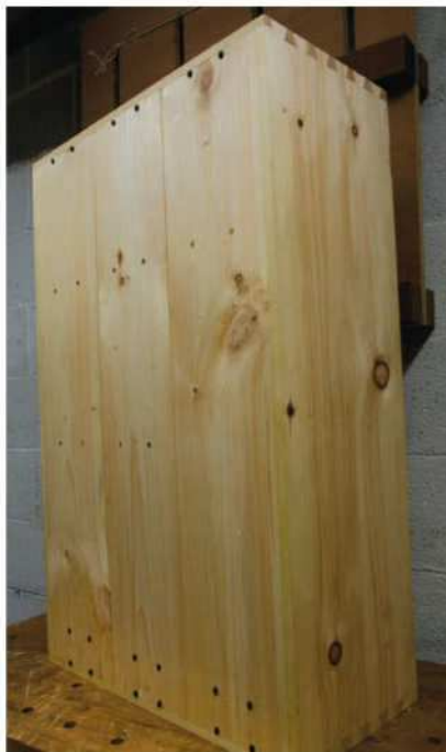
Cut nails. You can see the three rows of cut nails securing the backboards and the brass screws holding the kerfed blocks.
