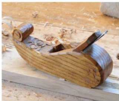
An ash plane. This little plane is based on Dutch examples from the late 17th-18th centuries. It's about 9" long and 2 1/4" wide.
