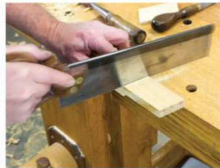
Lay out the shoulders. A crosscut-filed backsaw takes care of the shoulder cuts.
