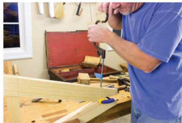
Join the legs. Use a \frac{1}{4} " drill centered in the auger hole; stop drilling when it just starts in the opposite leg. Just the one screw is all that is needed to secure the tops of the legs together.
