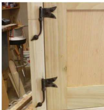
Needs adjustment. Any adjustments mean redrilling holes. Luckily, they'll most likely be covered by the hardware.
