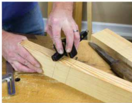
Gauge the mortise. Gauge the mortise width between the pencil marks on the insides and outsides off the legs.
