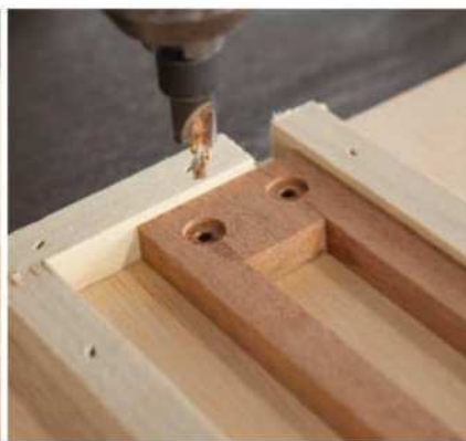
Quick work. The two fences on this jig allow you to slide the center assembly left and right to bore the holes and counterbores exactly \frac{7}{8} " apart.
