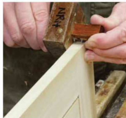
Transfer time. Set a mortise gauge to the width of the leaf and scribe the leaf width onto the door.
