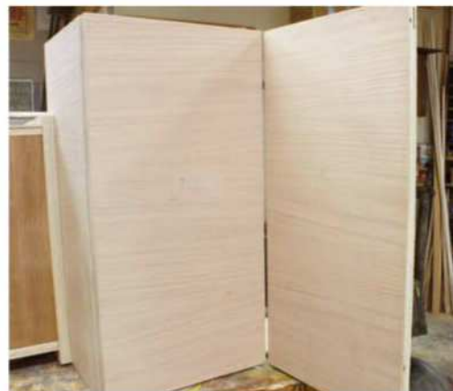
Mind the gap. You can adjust the gap between the doors by turning the adjustment screws. The vertical slot on the mounting plate allows for adjustments in height. The other two large screws allow for lateral adjustment and front-to-back tilt.
