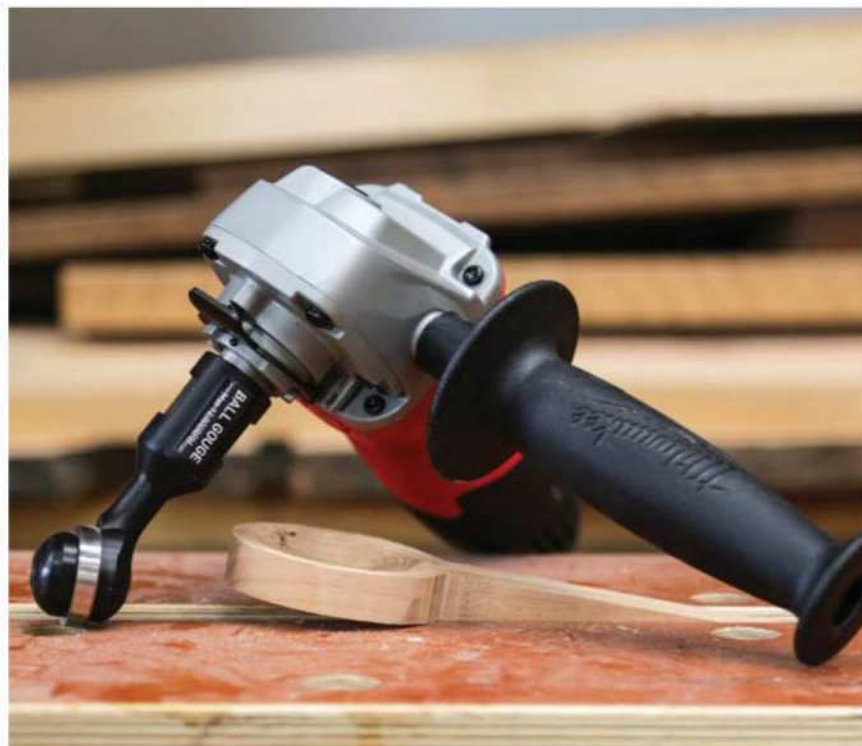
BYO grinder. Arbortech's ball gouge is compatible with most 4" and 4 1 / 2 " grinders with speeds between 9,000 and 12,000 RPM.
