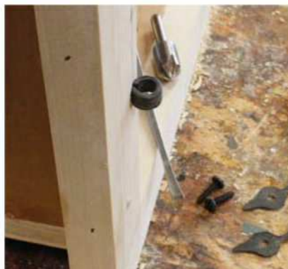
In deep. The eye bolt may need to be let into the face of the cabinet so the tail will lie flush.
