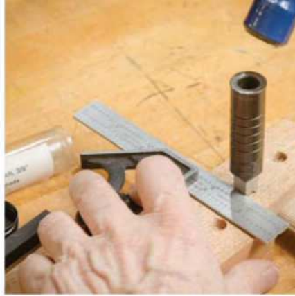
Hand-powered mortiser. If you don't have a hollow chisel mortiser, Lee Valley makes a square punch that works well. Use the punch to define the outside of the mortise and drill out the waste.
