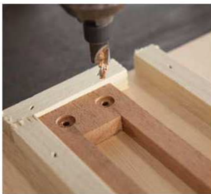
Quick work. The two fences on this jig allow you to slide the center assembly left and right to bore the holes and counterbores exactly \frac{7}{8} " apart.
