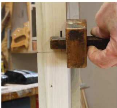
Eye first. Mark the center of the hole for the eye bolt, top and bottom.
