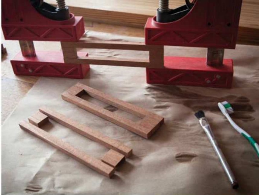
Make a hole. Glue up the rails and stiles of the middle section to create a hole for the kickstand and foot of the project.
