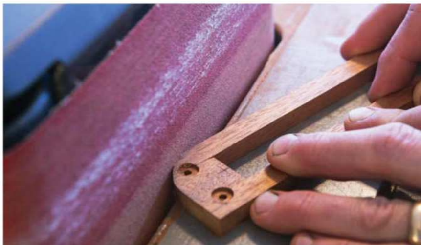
Sand the curve. Mark the \frac{7}{8} "-radius curve on the end of the middle assembly and sand it to shape.
