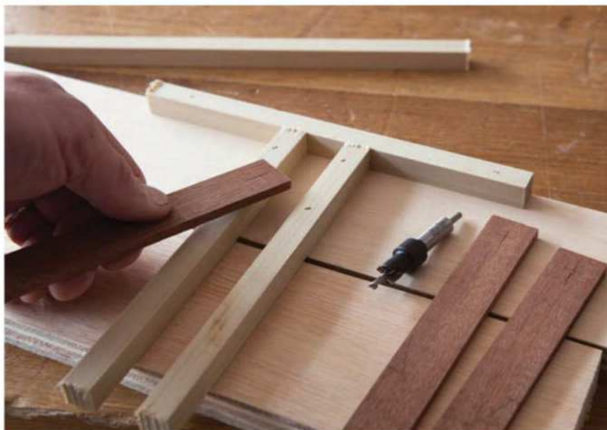
Even simpler. The jig for drilling the holes and counterbores in the rails and stiles is similar to the other jig, but the workpiece doesn't slide.
