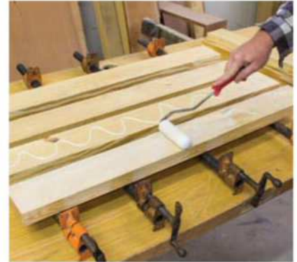
Glue it up. A small foam roller works well for spreading the glue evenly and quickly.
