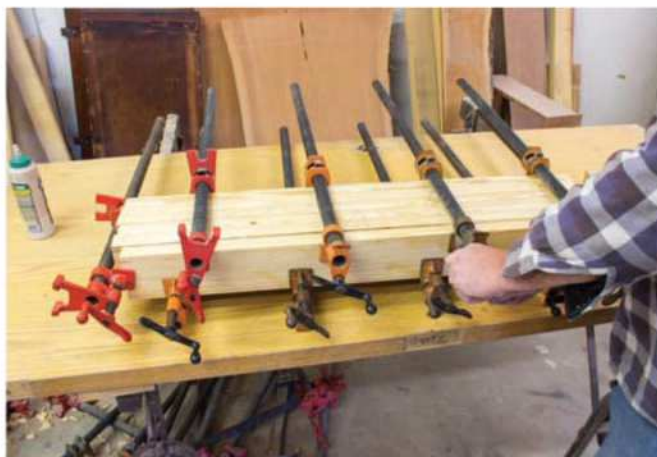
Clamp the beams together. Clamp both beams at once. I also have a scrap piece on the outside of the stack to prevent the clamps from damaging the beam surfaces.
