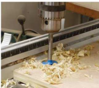
Press. A drill press is handy for drilling the hinge cup holes. The edge of the hole should be \frac{1}{8} " in from the hinge stile's edge.
