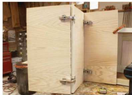
All set. The secondary door is attached by means of the bi-fold mounting plate.
