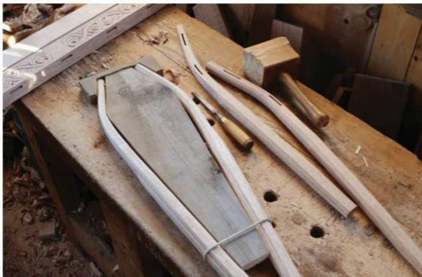
A great use for fast-growing oak. Rear posts for ladderback chairs, some in the bending form, others just mortised for the slats. These posts are 1 1/4" in diameter and have about 6 growth rings.
