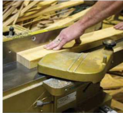
Square your stock. A powered jointer makes for fast work flattening stock.
