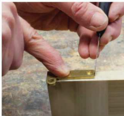
First mark. With the pivot end flush to the edge of the stile, mark the location of the other end using a knife. Also mark the edge of the pivot knuckle. Remove the hinge and scribe a square line across the edge of the door at both points.
