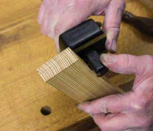
Tenon width. Set your gauge teeth to the width of your mortise chisel.
