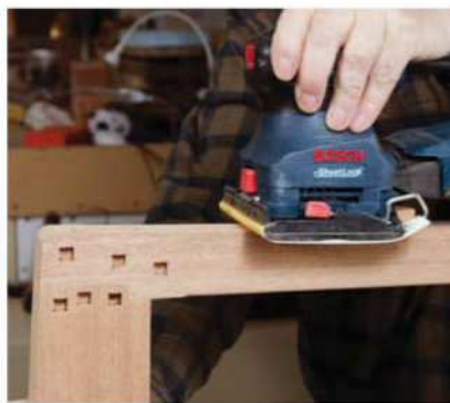
Detail work. Clean up the edges of the mirror by hand with scrapers or sanders. An edge sander or belt sander comes in handy for blending the sides and top of the mirror.
