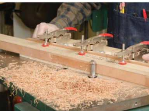
Start shaping. Shape your parts on a router table or shaper. You can also use the patterns to guide your handwork if you'd rather shape the parts by hand.
