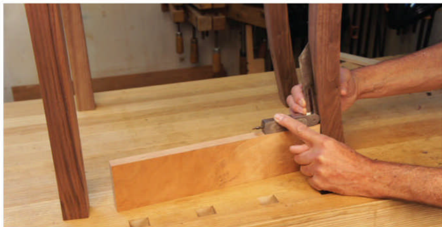
Double angles. To make things interesting, the back of the side stretcher has a compound angle. This gives you the secondary angle you need.
