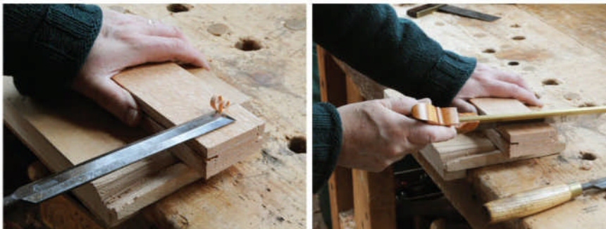
Full tilt. The sawn angle of the front angle is tricky – a chiseled trench guides the saw. Get close to the correct angle, but tune up the fit by planing the rail to fit.
