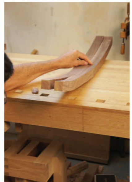
Are you flat? Check that the flats on the two legs are the same by placing the legs with the planed flats on a flat surface. The tops of the legs should be the same height off the surface. The leg bottoms don't matter as much.
