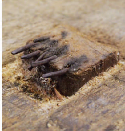
The lockjaw stop. This French bench uses rusty nails to secure the work. I have yet to cut myself on a metal planing stop during the last 12 years. So, this looks worse than it really is.
