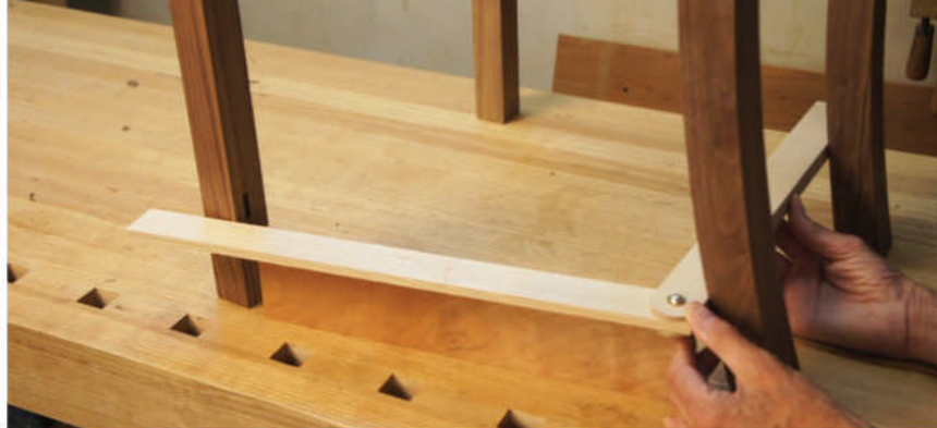
Quick-&-dirty layout tool. The angle for the slat stretcher is different than that for the side rail. An improvised shop-made bevel gauge is an easy way to figure out this angle.
