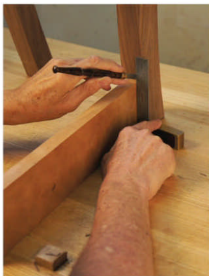
Flat to the floor. The layout in the back legs for the two side stretchers should be perpendicular to the floor, not parallel to the legs.
