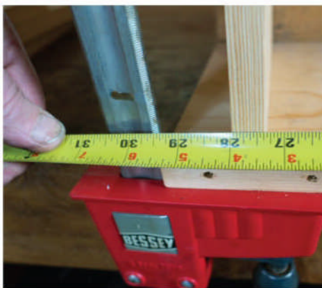
Tricky division? I want eight equal drawers, so if the opening is a light 27\frac{3}{8} ", how big should each drawer be?
