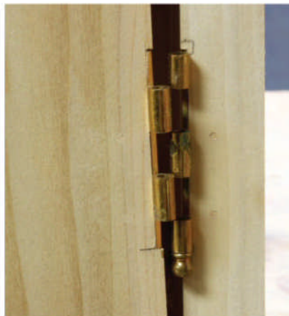
Sliding home. Place the door so that the hinge leaves fit together, then drop in the pins.
