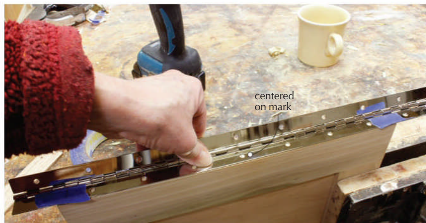
On center. The center of the door's length is marked in pencil and the hinge is positioned so that its center hole falls over that line.
