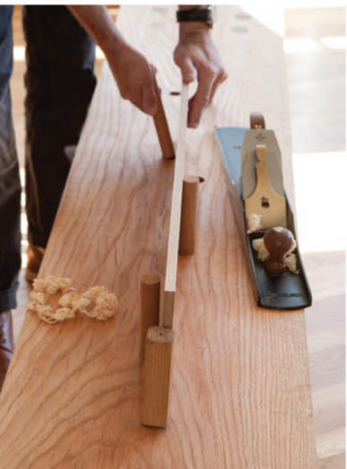
I've got this pegged. By having a selection of pegs that vary in length and girth you'll find it easy to secure most boards on the benchtop.
