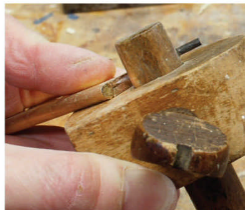
Revealing. Fixed-pin, non-swaged butts will be let into the door with the cabinet-side leaf protruding by the amount of your desired gap around the door, so I am setting the gauge shy of the barrel's thickness by about \frac{1}{32} ".
