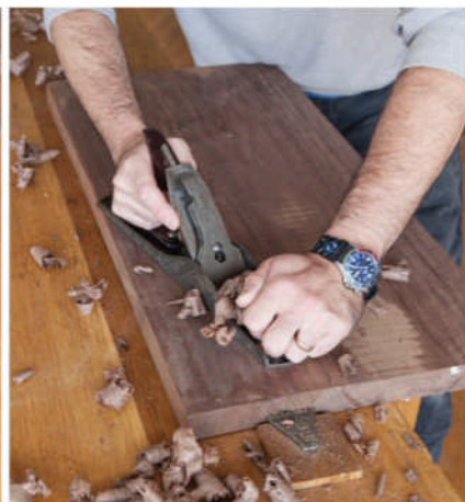
It's in the hip. This is how I typically deal with wide stock. Keep the plane in line with the planing stop and shift the board toward you as you work. When you reach the far edge, use your hip to press the board against the stop. If you have a face vise, move its jaw out to help support the board as well.
