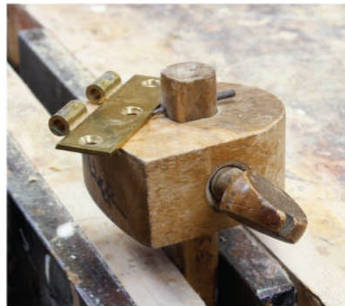
Full depth. The swaged loose-pin hinge is mortised flush with the wood, so set your gauge to the thickness of one leaf.
