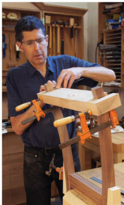
Joinery insurance. Make sure that the shoulders at the tops of the legs are aligned perfectly with a setup like this.
