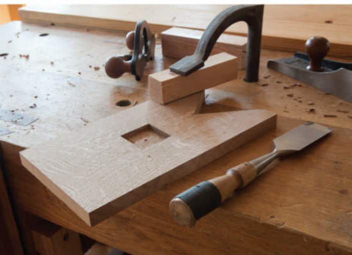
Every little bit helps. This shallow mortise in the underside of the palm helps prevent the palm from coming loose from the planing stop.
