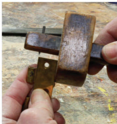
Leaf, no barrel. To lay out the width of a swaged loose-pin hinge mortise, set your gauge to just the width of each leaf.
