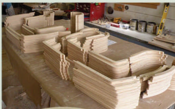
CNC is a new weapon. It takes piles of precisely cut plywood parts to make one Hollow Chair.
