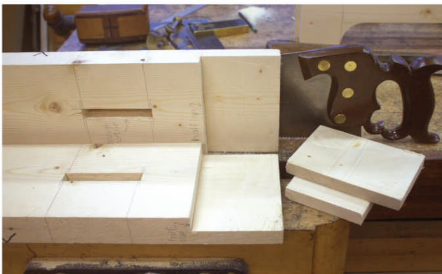
Half-lap tenon. Here's what the finished tenon part of the joint looks like on the ends of the legs.
