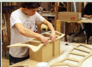
A Little Red Dresser takes shape. Cabinet fronts and backs are routed from a single template. Panels and ribs are glued and nailed in to connect the flat parts and create the curvy sides, which are then covered with bending plywood. Drawers are then hung on the interior ribs using commercial slides, and a pro paint job brings the piece together.
