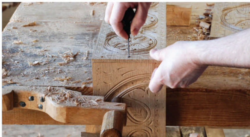
Pin locations. Here I'm working on a standard box (no slanted lid), but the method is the same for marking the bored holes for the square wooden pins.
