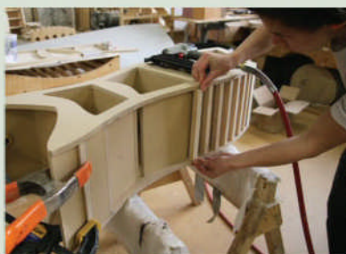
A Little Red Dresser takes shape. Cabinet fronts and backs are routed from a single template. Panels and ribs are glued and nailed in to connect the flat parts and create the curvy sides, which are then covered with bending plywood. Drawers are then hung on the interior ribs using commercial slides, and a pro paint job brings the piece together.
