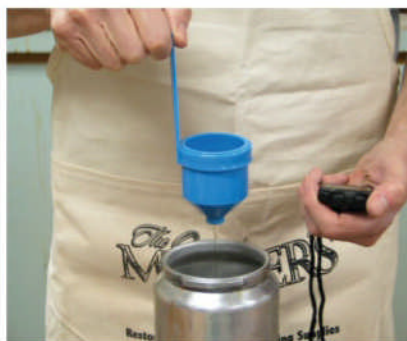
Viscosity cup. Finish manufacturers sometimes supply you with timing guidelines for measuring viscosity, typically using a Zahn #2 or Ford #4 cup. I've never used these cups because the manufacturer is assuming perfect temperature and humidity conditions, which I seldom have. Nevertheless, I'm not saying not to use them.
