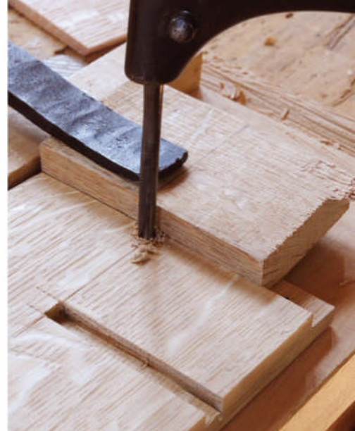
Backtracking saviour. Forgetting to bore this hole before rabbeting means you must clamp some stock in the rabbet so the bit doesn't slip down in there. It's clumsy but manageable.
