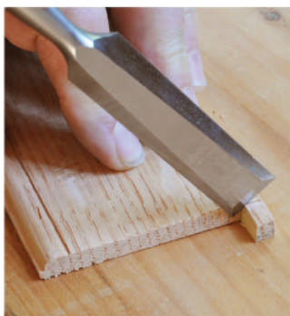
Pintle shoulder. Form a shoulder for shaping the pintle hinge round by pressing a chisel into the corner of the square pintle.
