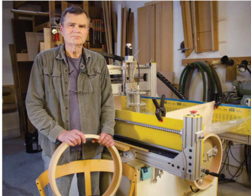
Shop-made. Curtis Erpelding designed and built his four-axis CNC. He uses it to make forms, parts and joinery for his bentwood stacking chairs and stools (among other things).
