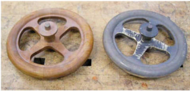
From wood to iron. Jim made wooden patterns for the vise jaws and handwheels (shown here are the handwheels), then had the parts cast in iron and nickel plated before mounting them on his reproduction bench.
