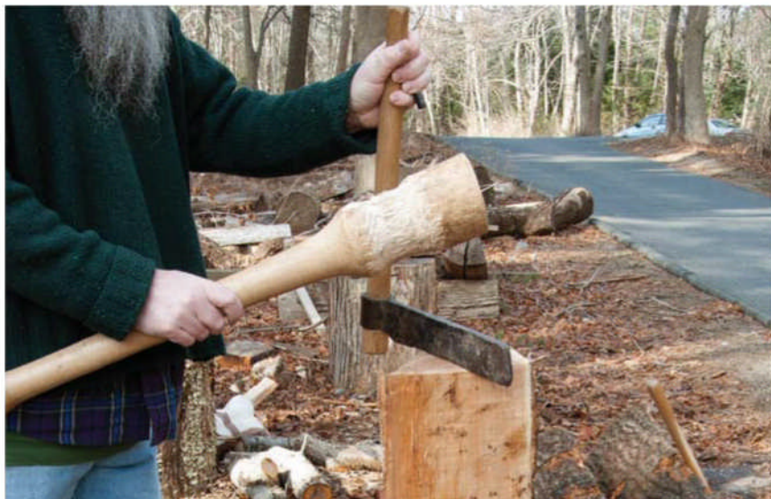
Yin & yang. The froe is an essential green woodworking tool, but it is nothing without its mate, the froe club.
