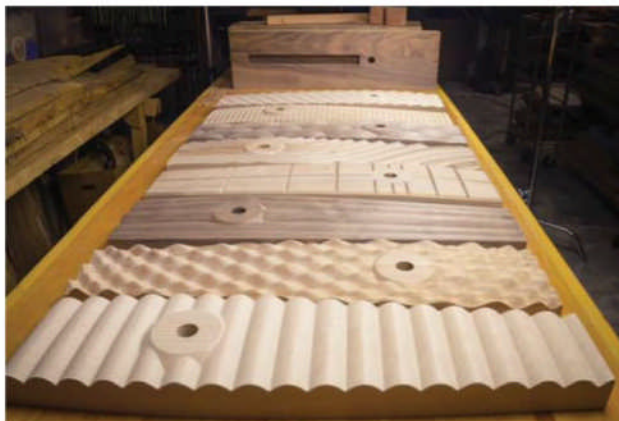
Bench chops. With the help of a CNC, I was able to realize the many different treatments I designed for these chops for leg vises on otherwise traditional Roubo benches that I made for a local wood-working group.
