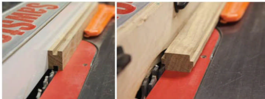
Tongues & grooves. I used a dado stack to cut these joints. When you cut the grooves on the fingers, run the finger through the blades twice – once with one face against the fence and a second time with the other face against the fence. This ensures the groove will be centered. Then cut the tongue to fit that groove.
