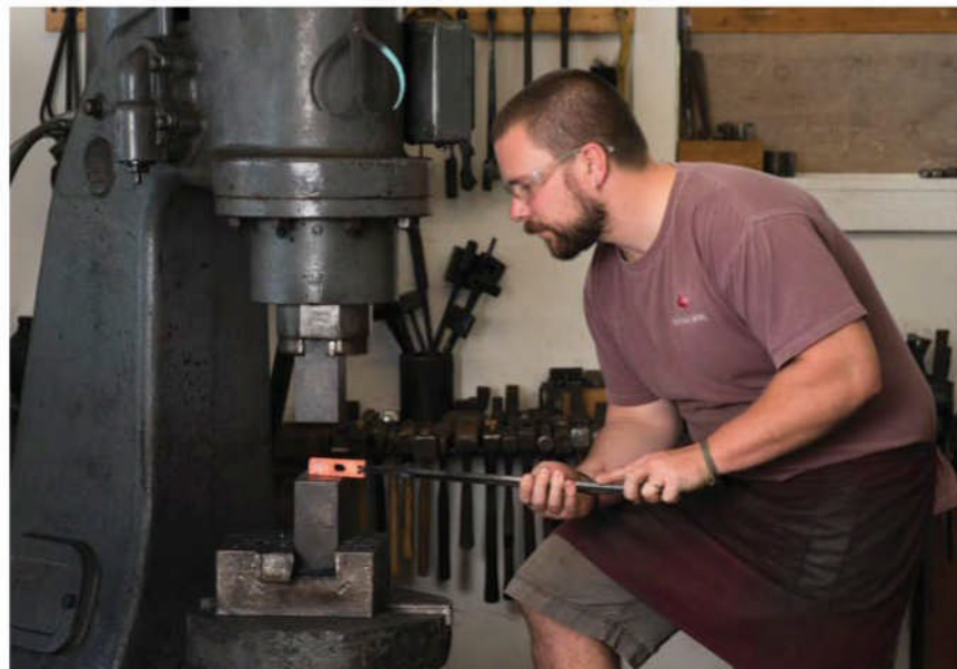
Hard work. Seth Gould is shown here hard at work forging a hammer head. His hammer-making process starts at the forge, followed by hand filing then carefully making wooden handles (you can see a finished hammer on page 4 in the Table of Contents).
