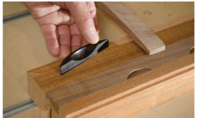
Repeat parts. Making multiples is another efficient CNC job, such as Spangler's ebony drawer pulls.
