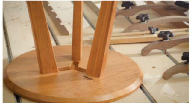
Joints. Spangler uses his CNC for complex joinery, such as this self-locking joint for the legs on a small table
