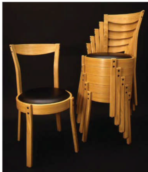
Glueless joinery. Erpelding's CNC innovations include the tight, glueless joinery pieces he makes in maple for his laminated stacking chairs and stools. After he blackens the wood, he fits the legs and pins them tight with brass pins.
