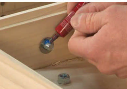
Hardware. Attach the handle with the 1\frac{1}{2} "-long \times \frac{1}{4} "-20 bolts. I'm using Loctite to keep the nuts from loosening – once dry, it acts as a mild glue, but can be reversed with some persuasion.
