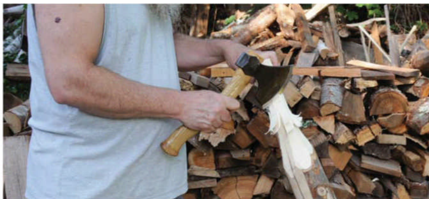
Get a grip. To keep the club from slipping out of my hand, I like to keep some thickness at the bottom end. So I have to flip the club and hew from the end toward the middle. I take great care when hewing this close to my hand.
