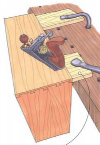
Lazy solution – use holdfasts to secure battens to bench
