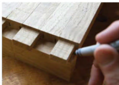
Completed fingers. With the tenons cut, clamp the fingers together and show the assembly to the ends of the frame. Mark the locations of the mortises.
