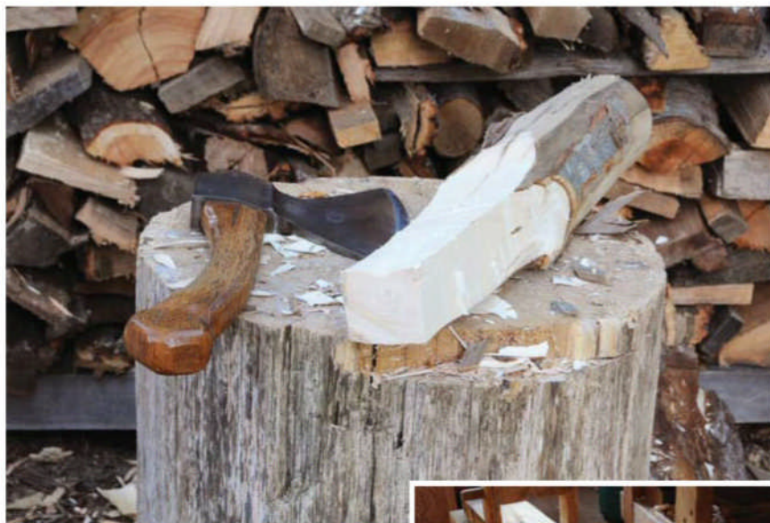
Start square. I'm after a round-ish handle, so I start by making it square, then octagonal, then round.
