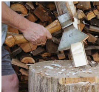
Up then down. When hewing, I start at the bottom, scoring the wood as I work my way up. Then I chop down, breaking off the chips.
