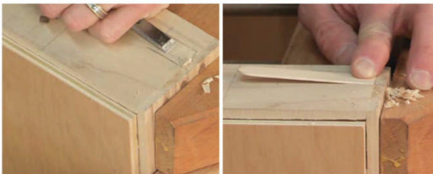
Spring latches. The mortises that hold the spring latches are pared with a chisel held at an angle to form a ramp, which causes them to stand proud. A tongue depressor is just the right size and thickness, but any thin piece of wood will work.
