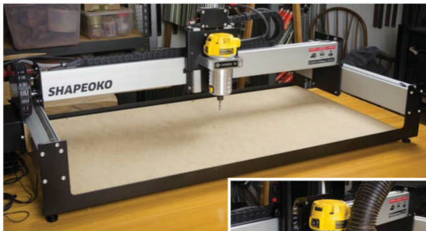
Home-shop CNC. The Shapeoko XL is an easy-to-build CNC option for the home woodworker. At right are shown two key accessories, the XYZ probe for easy setup and the SuckIt dust boot for easy cleanup.
