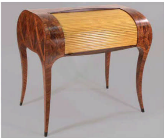
Lady's Desk. This kingwood, satinwood and Gabon ebony roll-top desk made use of digital tools in countless ways, including patterns, bending forms, detailed joinery, unfolded curved veneer patterns and more.
