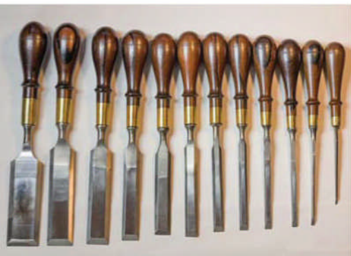
User-modified. Just like Studley's originals, this set of bench chisels has owner-made rosewood handles and ferrules.
