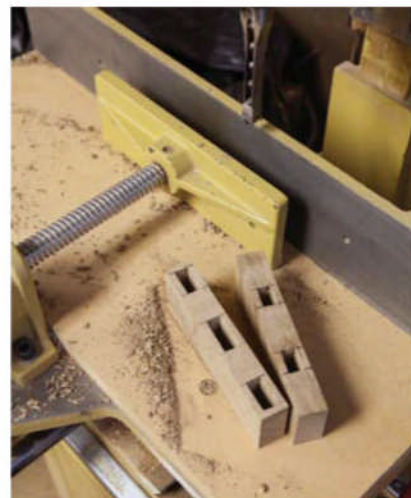
Twice mortised, once fit. To center the mortises, put one face against the fence and cut the joint, then turn the piece 180° with the other face against the fence.
