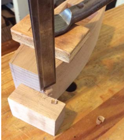
Stop. I use a 1/4"-tall stop-block to achieve chamfer cuts of a consistent depth.
