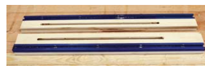
Miter fences. These are mirror images of each other – one for each side of the sled.
