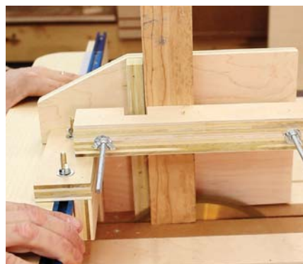
Tenon jig in use. Cut the tenon's cheeks with the jig, then the shoulders on the sled itself.
