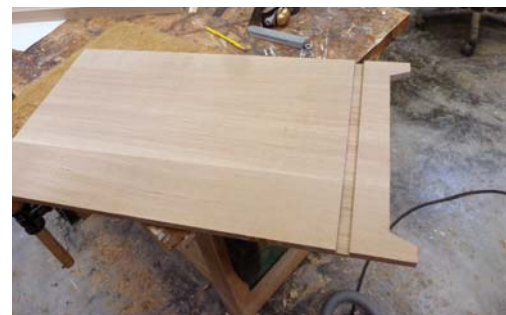
Lighten up. The angled cutouts on the side panels lighten the look of the bottom case.
