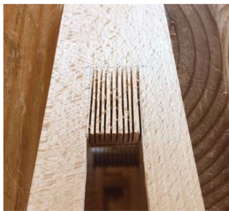
Slot cutting. Start by cutting a bunch of kerfs then pare the waste (above). Finish the slot so it's deep enough to clear the cap iron nut (at right).
