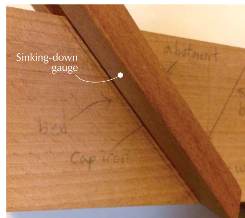
Angle judge. The sinking-down gauge is invaluable for checking the accuracy of the bed and breast surfaces.
