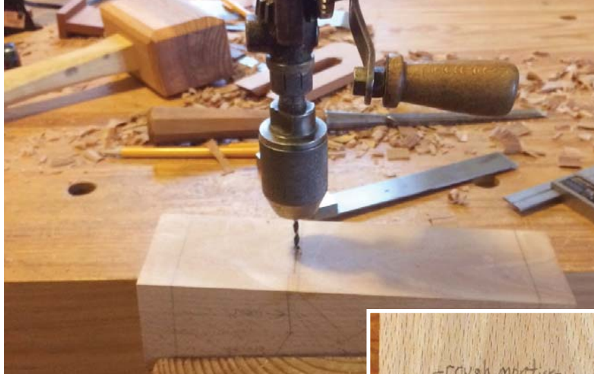
Drill the mouth. You'll save yourself a lot of work if you can drill closely spaced holes parallel to the wear angle. At right is the layout for the eight holes to waste out the mouth.
