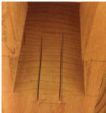
Slot cuts. These saw cuts are full depth at the top of the cap-iron slot and taper to nothing at the bottom – it's a bit like cutting a half-blind dovetail, without overcutting it.
