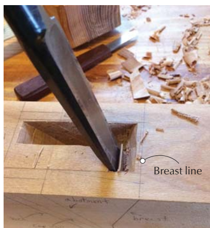
Rough mortise. Here, I've completed the first pass on the far side to rough out the mortise, and am just getting started on the near side.
