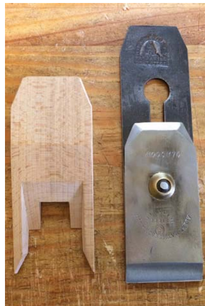
Matched bevels. A nice aesthetic touch for the top of the wedge are bevels that echo those on your iron.
