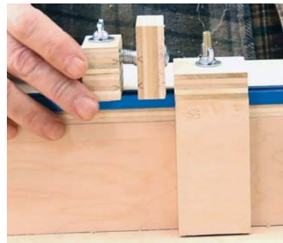
Stop. The micro-adjuster allows you to fine-tune the stop position on the T-track.
