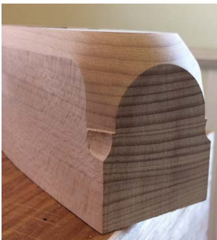
Details. The gouge cuts are a visually pleasing way to terminate the stopped chamfers, and a small fillet left above the gouge cut is a nice touch. A rounded heel is comfortable in the hand.
