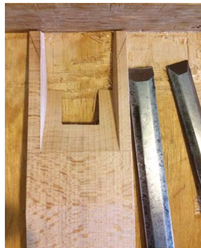
Form the secondary ramp. I butt the wedge fingers up against the back of my bench hook, pare with a chisel (left), then finish with a blunt chisel scraper (right). The only downside is that this is hard on the bench hook.
