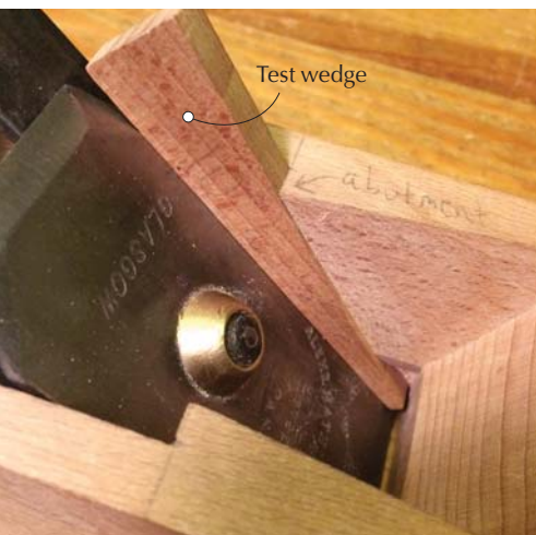
Mini-wedge. A narrow test wedge makes tuning the abutments a snap.
