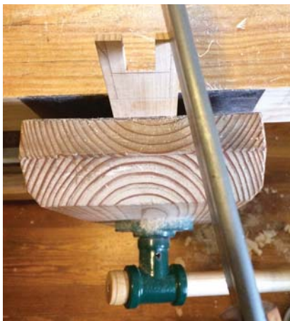
At an angle. When cutting out the fingers, angle your saw toward the center of the wedge.
