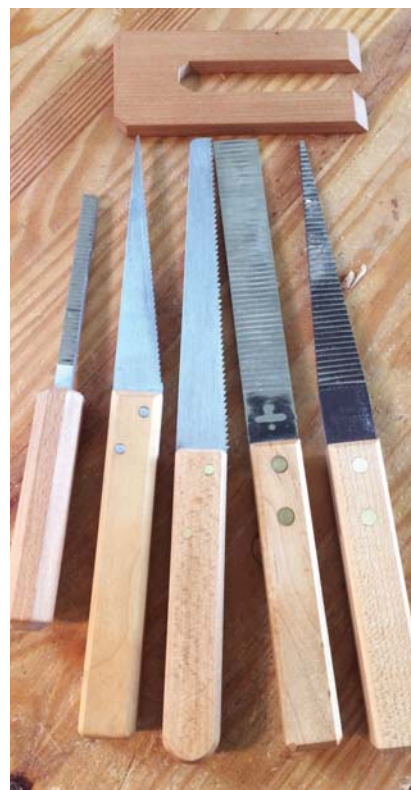
Tools for planemaking. From left are shown a \frac{5}{16} " mortise float, \frac{1}{8} " edge float, abutment saw, \frac{1}{8} " bed float and \frac{1}{8} " side float. At the top is a planemaker’s sinking-down gauge.
