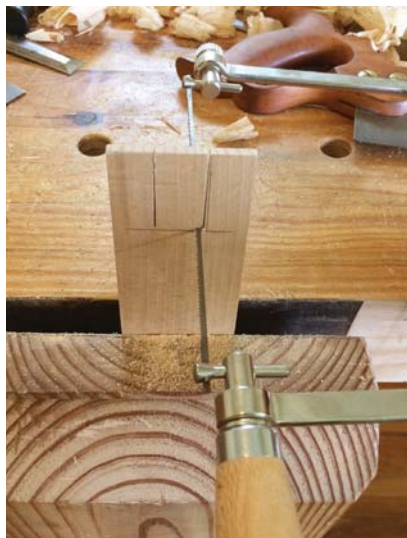
Two saws. Make the vertical cuts with a back-saw. Slide a coping saw down the kerf; move it back and forth while rotating your wrist. When you're at 90°, commence cutting the horizontal.
