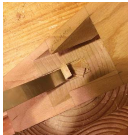
Defined walls. Sawing the sidewalls of the slot allows you to chop most of the waste aggressively, as I'm doing here, bevel down (which affords more control than bevel up).
