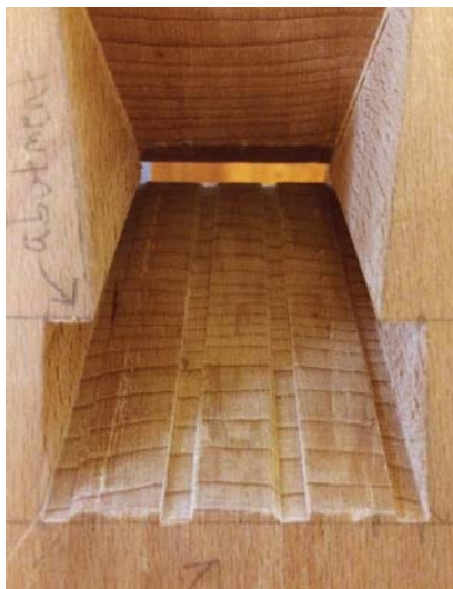
Float kerfs. An edge float makes it easier to cut a flat bed surface.
