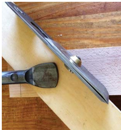
Clamp to scrap. It's easier to accurately trace the outline of the iron if you first clamp a piece of scrap to the bed line.
