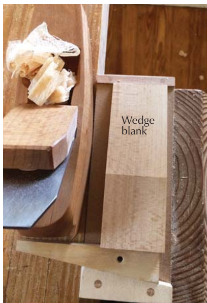
Wedge support. A simple fixture keeps the wedge from flexing while you're planing it.
