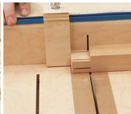
Tenon jig in use. Cut the tenon's cheeks with the jig, then the shoulders on the sled itself.
