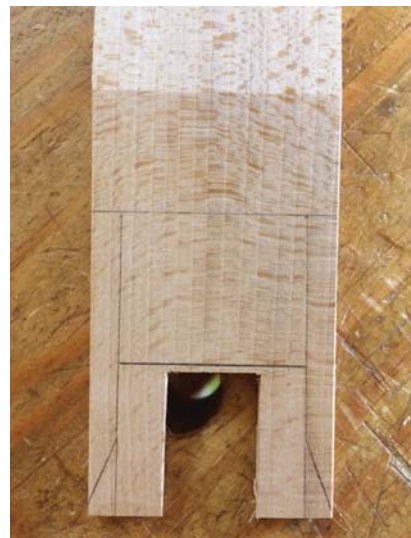
Wedge layout. Here are the wedge fingers and secondary ramp laid out. If your cap iron is nutless, you won't have the notch pictured here.
