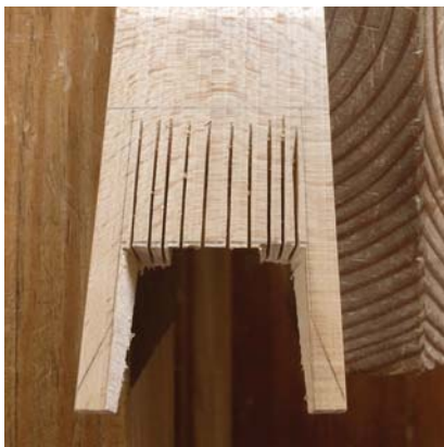
Kerf-cut the secondary ramp. If you have a slot for the cap iron nut, the kerf cuts will break through the slot.
