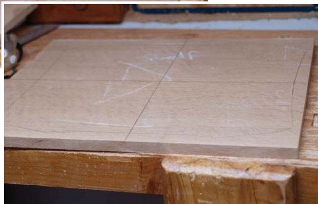
Cut it close. After tracing the shelf pattern, cut close to your layout lines.
