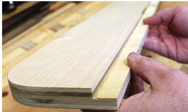
T-track rabbet. Size the rabbet in the upper fence panel carefully so that your T-track will be flush with both the top surface and the edge.
