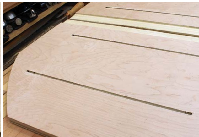
Slots. Rout slots down the center of the dados, creating a track for the shaft of your T-bolts to run in. You might also wish to round off the front corners of the panels, though it's not strictly necessary.
