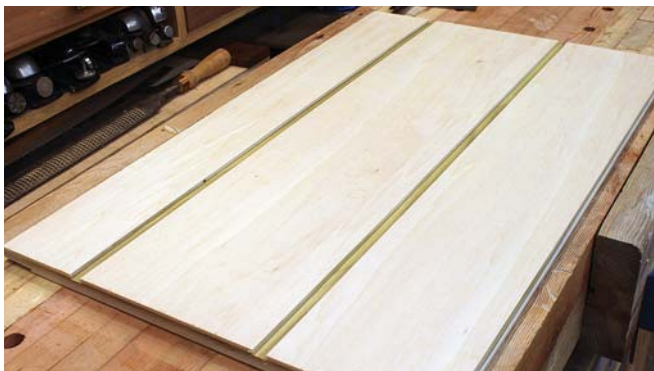
Dados & rabbets. Plow the dados in the bottoms of base panels, then the rabbets on the top interior sides.
