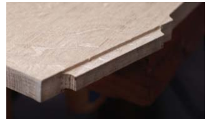
Tongued. Rabbet both sides of the shelf at each corner to form tongues.
