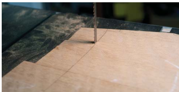
Cut it close. After tracing the shelf pattern, cut close to your layout lines.
