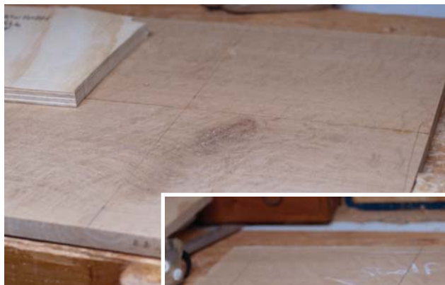
Lined up. Mark horizontal and vertical centerlines on the bottom of the shelf blank.
