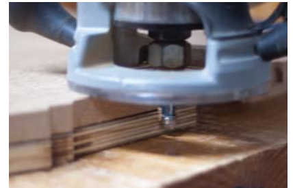
Final shape. Rout the shelf to final shape.
