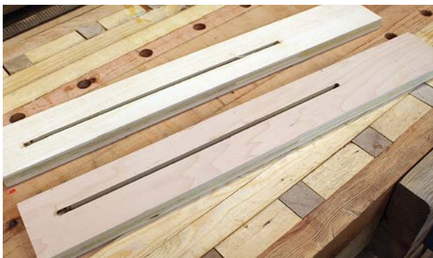
Fence extensions. Keep the slotted fence extensions close by; you'll soon use them as spacers.
