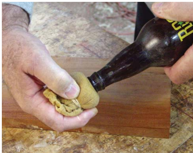
Bottled & ready. I dispense the shellac from a beer or wine bottle; that makes it easier to control the amount that goes onto the pad than dipping into a Mason jar.
