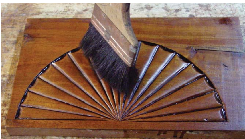
Dry brush. This process is done with an artist's dry brush, one with particularly soft and poufy bristles. The brisk motion is very much like dusting something, the brush just barely touching the surface. Like padding on shellac, this technique takes practice – but the visible results will tell you a lot about your progress.
