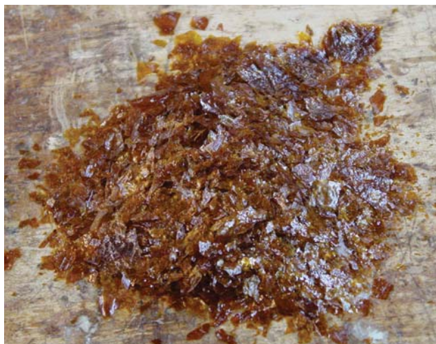
Just add alcohol. Liquid shellac goes bad after about six months, so I recommend dissolving flakes in denatured alcohol as needed.
