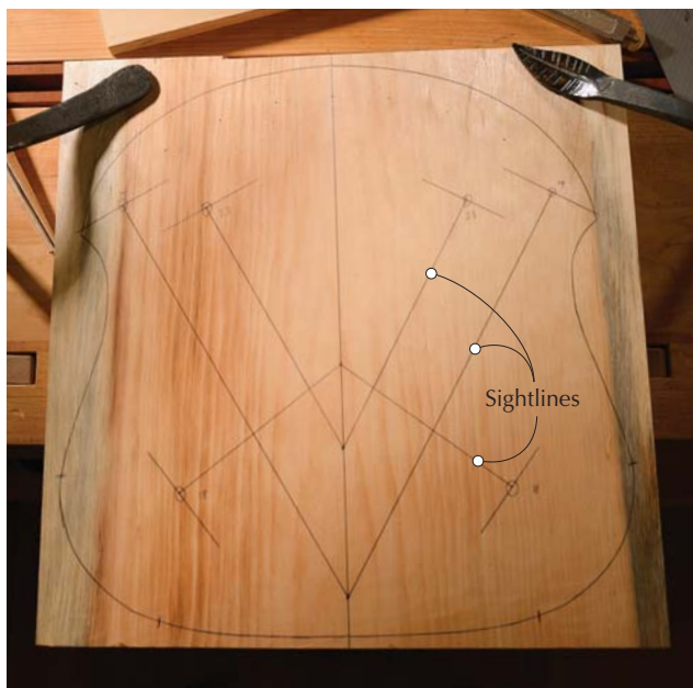
Sightlines. Sightlines are based on the rake and splay of a chair leg or arm post.
