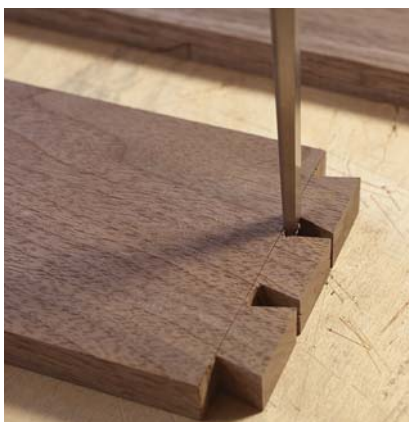
See the side. Chopping the last bit of waste is all about keeping your chisel 90° to the work. So sit to the side of the chisel so you can see when you are at 90°.
