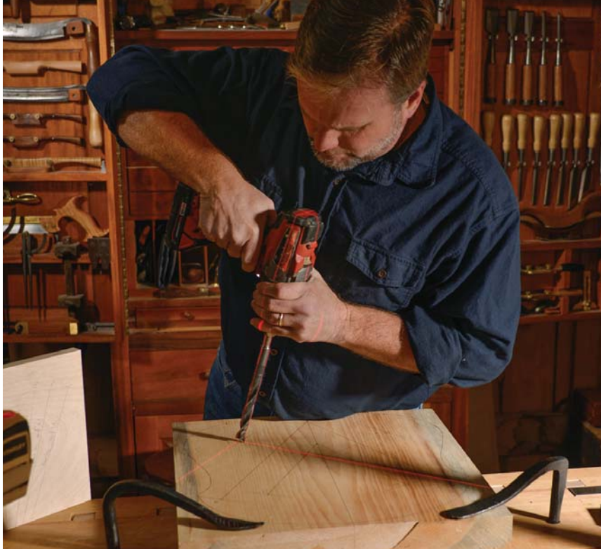
Bull's eye. Use the drill's casing to find the center axis of your bit.
