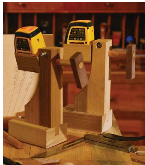
Scrap bases. Rotating bases position the lasers 9" off the top of the workbench, where the laser guides work best.
