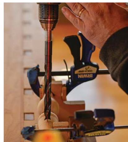
Get centered. Lasers can also help you find the center axis of legs and stretchers.
