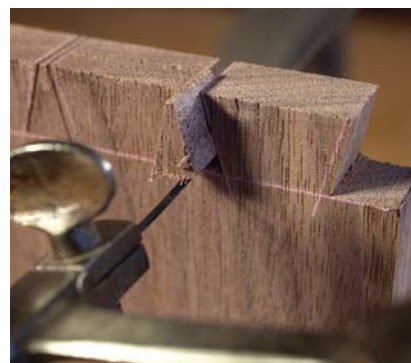
Start fretting. With thin stock, I use a fretsaw to remove the waste between the tails. Thick stock demands a coping saw or bowsaw. If you cut slowly, you'll be able to saw close to your baseline – saving lots of chopping.
