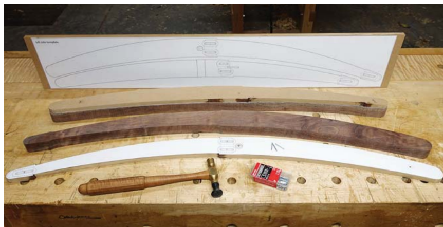
That was easy. Adhere the pattern to \frac{1}{2} " MDF, cut it out, tack it on, trim off the excess and rout with a pattern bit.
