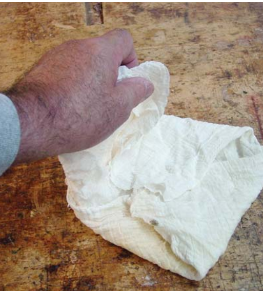
Polish pads. Make two pads out of tightly folded 90-pound lint-free cheesecloth; secure the pads with rubber bands.
