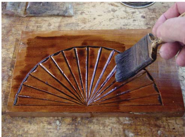
Brush on. Apply a heavy, wet coat of glaze using a natural-bristle brush.
