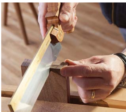
Gang of two. I gang-cut my tailboards whenever possible. This saves a lot of time and – for beginners – results in the tails' walls being more square. I think three tails looks nice here.
