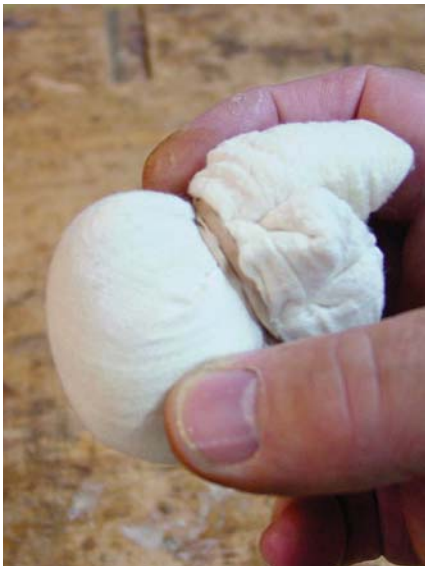
Polish pads. Make two pads out of tightly folded 90-pound lint-free cheesecloth; secure the pads with rubber bands.
