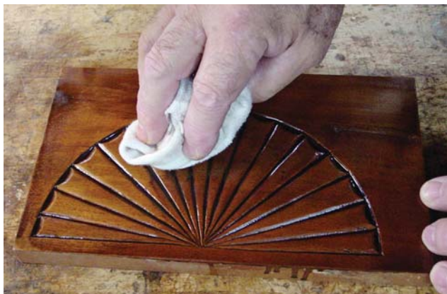
Wipe off. After 10-30 minutes, rub vigorously with a clean rag to remove as much glaze as possible from the high spots, allowing it to remain in low spots and crevices.
