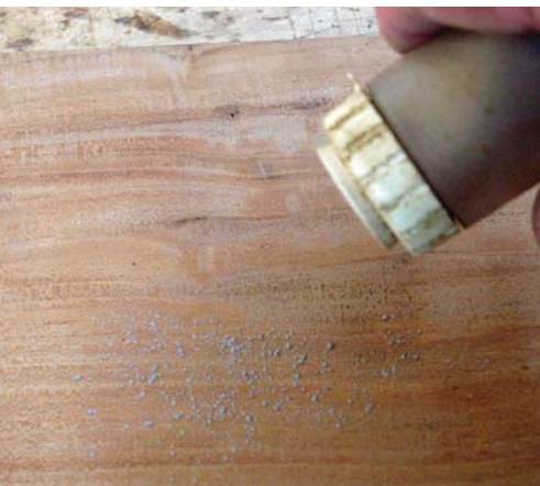
Shake it out. I dispense the tinted pumice from an inexpensive salt shaker.
