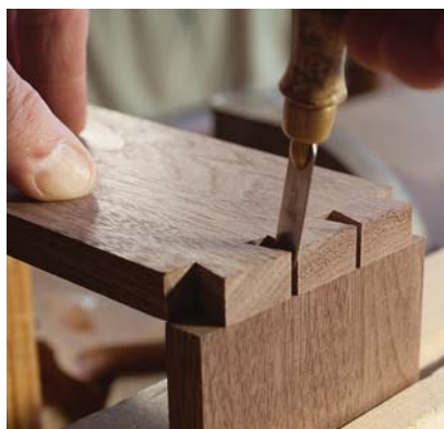
Don't be a pinhead. Most dovetail mistakes happen when transferring the shape of one joint to the other. Take your time and take great care. Even after 25 years of cutting this joint, I focus 100 percent at this step.
