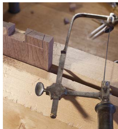
Slow is much faster. Again, take your time when fretsawing away the pin waste. A little care will save lots of boring chopping.
