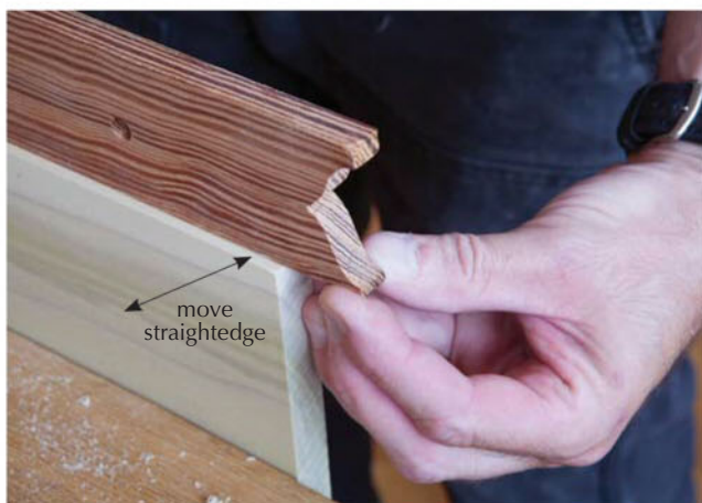
No drag. A straightedge placed on a second edge can tell you if the edge is convex, or if it is flat or concave. If the straightedge spins on the work, the work is convex. If the ends of the straightedge drag, then the edge is flat or concave.
