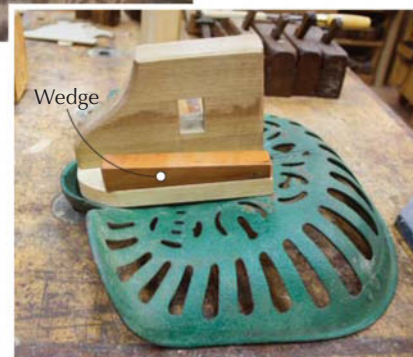
Even keel. This keel is sized so that the mortise is just below the bench of the horse; the wedge is inserted to keep the seat securely in place in its track.
