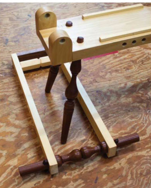
Almost ready. After knocking the legs in place, put the bench inside the assembled frame, then lift and turn it into place.
