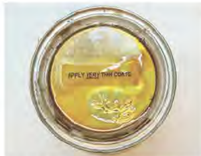
Thumbprint. Here is my thumbprint in Tried & True polymerized oil that is 20 years old. The oil barely even gelled.
