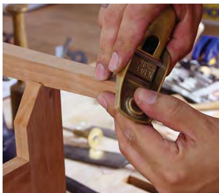
Protect your feet. A \frac{1}{8} " x \frac{1}{8} " chamfer around the bottom of all the legs protects the feet from chipping as you move the table.
