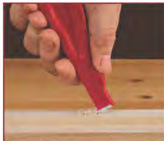
Get a finish quality cut using a pulling motion with the Mini Scraper at a high angle.
