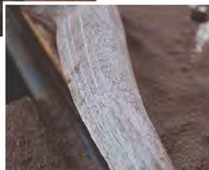
Second bevel. Here's the leg with the first bevels faired to the second set of lines, resulting in a rounded profile.
