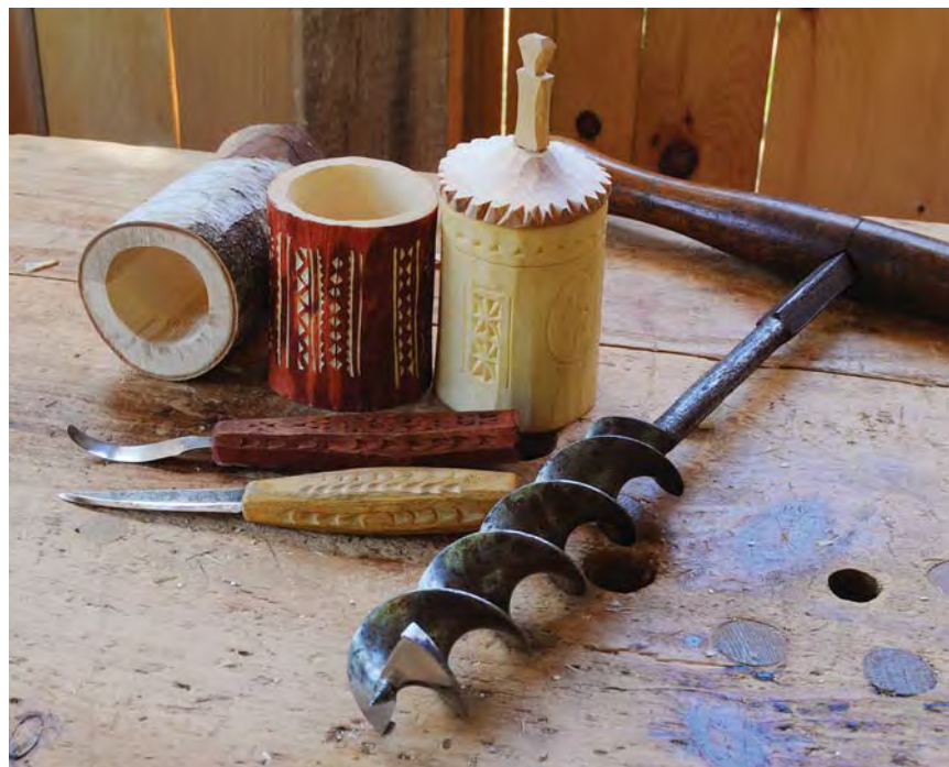
Shrink pots: deceptively simple. Bore then carve the green interior, pop a dry bottom in place, then wait. (And perhaps add a few decorative touches and a lid.)
