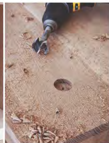
Follow the pilot. Put the tip of your Forstner in the pilot hole and drill \frac{1}{2} " down. Keep the drill as plumb as possible.
