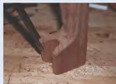
4 Define. Round off and undercut the toes, then fair the transition from the ankle to the foot.
