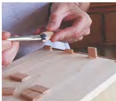
Paint the Domino. Use plenty of glue. I paint glue in the mortise and on the Domino. Glue is cheap; broken drawer joints are not.
