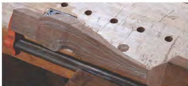
Guidelines. Four lines on each face will guide your rasp work as you shape the leg corners.
