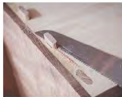
A flush finish. A flush-cut saw makes quick work of removing the extra 2mm protruding from the drawer sides. A plane finishes the job.
