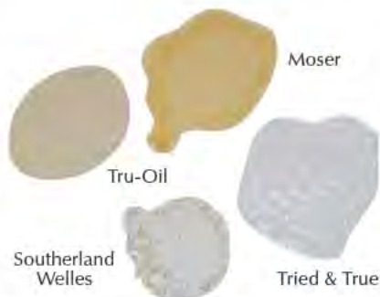
Puddles on glass. I applied puddles of all four products claiming to be polymerized on glass. Notice that Tru-Oil and Southerland Welles dry similar to drying oils, Moser’s Polymerized Tung Oil Varnish dries like varnish and Tried & True didn’t dry at all.
