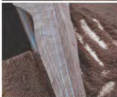
First bevel. Here's the leg with the first corner beveled to the outermost guidelines on two faces.
