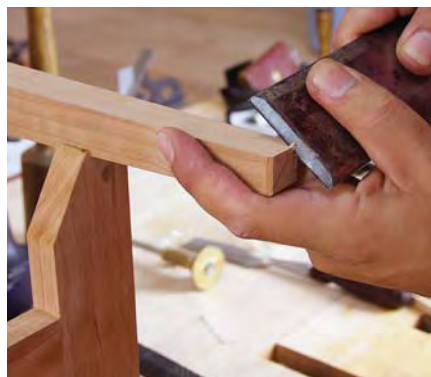
Protect your feet. A \frac{1}{8} " x \frac{1}{8} " chamfer around the bottom of all the legs protects the feet from chipping as you move the table.
