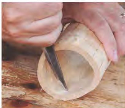
Get in the groove. After scoring the defining edges of the groove for the bottom, I use a Sloyd knife to remove the waste between.
