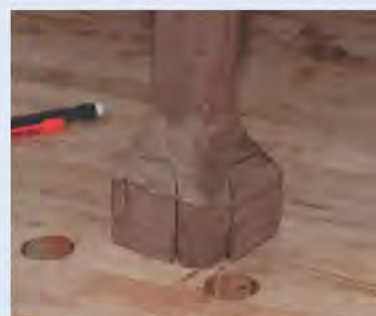
2 Stop cuts. Make shallow backsaw cuts to define the toes.
