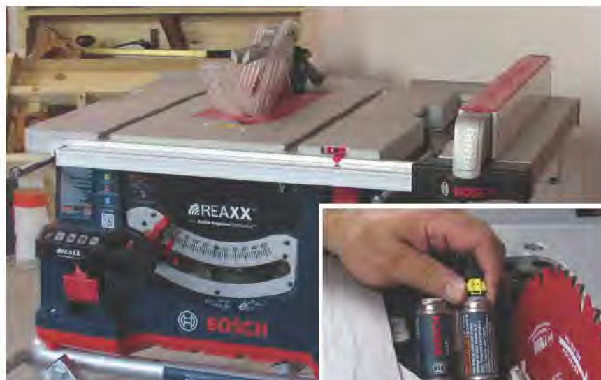
Old school meets new. Easy-to-use guard system and flesh-sensing technology converge in a top quality, high-performing saw.
