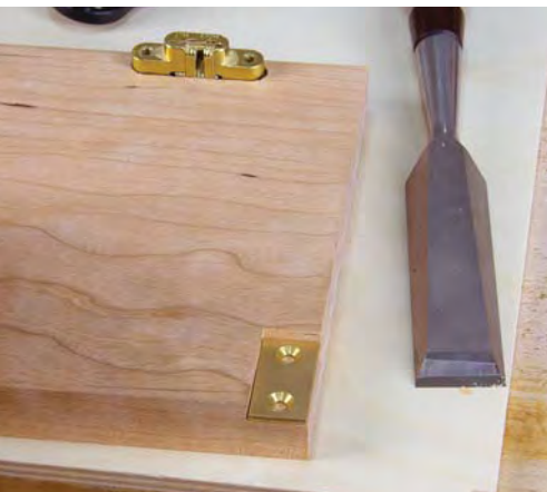
Strike install. One of three little brass pieces is the catch for the false apron's latch.
