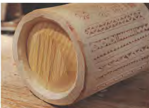
Pop in place. With a bit of pressure, pop the bottom in place to align with the grooves. Then wait for the pot to dry and shrink around the bottom.
