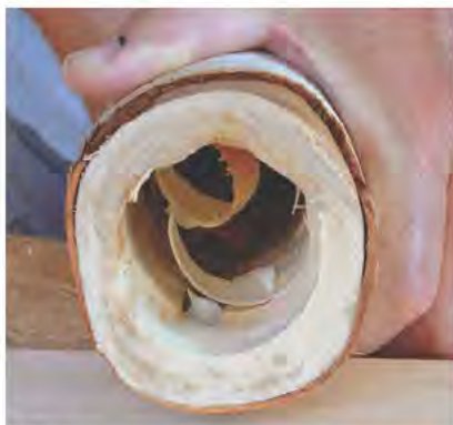
Wrap cuts. My hands turn in opposing directions as I hollow the interior with a hook knife.
