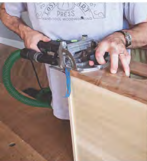
Plunge in. The Domino cuts a deep mortise through the drawer side and drawer front.
