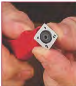
Just loosen the screw and rotate the blade and you have a sharp, fresh edge.
