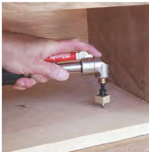
A hole to pilot you. A \frac{1}{16} " pilot drilled through both carcasses makes it easy to drill the 1"-diameter holes for the dowels. (The little block of wood? It's covering the flutes on a countersink bit – the only \frac{1}{16} " bit I have with a hex shaft to fit my right-angle drill.)
