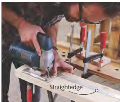
Leg rip. Use a straightedge as a saw guide and rip four 1 1/2"-square legs from the 2x6s.
