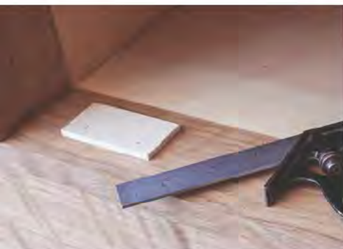
Drawer stops. My drawer stops are \frac{3}{16} "-thick poplar, which was scrap from making the drawers. Tack the stops in place with \frac{1}{2} " brads.
