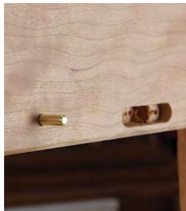
Drawer lock. A brass rod acts as a lock for the hidden drawer. Mark its length, cut it to size, and chamfer the ends using a small file and a drill, guiding it with a hole drilled in a piece of scrap. Mark where it ends on the inside of the false apron, and drill a hole, then countersink the rim.
