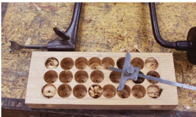
Hog it out. It's a lot easier and faster to drill out the bulk of the waste than to remove it with a chisel alone.
