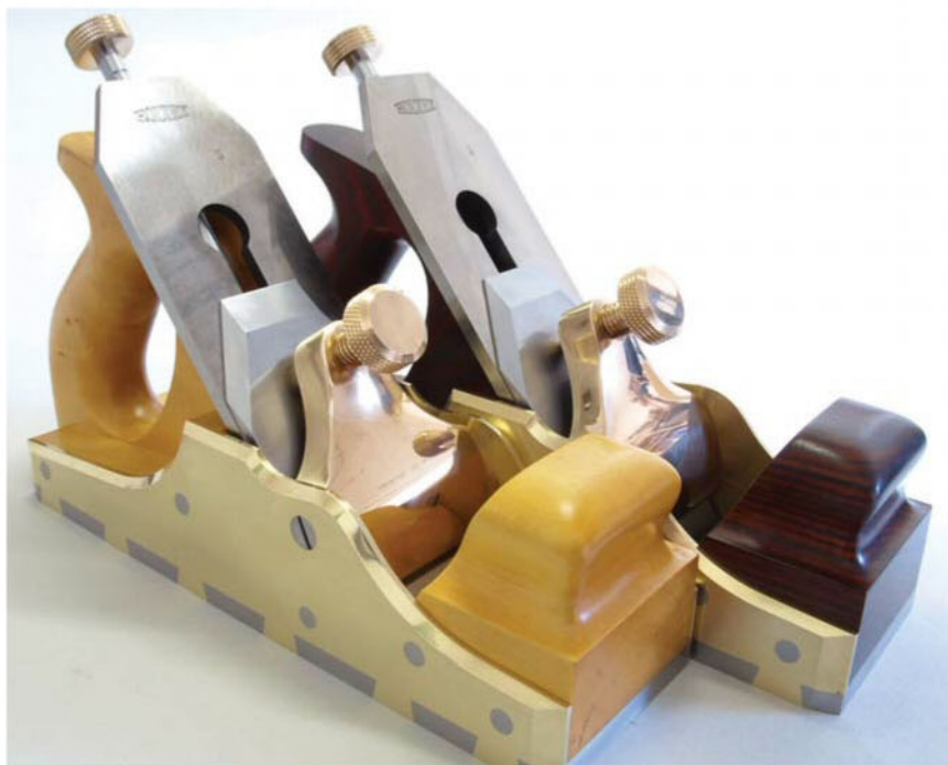
Better bun. The Holtey A13 features an improved front bun design over the original Norris plane.
