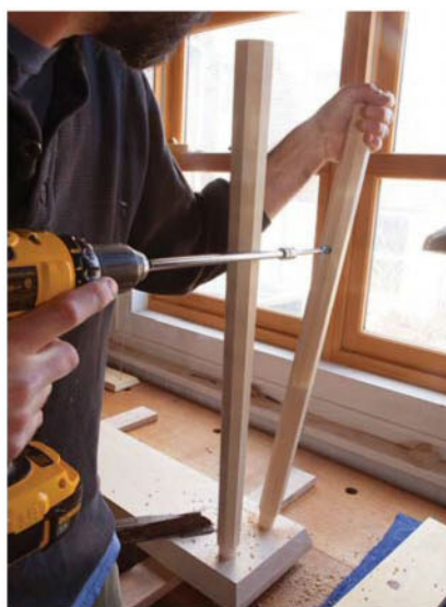
Hot-doggin'. Line up the shaft of the bit extension with the lines you marked on the leg near the drill. That is all the accuracy you need to drill this mortise.
