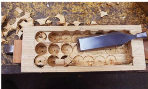
Rough removal. Work with the grain with a chisel to remove the waste between the holes
