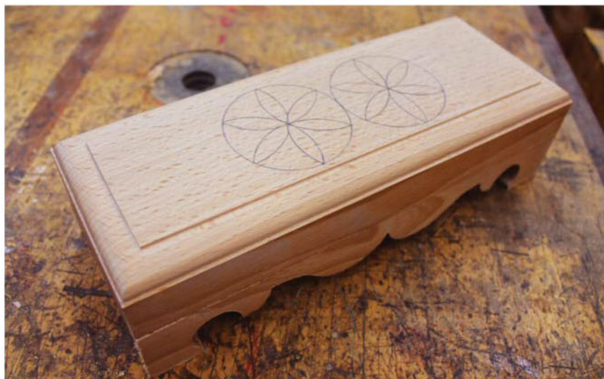
Penciled in. After scratching the design with compass points, use a fine pencil to trace the shallow recesses; this will help the design stand out.
