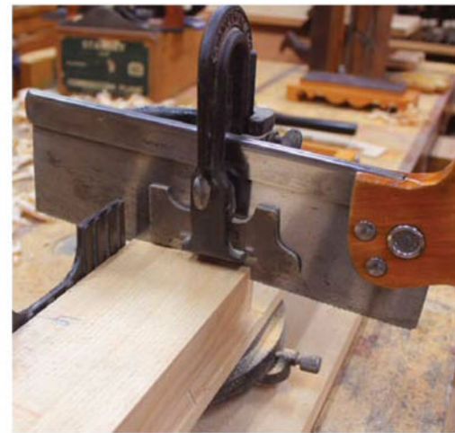
Miter box. Note that the reference edge is against the fence as I crosscut this workpiece to length.
