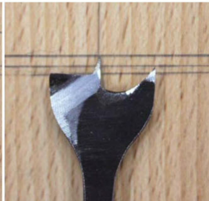
Modified. “Safe” files (which have one or more smooth edges) make quick work of modifying a centerpoint bit. On the left is the bit before I shortened the point; on the right I filed the point so it's about \frac{1}{8} " longer than the spur.
