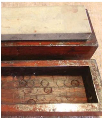
A bit of evidence. You can still see the marks from the bit spurs in this box lid.
