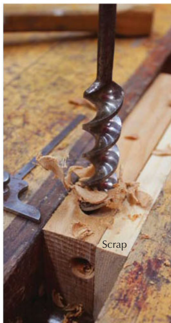
Bit selection. A No. 100 Jennings-pattern bit works for the long-grain holes, but for end-grain drilling, a centerpoint is the better choice.
