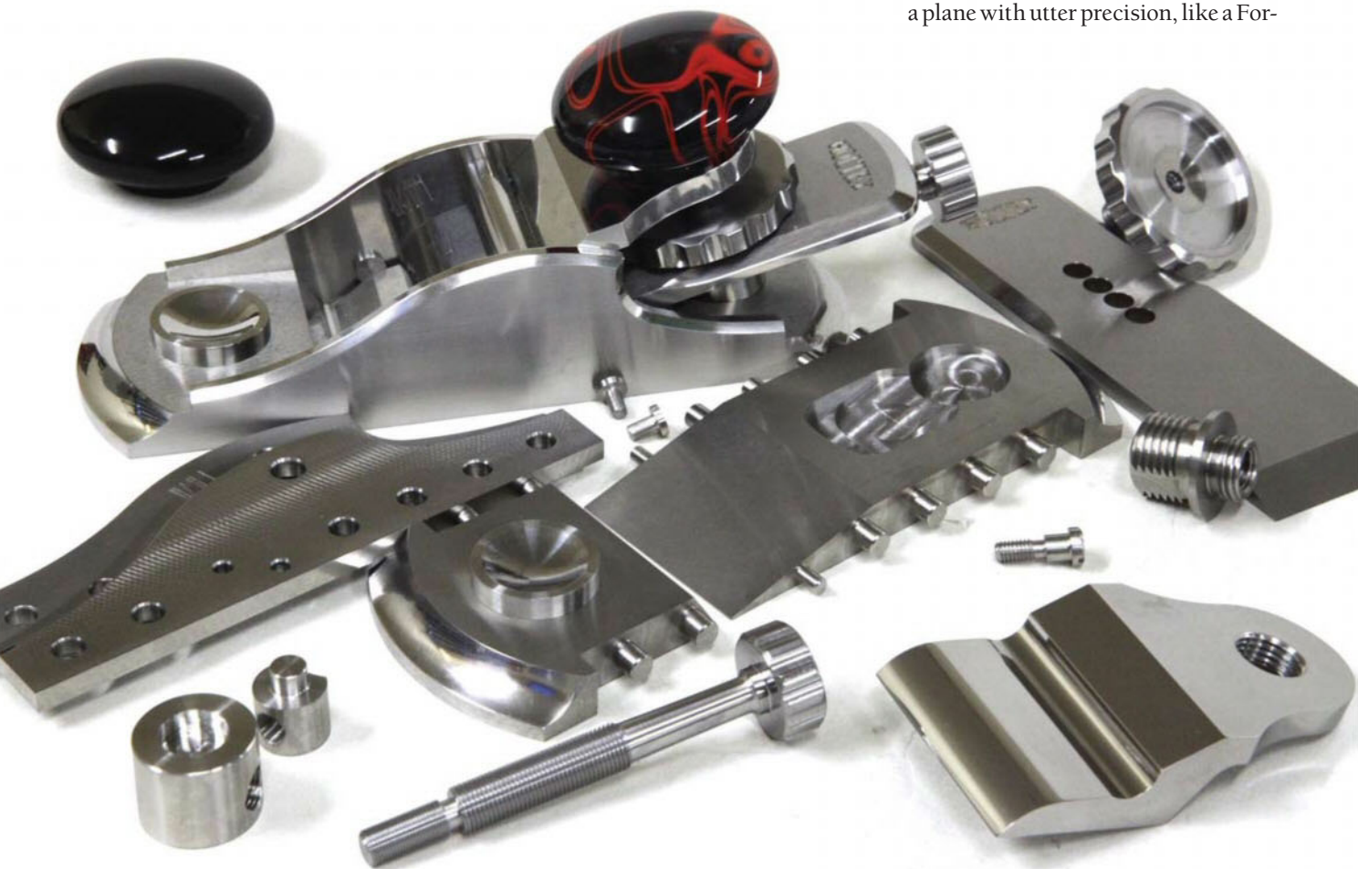
No. 983. Robin Lee convinced Holtey to develop the 983 block plane, show here in disassembled and complete form.
