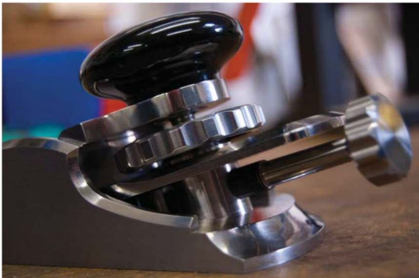
Under pressure. The blade-clamping mechanism of the 983 may not look unusual, but it addresses some common design flaws through meticulous attention to detail.
