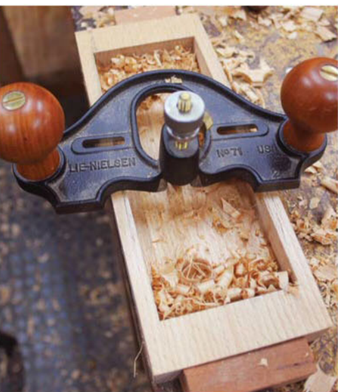
Rout it out. Use a router plane to reach the final depth and remove bit tool marks.
