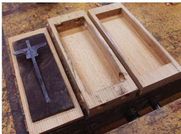
Piecework. Here's the rough-sized platform (with leather atop), the underside of the bottom with the cavity drilled and smoothed and holes drilled for the corner curves, and the hollowed-out top.
