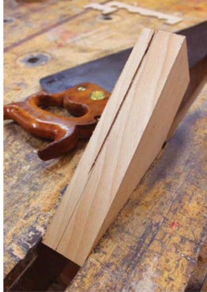
Platform. The waste from the top piece is sawn off; I'll size it to match my piece of leather, and use it as the platform.
