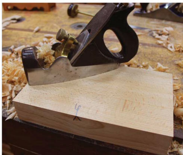
Reference surfaces. With one edge and one faced planed flat and at 90° to each other, you have references surfaces from which to scribe the final dimensions.
