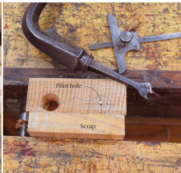
Bit selection. A No. 100 Jennings-pattern bit works for the long-grain holes, but for end-grain drilling, a centerpoint is the better choice.
