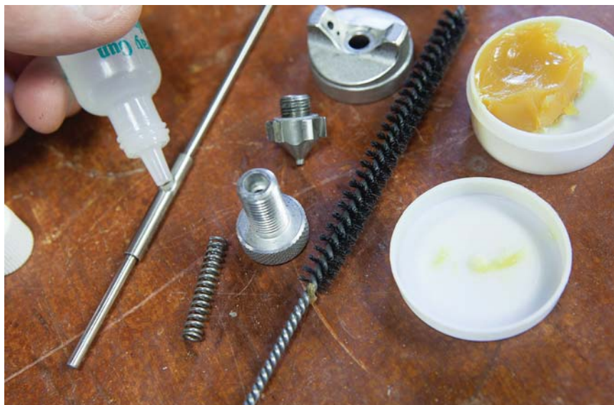
Stop sticking. Lubricating the interior parts prevents things from gumming up – even a few molecules of sticky finish can prevent parts from moving smoothly.
