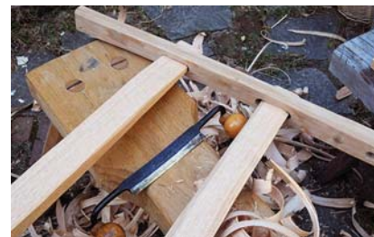
Rails. Use a hatchet or drawknife to shape the rails and fit the through-tenons (which needn't be tight), then peg or nail the braces in place.
