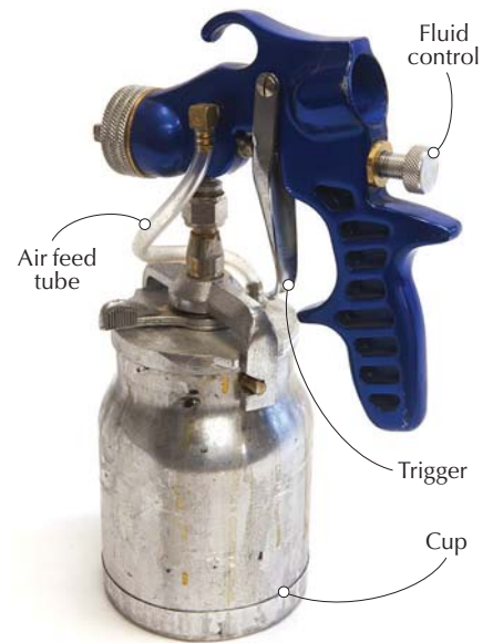
A simple spray gun. Here you can see the fluid control knob, the air cap, fluid tip and the “cup” – which holds the finish. These are the essential parts you need to be concerned with.
