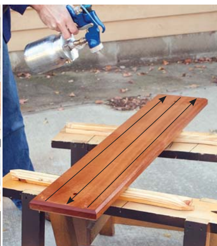
Front edge & face. Spray the front edge, then continue working on the face of the panel.
