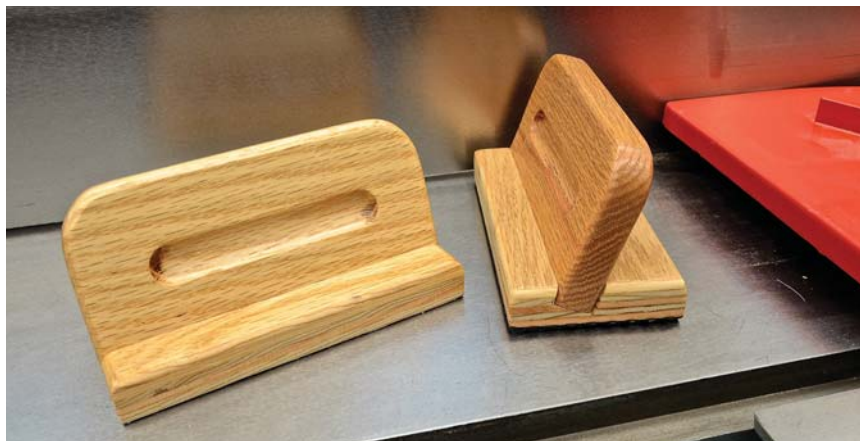
Closed for safety. The closed handle of this shop-made push pad design is safer than the typical D-handle commercial version – your hand can't get caught inside this handle.
