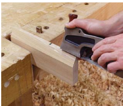
Don't wander. Try to take passes straight in line from one end of the profile to the other to get consistent results.
