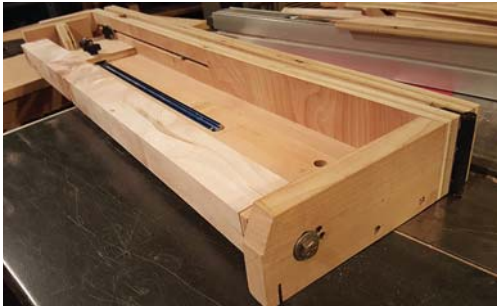
The foot in the jig. The leg is attached by a bolt that goes through the jig and into the threaded insert on the cartridge, which is screwed to the leg.
