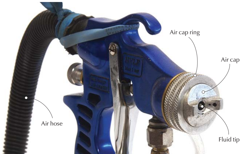
A simple spray gun. Here you can see the fluid control knob, the air cap, fluid tip and the “cup” – which holds the finish. These are the essential parts you need to be concerned with.
