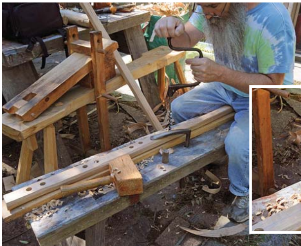
Bore & chop. Lay out your mortise locations, bore a hole at either end, then chop the waste between.
