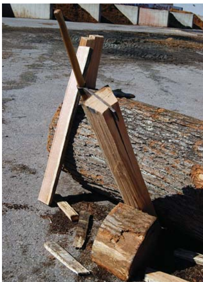
In a pinch. A log and a split section of wood can serve as a brake if need be.
