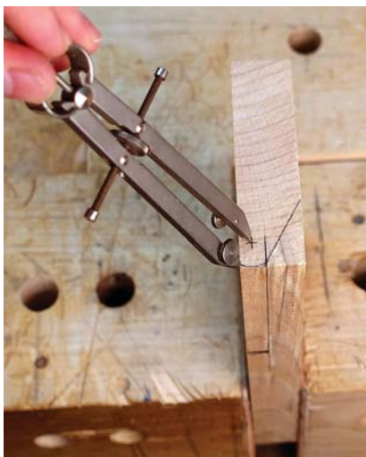
Round layout. Lay out the profile on both ends. Use a compass to accurately mark the arch.
