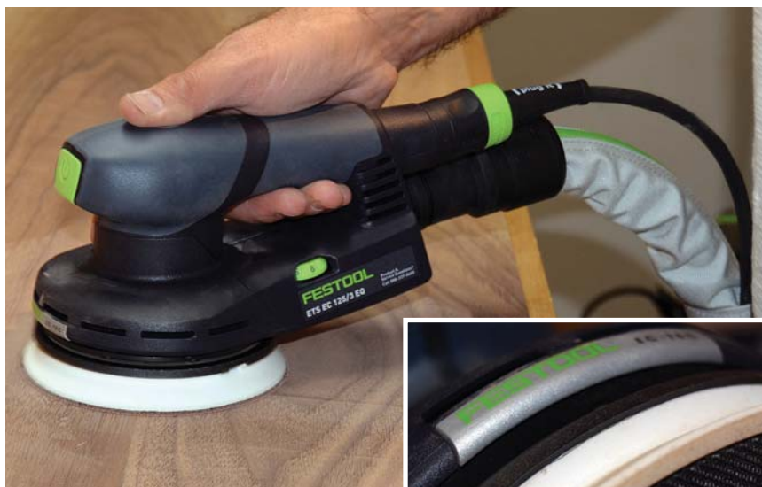
Low profile. The Festool EC125/3 delivers good performance and comfort in a low-profile tool. The dense backer pad (right) accepts any hook-and-loop sanding disc.
