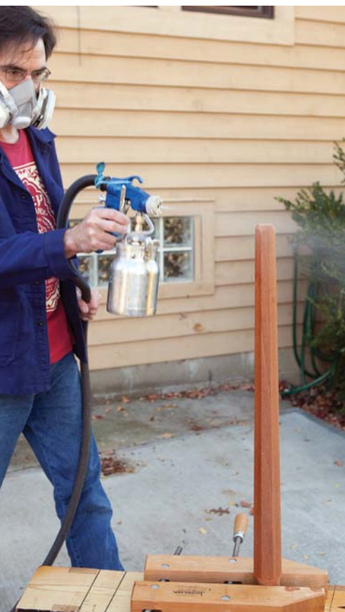
Horizontal fan. When spraying legs, I get them vertical and use a horizontal fan. This reduces the chance of getting dry spots on your legs.
