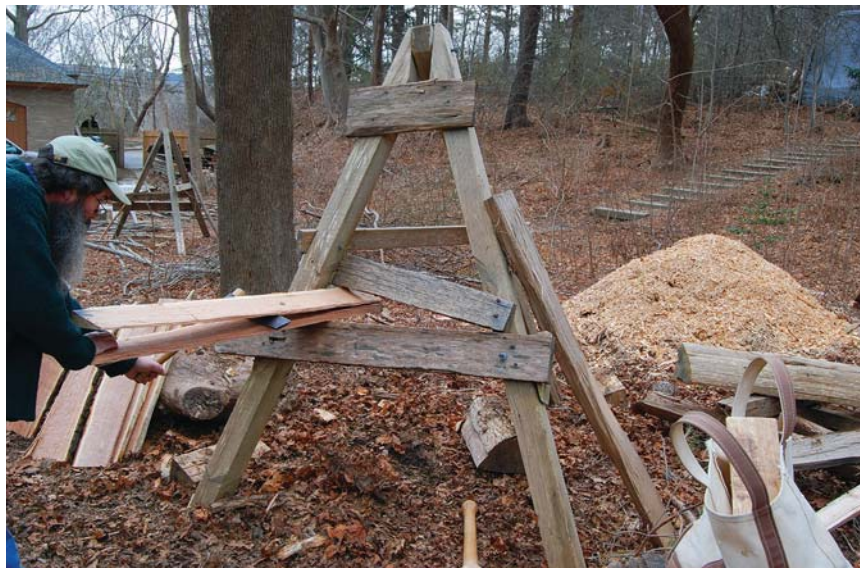
Sophisticated. The tripod riving brake shown here is the sophisticated version of a contraption to help hold logs and billets as they’re split with a froe.
