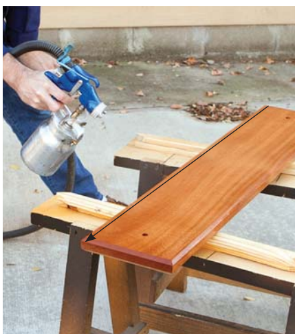
Front edge & face. Spray the front edge, then continue working on the face of the panel.
