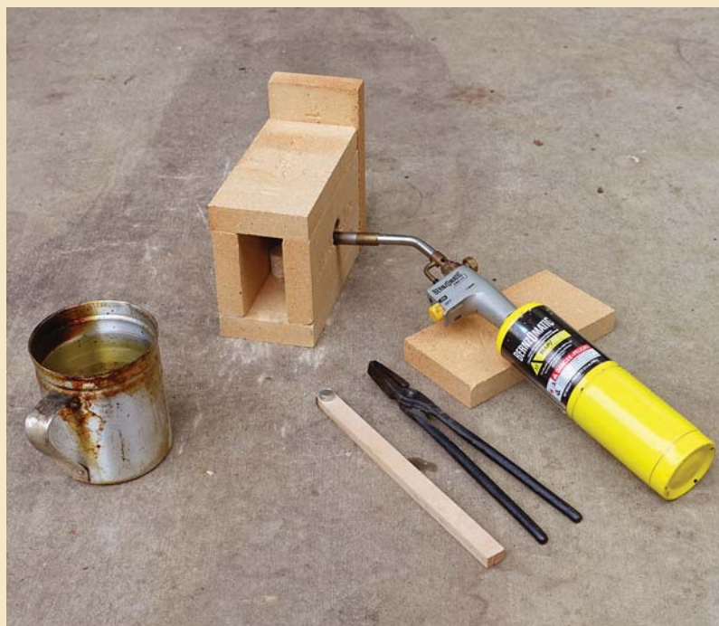
Even heat. A firebrick enclosure helps evenly distribute heat on the tool steel.
