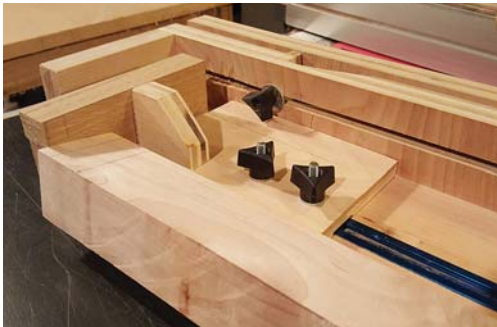
At the top of the jig. The carriage can be adjusted for legs of different lengths.
