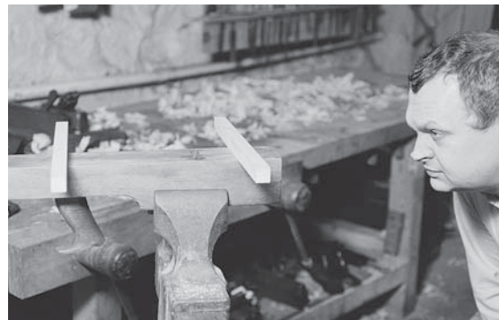
Level check. In a 1989 picture from "Restoring, Tuning & Using Classic Woodworking Tools," Dunbar shows how to use winding sticks to check a wooden plane's sole for twist.
