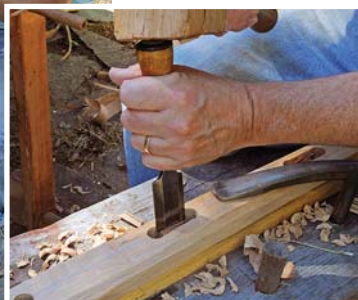
Bore & chop. Lay out your mortise locations, bore a hole at either end, then chop the waste between.
