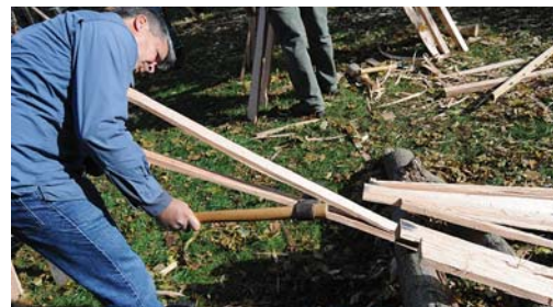
Forked. Here, a student is using a forked-tree brake as he rives oak with a froe.
