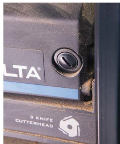
Look for it. A port such as this indicates the brushes of the motor will be easy to replace. Pick up the phone right now and order replacement brushes for your planer. They are good to have on hand.
