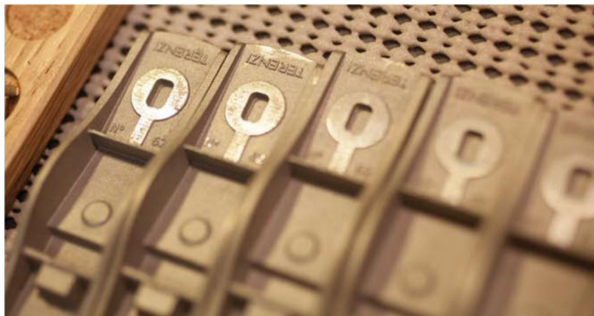
Tiny castings. Shown here are some of the quarter-scale white bronze bodies that Terenzi will mill into working bevel-up jack planes.
