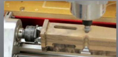
Using the turning system to mill the legs and mortise/tenon joints.
