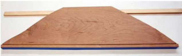
Ready to plane. Here's the largest shelf, shown upside down with the "ears" still intact. Both halves of the cleats are attached at the back, and the \frac{3}{8} " batten is attached at the front to the top surface with hot-melt glue.
