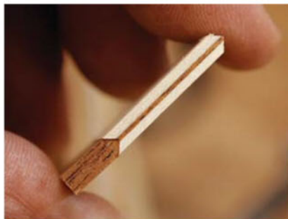
A perfect match. With the V-cuts centered on both pieces, they'll mate perfectly.
