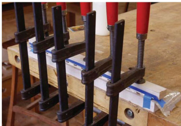
A perfect match. With the V-cuts centered on both pieces, they'll mate perfectly.
