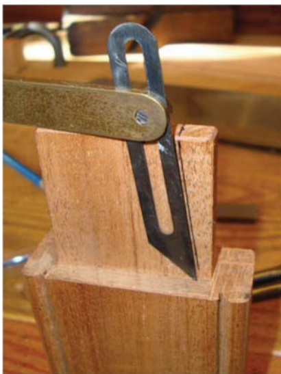
Split prevention. Cutting the wedge slots at an angle helps prevent splitting by reducing the bending friction at the base.
