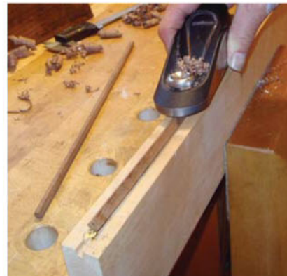
Enter the octagon. I make the square strip into an octagon by planing the facets on a shop-made jig. Count the number of strokes on each facet, and mark the square faces to keep track of the worked facets.
