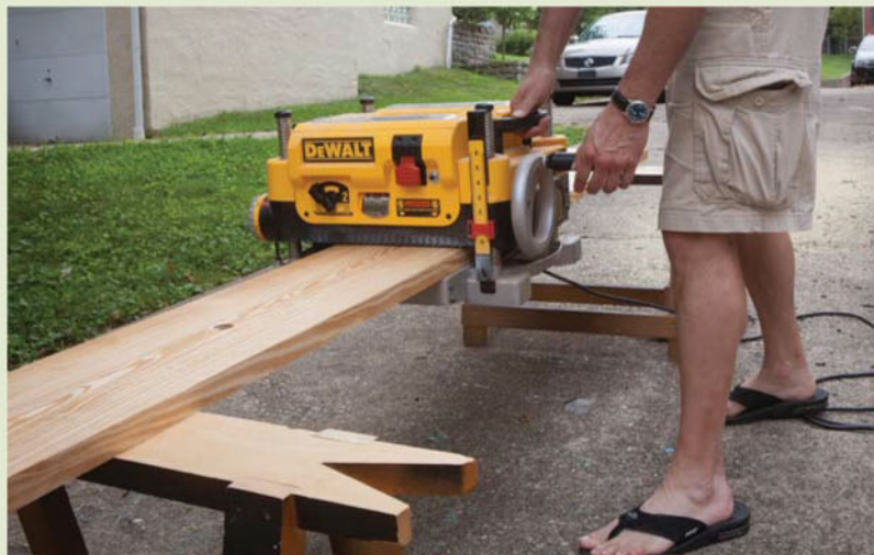
You need an extension cord. Yes, a planer can pull itself along like this for long and heavy stock. Do this outdoors and with a long extension cord. It's like walking a robotic dog.
