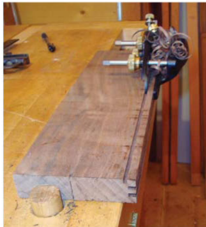
Plow it out. I make drawbore pegs from a strip of walnut by plow-planing thin grooves until a 1/4"-square strip is released.
