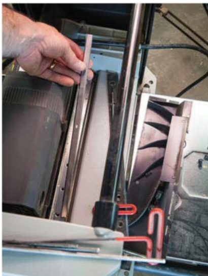
Presto change-o. Quick-change knife systems get you back to work in less than 30 minutes. Once you try one, you'll not willingly go back.
