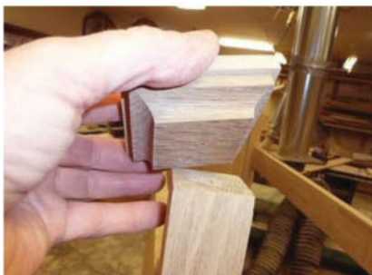
Nice feet. A \frac{1}{2} " cove and slightly larger base combine to create an eye-catching bottom detail to the feet.
