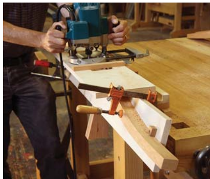
Multi jig. This simple jig guides a router fence to make quick work of the flats, and of the mortises for the side rails.
