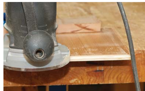
Router tenons. I used a router with a rabbeting bit to cut \frac{1}{4} "-thick tenons on the divider and shelf ends.
