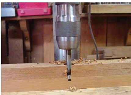
Hinges. The hinge spigots are fit into \frac{13}{16} " holes drilled into battens that will attach to the underside of the tabletop.
