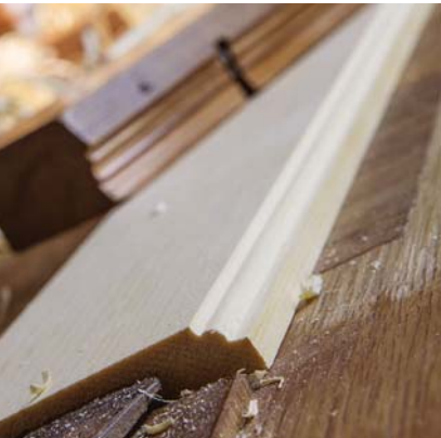
Completely stuck. Mould the entire stick of wood before cutting it apart for mitering. This ensures the moulding will match at the corners.
