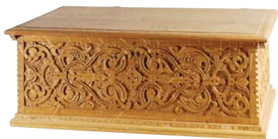
A box. In the 17th-century-style work I do, boxes aren't typically dovetailed. They're rabbeted, then nailed.
