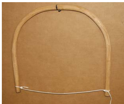
Strung up. Once a piece is cool to the touch, a single-plane bend can be tied in place with a string and removed from the form. Notice that the string shown here is loose; the wood continued to compress after it was removed from the form.
