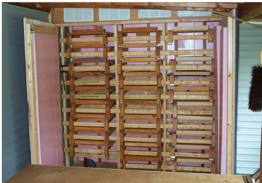
Stacks of arms. A continuous-arm chair back (bent in two planes) needs to stay on the bending form for three days, so the forms are stacked in a drying room equipped with a heater.
