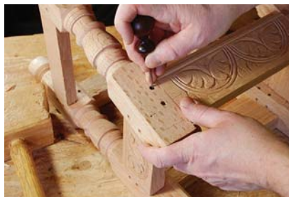
Mark. Use an awl to mark the hole location on the tenon. Then remove the tenon and offset the center point about 1/8" toward the shoulder, and drill.
