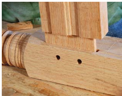
Fit. First, show the tenon to its mortise.
