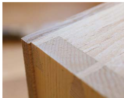
Proud bottom. Here you can see how the bottom protrudes from the end of the tray, making the tray a cinch to fit.
