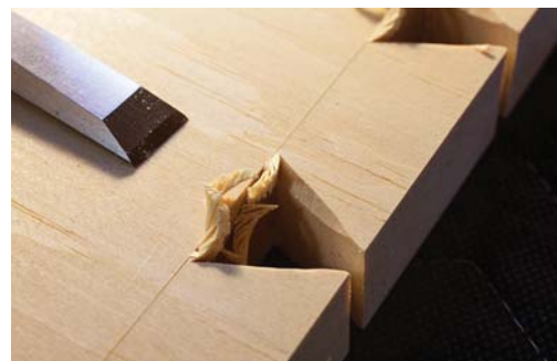
Ease the entry. Beveling the interior corners of the tail boards makes assembly easier. And you are much less likely to damage your tails when driving them into the pins.
