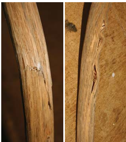
Tension shear & compression. In tension shear (left), the fibers simply tear during bending. A compression failure (right) – where fibers wrinkle instead of bend – typically occurs on an inside curve.
