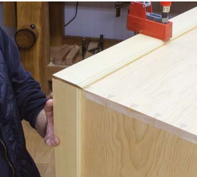
Miters all around. I begin mitering at one front corner of the chest. I get that joint perfect, then I make my way around the carcase.
