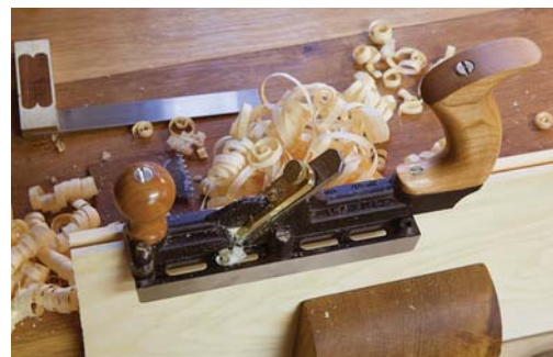
Groove your bottom, then tongue it. I use a tongue-and-groove plane to cut the joints on the long edges of the bottom boards. This plane cuts both the male and female bits.
