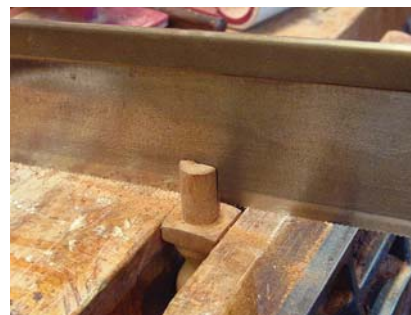
Kerf. Saw a kerf for a wedge to about \frac{1}{4} " above the tenon shoulder.
