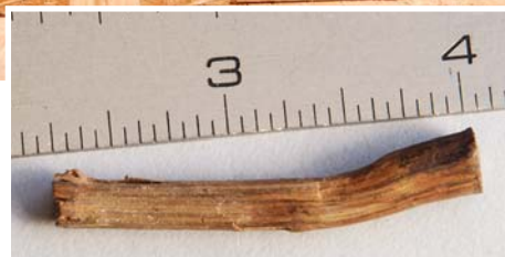
Built to last. The section cut above of a drawbored mortise-and-tenon joint shows how the peg snakes through an offset to pull together the mortise and the tenon. At right is a 17th-century peg, from a Braintree, Mass., joined chest.
