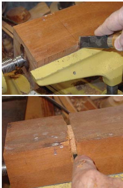
Nick & turn. After nicking the arris corners, turn the spindle round.
