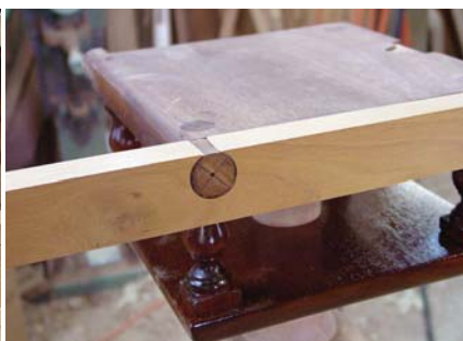
Hinges. The hinge spigots are fit into \frac{13}{16} " holes drilled into battens that will attach to the underside of the tabletop.
