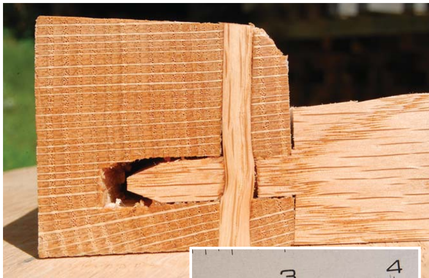
Built to last. The section cut above of a drawbored mortise-and-tenon joint shows how the peg snakes through an offset to pull together the mortise and the tenon. At right is a 17th-century peg, from a Braintree, Mass., joined chest.
