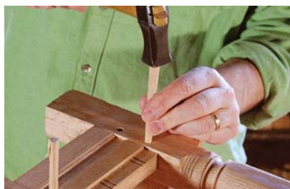
Pegged. Now drive a peg (preferably of riven oak) into each hole.
