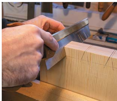
The gang's all here. When cutting through dovetails, I gang-cut the tail boards to save time and effort.
