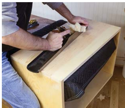
Long sleeves. Sleeve the assembled carcase over your benchtop to make it easy to level the front and back of the chest.
