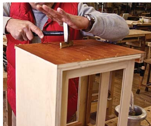
Hot hide. The carcass is veneered in the traditional manner, using hot hide glue and a veneer hammer. It's not difficult, but you must work quickly.
