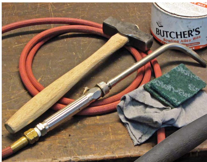
Tools. A torch, some wax and an abrasive pad are all you need to produce a rich black finish.
