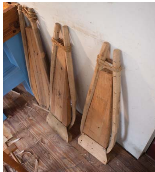
Ready for comfort. The back legs of Alexander's chairs are shaved to shape, steam-bent and then placed in these forms to dry, ensuring they hold their shape.
