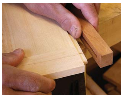
Staging strip. The front of the staging panel is attached with a stub tenon that stops just short of either end.
