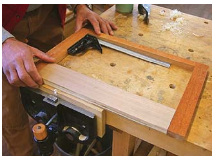
Face front. The face frame is joined with open mortise-and-tenon (stub tenon) joints; make sure everything is square before you glue up.
