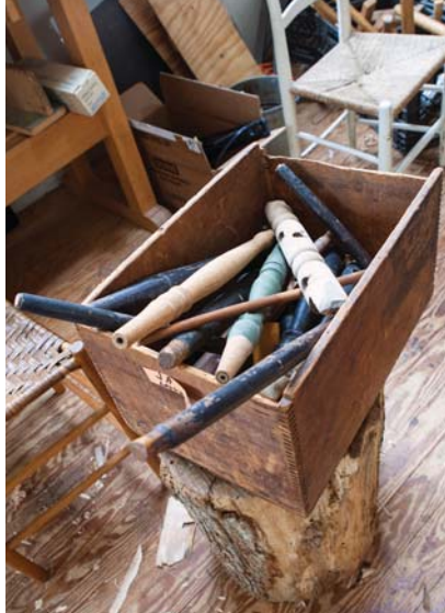
Broken chairs. Alexander's research has been informed by many bits of research, including looking at bits of chairs that have broken to learn why they failed.
