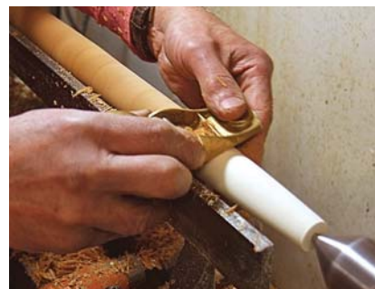
Foot joint. Use a small block plane to smooth the transition from holly to mahogany (mine is a Lie-Nielsen No. 102).
