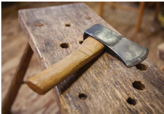
Almost homemade. Alexander enjoys making effective tools from inexpensive raw materials. Here, she made a useful side hatchet from a standard double-bevel hatchet.
