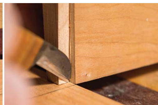
Narrow, then wide. First, mark the small end of the tail. (Note that your knife position is critical here, and be sure to mark both sides.) Then mark the wide end on the other edge of the pin board.
