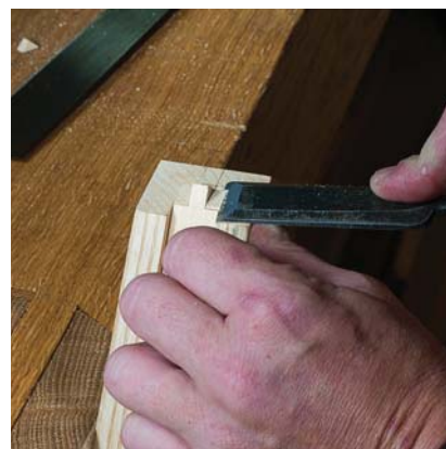
Pare to fit. Then pare the cheeks with a sharp paring chisel.
