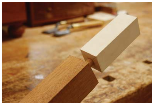
The drill. Prep, then drill the holly foot blanks to slip over the mahogany leg tenons.
