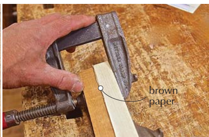
Leg prep. Before turning the legs, cut out a \frac{3}{4} " x 5\frac{1}{4} " section from the mahogany and glue in a piece of poplar, with heavy brown paper between the two species.
