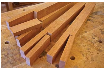
Leg prep. Before turning the legs, cut out a \frac{3}{4} " x 5\frac{1}{4} " section from the mahogany and glue in a piece of poplar, with heavy brown paper between the two species.
