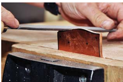
Smooth operator. After you've sawn the plates from the copper sheet, smooth the edges with a file.
