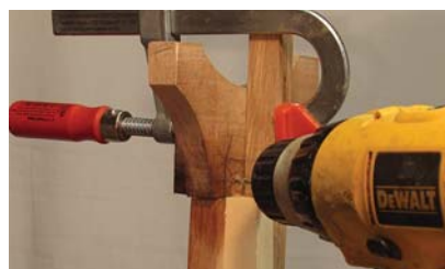
Drill. Mark the location of the stretchers onto the foot and drill pilot holes through the back of the foot and brace dado; this will help you locate screws to attach the side stretchers.
