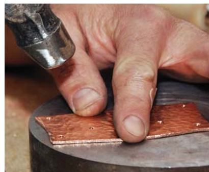
Border patrol. Use the flat face of the hammer to smooth the perimeter of the back plate, just a few 16ths in from the edge.
