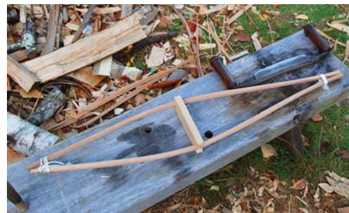
Space out. After limbering the wood for bending (either boiled water or a steambox will do), I tie the ends together and put a spacer in the middle, then let the parts dry.
