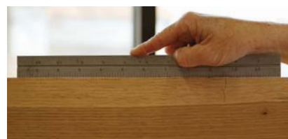
Straight edge. To confirm that the rule is straight along its length, show it to the edge of a jointed board. If there is light showing through, the rule is not acceptable.
