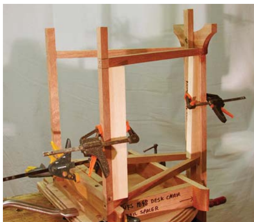
Assembly aids. Various fixtures and spacers hold the chair in alignment and help to locate parts during assembly.
