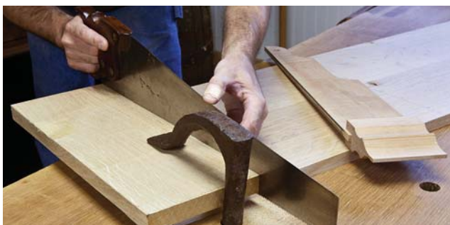
First wall. Clamp a batten on your layout line and saw the first wall of the dado. Press the sawplate against the batten to create a vertical cut.
