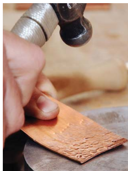
Tap dance. Many light taps with the ball end of a ball-peen hammer give the back plate its dimpled texture.
