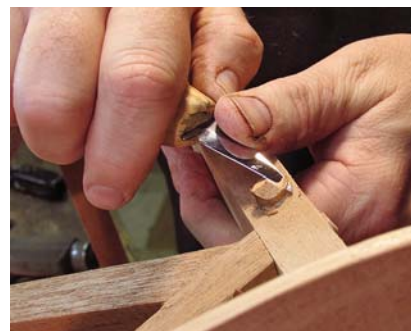
Faceted plugs. Shape the face of the wooden plugs with a carving knife.
