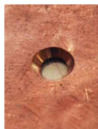
Border patrol. Use the flat face of the hammer to smooth the perimeter of the back plate, just a few 16ths in from the edge.
