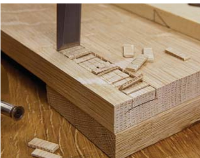
Chop & stop. The stopped groove for the interior rail is made the same way you made the dados for the shelves.
