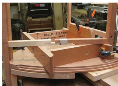
On the stick. The easiest way to measure the stretchers is to use an adjustable story stick.
