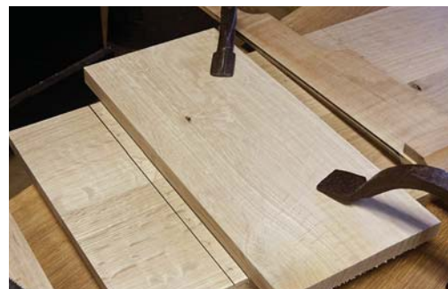
Second wall. Because of the set of the saw's teeth, clamp the batten so it covers your layout line for the second wall. This will ensure your dado isn't too loose.
