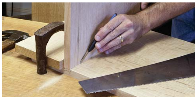
Don't measure. Use the mating shelf to strike the second wall of the dado. Use a pencil or knife to mark this wall.
