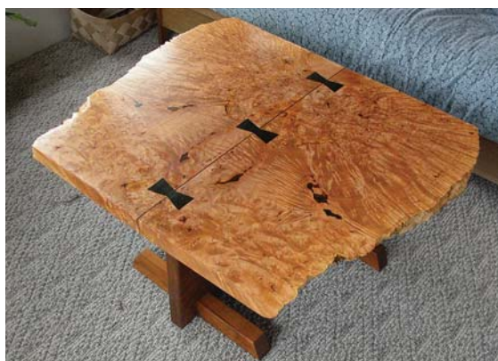
Butterfly aesthetics. Dumond uses contrasting woods as art elements in a coffee table with bookmatched burled maple slabs and ebony butterflies.
