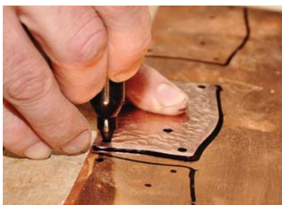
Trace the pattern. The back plates can be cut from the sheet copper using a variety of saws, from a band saw to a jeweler's saw
