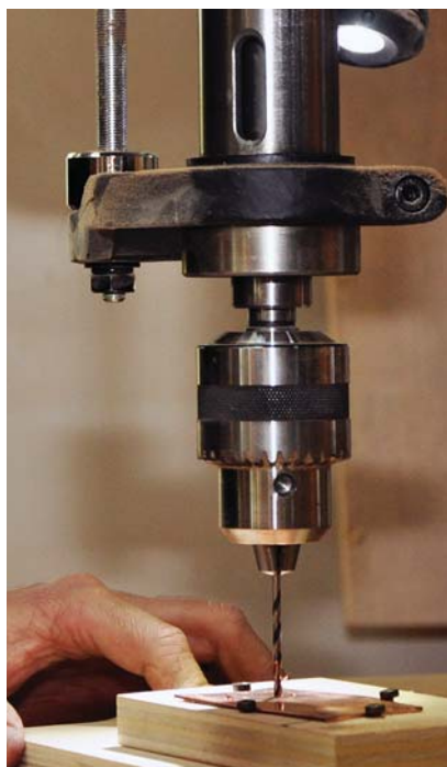
Drill safely. Secure the back plate when you drill the holes. Here I use angled screws to hold down the workpiece.
