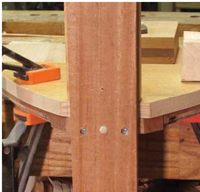
Back it up. Use the locator dowel to position the back onto the seat. Once the back is positioned correctly, drill pilot holes through the back and into the seat. Secure the back with screws.
