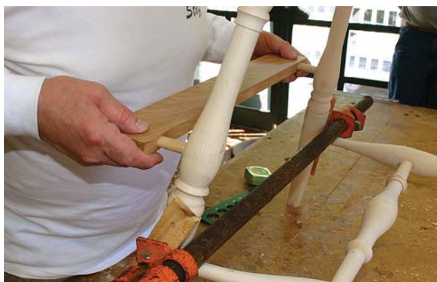
Squeeze play. A clamp across the legs allows the dowels to enter the holes in the footrest.
