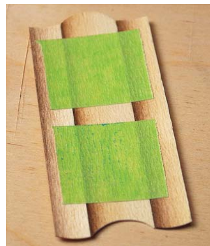
Stick together. Regular masking tape is sufficient to hold the sections tight as the workpiece is set into its recess.
