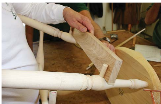
This to that. After placing the splayed dowels in the legs, hold the footrest against them and mark the location and the angle on the bottom face.
