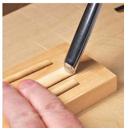
Burnt ends. Cut the concave curves after sand shading; if you cut before shading, the fragile points could be damaged.
