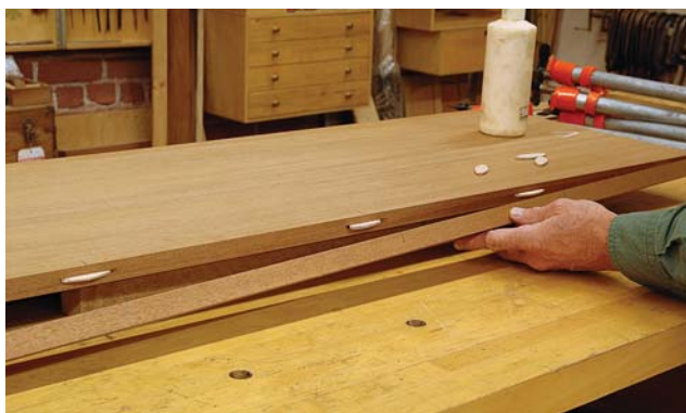
Alignment. Biscuits aren't needed to strengthen this joint, but they help keep the two legs and the panel aligned during assembly.
