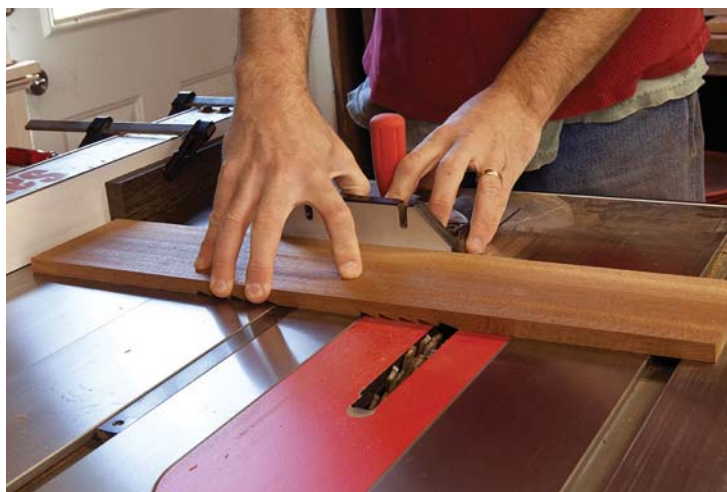
Easy birds. The birds' mouth shelf supports are cut simply and directly using a dado stack and a table saw. Note the stand-off block clamped to the fence.
