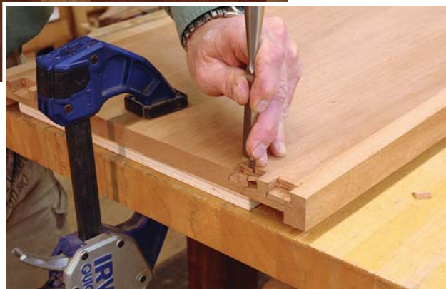
Saw then chop. Define the edges of the tail sockets with two saw cuts. Then chisel out the waste.
