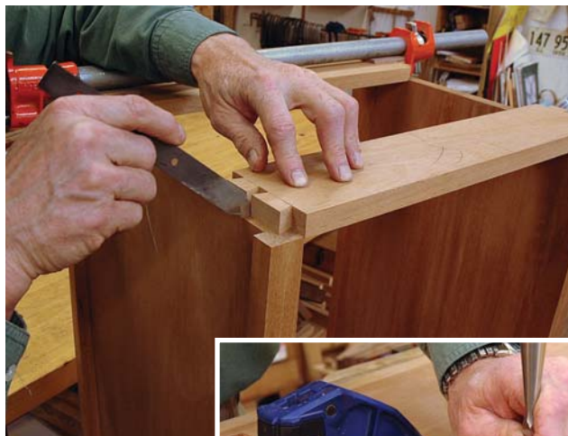
Tails on top. After adjusting the length of the top rails, cut the dovetails. With the rail in place, mark the sockets.
