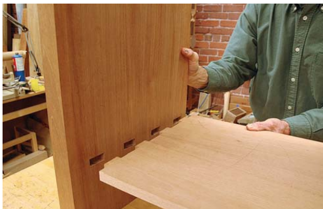
Trim & fit. Start at the front and work toward the back to fit the tenons in the bottom panel.
